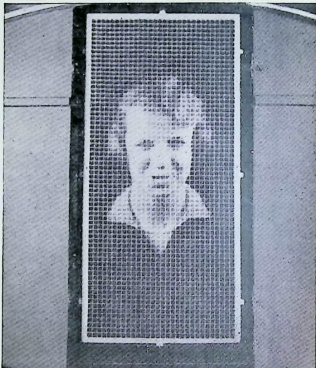
FIG. 2—This photograph gives an excellent impression of how the artist appeared on the Baird Lamp Screen when it was shown at Stockholm.
