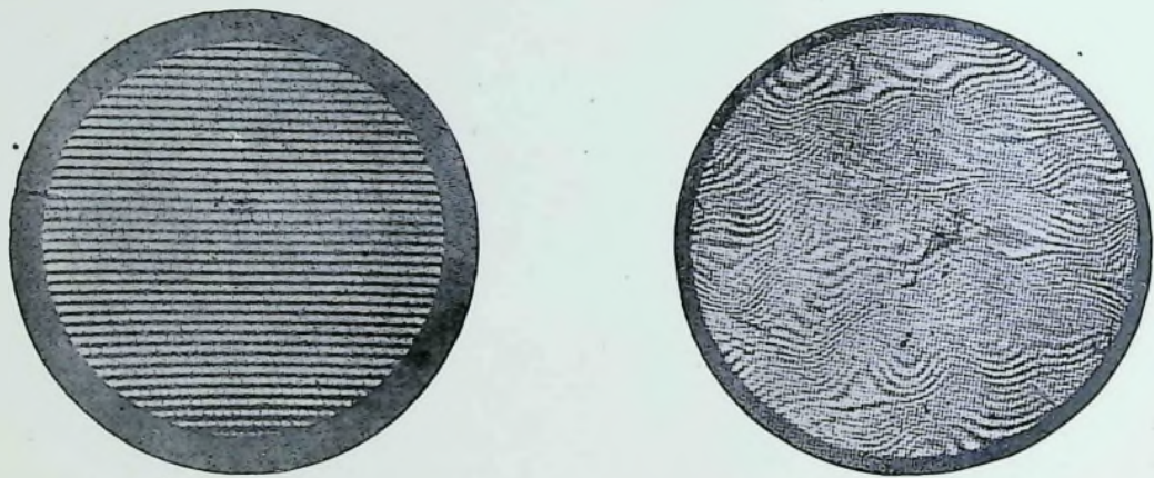
FIG. 19 - (on left) Quartz plate at rest (on right) in vibration
