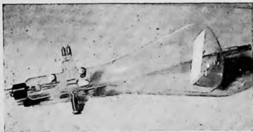
FIG. 28—Von Ardenne's latest cathode ray tube for variable speed television
