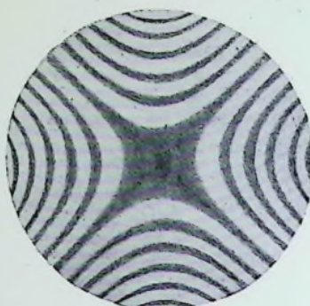
FIG. 11—Conoscopic image of uniaxial crystal cut parallel to axis
