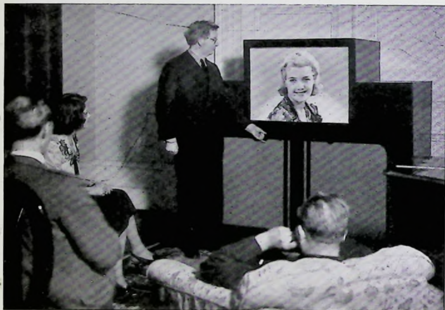
Mr. Baird's 600 line colour televisor. The screen receives either 600 line colour pictures or by pressing a button the B.B.C. 405 line monochrome pictures. It measures 2' 6" x 2' 0". The set includes an automatic record-changing radiogram and an all-wave wireless receiver.
