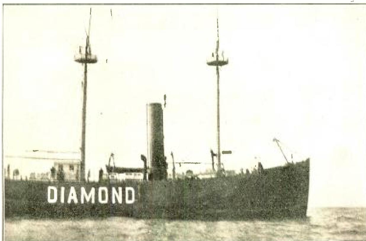
*Lightship No. 71, off Hatteras, showing the two-masted type of vessel whose stout steel hull can withstand the heaviest pounding of the seas*
