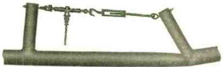
This cut, reproduced from a photograph of a test made to demonstrate the superiority of the Interlock Weld (the branch on the left) over the ordinary butt weld (the branch on the right), speaks for itself.
