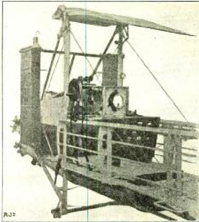
*Fig. 9.—Wireless set mounted on aeroplane*
