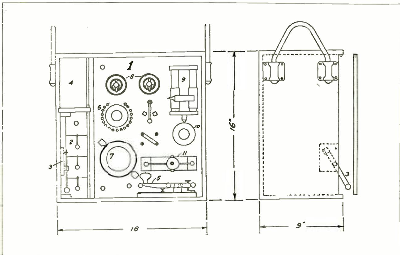
Fig. 3.—(1) Receiver, (2) Batteries, (3) Battery cutout, (4) Telephones, (5) Manipulating key, (6) Aerial tuning inductance, (7) Aerial tuning condenser, (8) Crystal holders, (9) Valve tuning condenser, (10) Intensifier, (11) Potentiometer
