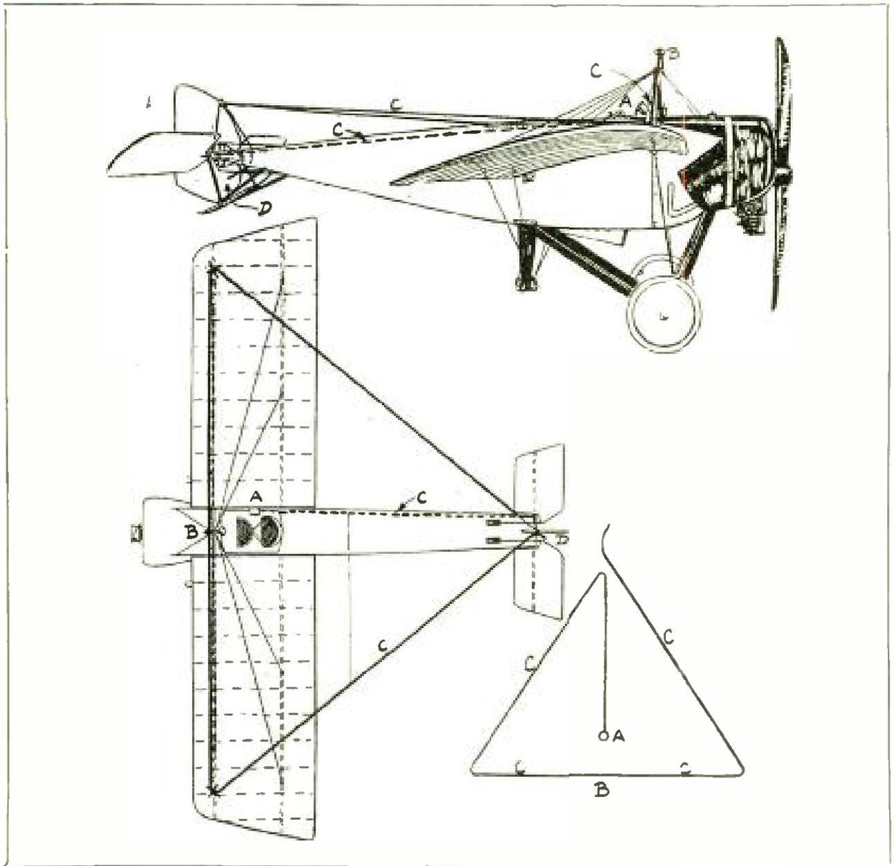
*Method of installing aerial on monoplanes used by French and Belgians in war*
