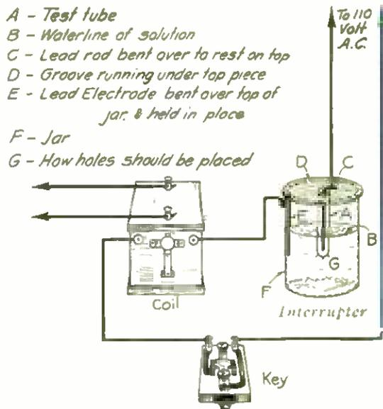
Primary Circuit Using Interrupter
