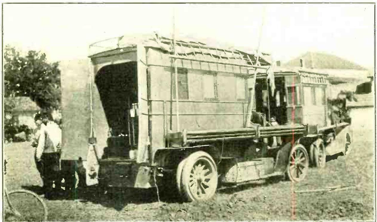
*French field wireless tractors used effectively as "mother stations" to communicate with the light portable sets*
