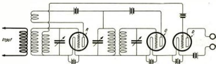
Figure 1—Method of varying the plate voltage coupled into the plate circuit. In this arrangement a third tube acts as a detector
