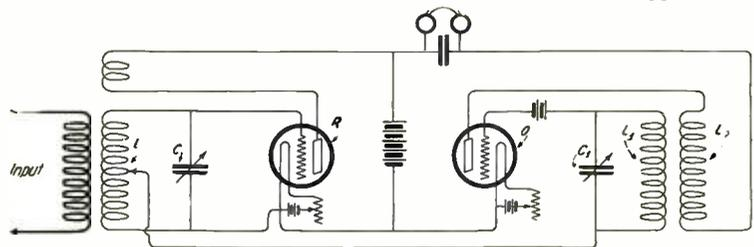
Figure 4—Shows how the oscillating tube is made to perform the additional function of a detector
