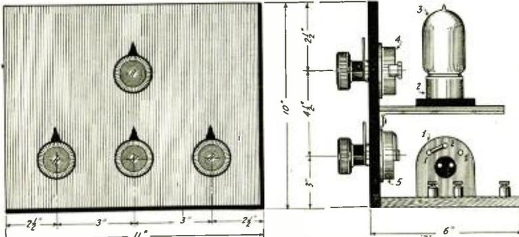
Figure 5A—Constructional dimensions of the radio frequency amplifier panel. 1—UV 1714 R.F. Amplifying Transformer; 2—Radio Corp. UR 542 Tube Socket; 3—Radiotrons—UV 201; 4—A-Battery Potentiometer—PR 536; 5—Filament Rheostats
