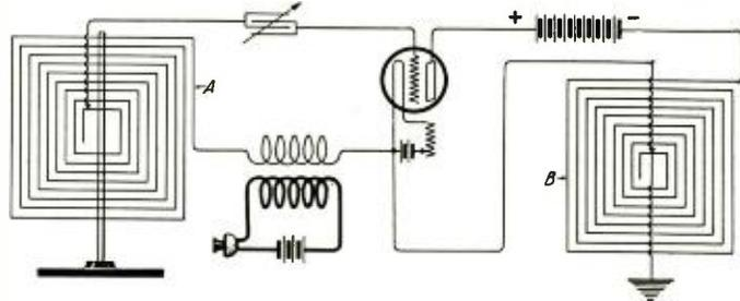
Circuit showing coupling coils used as the antenna
