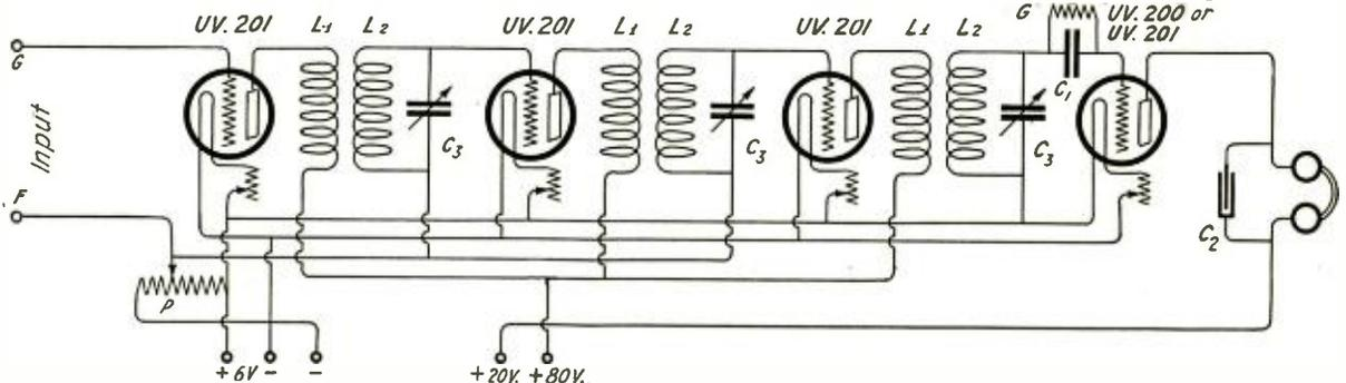
Figure 2—R.F. amplifier (tuned grid type) and detector.  $L_1, L_2$ —Coils coupled to each other.  $C_1$ —.0025 mf. grid condenser.  $C_2$ —.002 mf. phone condenser.  $G$ —2-megohm grid leak.  $C_3$ —.0005 mf. max. var. condenser.  $P$ —Potentiometer
