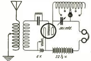
Ans. 1. Suggest that you employ the tuned plate circuit as shown. Wind a tube 10 inches in length by 3 inches wide with about eight inches of No. 24 D.C.C. taking a tap off every inch. Connect as shown.
