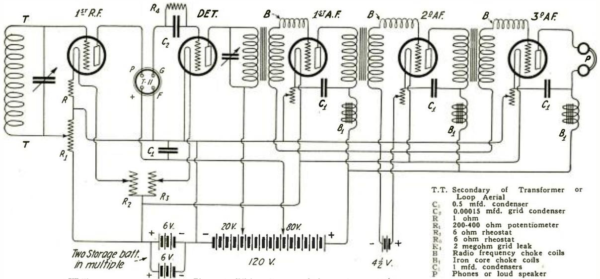
Figure 1—Wiring diagram of the maximum receiver
