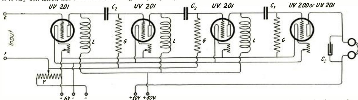
Figure 1—3-stage R.F. amplifier (choke coil coupling) and detector. L—Choke coils.  $C_1$ —.00025 mfd. grid condenser.  $C_2$ —.002 mfd. phone condenser. G—2-megohm grid leaks. P—Potentiometer.
