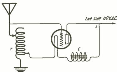
Hook-up for use of A.C. on filament and plate
