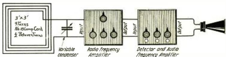
Figure 4—Combination of loop receiver with R.F. and A.F. amplifiers
