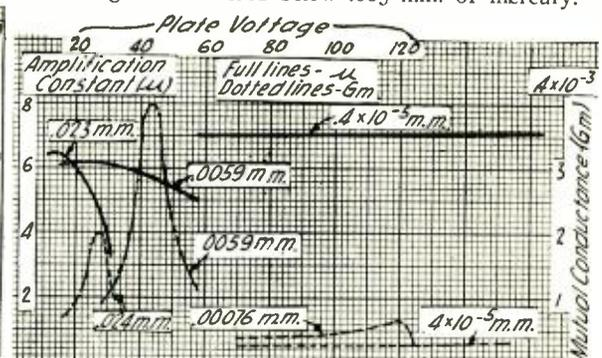
Figure 3—Amplification and conductance under varying plate voltages for different pressures
