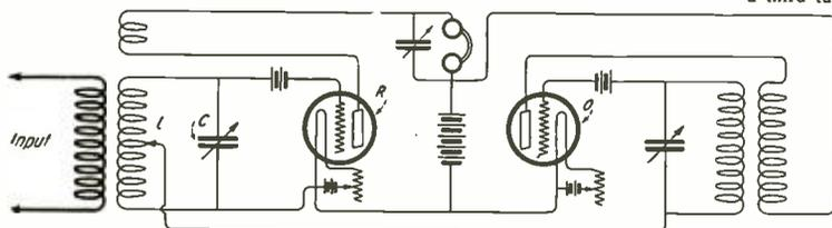
Figure 2—Manner in which the variation is introduced into the positive resistance of the tuned circuit. This is done by means of an oscillating tube O, the grid circuit of which is connected through the tuned circuit LC of the amplifying tube R
