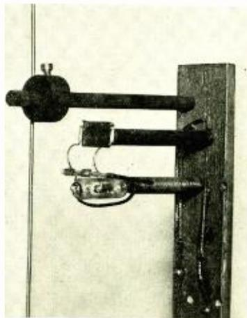
1-Meter transmitter used in the demonstration of directional radio. Transmitters of several hundred watts have been successfully used in tests of directional radio by reflectors on wavelengths between 1 and 15 meters
