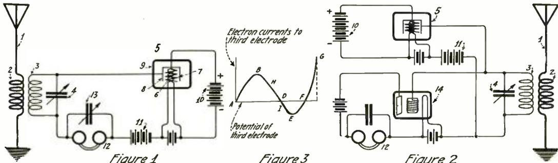
Hook-up to secure increased amplification and characteristic curve of the circuit
