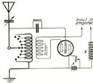
The hook-up used in the short-wave receiver at Oahu, H. T., for reception of Pacific Coast amateur signals
