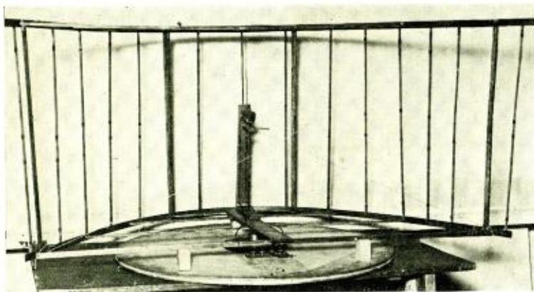
The semi-circular or "reflector" antenna used in the demonstration by Mr. Marconi. The signals at the receiver varied in intensity as the waves were directed at, or away from the receiver
