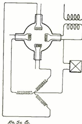
The rectifier for three-phase current
