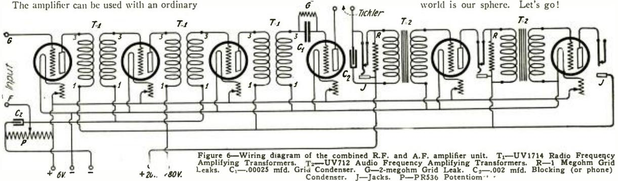
short wave regenerative receiver. The terminals of the receiver, usually connected to the detector, are led to the input of the amplifier. The plate variometer is connected to the tickler terminals in the plate circuit of the detector tube. The operation is no more difficult than that of the ordinary regenerative receiver, only one additional control, the potentiometer, being added.
