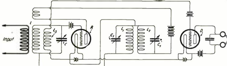
Figure 3—Manner in which simultaneous variation in both positive and negative resistances is obtained. This is accomplished by providing the amplifying tube R with a second feed back circuit  $L_1 C_1$  and  $L_2 C_2$ , adjusted to oscillate at some lower frequency
