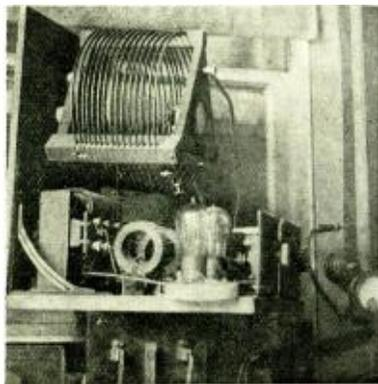
Self-rectification 10-watt C.W. set of 2OM station which has covered remarkable distances considering the receiver used
