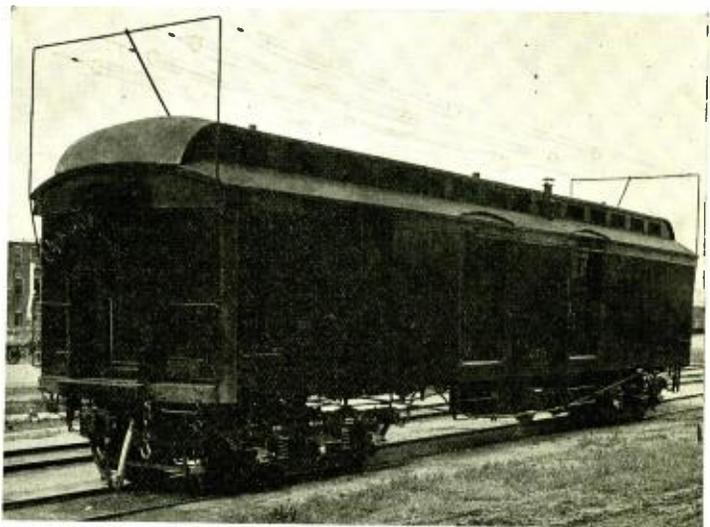
Car showing antenna designed by Earl Hull, operator at WKY
