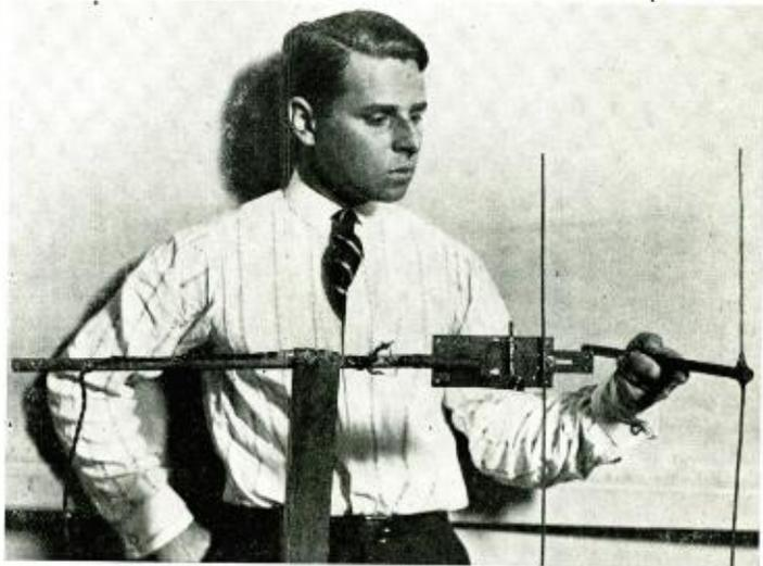
When another "antenna" or coil of wire, the period of which was the same as that of the transmitter, was placed in front of the receiving antenna, the signals entirely disappeared, illustrating very clearly the principle of absorption
