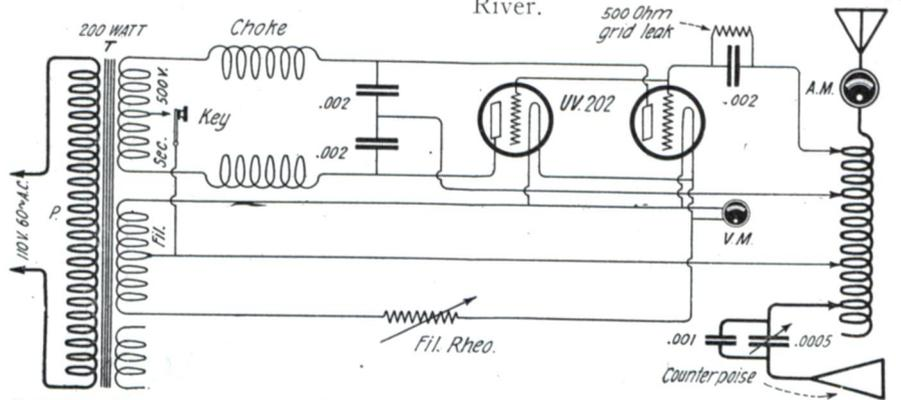
Full wave self-rectified 10-watt C.W. inductance 15 turns edgewise wound copper ribbon, 10 inches diameter—counterpoise alone used for ground as described
