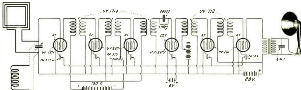
Figure 1—Hook-up of the R.F.-A.F. amplifier
