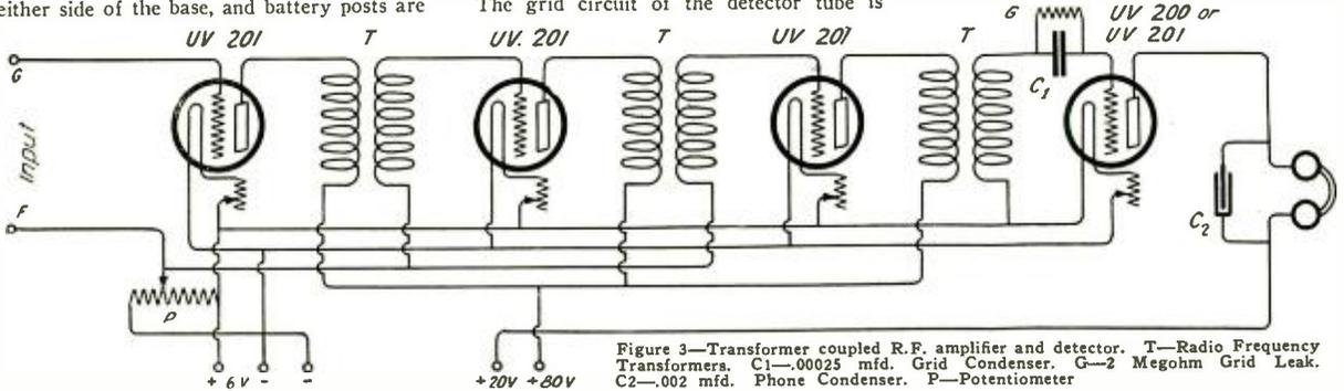
Figure 3—Transformer coupled R.F. amplifier and detector. T—Radio Frequency Transformers. C1—.00025 mfd. Grid Condenser. G—2 Megohm Grid Leak. C2—.002 mfd. Phone Condenser. P—Potentiometer
