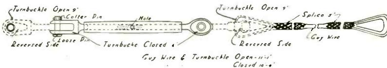
Until our supply is exhausted, we are offering the above Guy Wires for Antenna Construction. The turnbuckle is forged and machined and the wire twisted and tinned 5/32 inch diameter.
