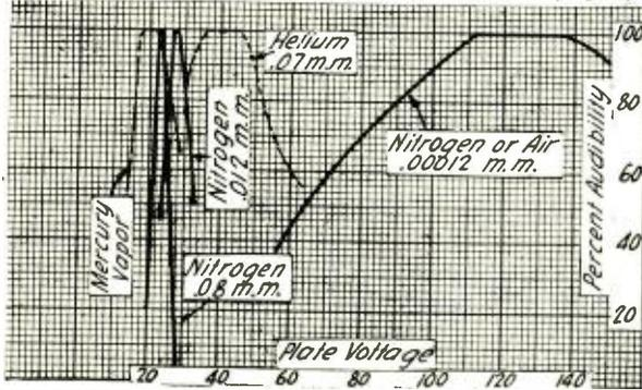
Figure 2—Effect of various gases on critical adjustment of voltage
