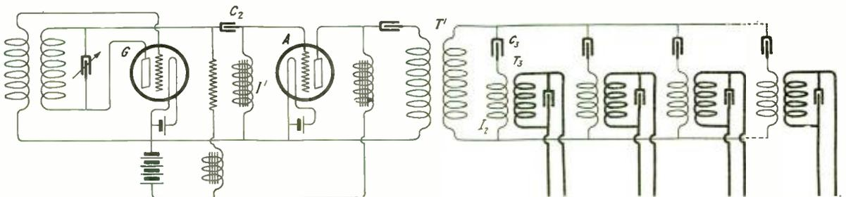
Figure 2—Circuit diagram of the harmonic generator
