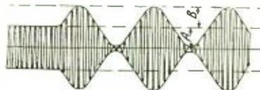
Figure 3—Equal upward and downward modulation  $A=B$
