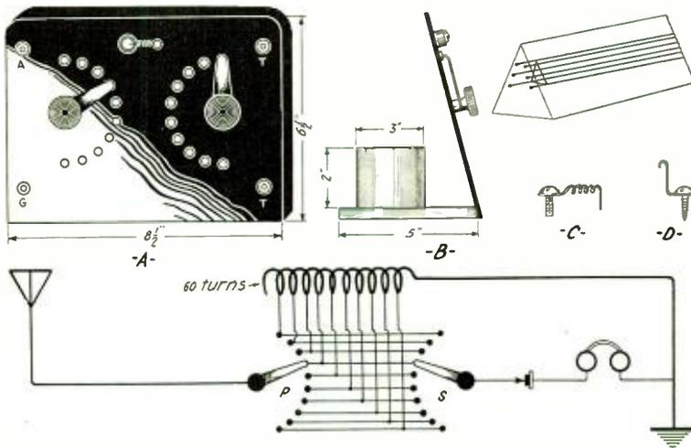
Simple and ingenious crystal tuner and detector with triangular cage-type antenna strung inside the gable roof of the house
