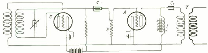
Fig. 1. Constant output oscillation generator
