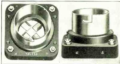
Our No. 666 positive contact socket has brass receptacle, nickel plated, moulded into bakelite socket. Allowance made in diameter of receptacle for the varying diameters of tube bases. Socket contacts insure certain and positive contact with the end and side of prongs of bulb. As socket is moved in the notch a pressure is immediately exerted on the side of the phosphor bronze contacts.
