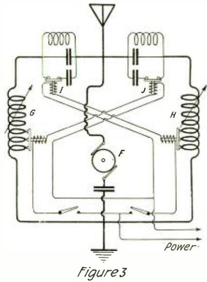
Wiring diagram of the system of duplex transmission on a single aerial and ground
