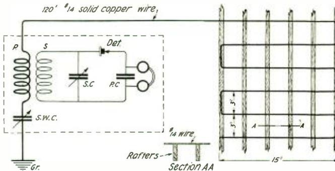
How the antenna was stretched over the rafters
