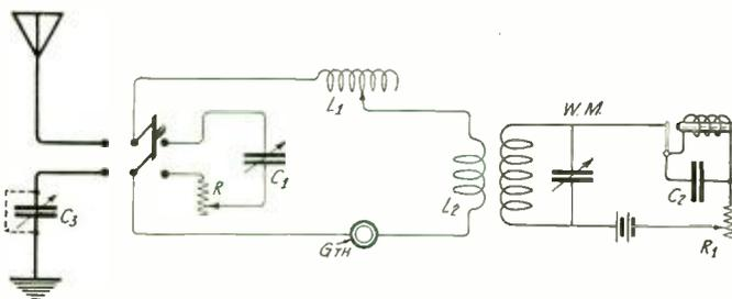
Figure 1. Diagram for testing antenna resistance
