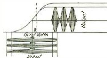
Figure 8—Amplifier distortion
