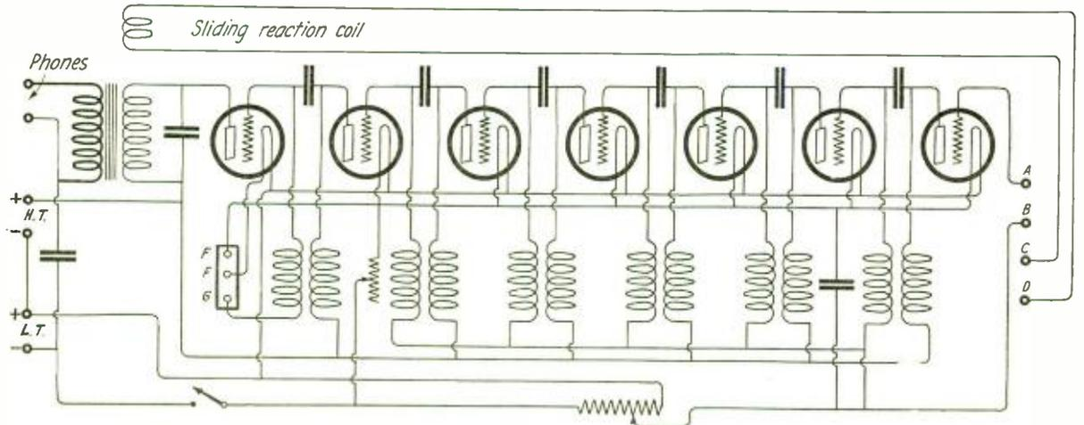
Fig. 5. Seven-tube amplifier especially suited for long-wave trans-Atlantic reception
