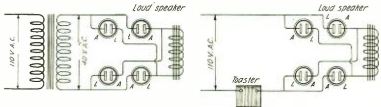
Circuit diagrams of the rectifiers for 60-cycle A.C.
