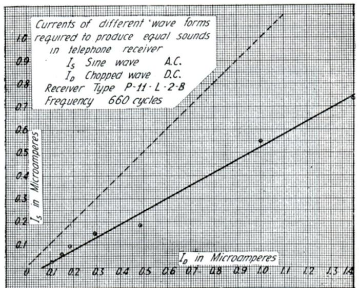
Figures 6 and 7—Graphs showing currents of different wave forms required to produce equal sounds
