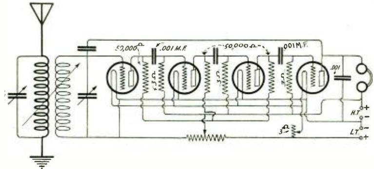
Figure 7. Resistance-capacity coupled amplifier system
