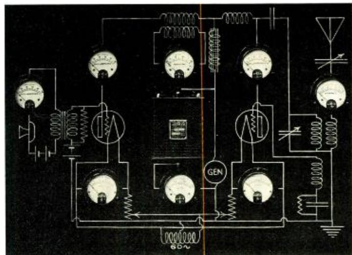
Diagram of a continuous wave transmitter, completely equipped with indicating instruments exhibited by the Jewell Instrument Company at the recent Chicago Radio Show, held in the Leiter Building
