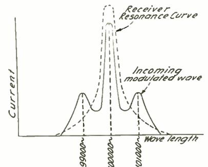
Figure 9—Distortion of modulated wave due to low receiver decrement
