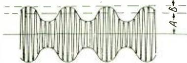
Figure 1—P. r cent modulation is  $B/A \times 100$
