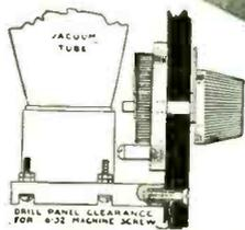
This illustration shows an easy, compact and efficient method of panel mounting FADA rheostats and sockets.
