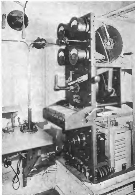
The RCA type SE-1060, 1 K.W. spark transmitter used in regular service
