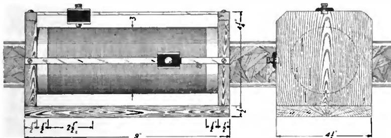
Constructional details of the two-slide tuner
