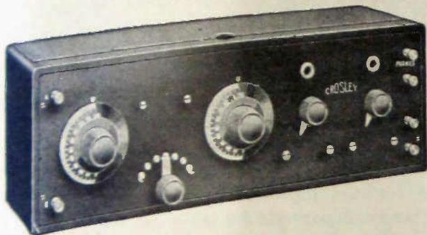
CROSLY RECEIVER MODEL VI. This set consists of one stage of Tuned Radio Frequency Amplification and Audion Detector. It is normally for use with head phones but is especially recommended to be used with any type of loud speaker. Additional amplification is unnecessary if head phones and horn are used in receiving local stations. Price, without phones, batteries or tubes .....\$30.00
