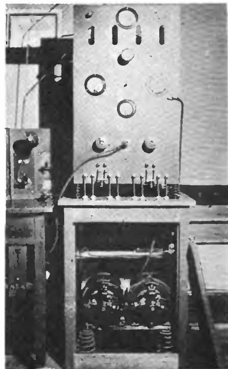
The transmitter with generator in the cabinet
