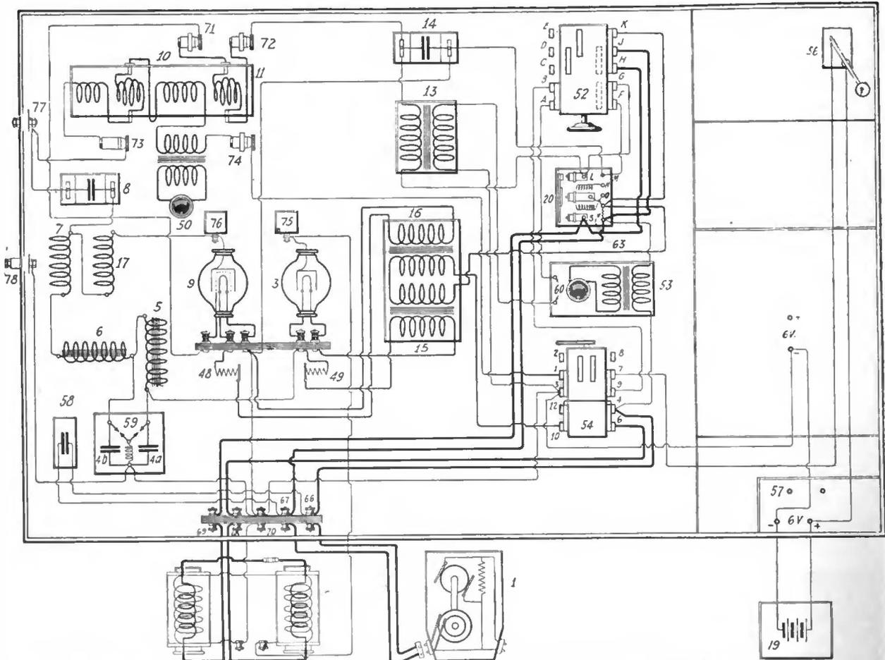
Circuit diagram of Marconi type YC-3 transmitter. The primary power circuit is shown in heavy lines and the speech circuit in thin lines. The microphone is connected to terminals 60
