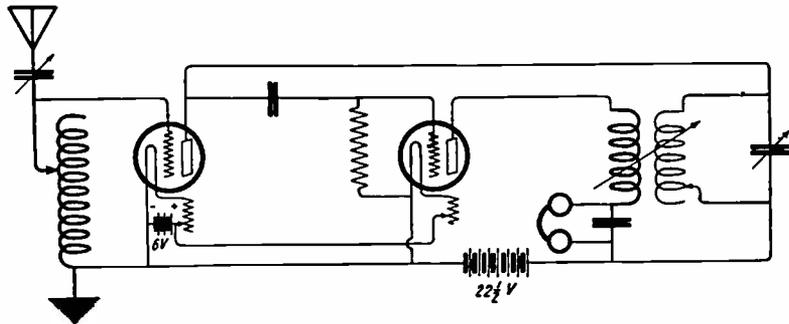
Receiver using a vario-coupler in the plate circuit
