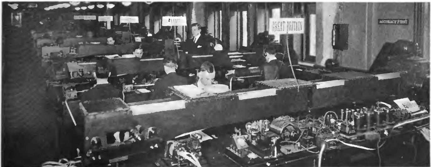
The great receiving room at 64 Broad Street hums with activity night and day, handling traffic at high speeds. Each table controls the complete circuit of a transmitter and receiver that works with a foreign country—transmitting on one side and receiving on the other. As the signs indicate, tables are devoted to service with Norway, France, Germany (2) and England (2)
