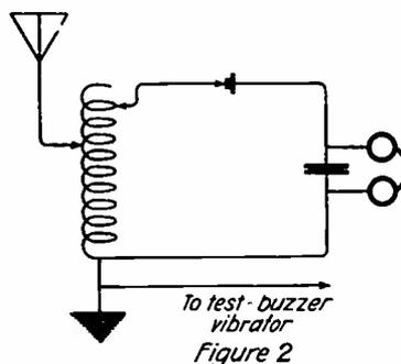
Diagram showing a double-slide tuner crystal set transformed into a regenerative tube set
