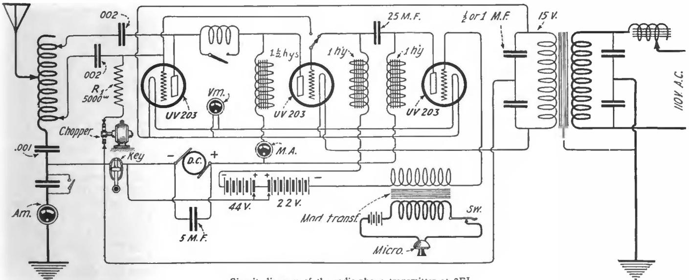
Circuit diagram of the radio-telephone transmitter at 2EL
