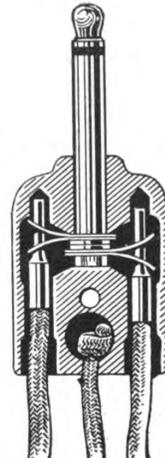
Interior of PACENT Universal Plug showing perfect insulation and spring terminals which insure perfect biting contact.
