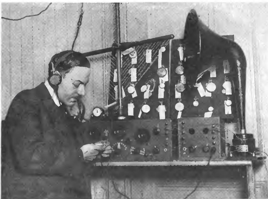
Simon Rimler, an American jeweler, has followed the precedent of his French brother craftsmen in installing a radio receiver for the purpose of securing the correct time by means of time signals. He listens to time signals from Arlington
