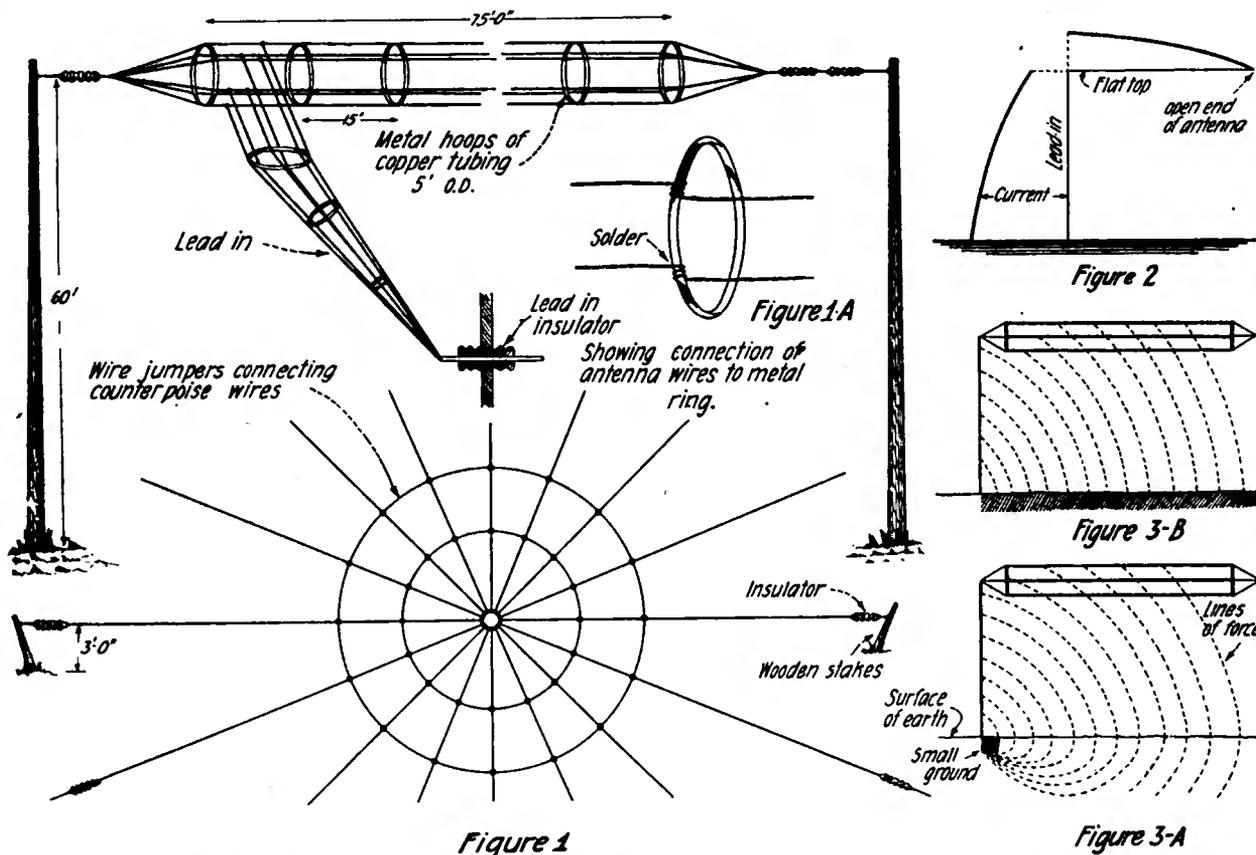
Figure 1—Six-wire cage antenna and counterpoise ground. Figure 2—Distribution of current along the antenna. Figure 3A—High current density and high resistance resulting from small ground. Figure 3B—Extended and uniform distribution of lines of force on large ground affords low resistance
