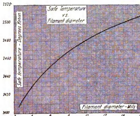
Figure 4—Safe temperatures for different filament sizes
