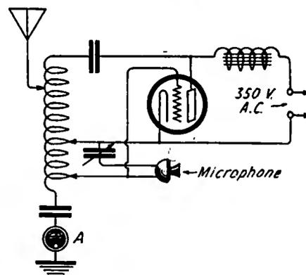
The voice is radiated a few meters above the carrier wave of the station. The modulation is reported as being of excellent quality with so little A.C. hum as to be practically negligible.
