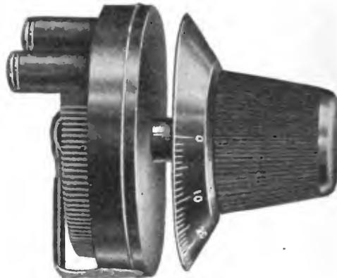
not only governs the filament, but also switches the plate circuit on and off. The usual connectors in the amplifier tube circuit
