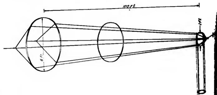
Constructional details of the cage antenna and details of the method of installation
