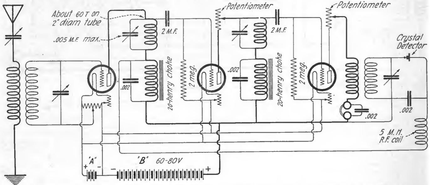
Figure 5—Reflex circuit using tuned plate circuit radio frequency amplifier and choke coils for audio frequency amplification—three stages r. f. and two stages a. f.—“Coto-coil” r. f. choke coils are suitable for use in place of the tuned circuit
