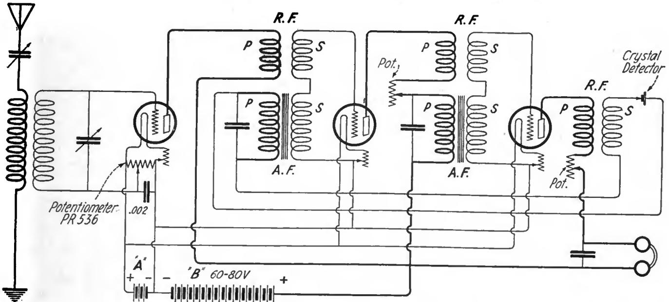
Figure 3—A three-tube reflex amplifier, containing three stages of r. f., crystal detector, and two stages a. f. amplification. Note use of resistances in plate circuit of last two tubes to prevent oscillation, instead of stabilizing potentiometer across the filaments as used in first tube
