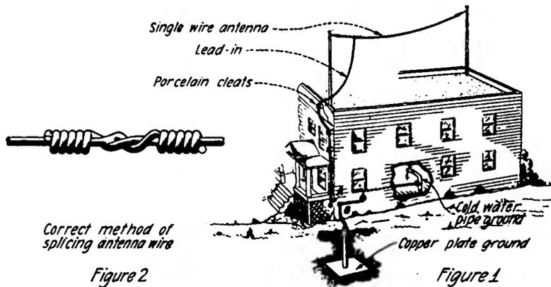
Figure 2 Correct method of splicing antenna wire
