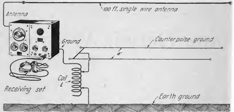
Figure 1—Combination of counterpoise and ground connected by a tapped coil to increase signal strength
