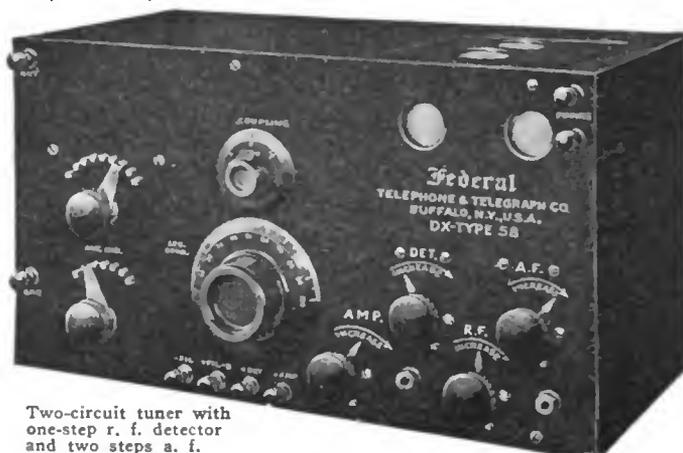
Two-circuit tuner with one-step r. f. detector and two steps a. f.
