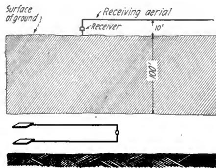
Figure 1—Relative position of transmitting and receiving apparatus for some of the tests
