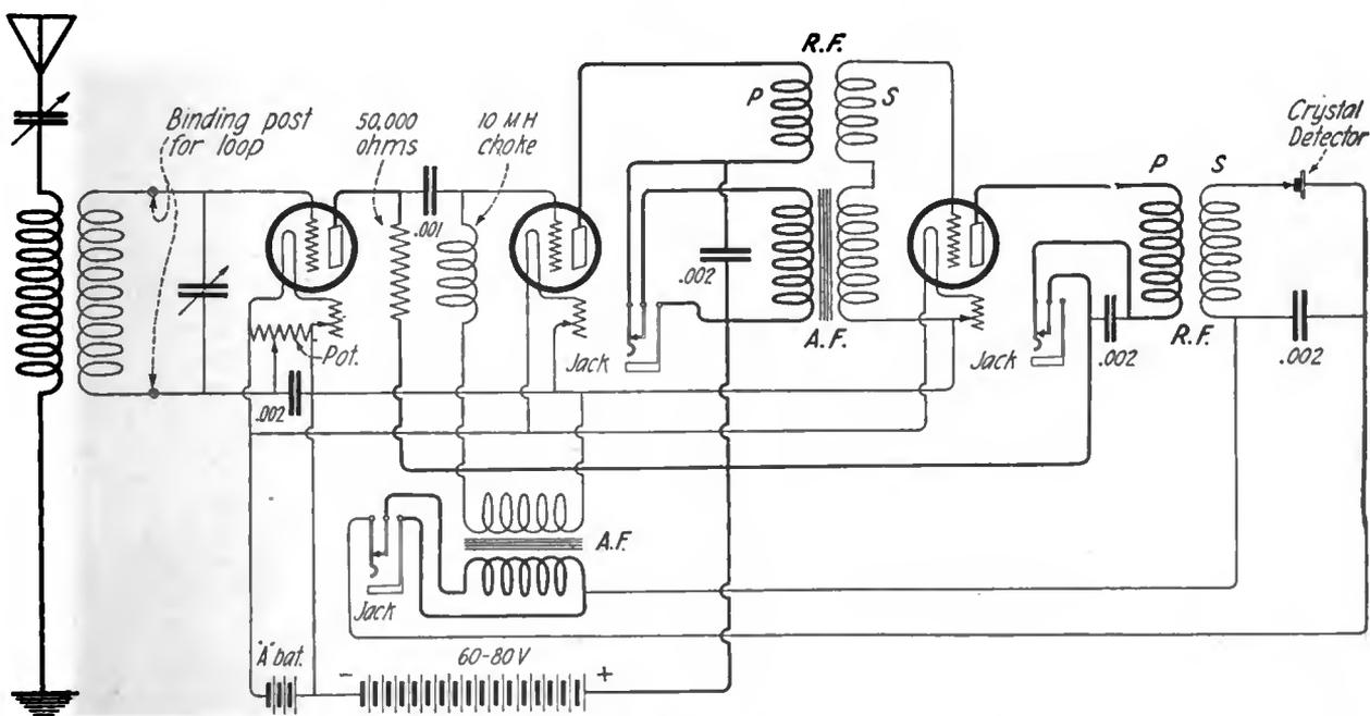
Figure 4—Circuit similar to that used in a commercial reflex amplifier. First r. f. stage is resistance coupled, then two transformer coupled r. f. stages with crystal detector and two stages of audio frequency. Jacks for phones or loud speaker on a. f. stages
