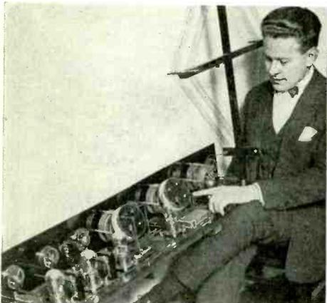
Mounting radio frequency transformers in tuned RF amplifiers at all sorts of peculiar angles seems to be quite a popular practice. Just why the special arrangement shown above was used is not clear, however, as the windings are in the same plane
