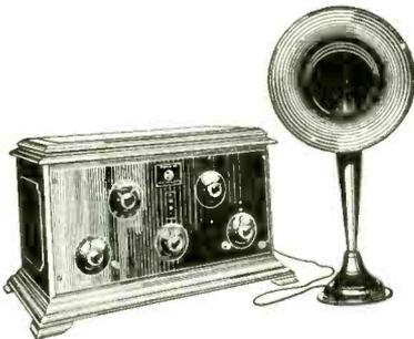
The Radiola VII is made up of two stages of transformer-coupled Radio frequency amplification, detector, and two stages of audio frequency amplification.
