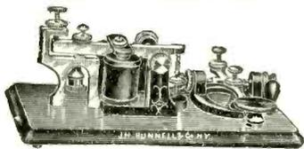
One dry cell is all that is required to operate this instrument.
