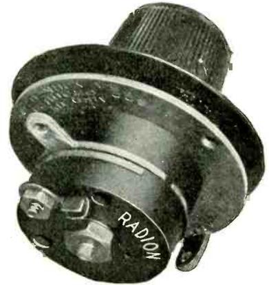
The manufacturers of the Amsco condenser have used Radion insulation in an endeavor to keep both the surface leakage and dielectric losses at a minimum.
