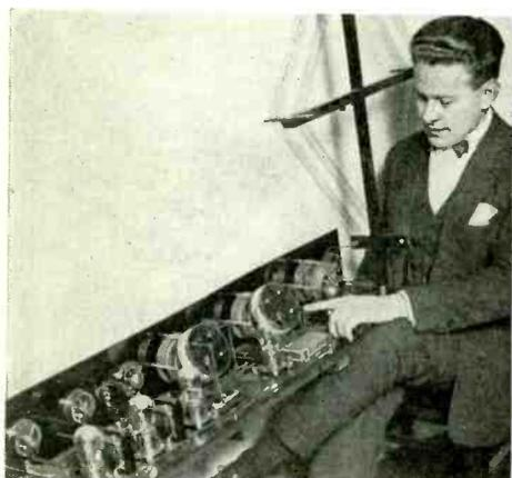
Mounting radio frequency transformers in tuned RF amplifiers at all sorts of peculiar angles seems to be quite a popular practice. Just why the special arrangement shown above was used is not clear, however, as the windings are in the same plane
