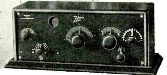
**Model 4R**—The new Zenith 4R "Long-Distance" Receiver-Amplifier comprises a complete three-circuit regenerative receiver of the feed-back type. It employs the Zenith regenerative circuit in combination with an *audion detector* and *three-stage* audio-frequency amplifier, all in one cabinet. Because of the unique Zenith "selector," unusual selectivity is accomplished without complication of adjustment.
