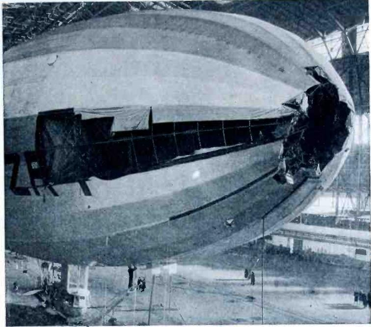
The Shenandoah in the hangar immediately after her return. The damaged bow reveals the third section within, on the left, which was nearly damaged. Had that section been destroyed, the ship would have met with disaster
