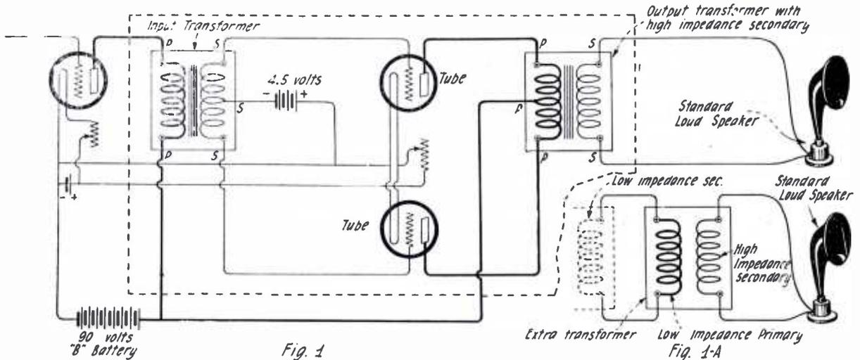
Fig. 1 Push-pull circuit connected to a high impedance loud speaker from the secondary winding of high impedance
