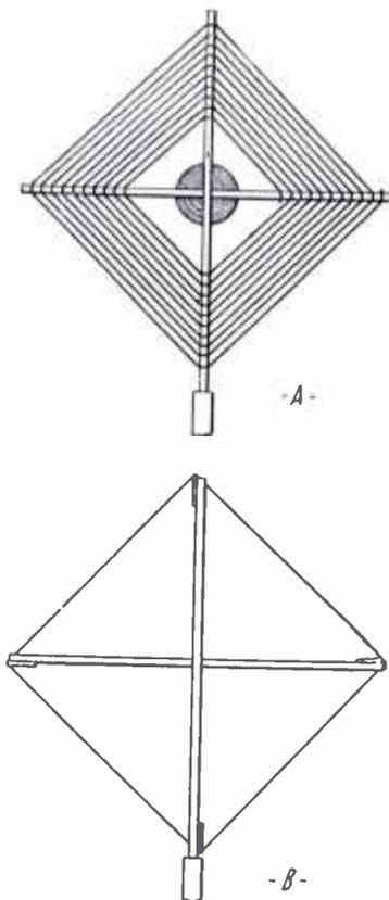
Figure 1—Square loop with oblique edges
