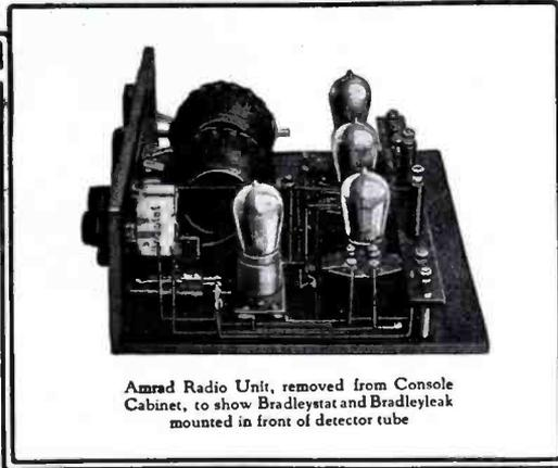
Amrad Radio Unit, removed from Console Cabinet, to show Bradleystat and Bradleyleak mounted in front of detector tube
