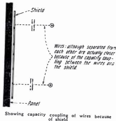
coupling between shield and instruments.
