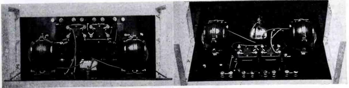
Top view—Through the use of straight direct connections run, in cambric tubing, wiring may be easily and quickly accomplished
