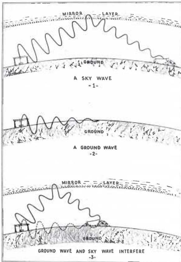
Action of reflected waves and ground waves
