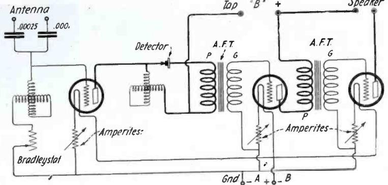
Circuit diagram of The Wireless Age three-tube receiver using one step of R. F. A., crystal detector and two steps of A. F. A.
