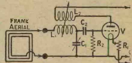
Fig. 2.—By slightly altering the receiver wiring the frame may be connected as shown here, the coil being used for obtaining reaction coupling. This diagram may be compared with that of Fig. 1.
