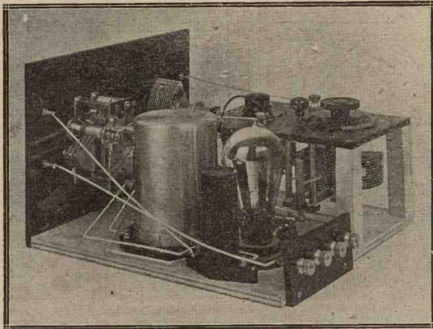
Care should be taken in placing the screened coil and choke coil to allow ample room for vibration of the valve.
