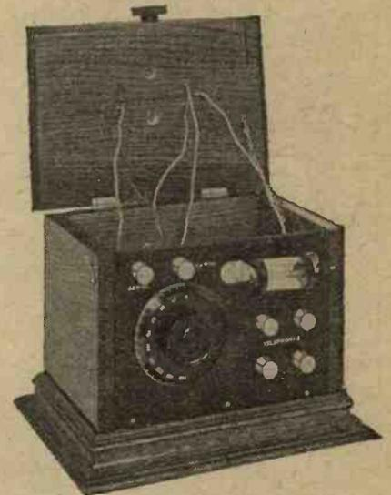
Holes are drilled in the lid of the cabinet to pass the leads to the coil holder.
