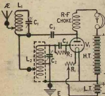
Fig. 1.—The earthed screen of the tuning coil is shown by the dotted line in this diagram.
