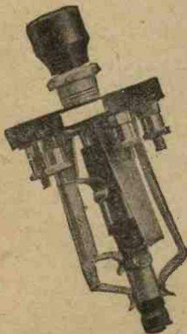
*A typical multi-contact push-pull switch. Only the knob and securing nut appear on the front of the panel.*
