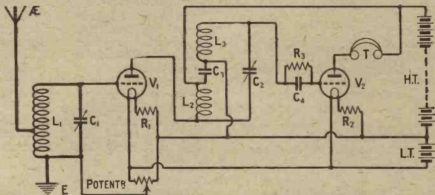
Fig. 2.—Suitable values for the components in this circuit are indicated in the article. A shunting condenser may be included between earth and L.T. negative across the potentiometer winding.
