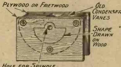
Fig. 2.—This method of cutting out the vanes for small condensers ensures that the finished vanes are flat.
