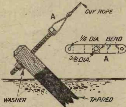
Fig. 4. A convenient form of stay tightener can readily be constructed in the manner indicated here.
