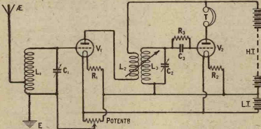
Fig. 1.—With this circuit varying degrees of selectivity may be obtained by altering the coupling between L2 and L3.
