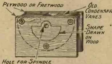
Fig. 2.—This method of cutting out the vanes for small condensers ensures that the finished vanes are flat.
