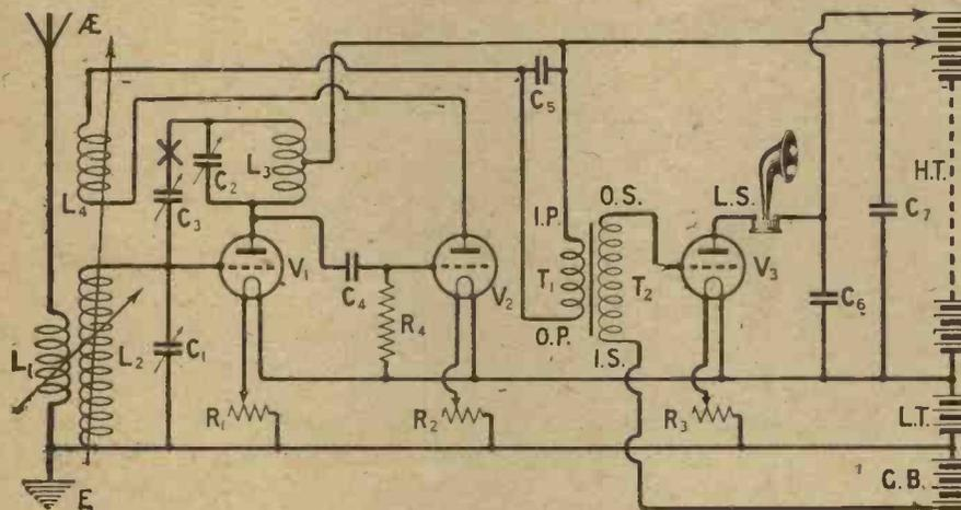
Fig. 1.—A fixed condenser connected in circuit at the point X will often cure noises due to trouble in the neutralising condenser C3.
