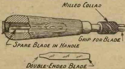
Fig. 1.—This neat type of screwdriver with blades of different sizes should prove valuable in any workshop.
