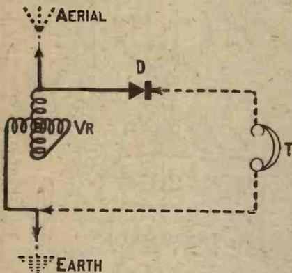
Fig. 1.—The two matchbox windings form the tuning variometer.
