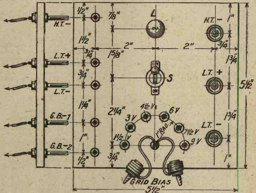
Fig. 2.—From the dimensions given here the panel may be marked out for drilling.
