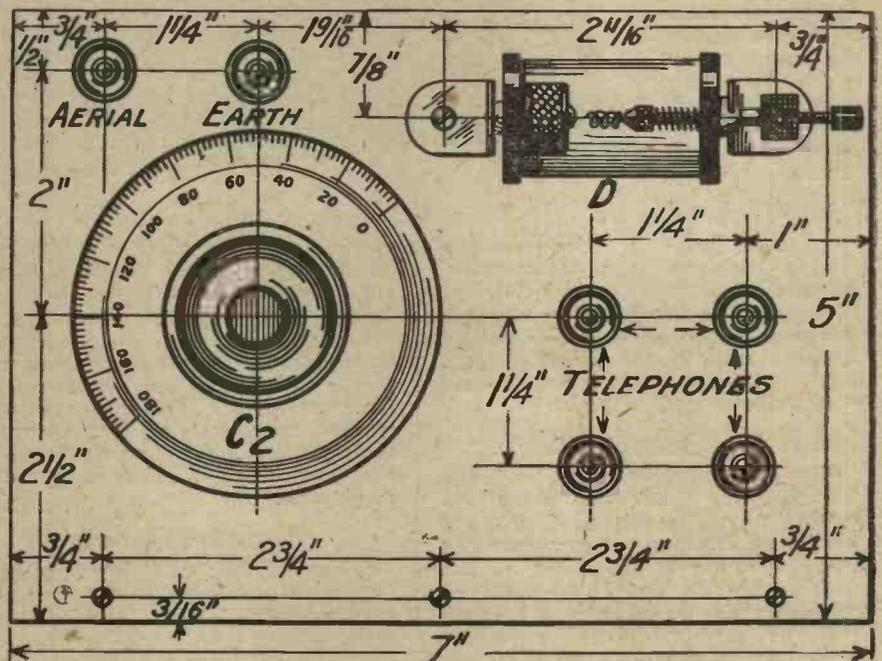
Fig. 2.—Those who use the components recommended will be able to take the necessary drilling dimensions from this diagram. Blueprint No. C1061A.
