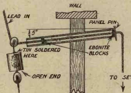
Fig. 5. This lead-in arrangement will prevent rain from running down the lead direct on to the wall, with consequent loss of efficiency.
