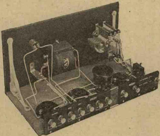
The wiring of the on-and-off switch should be left until the other connections have been completed.
