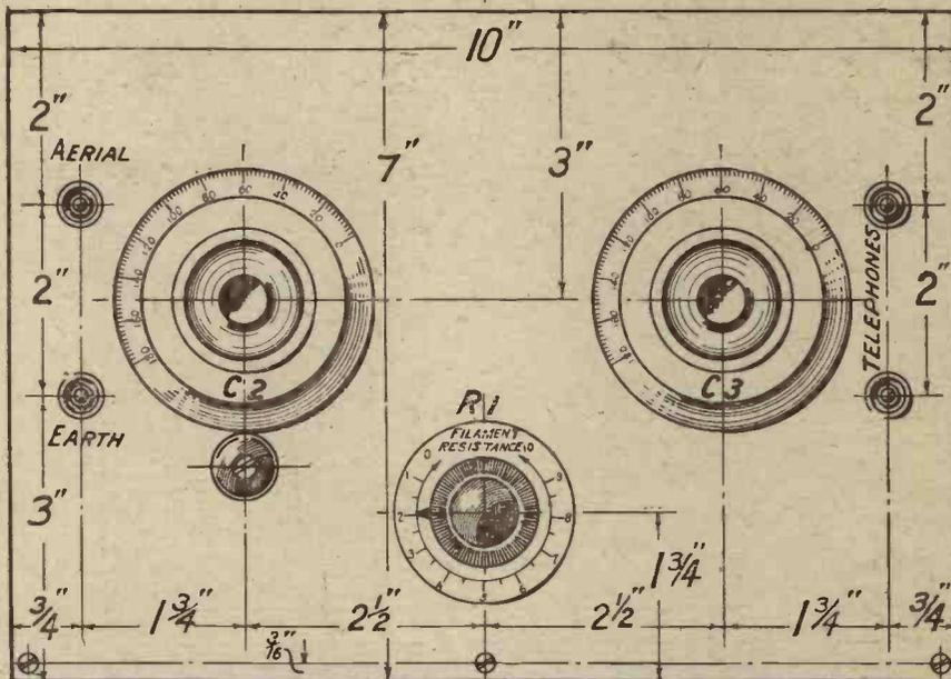
Fig. 2.—The condenser on the left tunes the grid circuit, while that on the right is for reaction. Drilling dimensions may be taken from this diagram, and blueprint No. C1060A is also available.
