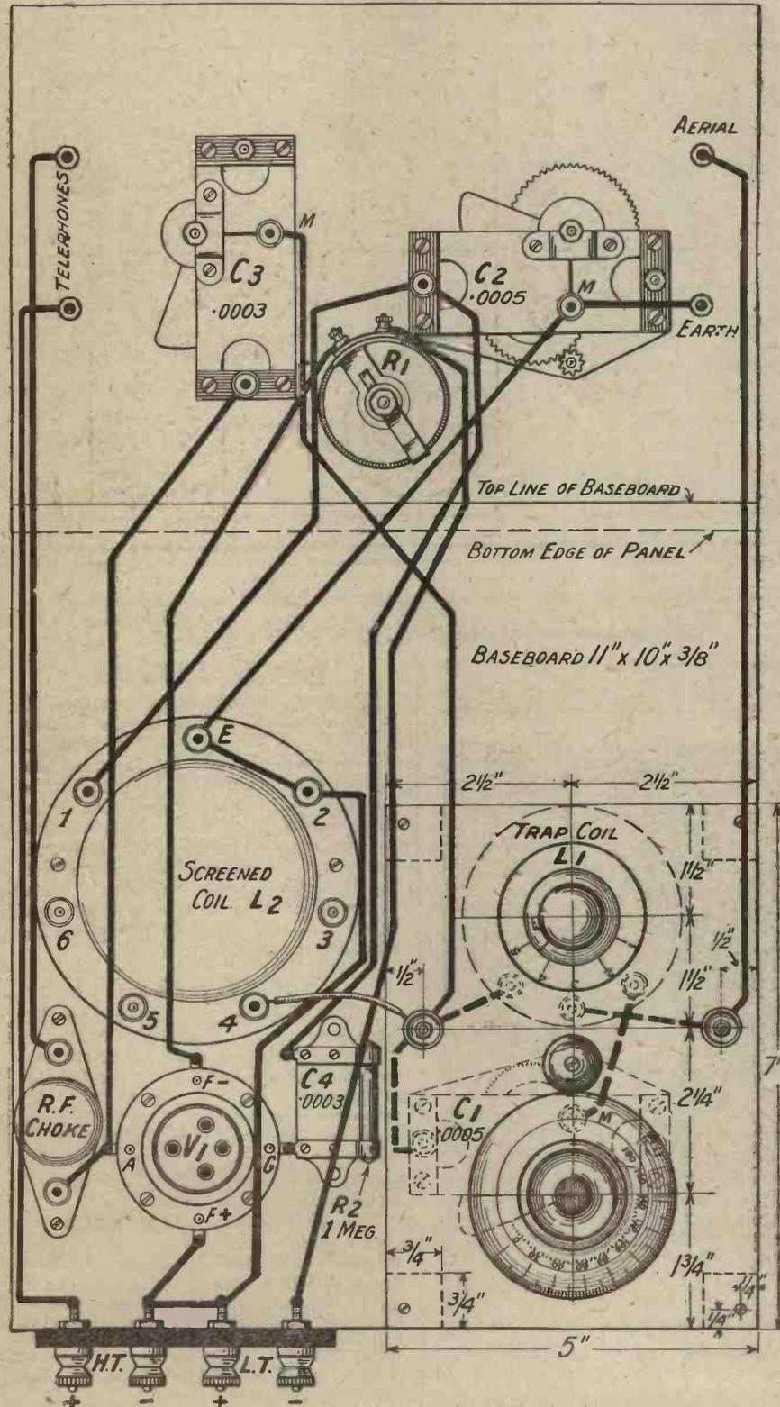
Fig. 3.—The layout of the components given here should be carefully followed in assembling the set. Blueprint No. C1060B is also obtainable with the aid of the Coupon in this issue.
