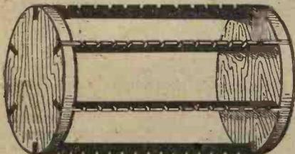
Fig. 3.—The notches in a former of this kind may be made with a hacksaw if the spacing is fairly wide.
