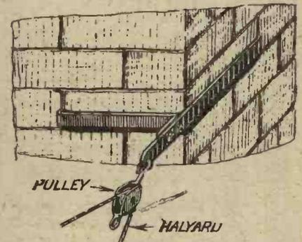
Fig. 2. The method of attaching to a chimney the bracket illustrated in Fig. 1 is shown here.
