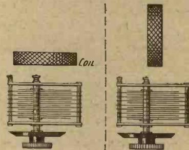
*Fig. 2.—A coil should not be fixed so that it has in its field a large mass of metal. The position shown on the right is more satisfactory.*
