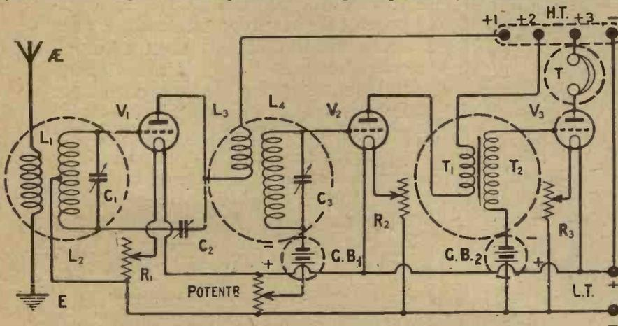
Fig. 1.—Excessive resistance is especially undesirable in the parts of this circuit enclosed within the dotted circles.
