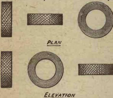
Fig. 1.—Undesirable coupling effects between coils may be minimised by placing them in the positions shown here.
