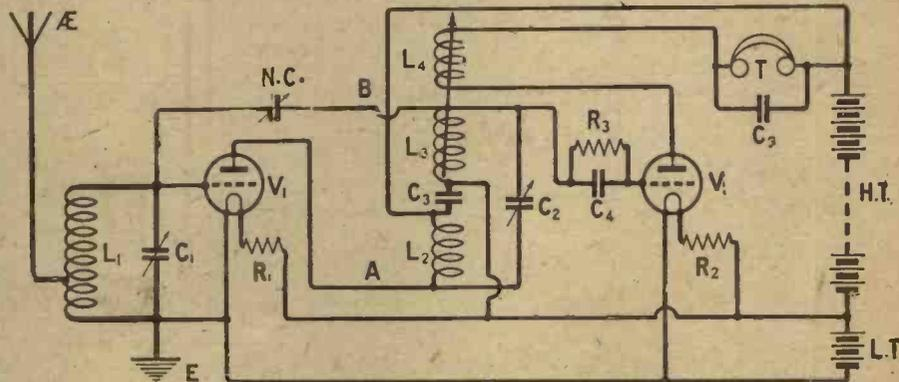
Fig. 3.—This circuit, a further development of that given in Fig. 2, incorporates a neutralised H.F. valve and a reaction coupling coil  $L_4$ .
