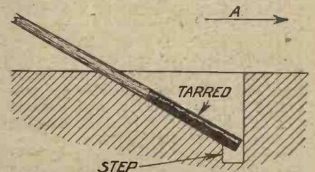
Fig. 3. This shape of hole will greatly simplify the erection of an aerial mast. The base of the mast may be tarred to give it a longer useful life.
