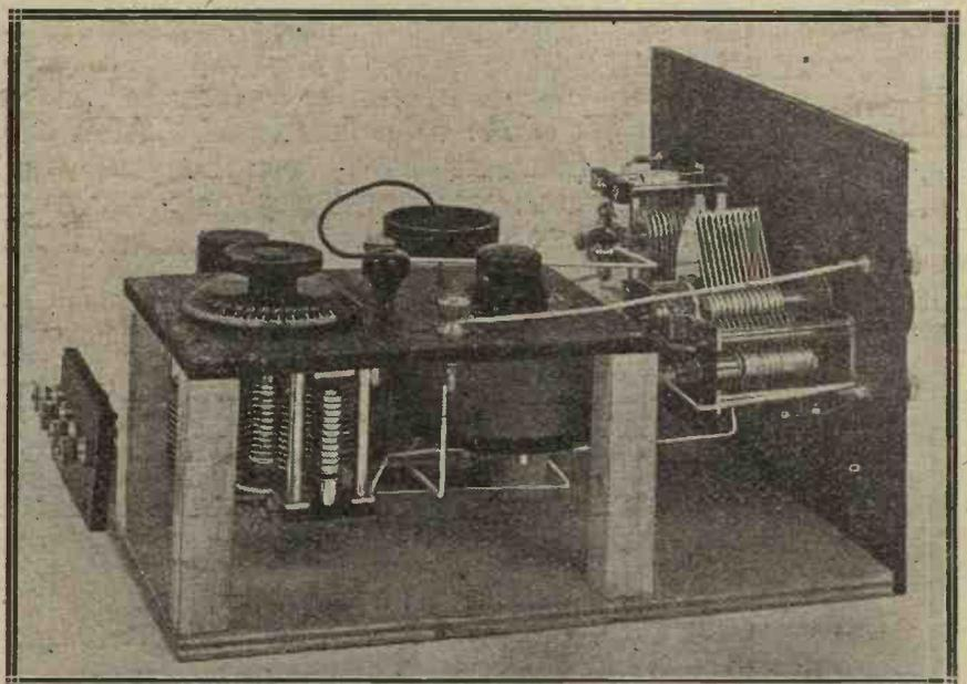
A separate panel, supported on four wooden legs, carries the trap circuit tapped coil and variable condenser.
