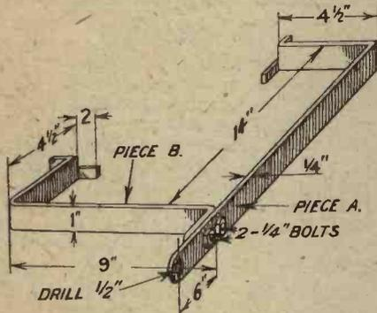
Fig. 1. Showing how a strong chimney bracket may be constructed.
