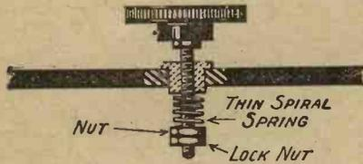
Fig. 5.—Showing how an intermittent spindle contact may be put right.
