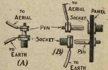
Fig. 1.—With this device it is impossible to connect aerial and earth the wrong way round.
