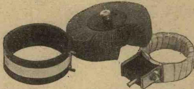
Three examples of modern coils (left to right), single-layer, toroid and standard plug-in.
