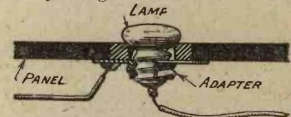
Fig. 4.—The lead on the right in this diagram may be soldered direct to the lamp as shown, or alternatively a spring contact may be devised.
