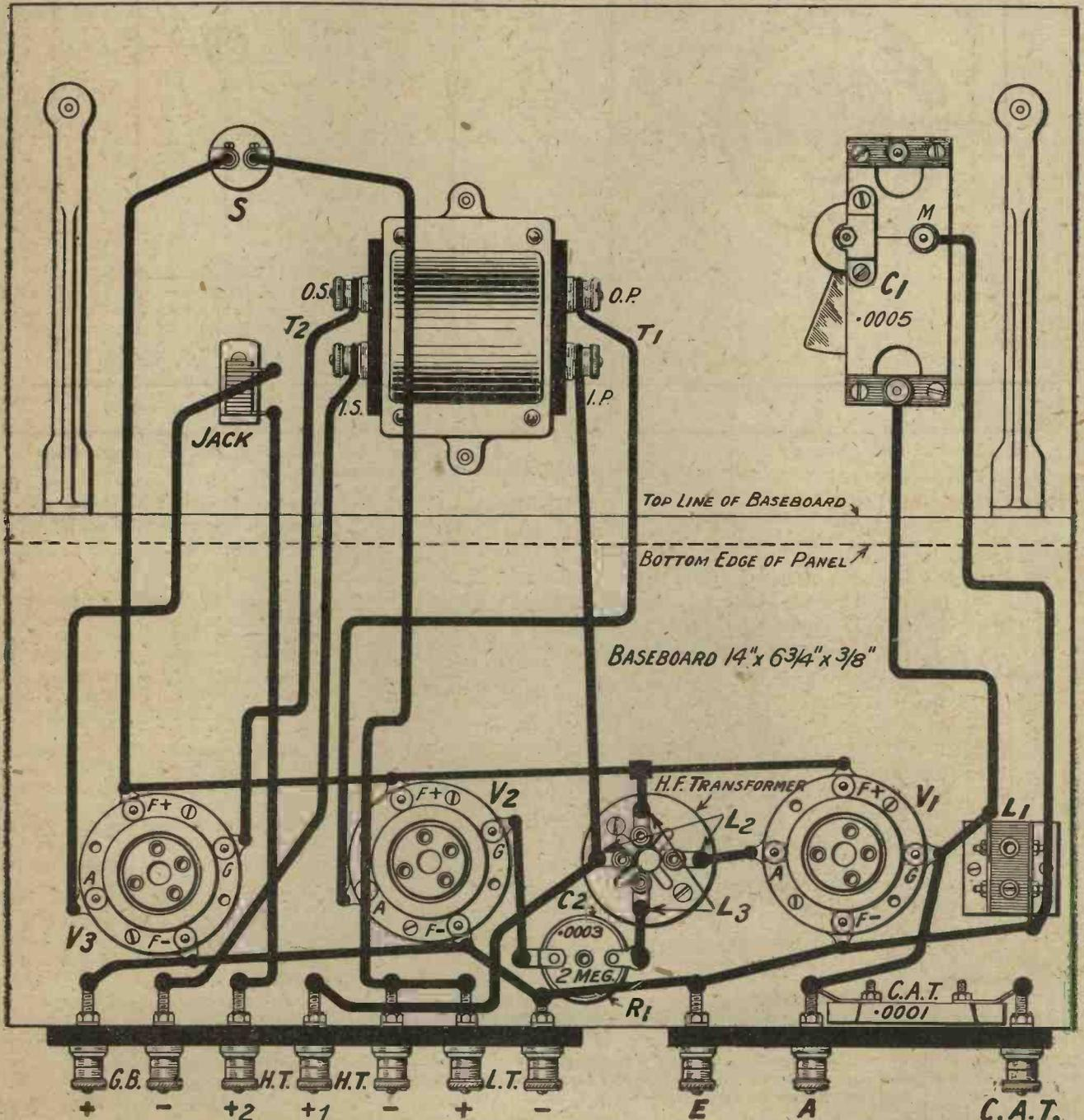
Fig. 3.—This diagram, in conjunction with the special instructions on the opposite page, should make the wiring connections quite clear. This is available in blueprint form, No. C1058B.
