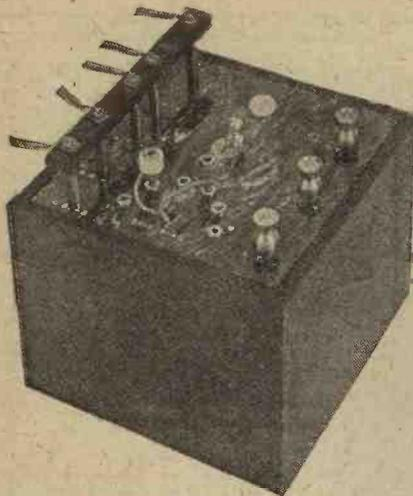
The grid battery is housed in the box, the leads on the left being for connection to the receiver.
