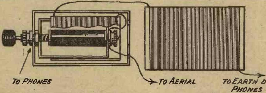
Fig. 2.—This diagram should make quite clear the arrangement of the boxes and the detector.
