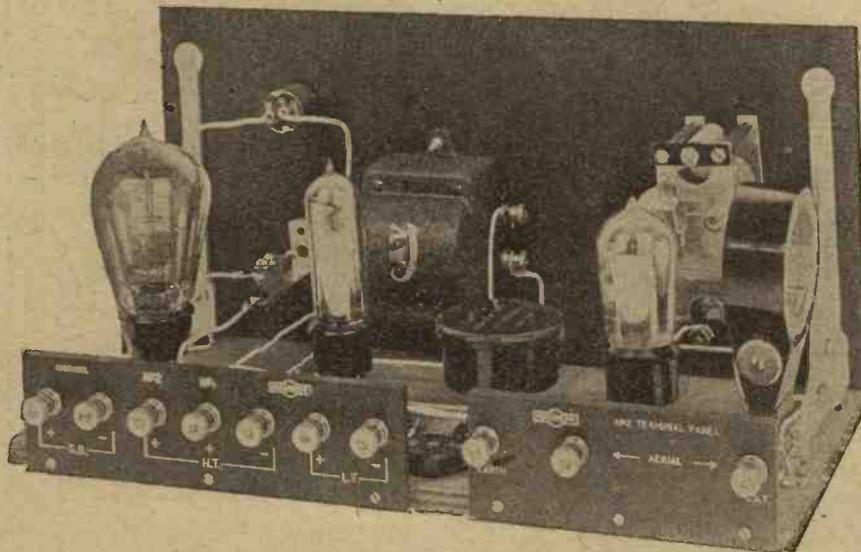
Valves of types suitable for the different functions should be used in order to obtain the best results. They must be of similar filament voltage rating, as no resistances are used.
