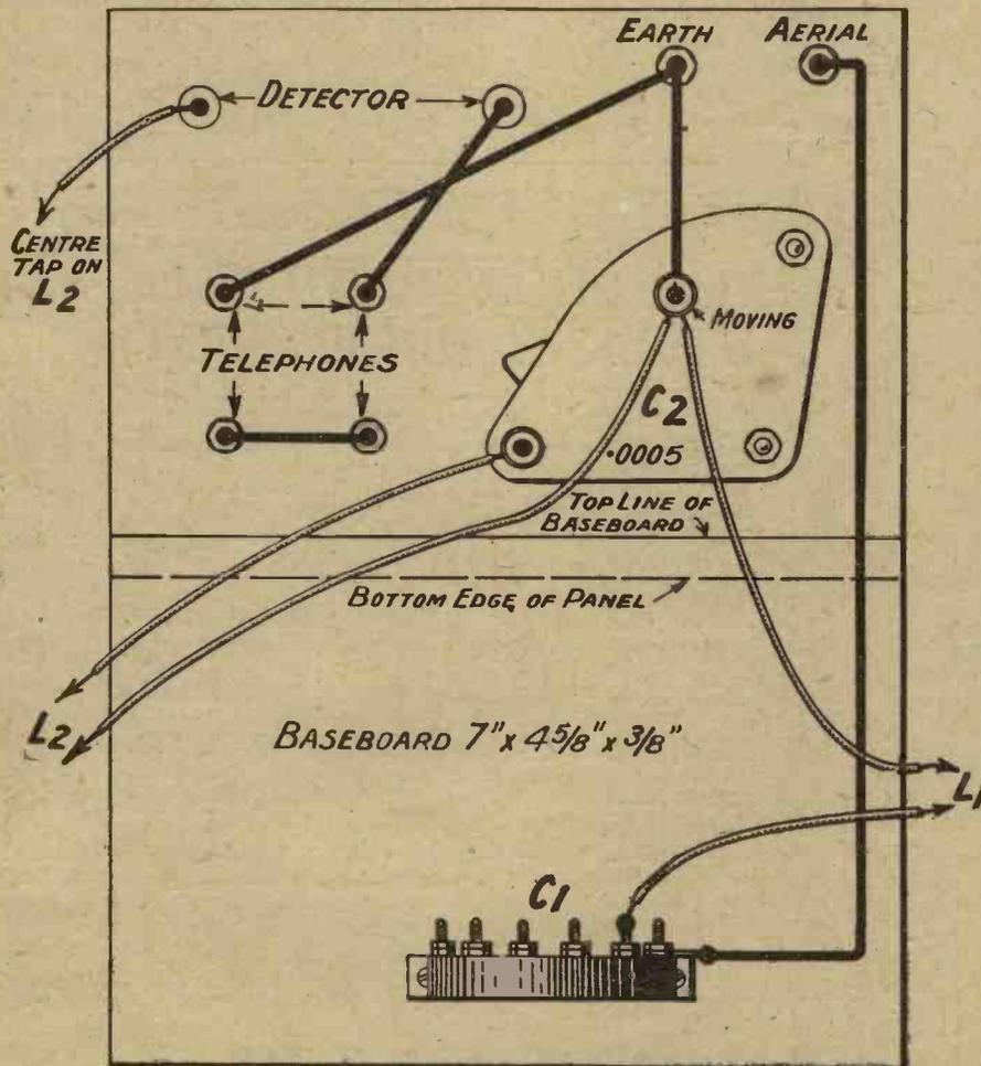
Fig. 3.—The wiring of the set is straightforward. The flexible leads are attached to the coil holder when the set has been fixed in the cabinet. Blueprint No. 1061B.
