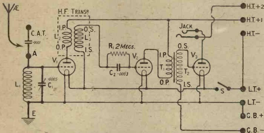
Fig. 1.—Plug-in units are used for the H.F. transformer, making alterations in the wavelength range a simple matter.
