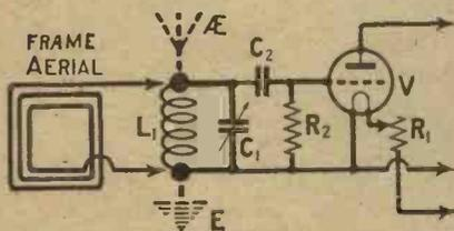
Fig. 1.—This method of connecting a frame aerial to the aerial and earth terminals of an existing receiver would not be satisfactory, as the coil and frame would be in parallel.
