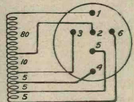
Fig. 4.—Details of the tuning coil and the connections on its base are shown here for the benefit of those who wish to wind their own coil.
