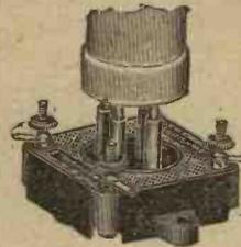
The ANTI-VIBRO VALVE HOLDER (baseboard mounting). Low capacity Valve Legs mounted on a soft rubber base, suspended on four phosphor bronze springs, enclosed in a high quality moulding.
