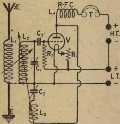
Fig. 1.— To reduce hand-capacity effects it is generally advisable to earth the L.T. battery, as shown by the dotted line.
