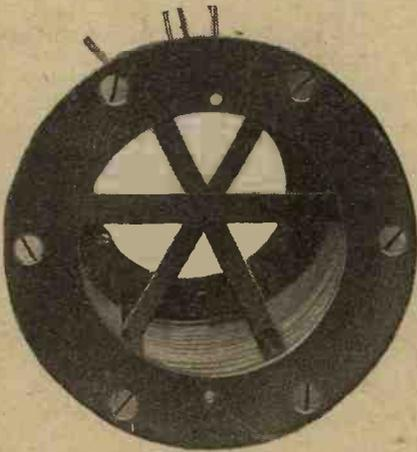
In this type of coil the amount of solid material inside the winding is reduced as far as possible.
