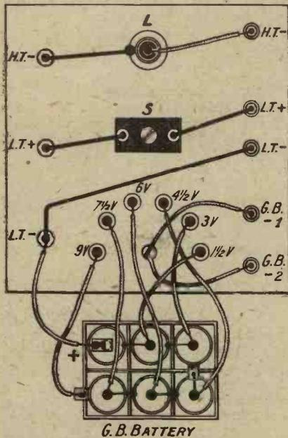
Fig. 3.—This diagram should be carefully followed when the cell connections are being attached.
