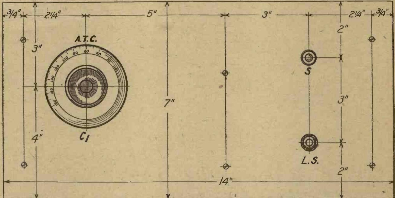
Fig. 2.—The few dimensions required for marking out the panel may be taken from this drawing. Blueprint No. C1058A may also be obtained if desired.
