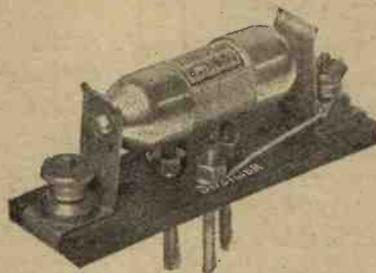
High resistances are conveniently made up into small sealed cartridges, constancy of value being a matter of importance.
