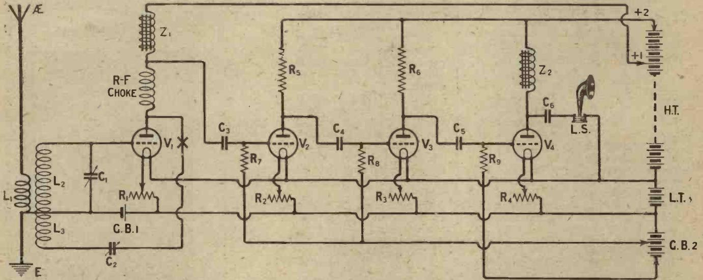
Fig. 2.—In a receiver employing a circuit of this type, poor performance may be due to faults in the anode resistances or grid leaks.
