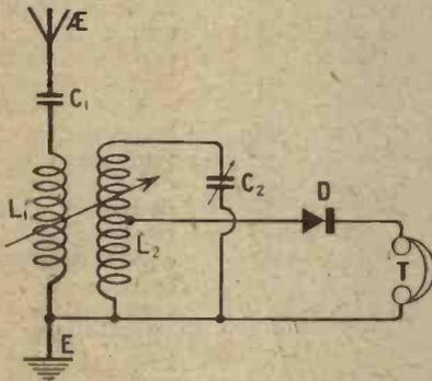
Fig. 1.—An untuned primary and centre-tapped secondary are used to give the requisite degree of selectivity.
