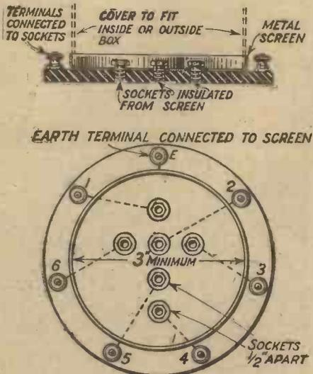
Fig. 5.—The standard mounting of the type of screened coil developed by the author is shown here.
