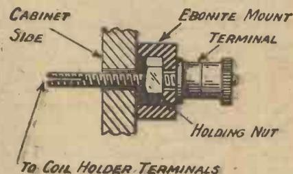
Fig. 1.—The ebonite strip carrying the terminals is screwed to the outside of the cabinet.
