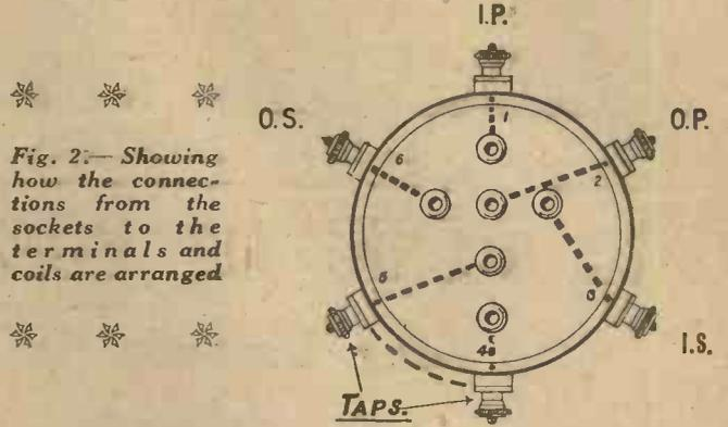
Fig. 2.—Showing how the connections from the sockets to the terminals and coils are arranged
