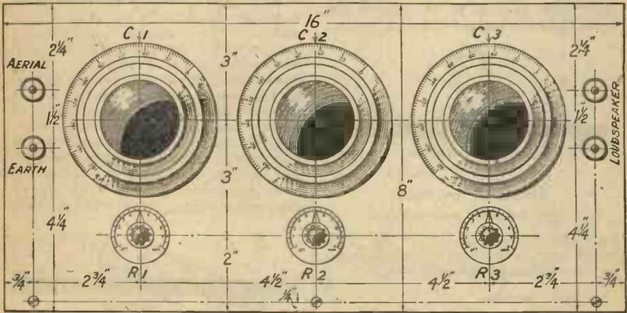
All drilling centres may be obtained from front-of-panel diagrams of this type.
