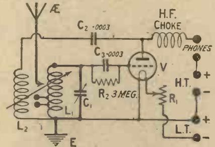
Fig. 1.—The aerial may be tapped on at any one of three points to obtain the required degree of selectivity.
