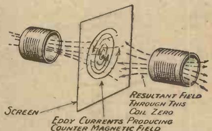
Fig. 4.—The magnetic field from one coil will produce eddy currents in the screen which will cancel out the effect of the field.
