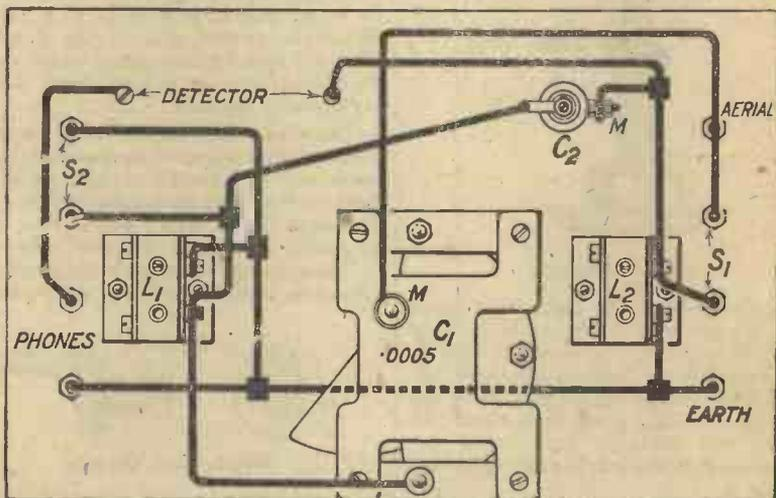
A typical back-of-panel wiring diagram. All soldered connections are shown by "blobs."
