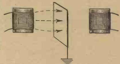
Fig. 2.—The introduction of an earthed screen provides an effective barrier to the capacitive coupling.
