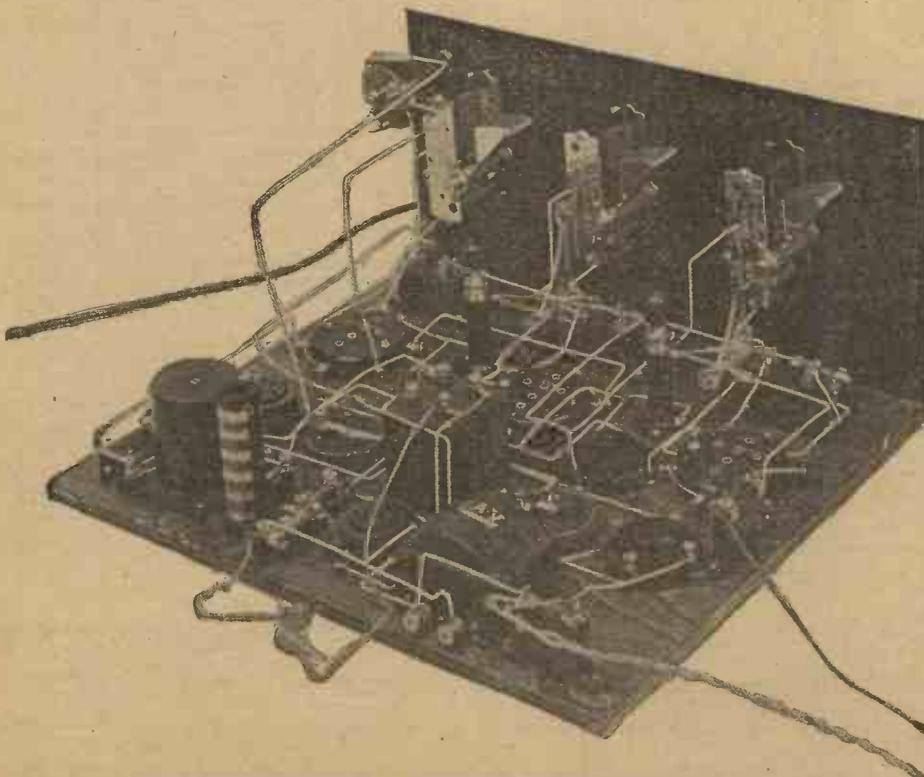
The two leads with wander plugs are for the grid bias battery, which may be placed inside the cabinet.
