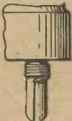
Fig. 3.—A piece of wire fixed in the cleft of a valve pin will ensure a good contact with the socket.
