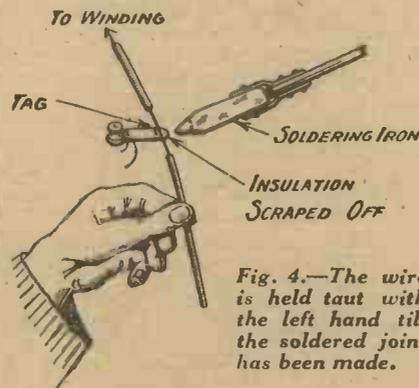
Fig. 4.—The wire is held taut with the left hand till the soldered joint has been made.
