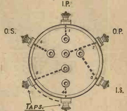
Fig. 2.—Showing how the connections from the sockets to the terminals and coils are arranged
