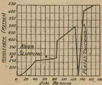
Fig. 2.—This chart illustrates the straight-line-wavelength principle as exhibited by a (very) variable condenser.
