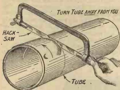
This shows the proper method of cutting an ebonite or cardboard tube.
