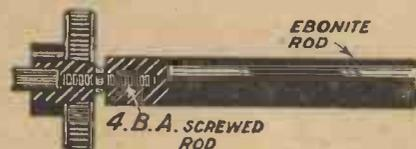
Fig. 3.—An easily fitted extension handle for a condenser dial.
