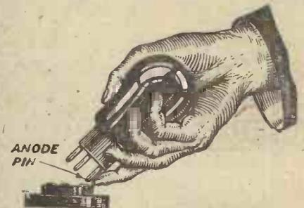
Fig. 1.—This method of inserting a valve in its holder will prevent damage to the filament.
