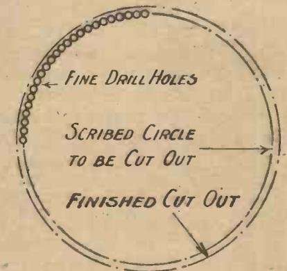
Fig. 1.—When no special tool is available, a large hole may be made in the manner shown.
