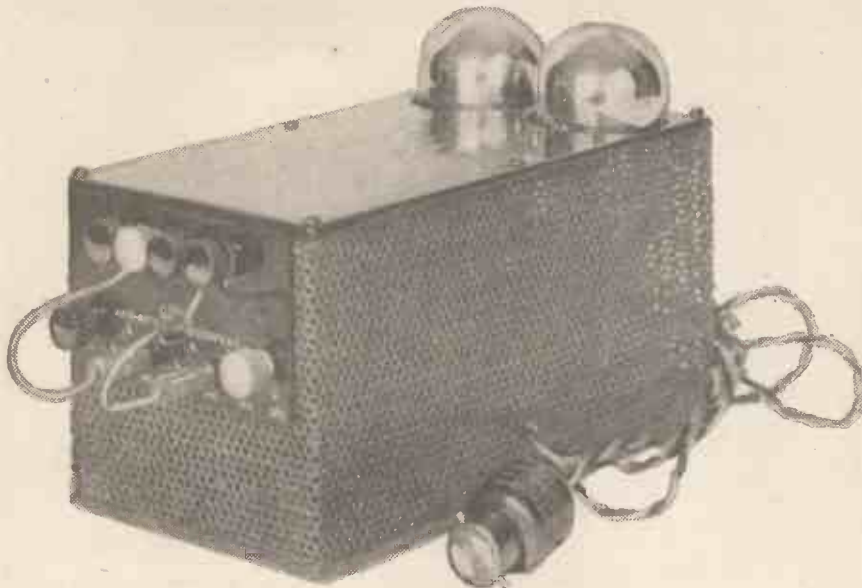
The Climax H.T. unit for A.C. mains.
