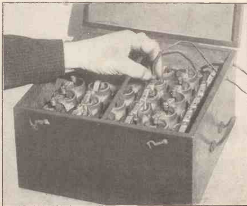
An H.T. battery consisting of a group of wet Leclanche cells. This type of anode battery is becoming very popular.
