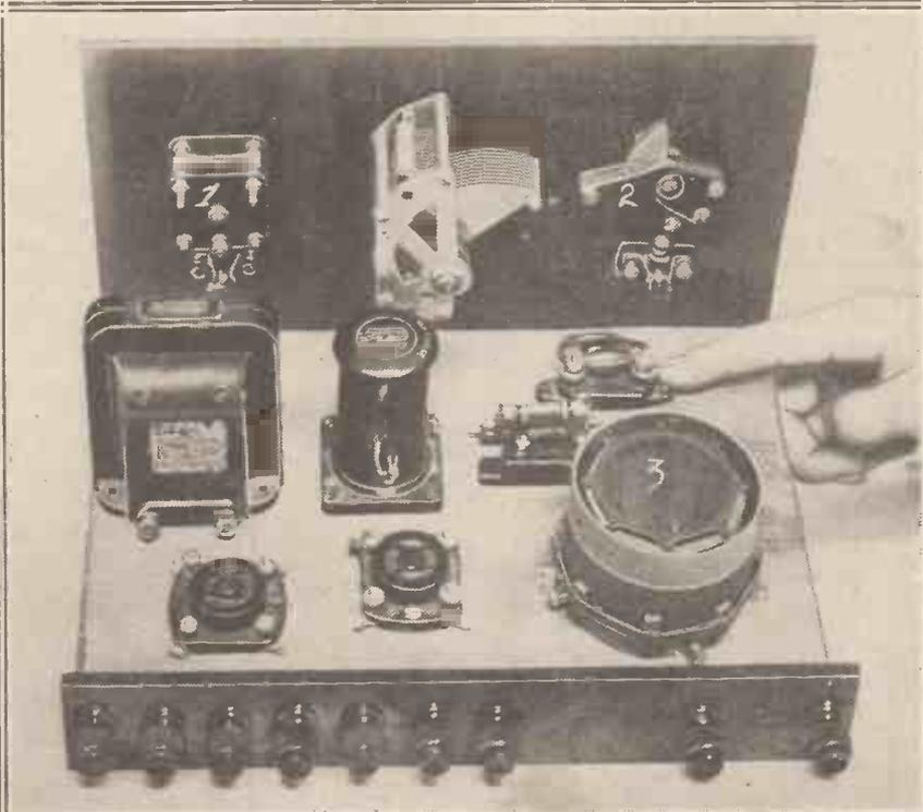
Selected Circuit No. 23 is a "hot" two-valver, and here the parts are shown correctly positioned. (1) is the differential reaction condenser; (2) Brookmans condenser, and (3) the dual-range coil. The pointing finger shows the .002 compression-type condenser and Spaghetti resistance that form the "Interleave" coupling.
