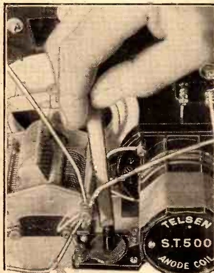
The selectivity range adjuster should be screwed up tight for the first tests. If any further adjustments are made, the hand should be removed each time when noting the effect.
