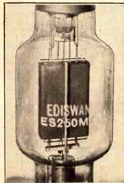
One of the new "graphite valves"—a 250 watts dissipation type. In the heading are also shown a larger type and the E.S.75H. mentioned in the article.
