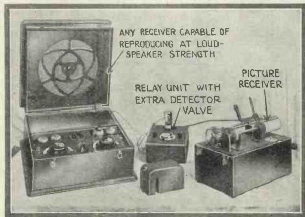
Fig. 2.—Complete apparatus for receiving wireless pictures. The cost is just over £20, exclusive of the ordinary radio set. Two models of the Fultograph are made, one in oak and the other in mahogany; each requires an extra rectifying valve
