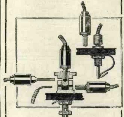
The diagram above shows the use of a spring jack attached to a socket for use with 'phone or loud-speaker jack ends or plugs. Also the famous
