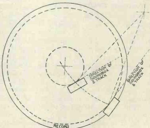
Fig. 10.—Modern needle-track alignment
