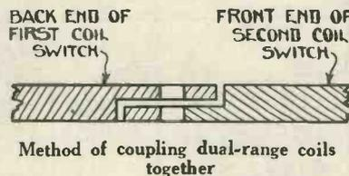
Method of coupling dual-range coils together
