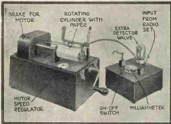
Fig. 3.—On the left is the picture receiver proper, while on the right is the relay unit. Round the cylinder is placed a piece of special absorbent paper which has been damped with a chemical solution. The picture is formed on this paper by varying currents passing from the needle point to the metal cylinder
