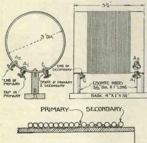
Fig. 2.—Details of aerial-grid transformer used in the Touchstone
