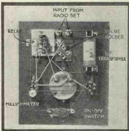
Fig. 11.—Underneath view of the relay unit, showing the arrangement of the various parts. The relay is short-circuited while the actual picture signals are being received and comes into use to release the catch-stop at the beginning of each revolution of the receiving cylinder
