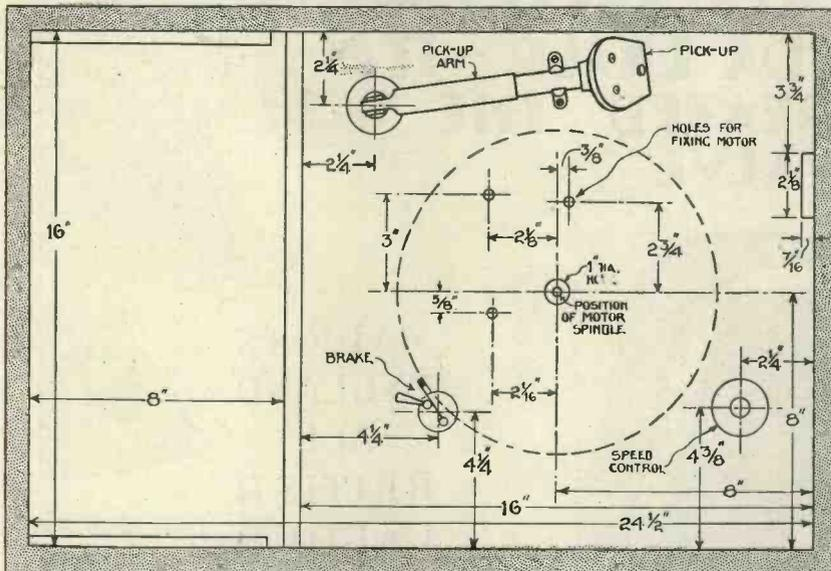
This diagram shows how the turn-table and motor, and pick-up and tone-arm, are mounted in position
