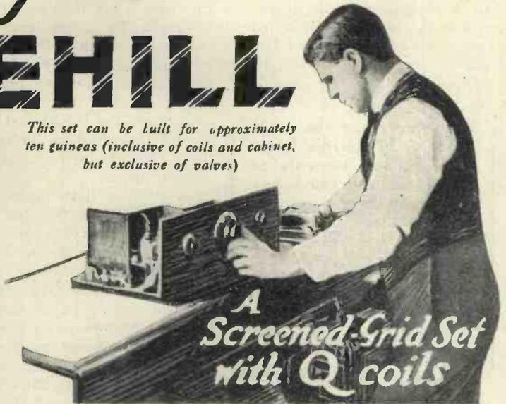
In this article J. H. REYNER, B.Sc., A.M.I.E.E., describes the construction of a new one-dial all-wave set comprising screened-grid high-frequency amplifier, anode-bend detector and two stages of transformer-coupled low-frequency amplification
