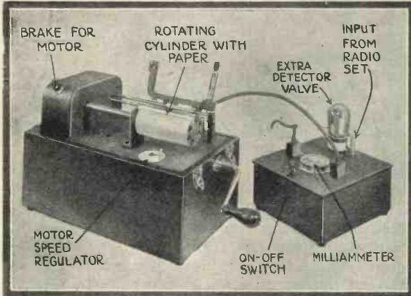
Fig. 3.—On the left is the picture receiver proper, while on the right is the relay unit. Round the cylinder is placed a piece of special absorbent paper which has been damped with a chemical solution. The picture is formed on this paper by varying currents passing from the needle point to the metal cylinder
