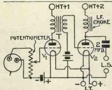
Fig. 9.—Complete amplifier connections
