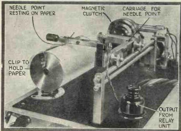
Fig. 4.—Here the needle point is seen resting in position on the paper; it is moved over the cylinder by means of a threaded rod (approximately 64 threads to the inch). The needle should be wiped after each picture has been received
