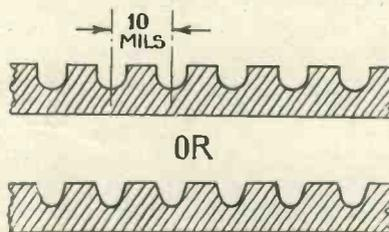
Fig. 1.—Grooves in a record
