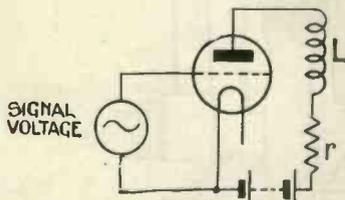
Fig. 1.—Power valve with loud-speaker in anode circuit
