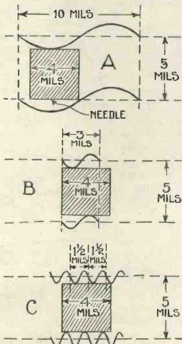
Fig. 7.—Needle size and different frequencies
