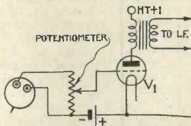
Fig. 6.—How pick-up is connected. It is across the ends of a 200,000-ohm Rothermel potentiometer and the grid of the valve is connected to the moving contact.
