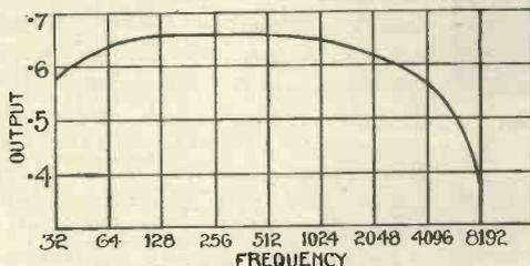
Fig. 6.—Amplification-frequency curve of Touchstone R.C. stage
