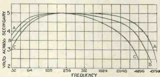
Fig. 4.—Curve for Brown transformer and Cossor valves. Curve A is with 16,000-ohm valve; curve B is with 20,000-ohm valve; and curve C is with 28,000-ohm valve
