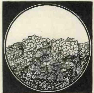
Fig. 3.—Enormously magnified surface of aerial (copper) wire, converted into a mass of bluish green soluble crystals (non-conductive and loose), by the action of sulphuric acid formed from sulphur in the atmosphere
