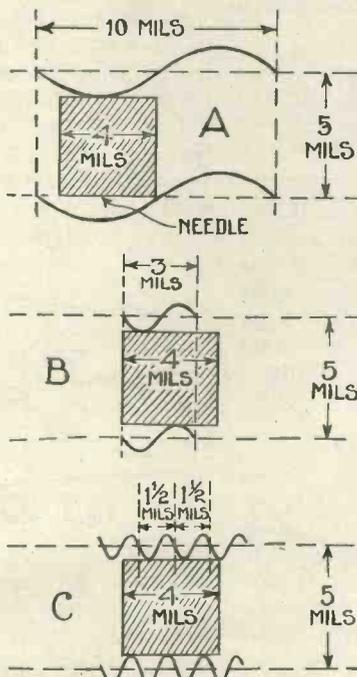
Fig. 7.—Needle size and different frequencies
