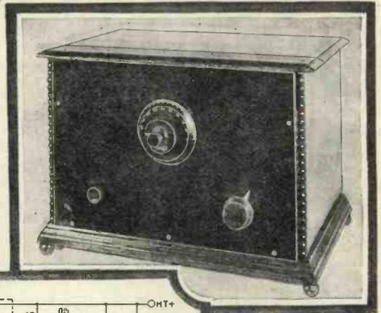
Fig. 11 (above).—This is the completed three-valver in a Pickett Cabinet
