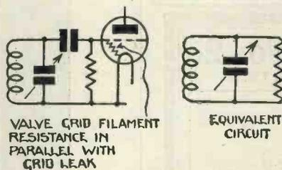
Fig. 1.—Circuit of Leaky-grid detector
