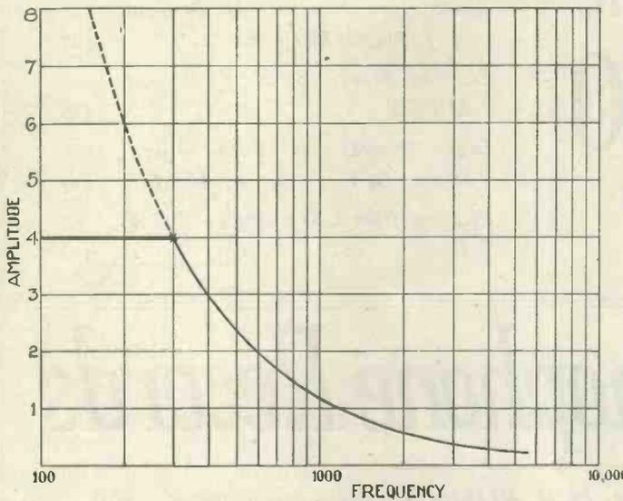
Fig. 4.—Record frequency-amplitude curve
