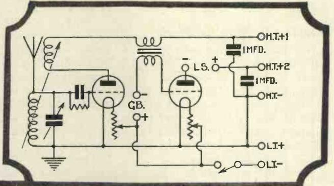
Fig. 4.—Circuit used; note the old-type magnetic reaction. The valve combination is a detector and a transformer-coupled low-frequency amplifier
