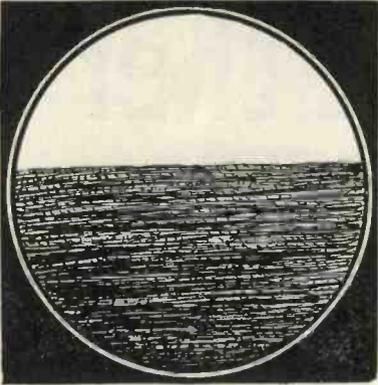
Fig. 1.—Enormously magnified surface of aerial (copper) wire, showing its fresh, lustrous, fibrous formation
