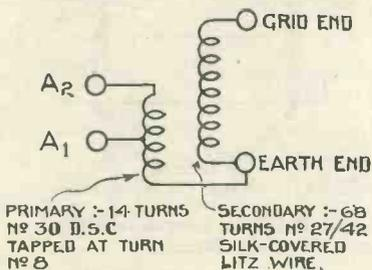
Fig. 1.—Showing variation of selectivity by tapping on the aerial-grid coil
