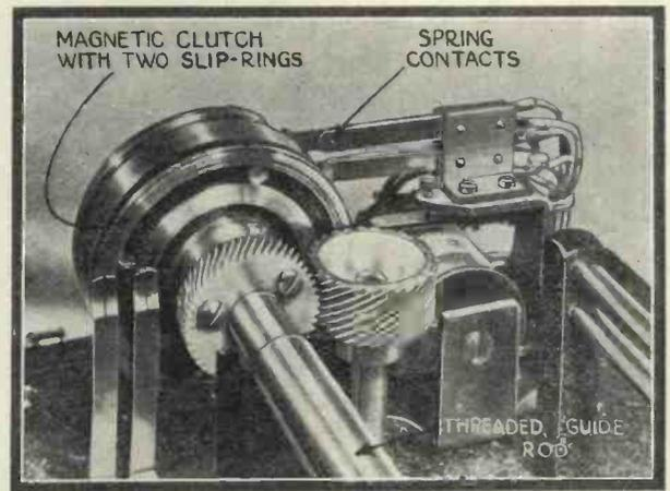
Fig. 6.—The catch-stop, magnetic clutch, and relay are actuated by projections on the cam plate, behind the magnetic clutch, which engage with the spring contacts on the right
