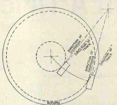
Fig. 9.—Bad needle-track alignment
