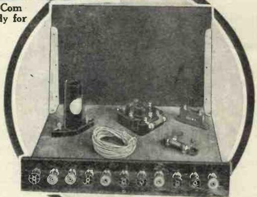
Fig. 7 (above).—Additional components needed for the new set. Notice how few there are and estimate the cost. In the centre is the new Dubilier resistance-coupling unit and valve holder combined.
