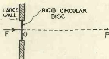
Fig. 4.—Sound at  $P$  is proportional to acceleration of disc, which is 2 in. diameter, and  $P$  is 2 ft. or more from  $O$
