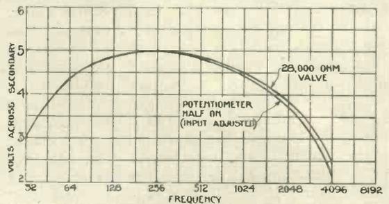
Fig. 8.—Curves with different potentiometer settings
