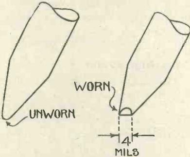
Fig. 6.—How a needle wears
