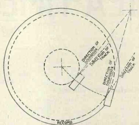
Fig. 9.—Bad needle-track alignment
