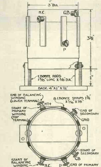
Fig. 4.—Details of intervalve H.F. transformer
