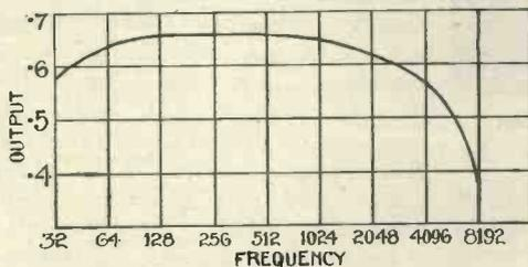
Fig. 6.—Amplification-frequency curve of Touchstone R.C. stage
