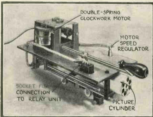
Fig. 9.—Here is the picture receiver removed from its case. The double-spring motor must be wound up for the reception of each picture, which takes four minutes to come through
