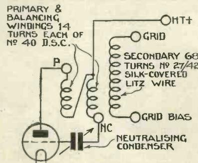
Fig. 3.—Circuit of H.F. transformer
