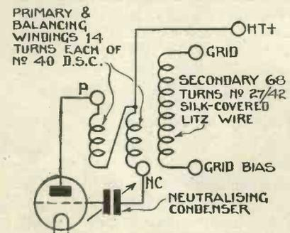
Fig. 3.—Circuit of H.F. transformer
