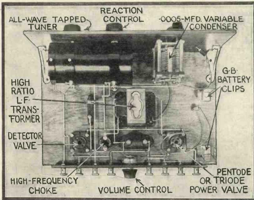
This view of the Meteor Two clearly shows the layout of the parts on the baseboard. Note that provision is normally made for a 9-volt grid-bias battery on the baseboard, but for some valves a 16½-volt battery may be required
