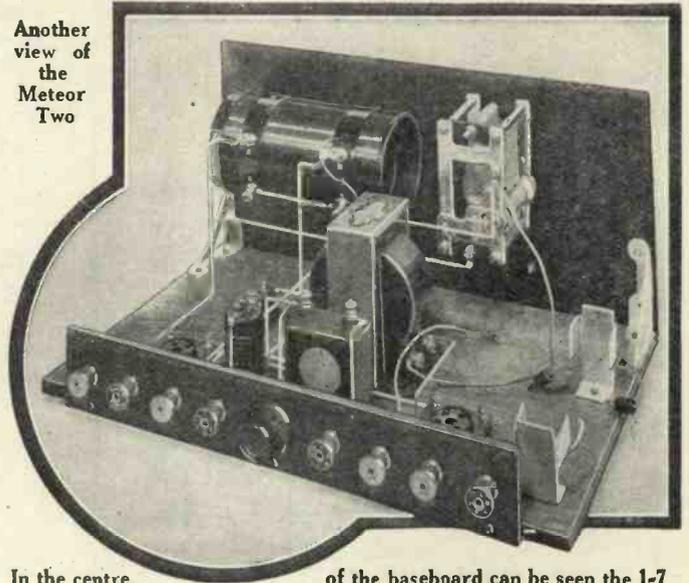
In the centre of the baseboard can be seen the 1-7 low-frequency transformer
