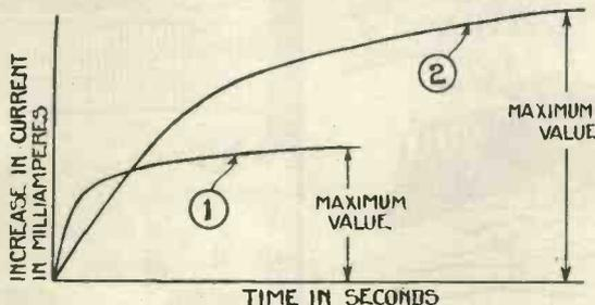
Fig. 2.—Showing rise of current through loud-speaker of Fig. 1 when a voltage is suddenly applied to grid of valve
