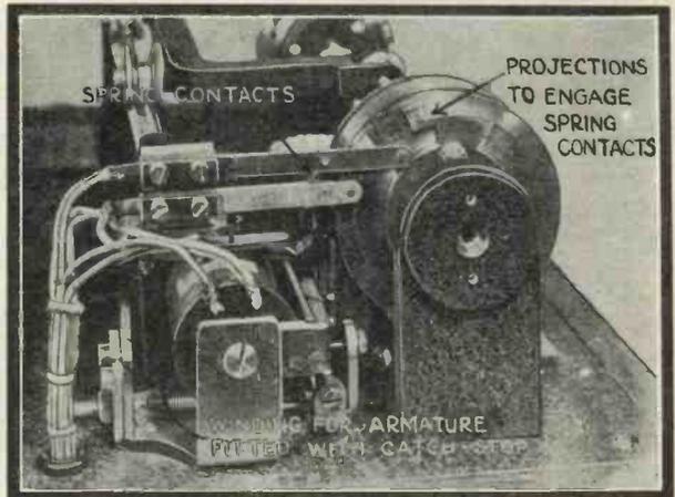
Fig. 8.—This photograph clearly shows the projections on the cam plate for actuating the spring contacts which control the catch-stop and magnetic clutch for stopping and starting the cylinder. This mechanism is protected by a metal cover
