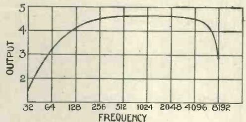
Fig. 5.—Amplification-frequency curve of the Touchstone
