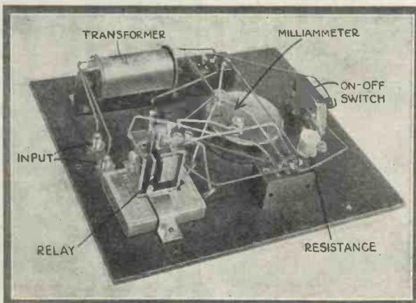
Fig. 12.—Another view of the relay unit. The transformer has a step-up ratio of 1 to 6 and is connected across the input terminals. The valve is adjusted to give a zero milliammeter reading before a connection is made to the input terminals
