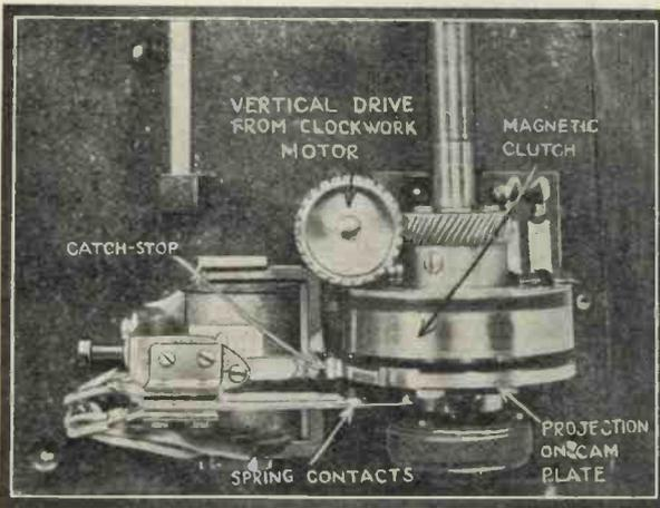
Fig. 5.—The catch-stop stops the cylinder from rotating when required and the clutch is withdrawn at the same time, thus allowing the motor to run continuously at the same speed
