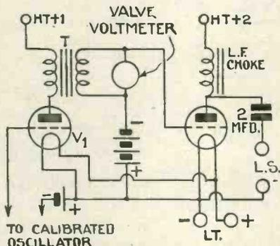
Fig. 3.—Circuit of Amplifier when testing Transformer-Valve Combinations
