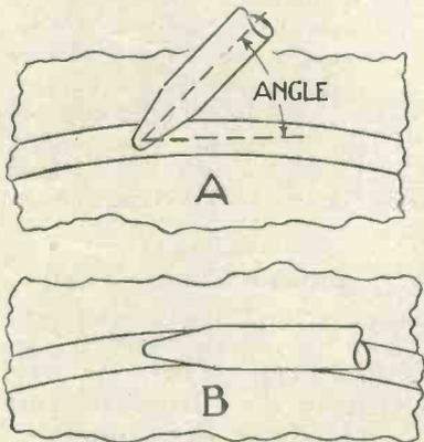
Fig. 8.— Needle angle
