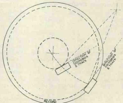
Fig. 10.—Modern needle-track alignment
