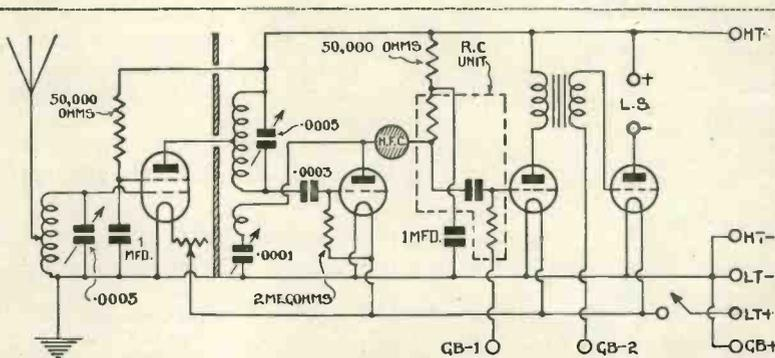
Circuit of the Economy Screened-grid Four, which comprises H.F., detector, and two L.F. stages
