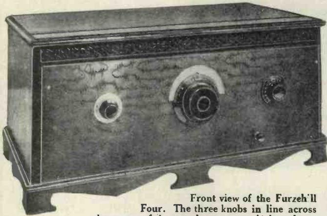
Front view of the Furzehill Four. The three knobs in line across the centre of the panel are respectively volume control, main tuning condenser, and reaction control. Below are the wave-change and on-off switch knobs
