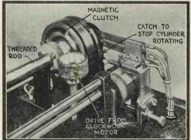
Fig. 7.—On the right can be seen the armature with its catch-stop and the winding which actuates it. The threaded rod drives the cylinder and, at the same time, moves the needle carriage over the paper  $1/64$  in. at a time
