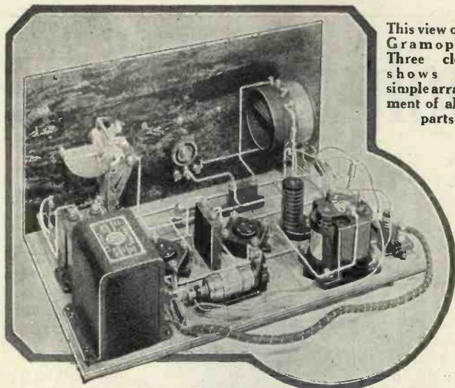
This view of the Gramophone Three clearly shows the simple arrangement of all the parts
