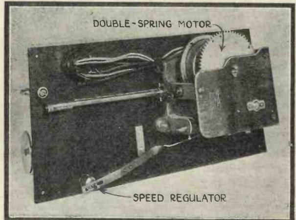
Fig. 10.—Here is another view of the double-spring motor, which is of the gramophone type. It is necessary to adjust the speed regulator so that the cylinder synchronises properly at each revolution
