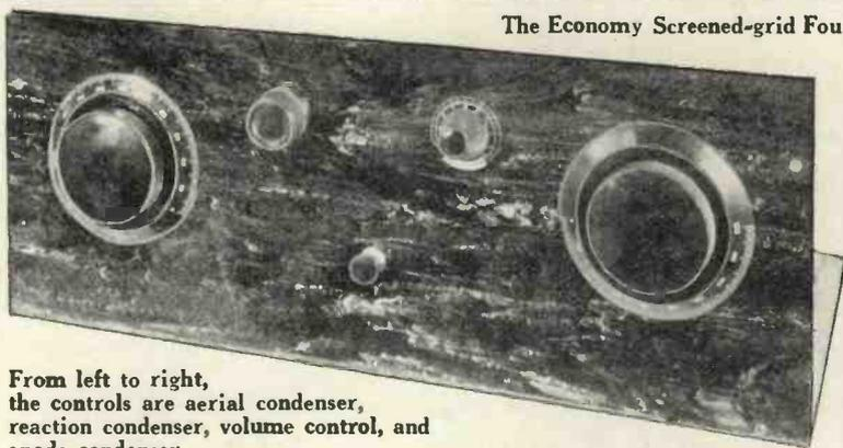
From left to right, the controls are aerial condenser, reaction condenser, volume control, and anode condenser
