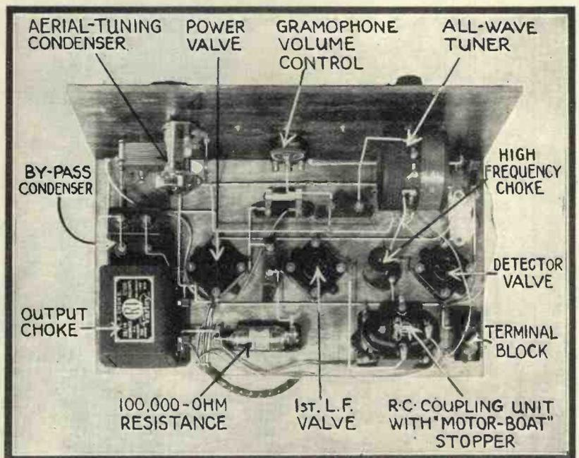
This plan view of the receiver portion of the Gramophone Three clearly shows the arrangement of all the parts. It will be seen that the wiring is exceptionally easy and will present no difficulty even to the beginner.
