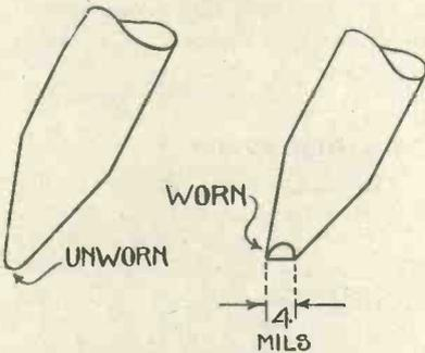
Fig. 6.—How a needle wears
