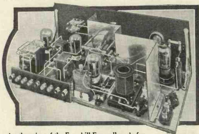
Another view of the Furzehill Four, all ready for use with the valves in position. The biasing battery for getting the best anode-bend point can be seen close to the main terminal strip
