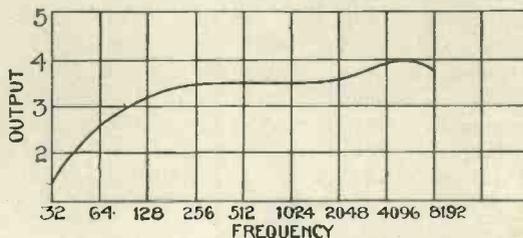
Fig. 7.—Amplification-frequency curve of Touchstone transformer stage
