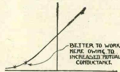
Fig. 2—Position of anode-bend point on valve characteristic
