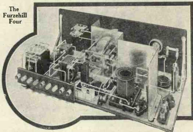
The compact layout of the Furzehill Four is apparent from this photograph, which clearly shows the arrangement of all the parts: Note especially the position of the screening
