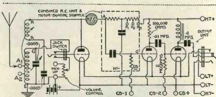
This is the circuit utilised in the Gramophone Three. The combination comprises an anode-bend detector followed by two stages of resistance-capacity coupled L.F. amplification
