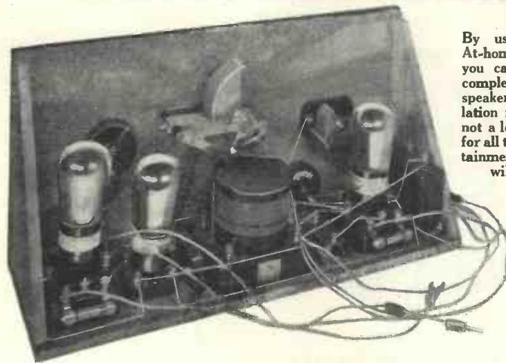
A back view of the completed At-home Three with the valves in position
