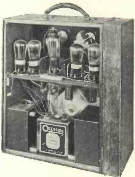
Front view of the Wayfarer, showing the internal components.
