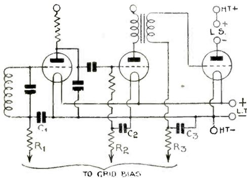
Fig. 1.—Grid-circuit filters
