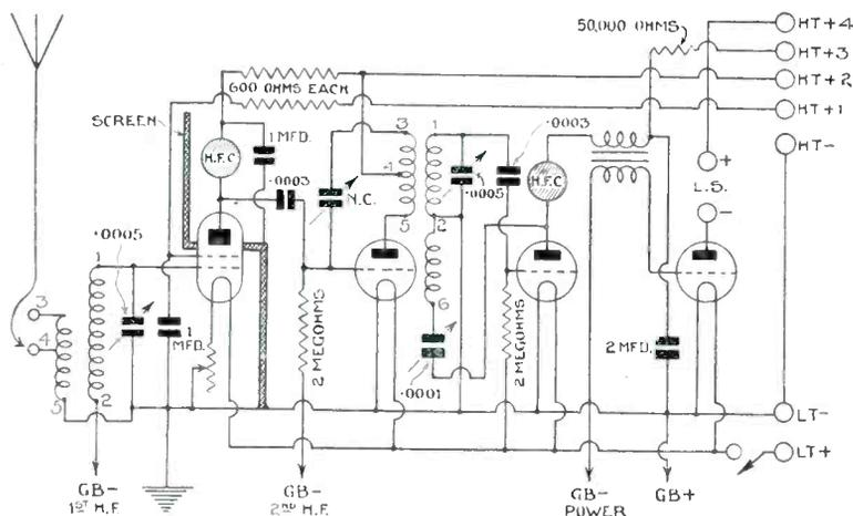
Circuit of the Arrow Four, which combines a screened-grid valve with a three-electrode high-frequency amplifier
