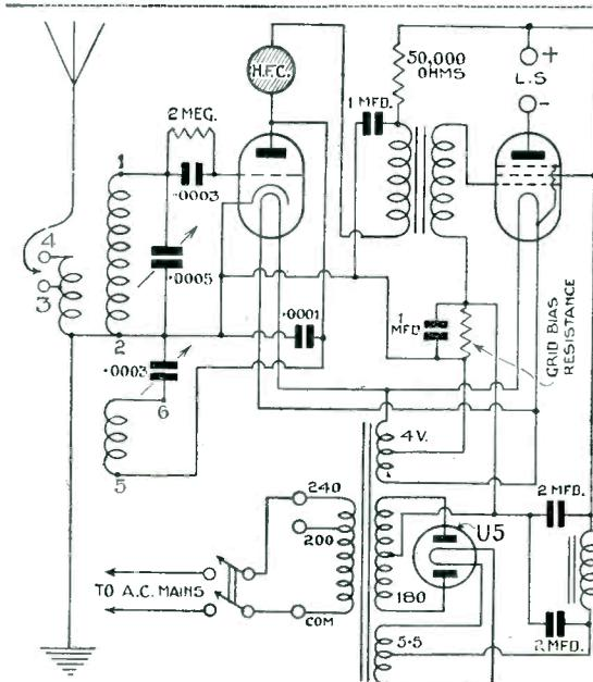
Circuit of the Stay-put Two—an All-A.C. two-valver with dual-range coils
