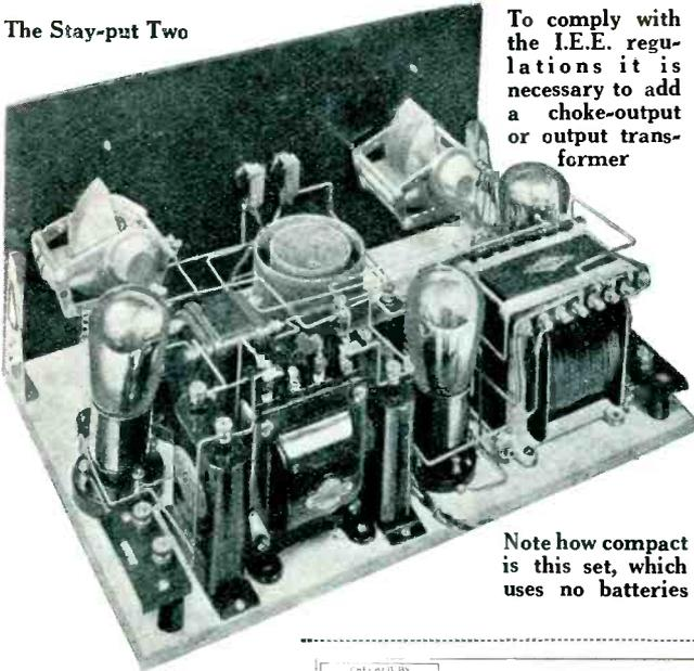
To comply with the I.E.E. regulations it is necessary to add a choke-output or output transformer
