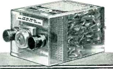
The electrolyte in C.A.V. non-spillable batteries differs from all previously known jellied acid electrolyte, in so far that it is not a solid mass but possesses a cohesive honey-comb like structure, whereby free distribution of the gases evolved during charge and discharge is ensured.
