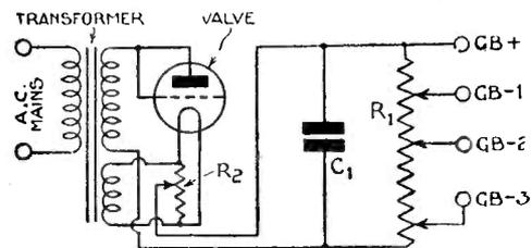
Fig. 5.—Simplified form of grid-bias unit with valve rectifier
