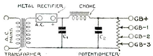
Fig. 2.—Grid-bias unit using metal rectifier
