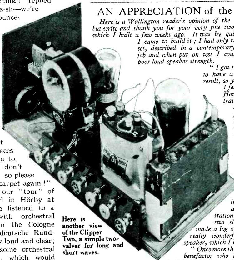
Here is another view of the Clipper Two, a simple two-valver for long and short waves.
