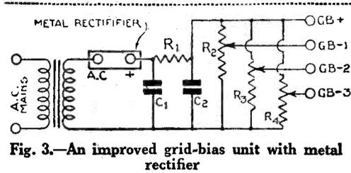
Fig. 3.—An improved grid-bias unit with metal rectifier
