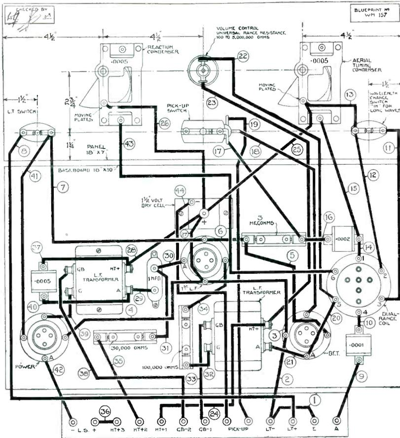
This layout and wiring diagram of the Fanfare Three can be obtained as a full size-blueprint for half-price (that is, 6d., post free), if the coupon on page iii of the cover is used by September 30. Ask for No. WM157. Connect up in numerical order
