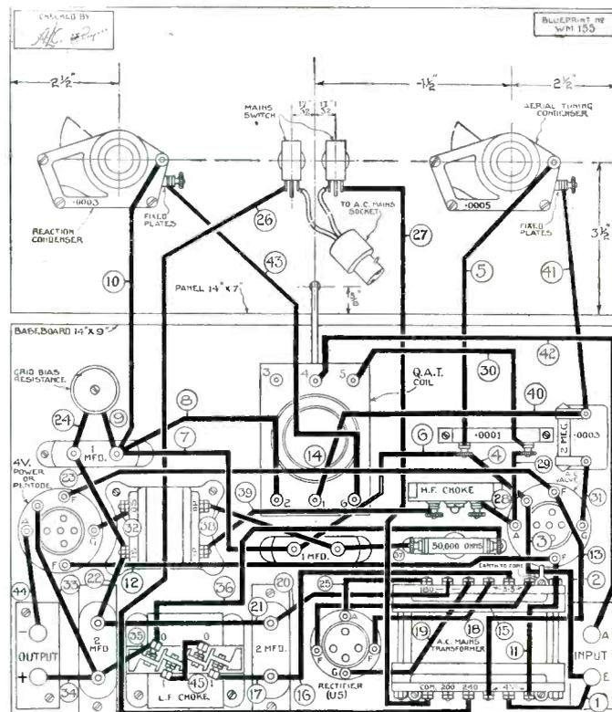
This layout and wiring diagram of the Stay-put Two can be obtained as a full-size blueprint for half-price (that is, 6d., post free) if the coupon on page iii of the cover is used by September 30. Ask for No. WM155. Connect up leads in numerical order.
