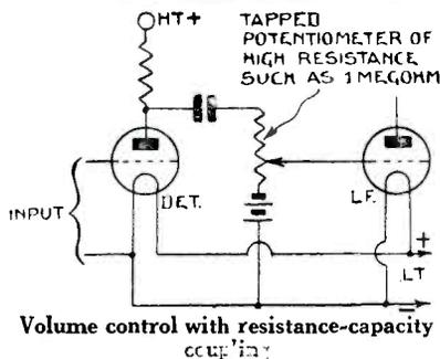
Volume control with resistance-capacity coupling
