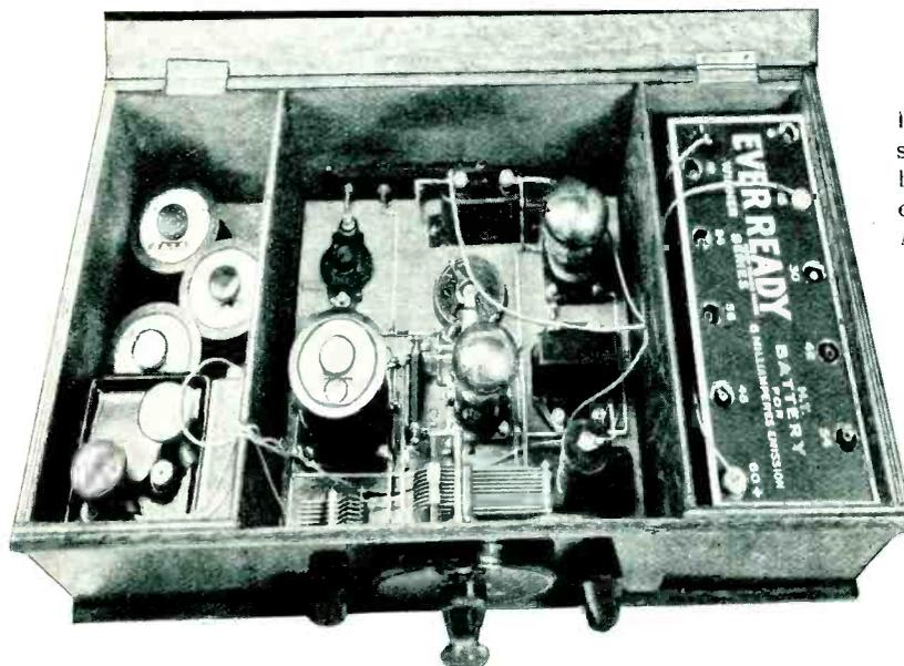
This photograph shows the batteries and spare coils in position in the special compartments provided for them
