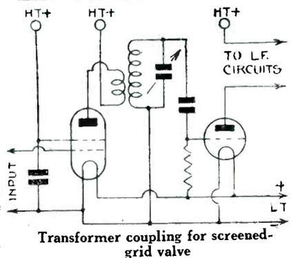
Transformer coupling for screened-grid valve
