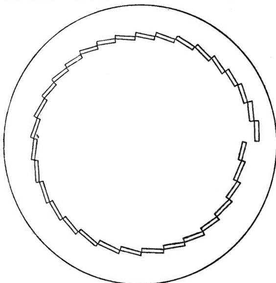
Arrangement of slots in scanning disc
