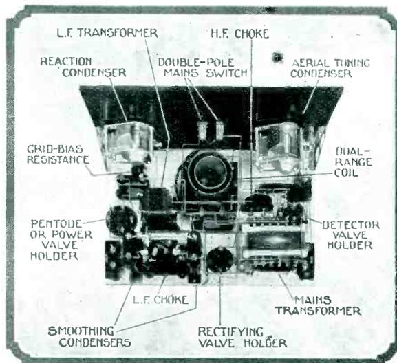
This plan view of the Stay-put Two clearly shows how all the components are arranged
