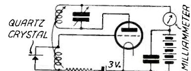
Oscillating circuit with crystal control
