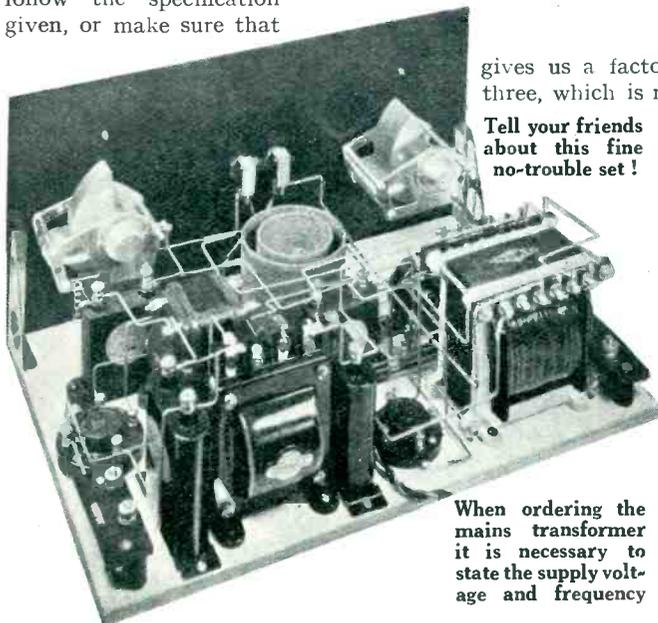
When ordering the mains transformer it is necessary to state the supply voltage and frequency
