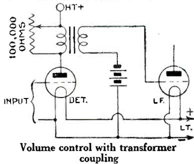
Volume control with transformer coupling
