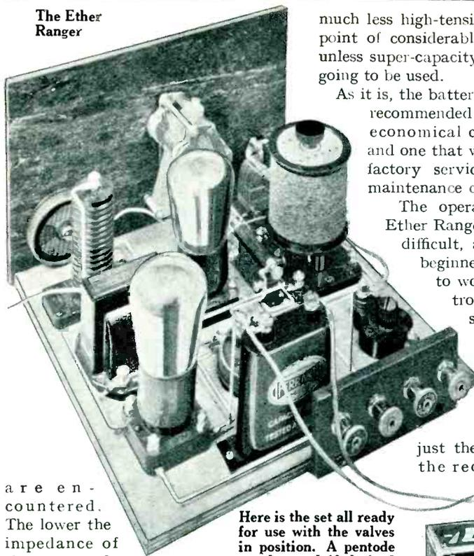
are encountered. The lower the impedance of the power valve (within limits, of course), the better is the quality of reproduction.
