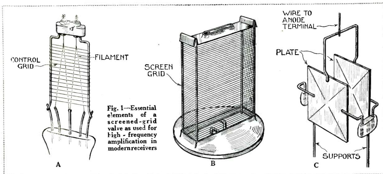
Fig. 1—Essential elements of a screened-grid valve as used for high-frequency amplification in modern receivers
