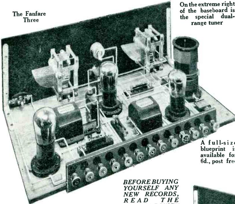
On the extreme right of the baseboard is the special dual-range tuner
