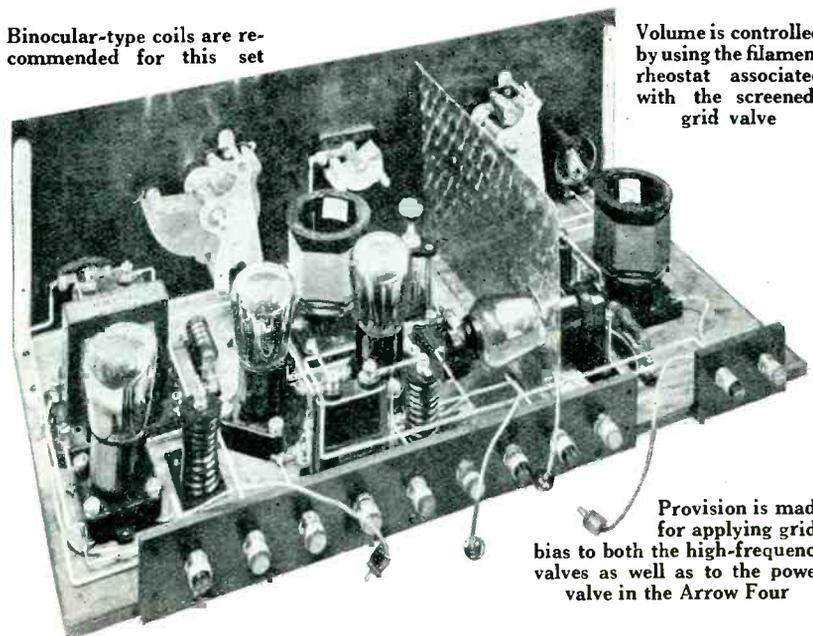
**Volume is controlled by using the filament rheostat associated with the screened-grid valve**
