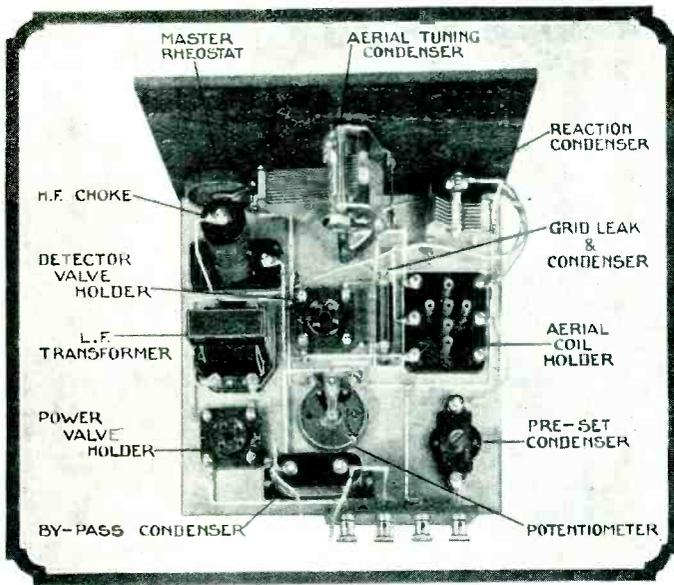
the voltage applied to the detector to as low a value as possible without decreasing the signal strength.
