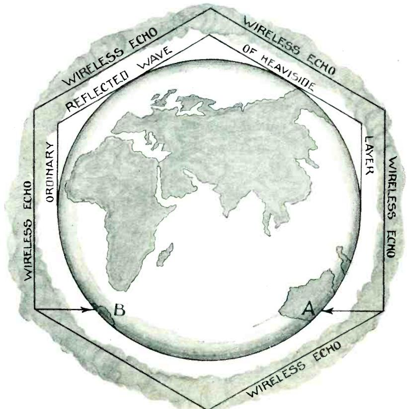
Diagram showing Heaviside layer theory of wireless echo. Wireless waves are radiated from the earth at A, travel round the world (thick line) about 100 times within the confines of the layer and, by some freak, return to the earth at B.
