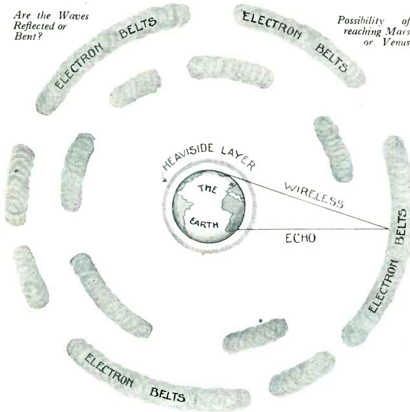
Diagram showing electron belt theory of wireless echoes. The wireless waves from the earth penetrate the Heaviside layer—strike the electron belt and are reflected back to earth
