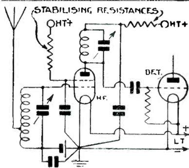
Positions of stabilising resistances in screened-grid valve set
