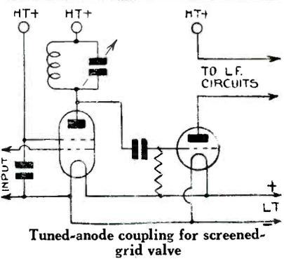
Tuned-anode coupling for screened-grid valve
