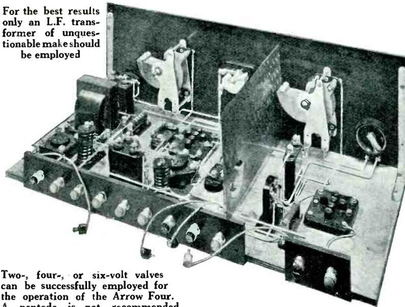
Two-, four-, or six-volt valves can be successfully employed for the operation of the Arrow Four. A pentode is not recommended
