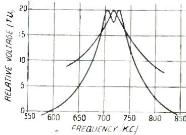
Tuning curve for coupled circuits
