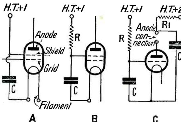
Fig. 2.—Arrangements of grid and anode filters
