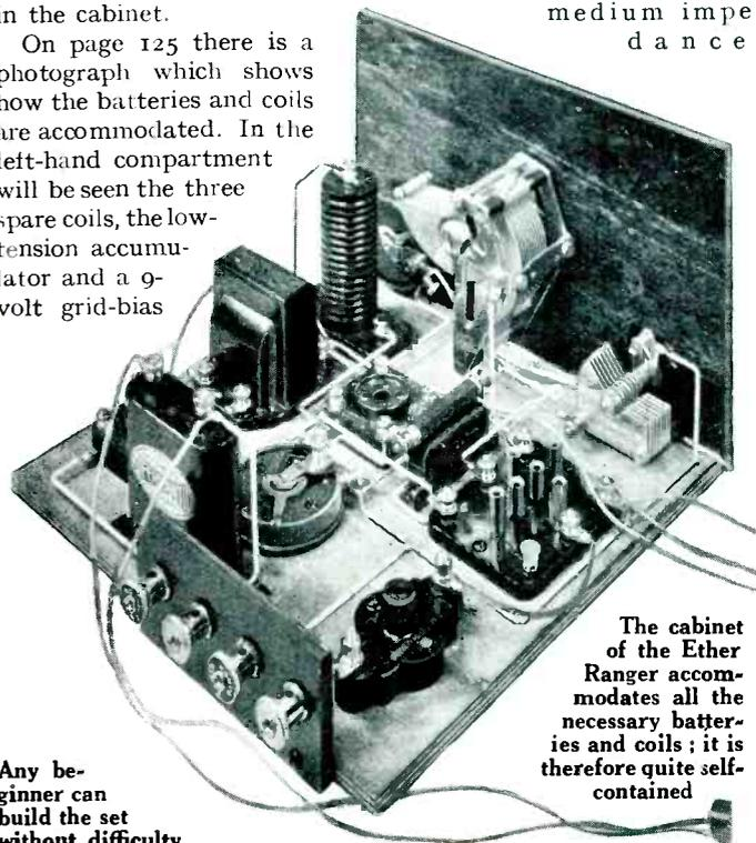
The cabinet of the Ether Ranger accommodates all the necessary batteries and coils; it is therefore quite self-contained
