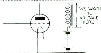
Fig. 1.—Typical interval transformer circuit
