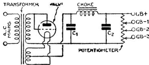
Fig. 4.—Grid-bias unit using valve rectifier
