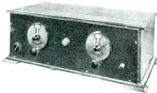
IT has been our object in designing the Arrow Four to provide an extremely powerful and selective four-valver incorporating two stages of high-frequency amplification, but with very simple tuning.
