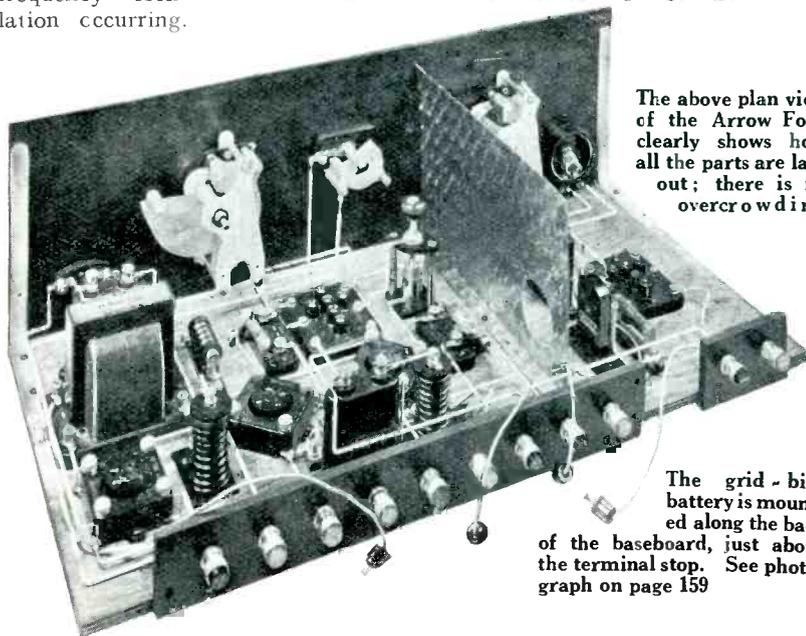
The grid-bias battery is mounted along the back of the baseboard, just above the terminal stop. See photograph on page 159
