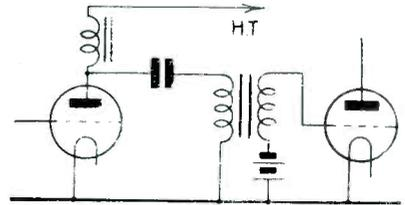
Fig. 2.—Choke feed to transformer primary
