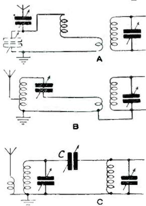
Three types of aerial circuits with magnetic and capacity couplings
