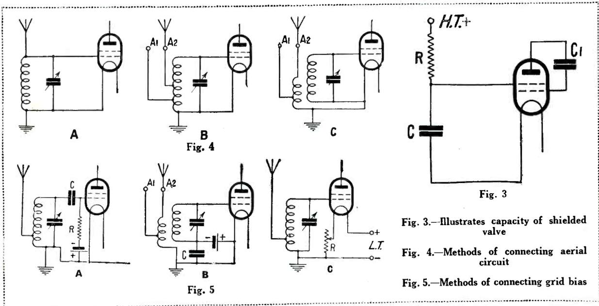
Fig. 3.—Illustrates capacity of shielded valve
