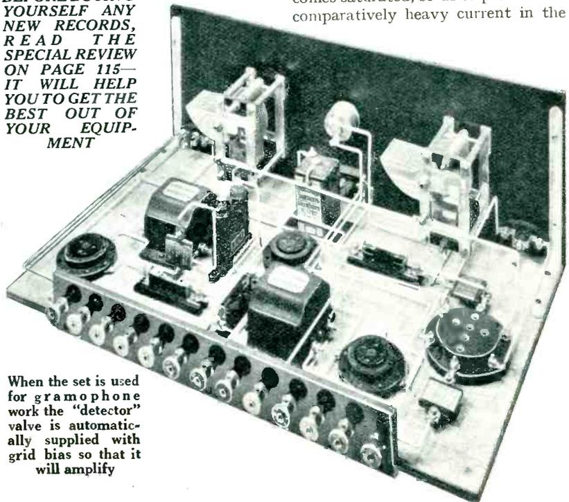
When the set is used for gramophone work the "detector" valve is automatically supplied with grid bias so that it will amplify
