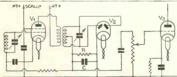
Fig. 9.—Automatic volume control operating from a full-wave detector
