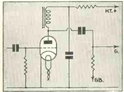
Fig. 5.—Choke-coupled detector circuit to avoid large drop in high-tension voltage
