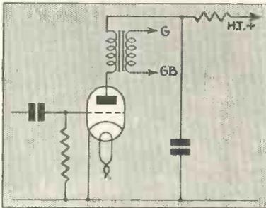
Fig. 6.—Typical circuit with standard low-frequency transformer coupling
