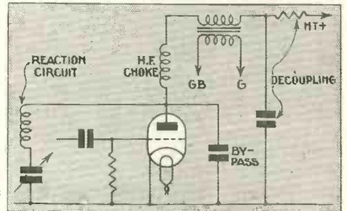
Fig. 8.—Transformer-coupled circuit with addition of high-frequency choke and anode by-pass condenser
