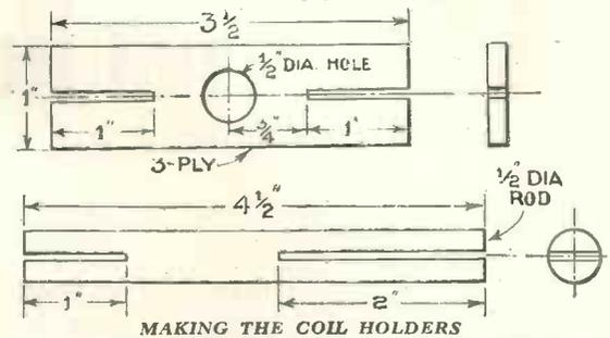
Fig. 6a.—Details of the coil holders, which are made from three-ply wood and  $\frac{1}{2}$ -in. rod
