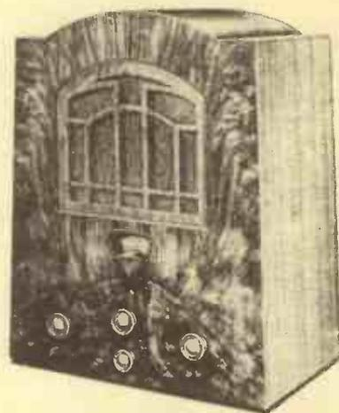
An all-electric three-valver, the Brownie Dominon receiver. It has a moving-coil loud-speaker
