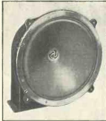
For the Seventy-Seven Super it was decided to utilise the Baker standard model permanent-magnet moving-coil reproducer, of which a photograph appears above. This loud-speaker is provided with an output transformer.
