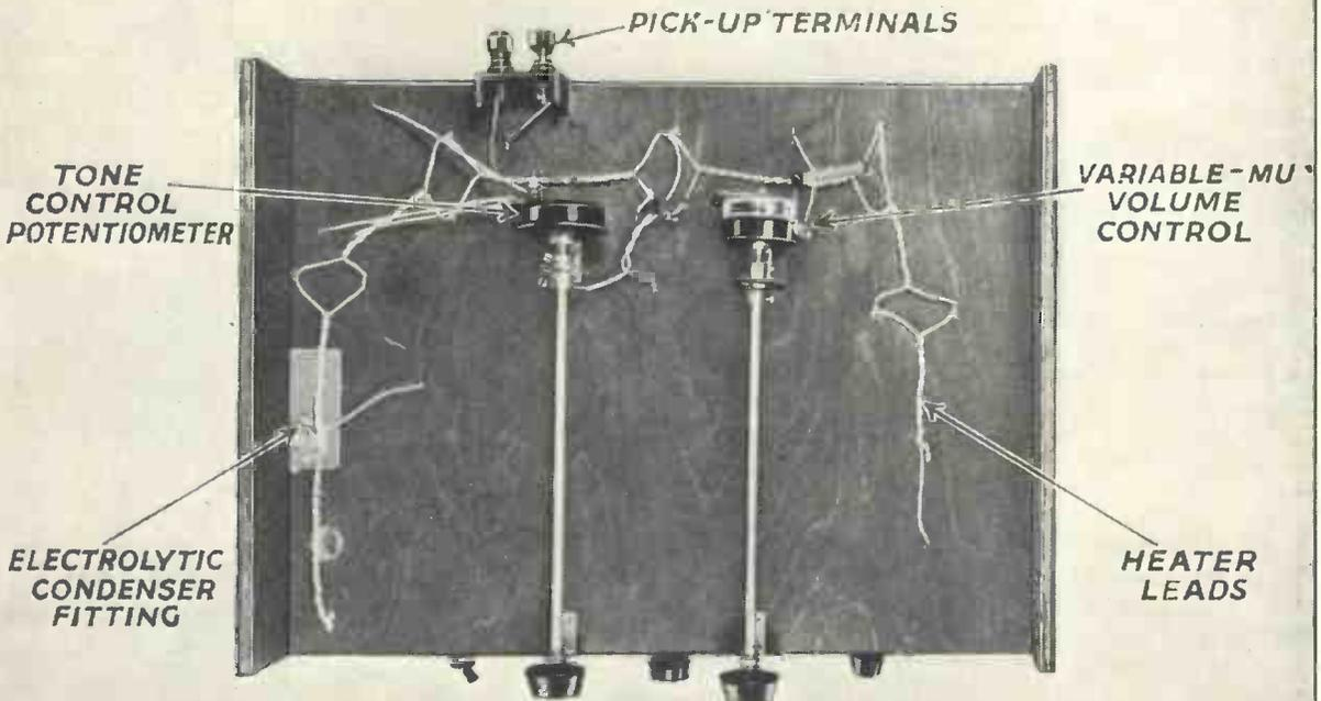
A view of the under side of the baseboard-chassis showing the potentiometers for radio volume control and for tone control. In this way long leads are avoided
