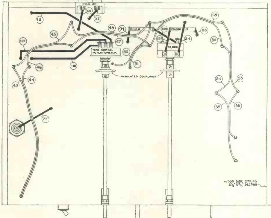
If desired a full-size blueprint can be obtained for half price, that is 9d., post free, if the coupon on the last page of the issue is used by December 31. When ordering ask for blueprint No. WM305. It should be noted that all the connecting wires are numbered separately in the best order of assembly; connect up in the proper numerical sequence and it will be impossible to make a mistake
