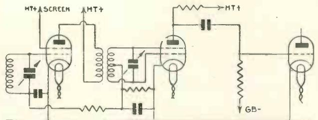
Fig. 10.—Automatic volume control with a Wunderlich valve detector
