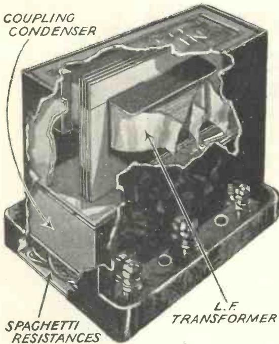
A sectional view of the Bulgin Transcoupler, one of the first examples of the parallel-feed transformer. Note the use of spaghetti resistances
