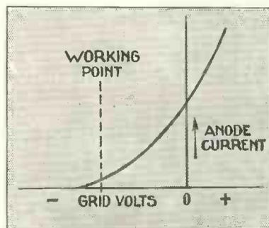
Fig. 2.—Typical characteristic valve curve, showing position for anode-bend working
