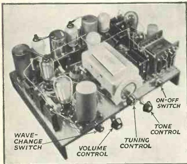
HOW THE CONTROLS ARE ARRANGED
