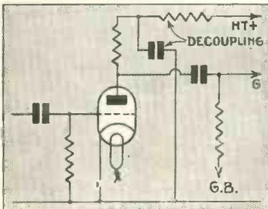
Fig. 4.—Decoupled detector circuit with resistance coupling to next valve
