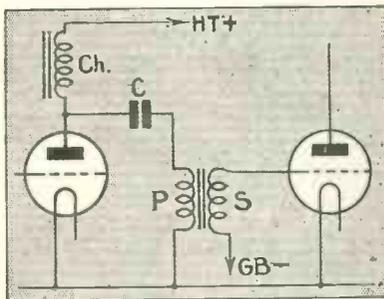
Fig. 1.—Valve anode circuit with iron-cored low-frequency choke
