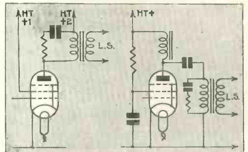
Fig. 5.—Output circuits for pentode valve, with and without a choke-condenser filter
