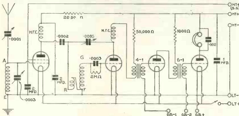
NEW SCREEN-GRID FOUR-VALVE CIRCUIT
