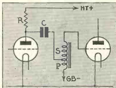
Fig. 3.—A further modification with the primary and secondary of the transformer connected together
