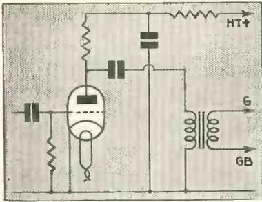
Fig. 7.—Transformer circuit with resistance feed to conserve the primary inductance at a high value
