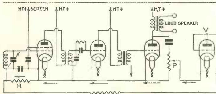
Fig. 11.—Automatic volume control operating from an extra valve controlled by the output circuit
