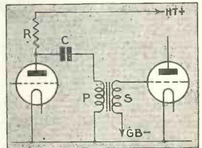
Fig. 2.—A high resistance substituted for the low-frequency choke of Fig. 1
