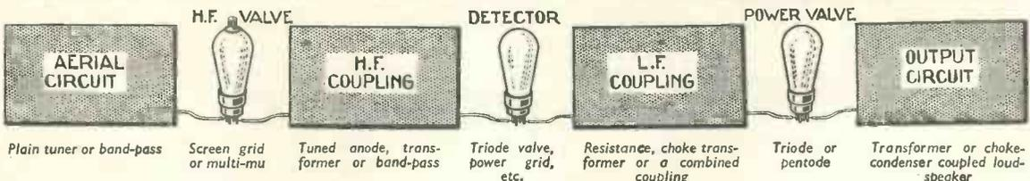
Fig. 1.—Skeleton layout of three-valve circuit with the chief combinations indicated
