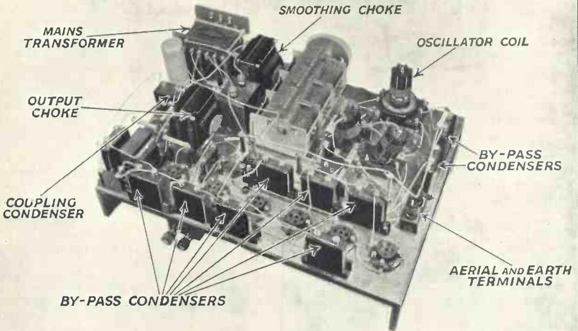
A back view of the Seventy-seven Super showing how well laid out the parts are. Although the set looks big there are no snags in the construction
