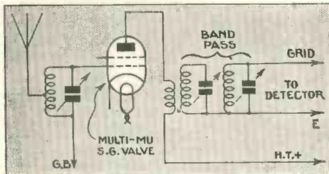
Fig. 9.—Circuit with band-pass tuning between a variable- $\mu$  valve and the detector
