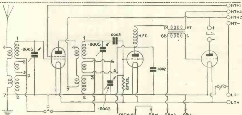
The valve combination consists of a screen-grid detector and a power stage
