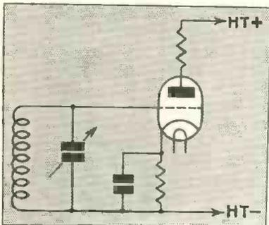
Fig. 1.—Typical circuit for an anode-bend system for A.C. working
