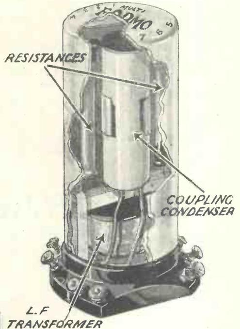
The low-frequency transformer is placed at the bottom of the case of the Formo Multicoupler, which has a tubular coupling condenser
