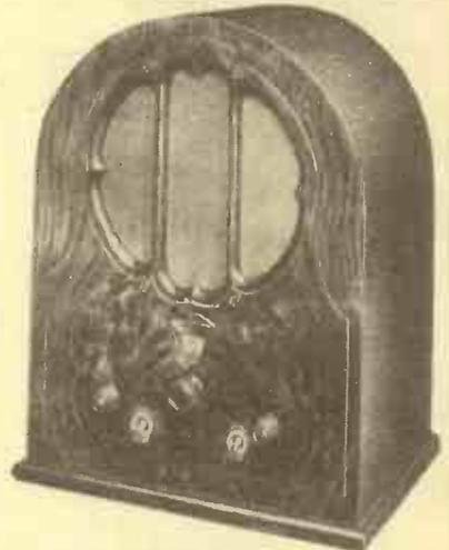
Cossar model 221 De Luxe, a battery two-valver. The loud-speaker adjustment is at the back
