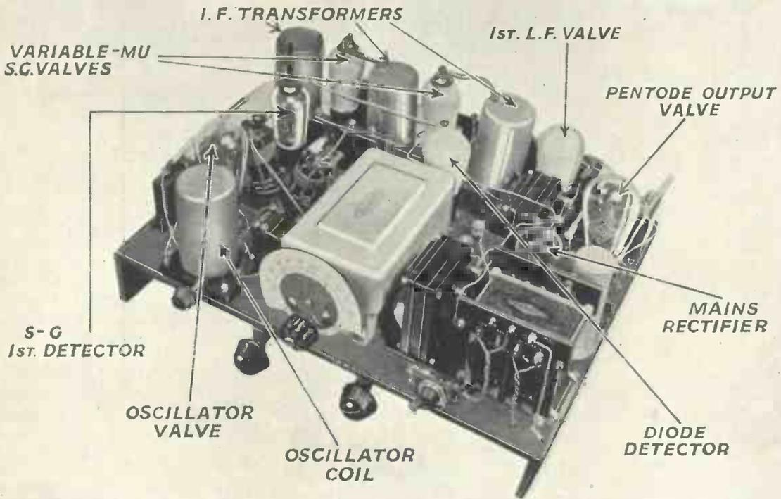
Here is the completed assembly of the Seventy-seven Super with all the valves and coils in position. The top of the baseboard is covered with metal foil
