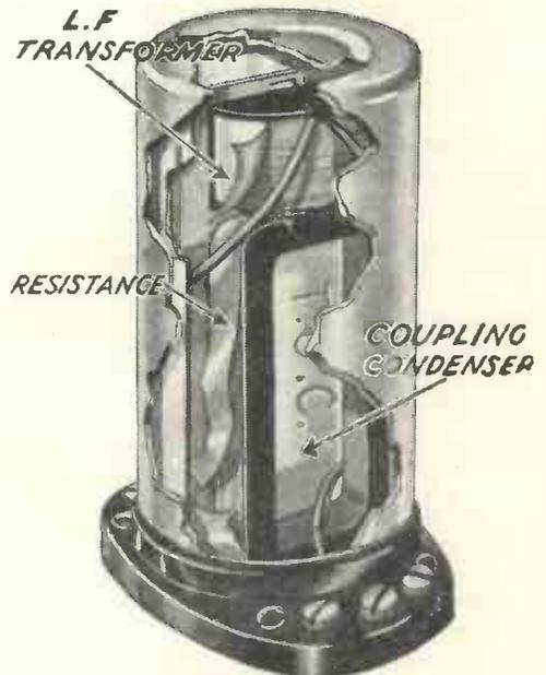
In the Benjamin Transfeeda the coupling resistance is wound on a special bobbin, as shown in this sectional view
