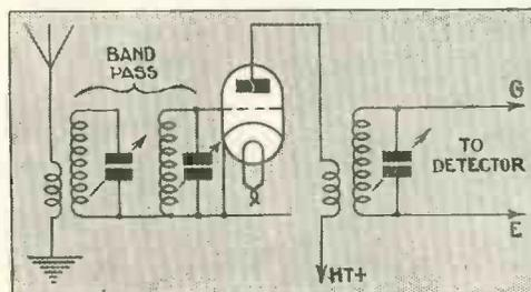
Fig. 10.—Circuit with band-pass tuning between the aerial and the valve
