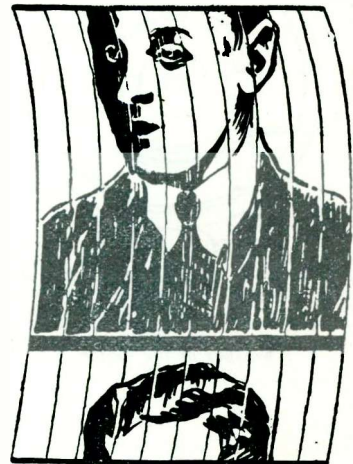
If the picture is split horizontally a very slight alteration of speed will correctly frame the image
