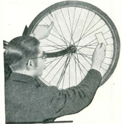
A card held against a rotating bicycle wheel produces a pitch which varies with the speed of the wheel, illustrates note frequency
