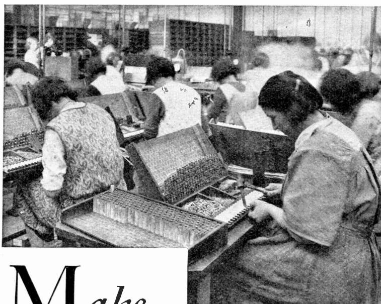
The G.E.C. have a huge factory at Coventry devoted to the manufacture of high-tension batteries. Here workers are seen soldering the wander-plug sockets to the finished 1.5-volt cells
