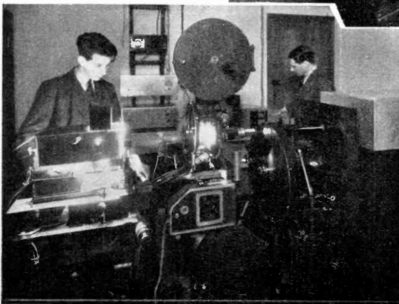
The older mechanical scanning of c.n. film for television transmission. Even by this method results showing considerable detail could be obtained.
