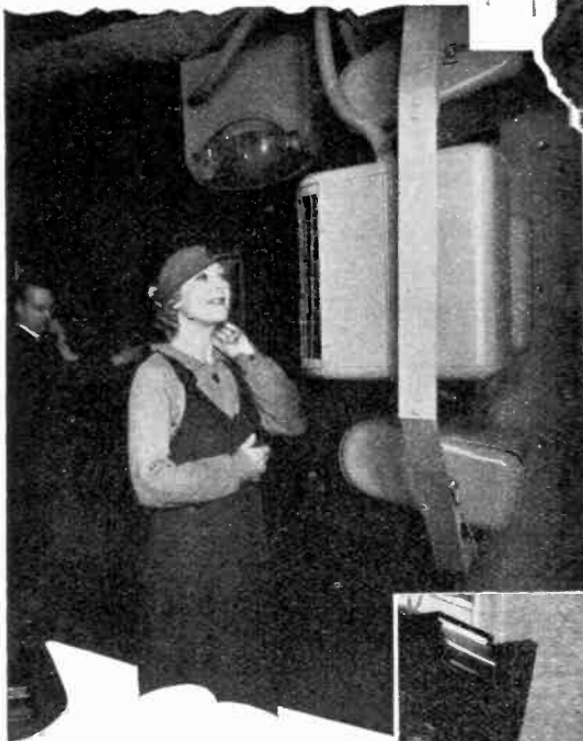
Miss Alma Taylor televising a new hat. The photo-electric cell's are enclosed in the white casing. Spotlight scanning is being used above the artist
