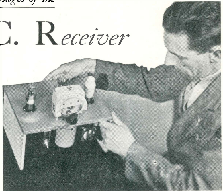
The photograph on the right shows one of the experimental models of the new "Unicon" two-valver. Full constructional details of this efficient receiver will appear in our next issue
