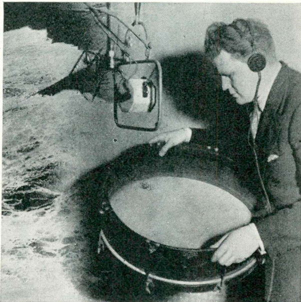
A sound rich in transients is that of the sea beating on the shore. Such sound is "manufactured" for broadcasting purposes by means of a drum containing lead shot slowly rocked in front of the microphone
