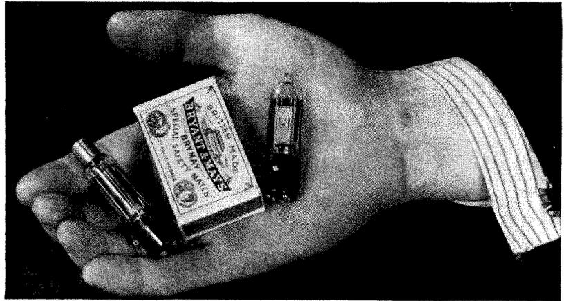
A couple of the Hivac midgets compared with a familiar object. Those actually used in the set are of the type with pins instead of the button contacts seen here
