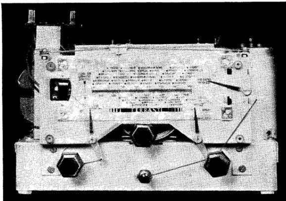
"... The all-in tuning scale on which one can see whether the station being received is correctly tuned in, tone-control setting, together with a calibrated scale in wavelengths and stations"
