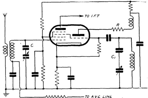
Fig. 2.—Triode-hexode frequency-changer for short waves. The condensers C and C<sub>1</sub> serve to restrict tuning ranges and resistance R prevents "squegging"
