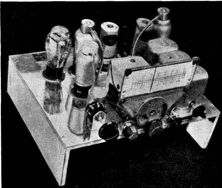
There are five controls for the Varsity Four. From left to right they are: combined on-off switch and volume control, local-distance switch, main tuner, variable selectivity control and wave-change switch. The tuning scales calibrated in metres
