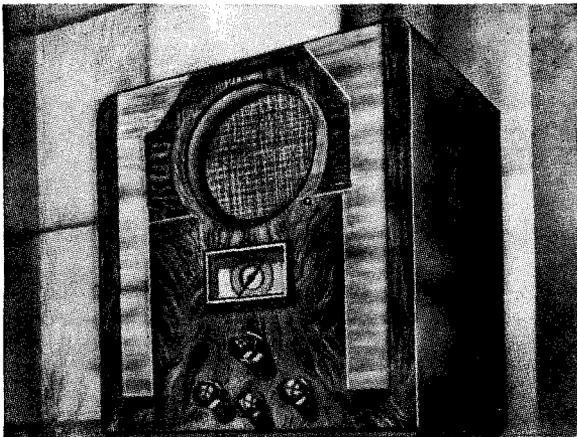
Prices of efficient all-wave receivers have tumbled this last few months. This R.A.P. all-wave superhet, which covers a waveband of from 19.5 to 52 metres in addition to the normal broadcast bands, is for operation off either A.C. or D.C. mains and costs twelve guineas
