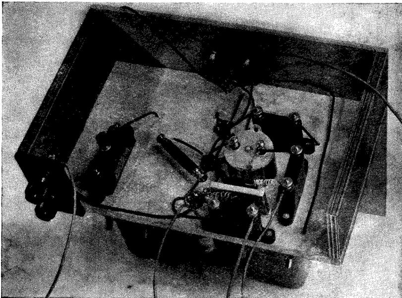
One of the virtues of the Minitube design is that compactness has not been taken to unpractical lengths and there is no awkward cramping together of the components
