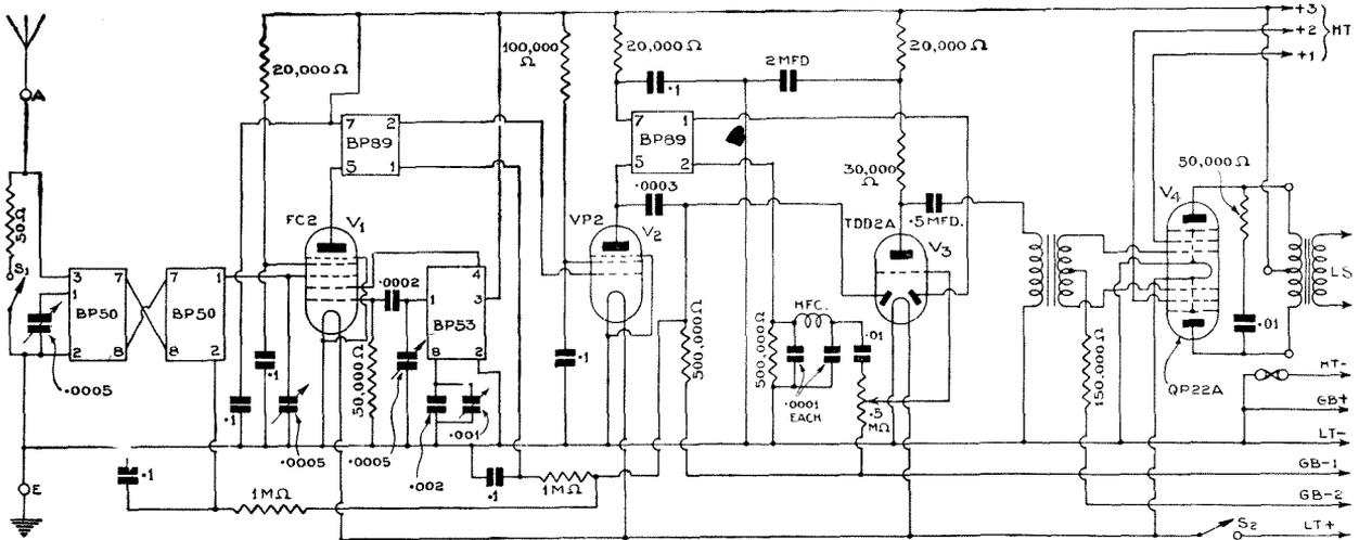
The theoretical circuit of the Varsity Four. It follows straight forward lines with two pre-selector circuits working into an octode frequency changer: then follows a high-frequency pentode as the intermediate-frequency amplifier and a double-diode-triode second detector feeding into a Q.P.P. output stage
