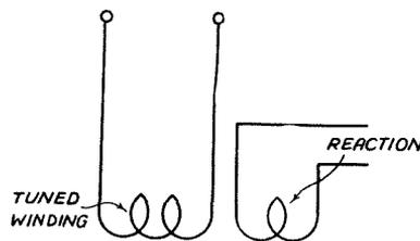
Fig. 4.—In short-wave receivers it is often necessary to take account of mutual inductance effects between the leads running to reaction and tuning coils as well as between the coils themselves
