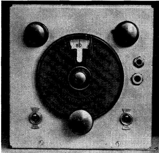
The metal front of the case carries the controls, set out as follows: top left, wave-range switch; top right, output strength; bottom left, audio-frequency on-off switch; bottom right, main on-off control. The two jacks provide the necessary inlet and outlet points. (See circuit diagram)
