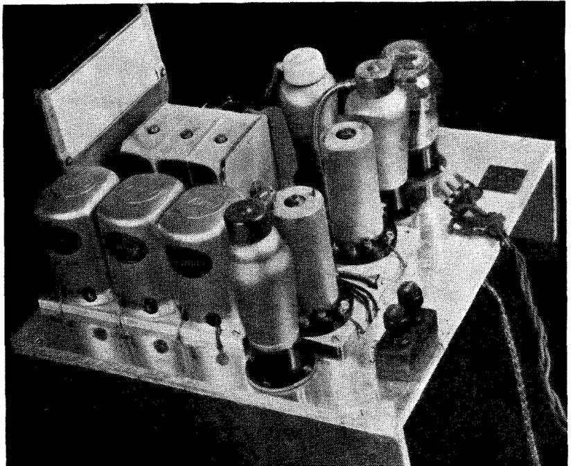
This view of the Varsity Four emphasises the business-like nature of the design. The three coils seen on the left comprise the two band-pass and the oscillator coils, but note carefully that the oscillator coil is mounted in the centre
