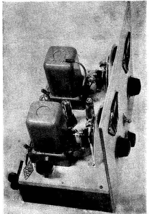
A wooden panel is used and the intention is that this shall be polished to harmonise with the cabinet finish. When finally fitted up the wave-change switch will be controlled from a knob on the side of the cabinet with the aid of a coupling to the rod passing through the coil units
