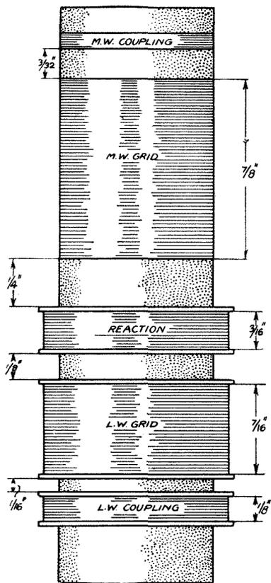
The coil is wound on a small piece of 1-in. diameter tube; note carefully the spacings between the windings
