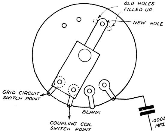
This sketch shows how the special wave-change switch is arranged and connected
