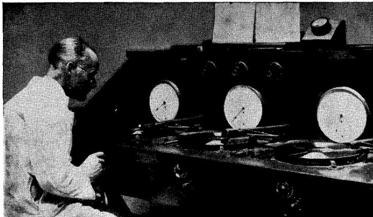
This is the apparatus used at the H.M.V. recording studios for transferring sounds from one or more records for embodying in a new record. Excerpts from up to three records can be re-recorded at once, faders being used for control
