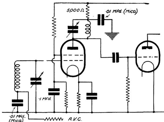
Fig. 6.—A simple form of tuned-anode circuit for direct high-frequency amplification on short waves
