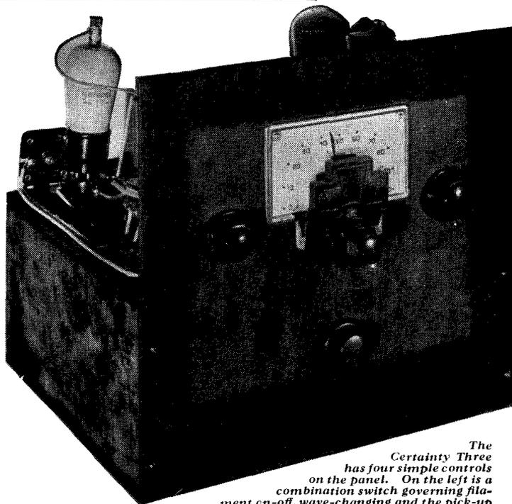
The *Certainty Three* has four simple controls on the panel. On the left is a combination switch governing filament on-off, wave-changing and the pick-up circuit. The tuner is above the reaction condenser in the centre while the volume control is on the right.
