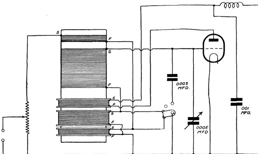
This diagram of the connections of the high-frequency oscillator valve provides a key to the start-and-finish sequence of the coil windings
