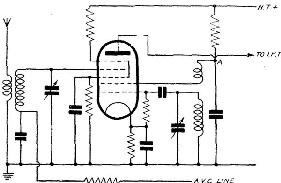
Fig. 1.—A simple pentagrid circuit for short waves. The voltage on A must be well above the voltage on the screen to ensure the most favourable working conditions
