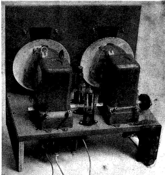
The only terminals required are those for aerial and earth; the loudspeaker is connected direct to the terminals of the fixed condenser, seen near the back of the underside of the baseboard
