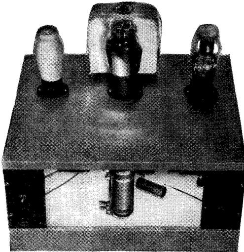
Considerable care was taken in the design of the Unicon Two to provide adequate space and ventilation for the main voltage-dropping resistance. Any cabinet used for the set should be provided with openings in the back (covered with wire gauze or perforated zinc) to maintain this feature
