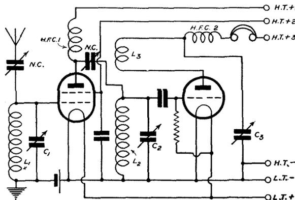
Fig. 3.—A two-valve short-waver with a high-frequency amplifier and leaky-grid detector. There is no difficulty in ganging the condensers  $C_1$  and  $C_2$
