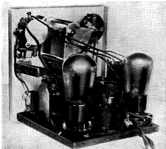
The exact layout of the parts is not important so long as undue liberties are not taken, but the placing shown here leads to simple assembly and wiring
