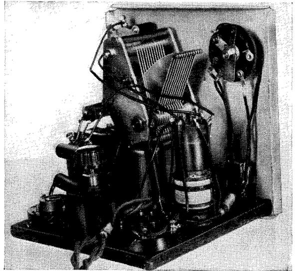
The potentiometer controlling the reaction effect in the audio-oscillator circuit is mounted inside the unit in the position shown here
