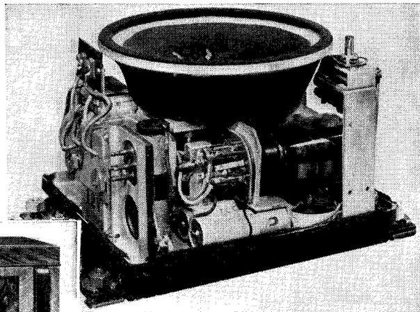
Showing the loud-speaker and vibrator unit of the new 20-guinea Marconiphone car-radio outfit. The compactness of the unit can be gauged by comparing the size of the valve with the loudspeaker
