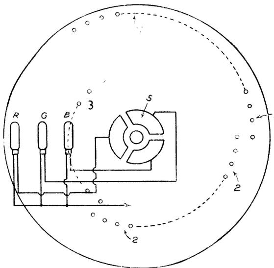
Fig. 2.—Illustrating the basic arrangement for three-colour scanning by means of the disc system
