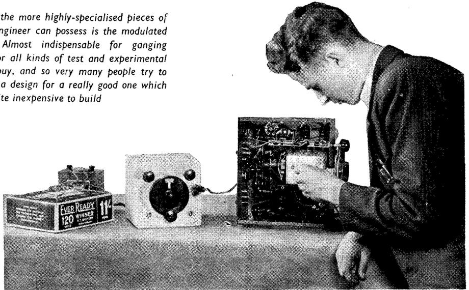
**L**ITTLE useful service work can be carried out on the modern receiver without the aid of a signal generator. A signal generator, as the name almost implies, is in reality a miniature transmitter. When a signal generator is very simply constructed it is generally referred to as a modulated oscillator.
