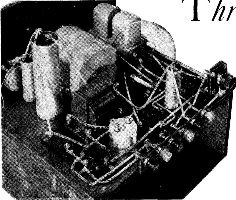
This view of the Certainty Three shows very clearly the layout of the components and wiring on top of the wooden chassis. The batteries are accommodated underneath
