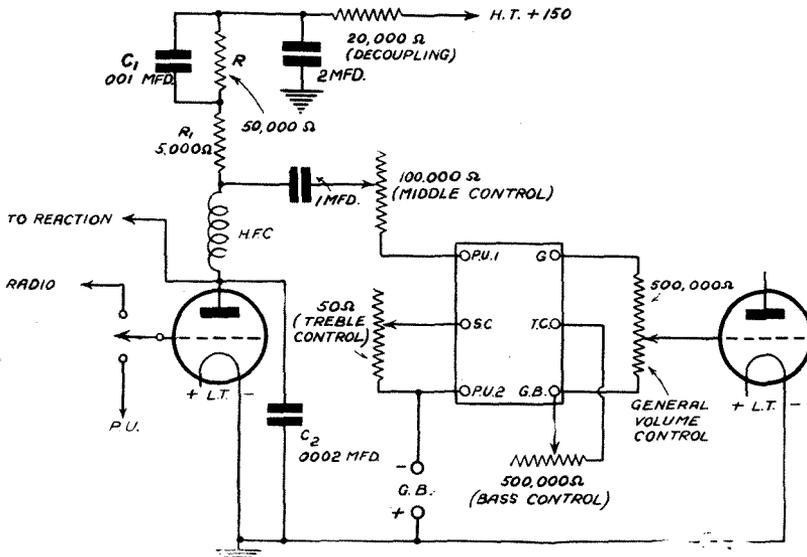
Fig. 2.—The theoretical circuit of the tone-control system recommended by the author; the bass and treble controls work independently of each other and the main volume control has little effect on the whole of the response curve
