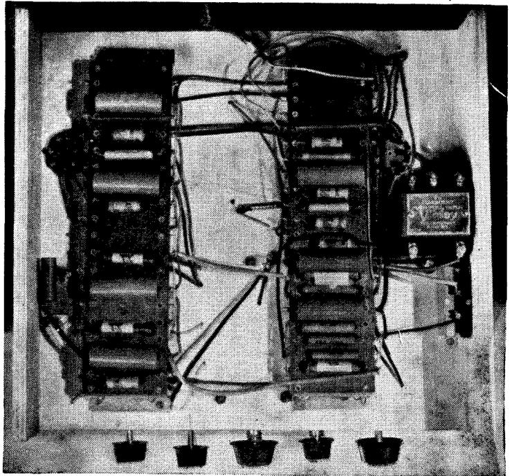
A view of the underside of the Varsity Four. It is important to note that wires of sufficient length must be soldered to certain of the valve holders before the resistance and condenser strips are mounted over them
