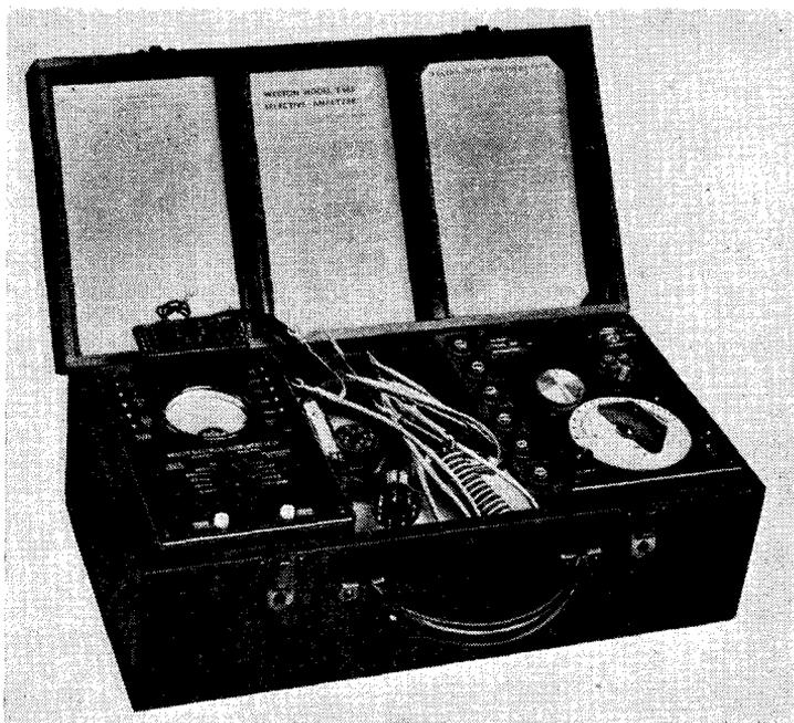
The sort of de-luxe equipment to make a service engineer's mouth water: a portable outfit incorporating the ever-useful Weston Analyser, sundry special gadgets and conveniences, and a type 562 oscillator.
