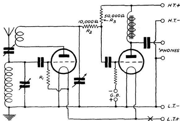
Fig. 1.—Probably the most common form of short-wave receiver, the straight detector-and-one-L.F. type
