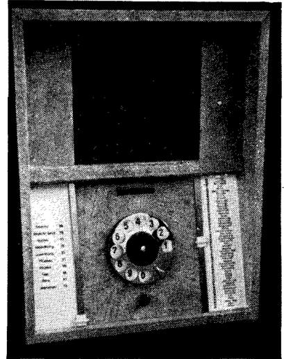
A novel tuner shown at the Berlin Show. The stations are listed on each side of the dial together with a number. When the number is dialed, the set automatically tunes itself to the required station
