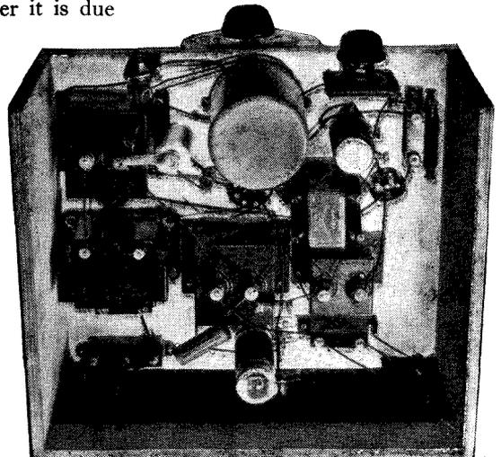
This view shows how space has been left in the assembly for any additional microfarads which may be required for hum-suppression
