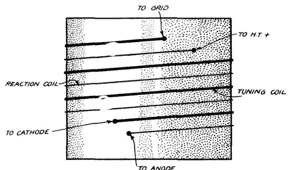
Fig. 3.—It is often helpful on short waves to interleave the reaction and tuned-grid windings
