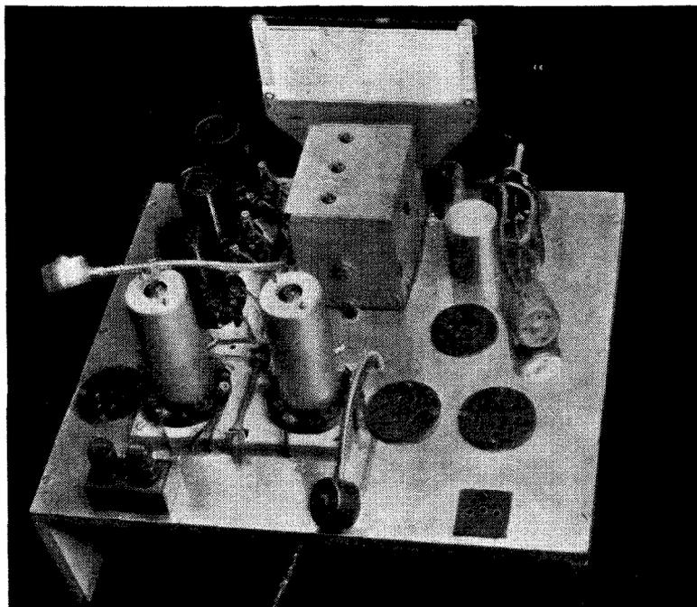
*This photograph taken minus valves and coil covers emphasises the simplicity of the layout on the upper side of the metal-covered wood chassis. Note the three-way socket on the front at the right for the loudspeaker connections*
