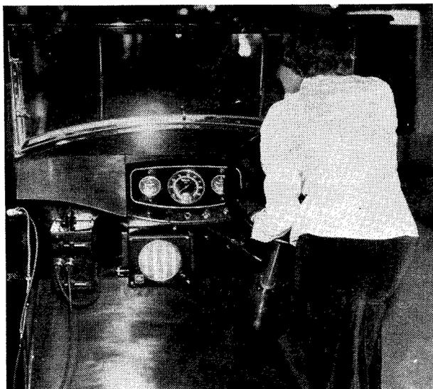
Marconiphone displays its first car-radio outfit in this novel setting at Olympia. Note the neat layout of the set and loudspeaker units
