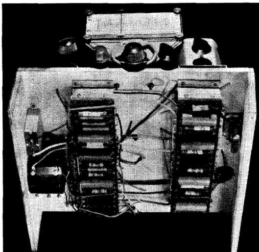
*The designer makes use in the Varsity Four of the same system of resistance and condenser mounting found so successful in the Stenode receivers. The condensers are mounted first of all on the strips before the latter are placed in position on the underside*
