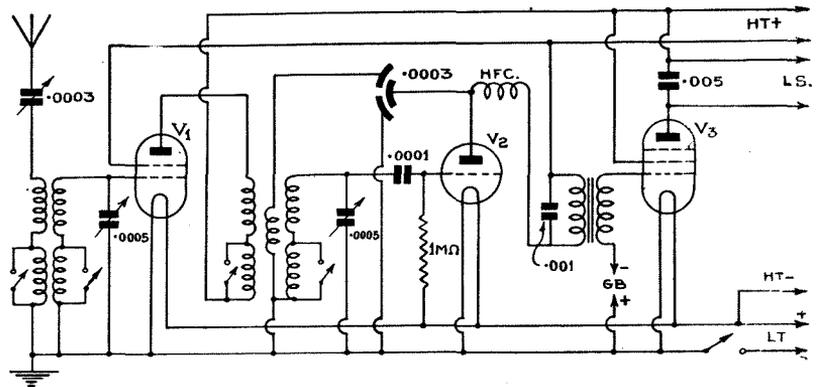
*Despite its small physical dimensions, the Minitube uses a full-sized electrical circuit with a hard-working stage of high-frequency amplification, differential reaction, and a pentode output stage giving very satisfactory volume and quality*
