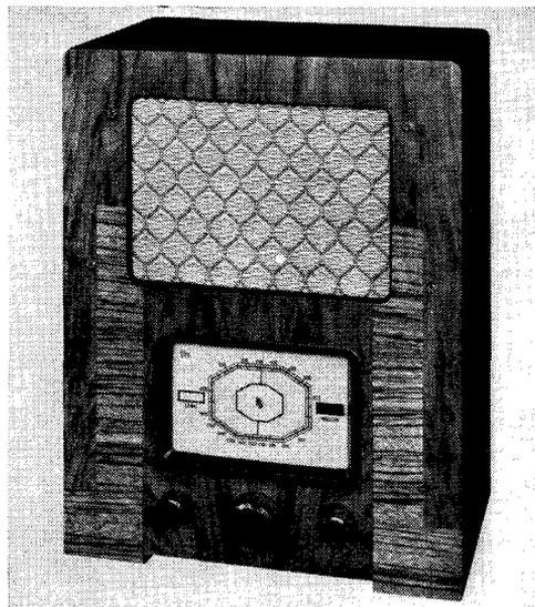
One of the new K.B. receivers, showing the Fototune dial. Note the two apertures where the station names appear
