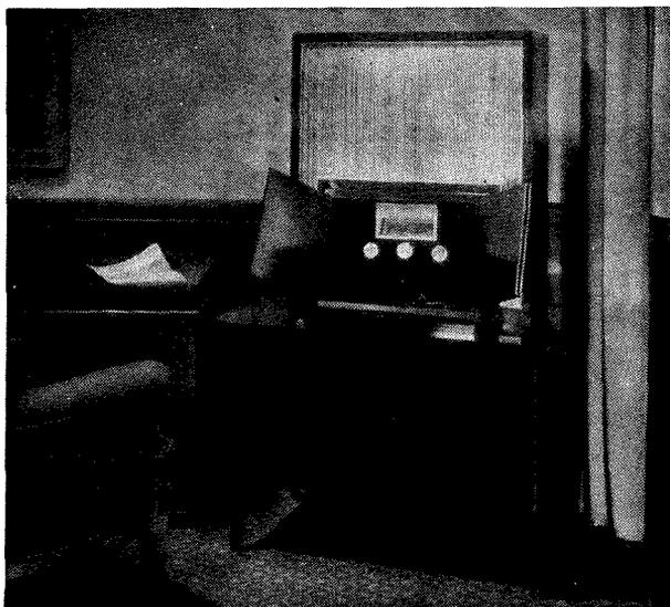
Germany's latest high-fidelity radiogram for local reception. Made by Siemens, the set employs two matched loudspeakers—fitted behind the screen at the top—operated by a four-valve "straight" circuit with a powerful push-pull output stage
