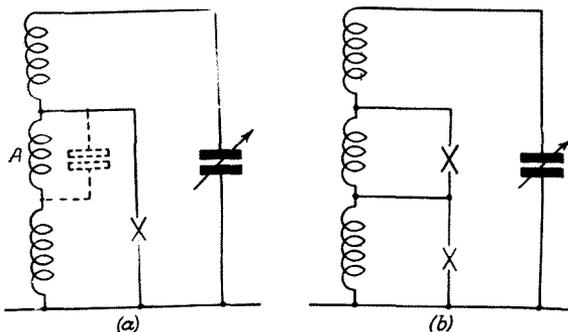
Fig. 5.—For real efficiency on short waves it is often necessary to elaborate slightly on the simple wave-change switching arrangement shown at A and use some such method as B
