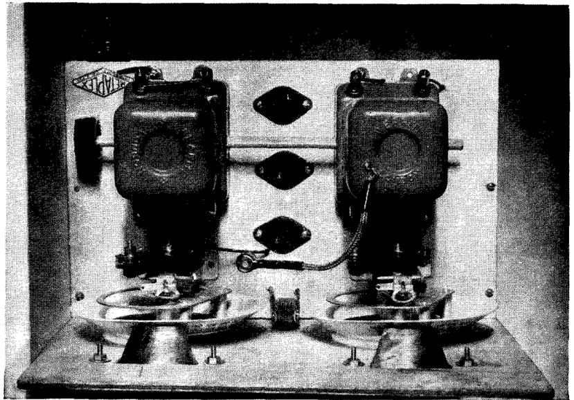
Note the flex lead from the right-hand coil unit. As supplied, this has a tag connector, but it is easy to remove this and solder in its place the special top connector supplied with the midget screen-grid valve
