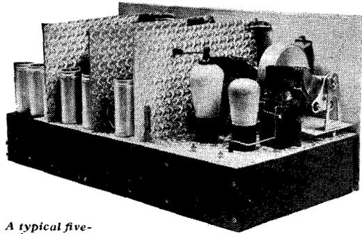
A typical five-valve short-wave super-het built by a member of the D.A.S.D., the German short-wave amateur's organisation. Note that a wooden chassis with an aluminium covered top is used
