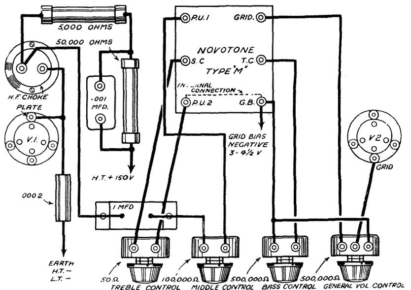
Fig. 1.—How the author arranged his friend's receiver with the four tone-control knobs on the panel to enable him to get quality suited to his own particular whims. The Gambrell Novotone plays a large part in the arrangement
