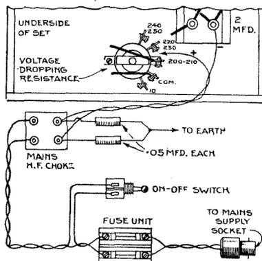
Schematic diagram illustrating the connections of various auxiliary devices to be fitted as required when the set is finally placed in its cabinet
