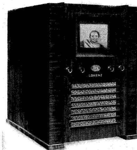
One of the Lorenz-Von Ardenne television receivers shown at the German radio exhibition. The sound channel employs a three-stage reaction circuit while vision is handled by a four-stage superhet arrangement. The picture size is roughly  $8\frac{1}{2}$  in. by  $7\frac{1}{2}$  in., and a cathode tube is used
