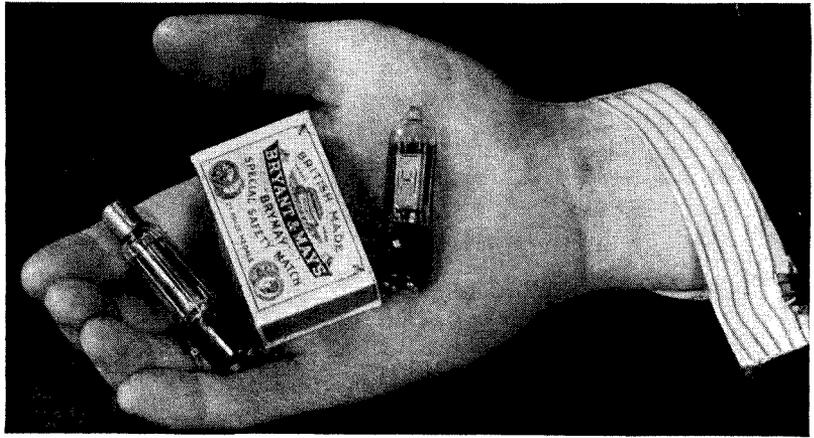
A couple of the Hivac midgets compared with a familiar object. Those actually used in the set are of the type with pins instead of the button contacts seen here
