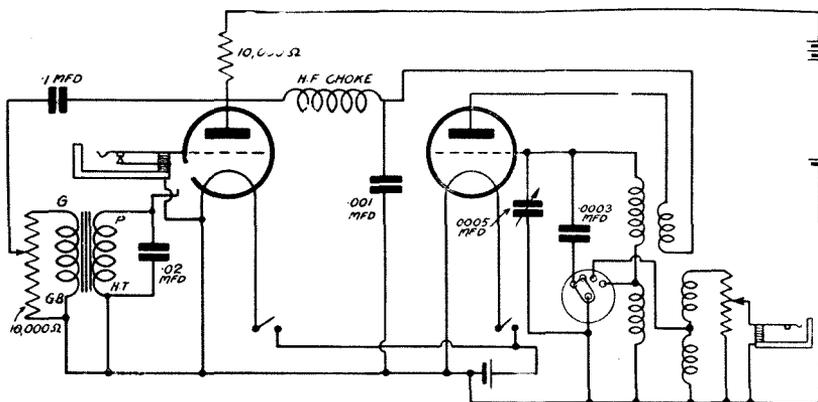
The complete circuit showing the high-frequency oscillator valve (right) and the audio-frequency generator (left). The jack in the grid circuit of the latter enables external modulation to be applied if desired
