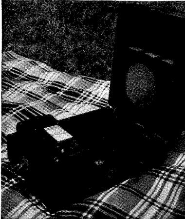
The modern German battery portable. This Korting model is a four-valver with moving-coil reproducer and costs 315 marks complete
