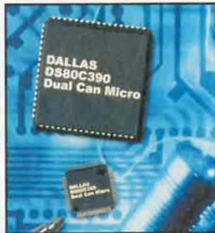
memory and 4Mbyte of external program memory. Applications include factory automation, marine control and navigation, industrial control systems, and HVAC control.
