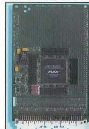
board based upon the Altera Flex 6000 family of programmable logic devices. The board provides a Flex 6000 quad-flat-pack device, onboard
