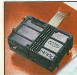
product can be supplied with a standard stack height or with a raised floor that lets components be mounted on the PCB beneath the connector. It is possible to use a variable thickness connector as the lower part. The connector is assembled using clip-on techniques and the module's spring contacts. *AMP*
