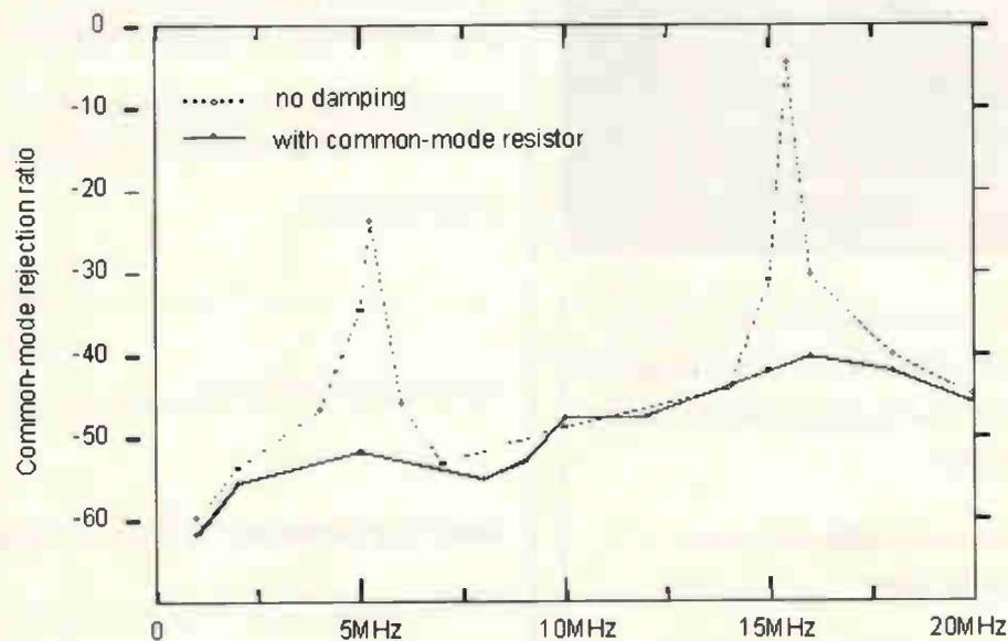
Fig. 10. Frequency response of floating configuration, again with and without the common-mode resistor.
