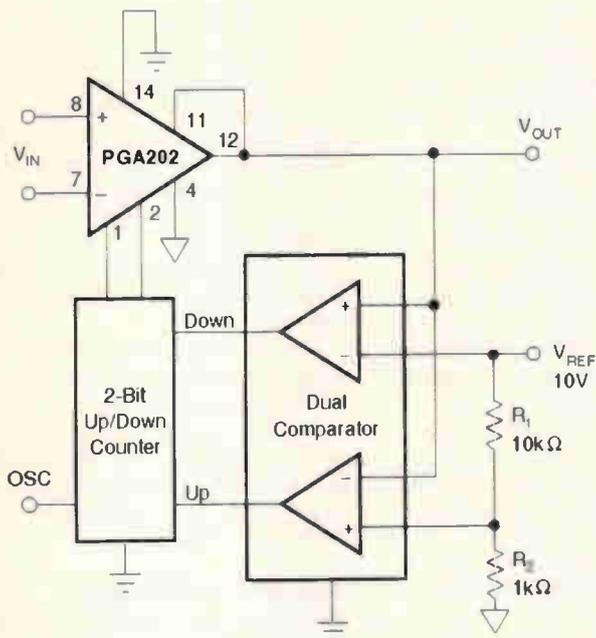
Fig. 1. Using a programmable-gain instrumentation amplifier as an auto-ranging gain control. The PG202 provides decade ranging steps. Its companion PG203, provides binary ranging.
