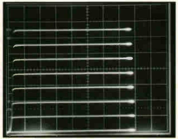
**Fig. 12.** Characteristics of a VN46AF N channel MOSFET, 1mA/div vertical, 2V/div horizontal, 1V/step  $V_{gs}$ , 12V nominal  $V_{ds}$ .
