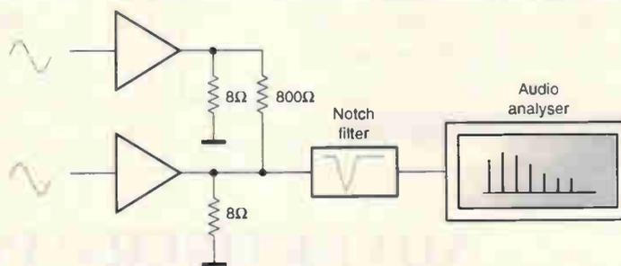
*A means of measuring 'load-induced intermodulation distortion'.*
