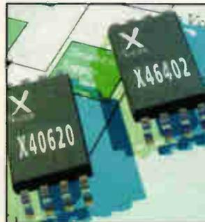
Both let the user select the low voltage reset trip points for the independent low voltage monitors. One monitor can be programmed from 1.7 to 3.5V and the other from 2.4 to 3.5V. The X46402 has user selectable security features such as memory partitioning and password protected memory. It also includes user selectable watchdog timeout selection intervals from 200ms to 1.4s. The watchdog timer function can be disabled for system software debugging.
