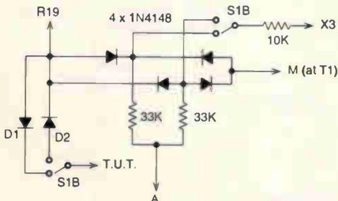
Fig. 5. An arrangement, one of several possible, for avoiding spot-burn when Z modulation cannot be used.
