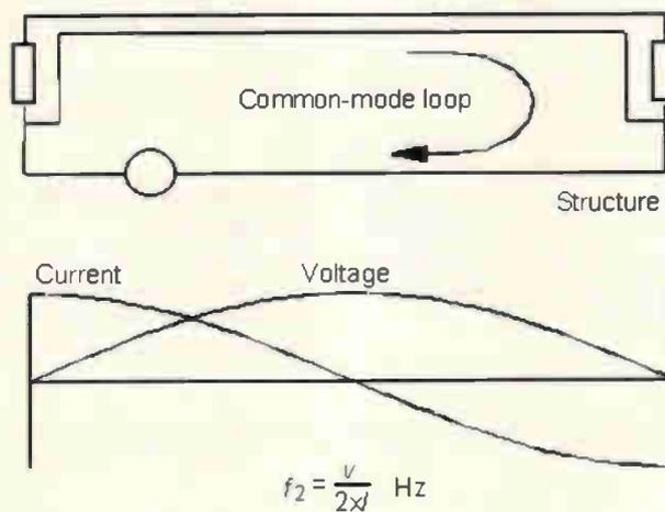
Fig. 4. Half-wave resonance response of the common-mode loop when both ends of the return conductor are grounded.
