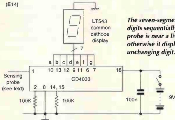
*The seven-segment display flashes digits sequentially when the probe is near a live conductor, otherwise it displays a single unchanging digit.*
