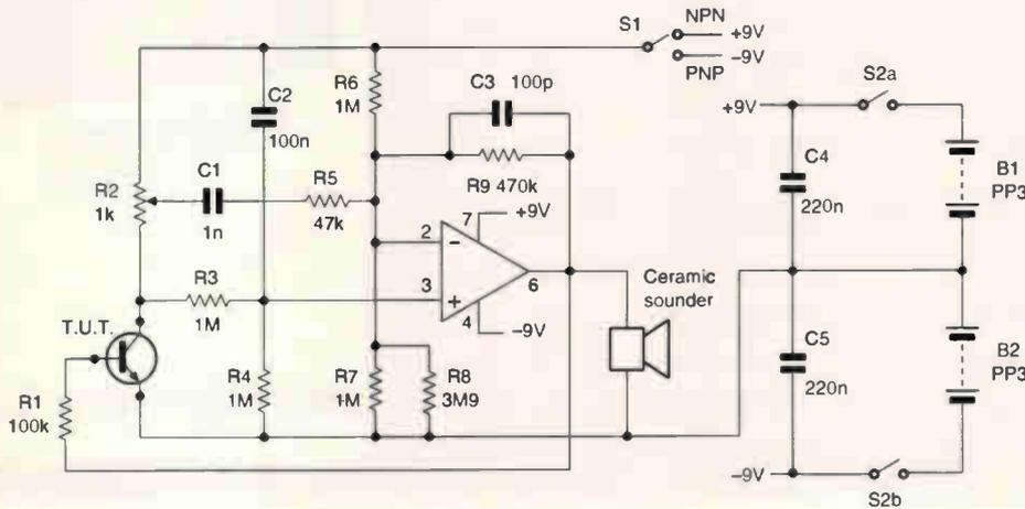
*This  $h_{fe}$  tester indicates the AC current gain of a transistor at the point where a tone is just audible.*
