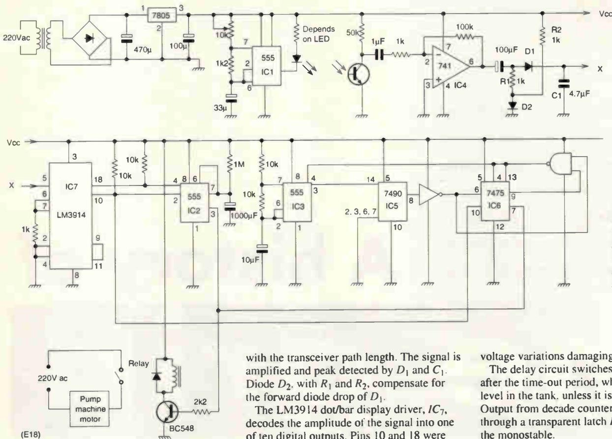
*This circuit maintains the water level between fixed limits and safely auto-restarts after a mains outage.*
