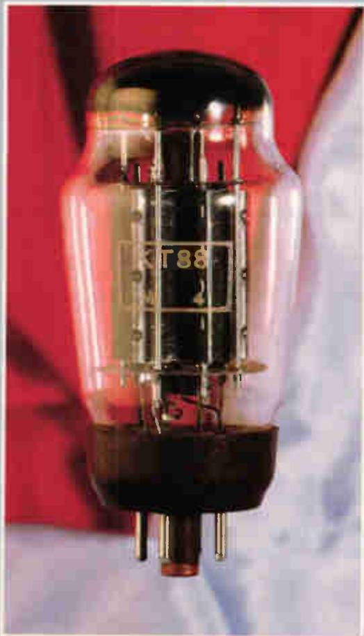
**W**hile the power efficiency of valves is largely determined by the performance of the cathode, other important properties depend on the nature and geometry of the valve's grid, or grids. These properties are gain, linearity, distortion, band width, and to some extent noise.
