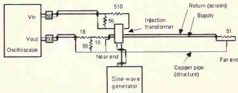
Fig. 5. Test set up for coaxial cable - grounded. Here, the 'supply' conductor is the core of a coaxial cable.
