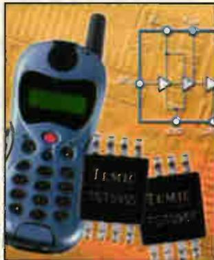
925MHz to 960MHz GSM mobile phones. The companion device, the TST0951 is designed for mobile phone applications in the frequency range of 1800MHz to 2000MHz. The LNAs incorporate a 2-stage amplifier and switchable gain and offer a noise figure of 2.2dB in high-gain mode. The large signal capability is the equivalent of IIP3 equal to  $-7\text{dBm}$  in low-gain mode, and
