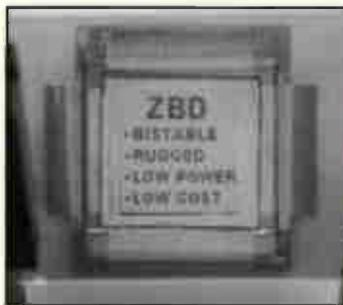
*Boinnng... DERA in Malvern is presenting a paper on its zenithal bistable device – ZBD – pronounced zebedee – an LCD which keeps its image after power is removed.*
