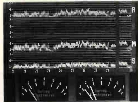
PPM10 In-vision PPM and Chart Recorder generates a display emulating the well known coaxial TWIN movements for monitoring stereo audio levels and mono compatibility. Also: **STEREO TWIN METER BOX** comprising two PPM9 boards, featuring inherent stability with low under microprocessor control. A free standing mains powered box frequently used for the final stereo monitoring when working to broadcast standards. Manufactured under licence from the BBC.
