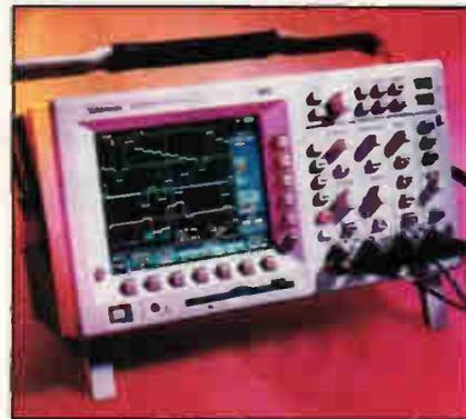
BT.601 digital video waveforms, allowing them to verify source, timing and amplitude. The module operates in TDS3000 series DPOs, and so is intended to provide digital video engineers with a single instrument for qualitative troubleshooting of digital video signals.
