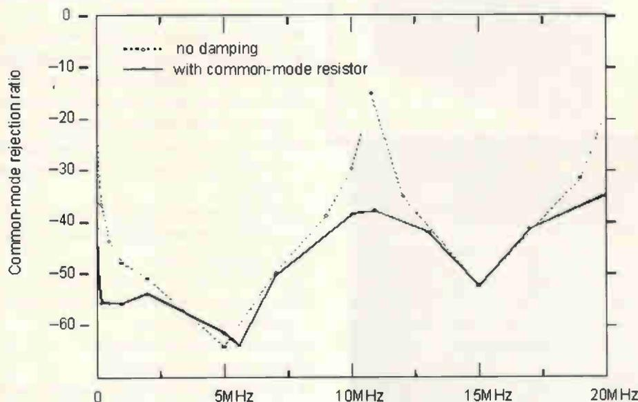
Fig. 9. Frequency response of grounded configuration, comparing results of testing the grounded configuration with and without the common-mode resistor.
