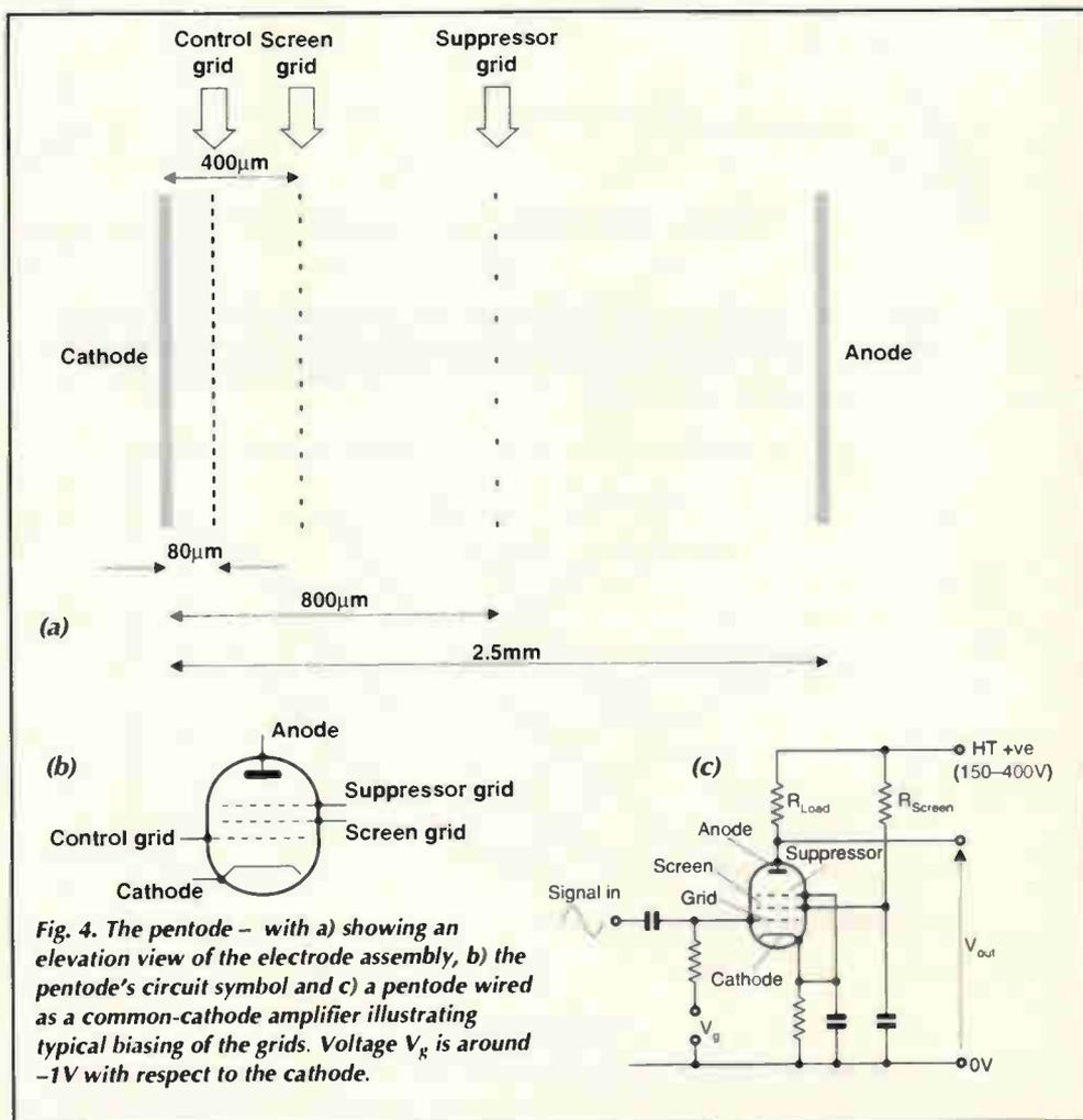
Fig. 4. The pentode - with a) showing an elevation view of the electrode assembly, b) the pentode's circuit symbol and c) a pentode wired as a common-cathode amplifier illustrating typical biasing of the grids. Voltage V<sub>g</sub> is around -1V with respect to the cathode.
