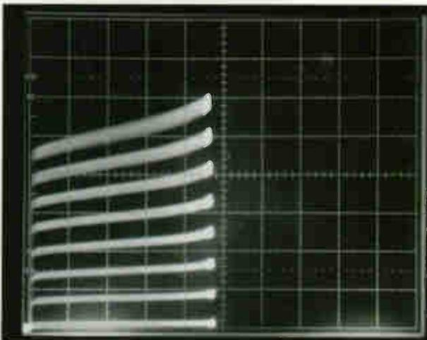
**Fig. 11.** Characteristics of a BC184B, 10mA/div vertical, 10V/div horizontal, 20 $\mu$ A/step  $I_b$ , 32V  $V_{ce}$  nominal.
