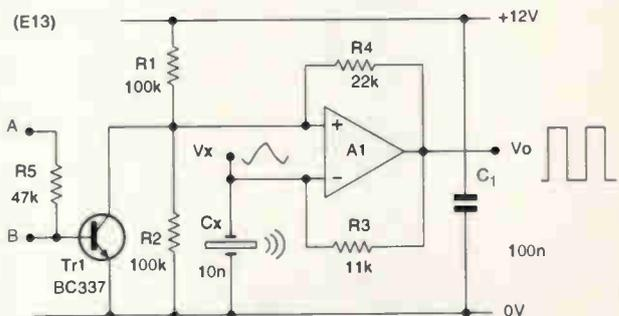
*The piezo ceramic sounder itself acts as the frequency-determining capacitor in this sounder circuit.*
