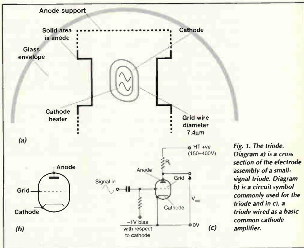
Fig. 1. The triode. Diagram a) is a cross section of the electrode assembly of a small-signal triode. Diagram b) is a circuit symbol commonly used for the triode and in c), a triode wired as a basic common cathode amplifier.
