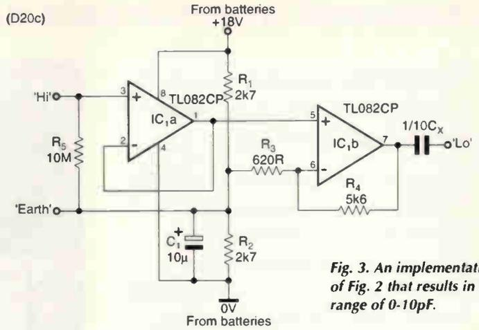
Fig. 3. An implementation of Fig. 2 that results in a range of 0-10pF.
