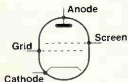
Fig. 2. Circuit symbol of a tetrode.
