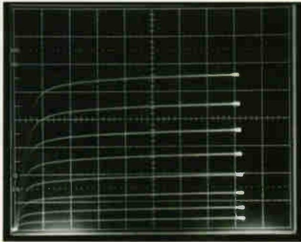
**Fig. 9.** Characteristics of an n-channel JFET: BF244A, nominal 12V  $V_{ds}$ , 1mA/div vertical, 2V/div horizontal, 0.2V/step  $V_{gs}$ .
