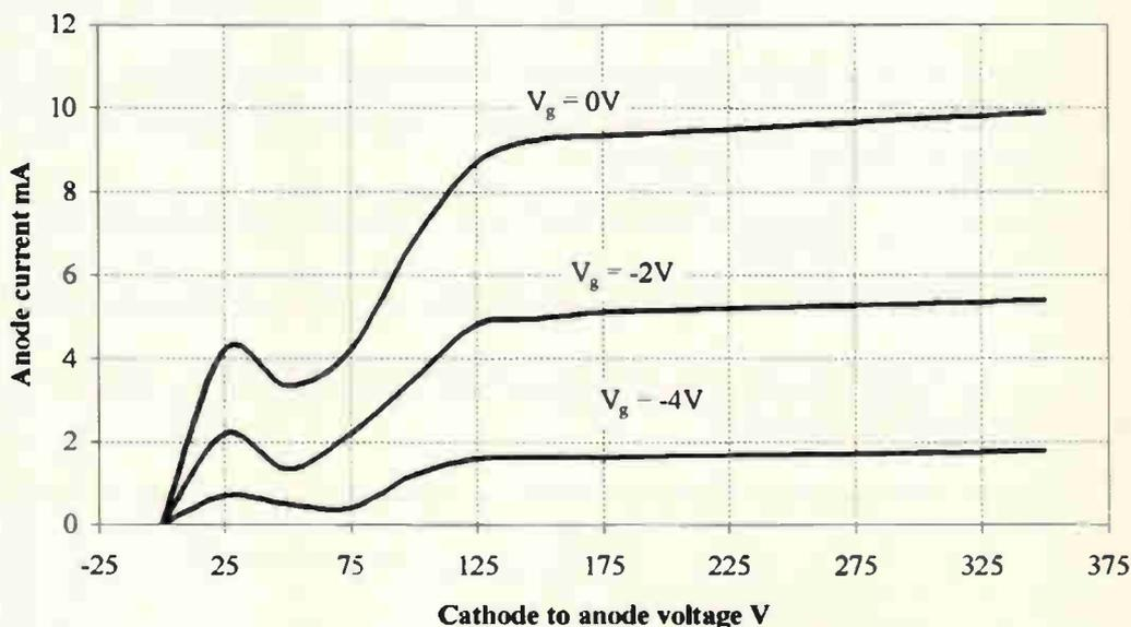
Fig. 3. V-I characteristic curves for a small-signal tetrode. The curves represent the relationship between anode current and anode voltage for various fixed control grid to cathode voltages (V<sub>g</sub>). The kink between 25 and 75V on the anode is due to the exchange of secondarily emitted electrons between the anode and screen. Notice the negative impedance between 25 and 50V.
