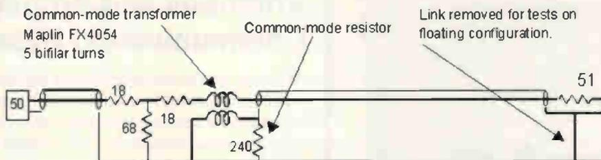
Fig. 8. Inserting a common-mode resistor.
