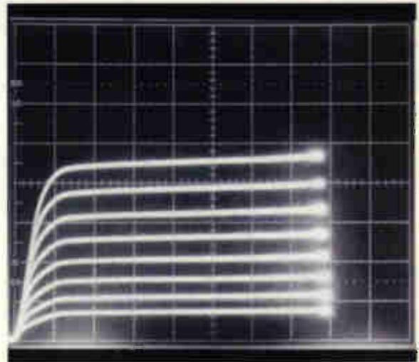
**Fig. 16.** Characteristics of an MEM614 dual-gate MOSFET, 2mA/div horizontal, 100mV/step  $V_{g1}$ , 16V nominal  $V_{ce}$ , see text.
