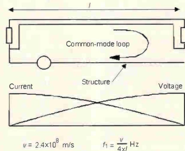
Fig. 3. Floating configuration at its first resonance point - i.e. quarter-wave.
