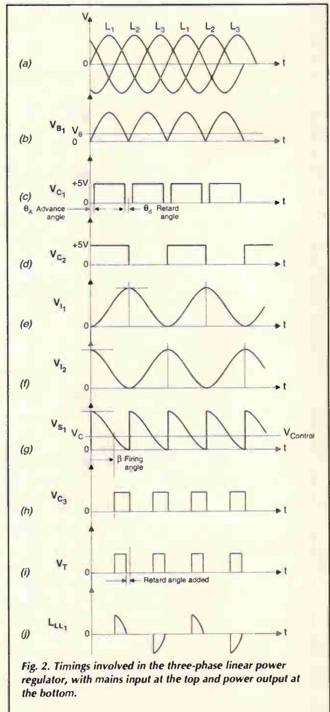
Fig. 2. Timings involved in the three-phase linear power regulator, with mains input at the top and power output at the bottom.
