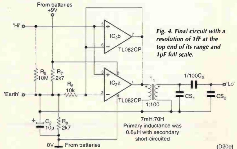
Fig. 4. Final circuit with a resolution of 1fF at the top end of its range and 1pF full scale.
