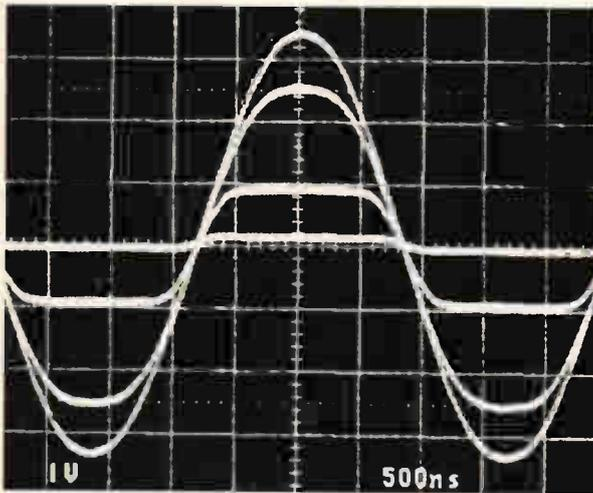
Fig. 4. Adjustable soft-limiting of this 200kHz sine wave was obtained by setting the  $V_{control}$  voltage to  $-5V$ ,  $-4V$ ,  $-3V$  and  $-2V$  in turn.
