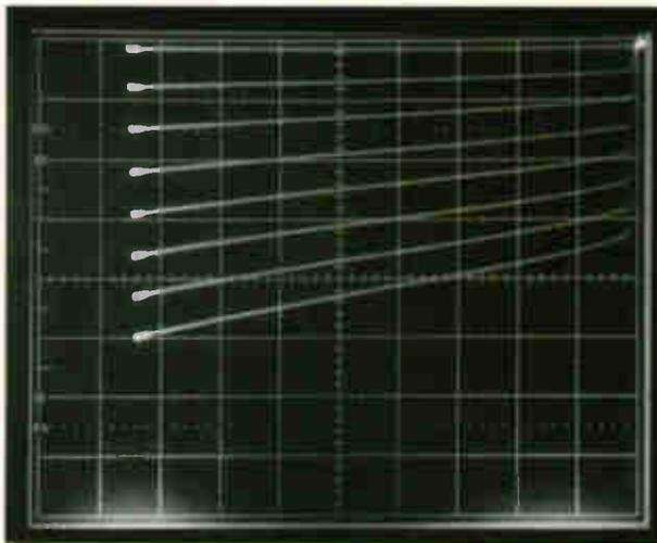
**Fig. 10.** Characteristics of a BC214L; nominal 12V  $V_{ds}$ , 1mA/div vertical, 2V/div horizontal, 2 $\mu$ A/step  $I_b$ .
