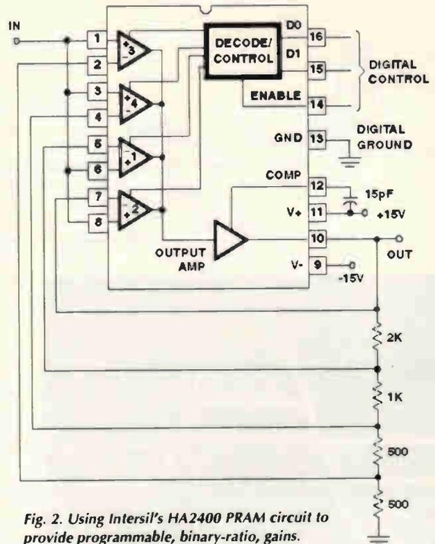
Fig. 2. Using Intersil's HA2400 PRAM circuit to provide programmable, binary-ratio, gains.
