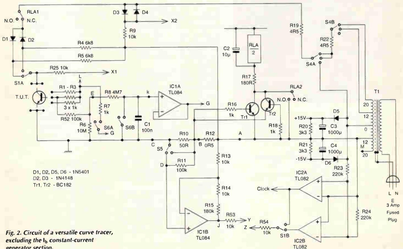
Fig. 2. Circuit of a versatile curve tracer, excluding the  $I_b$  constant-current generator section.
