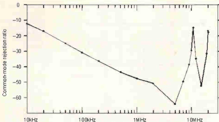
**Fig. 6. Frequency response of grounded configuration confirms that common-mode rejection at low frequencies is low, but useful.**
