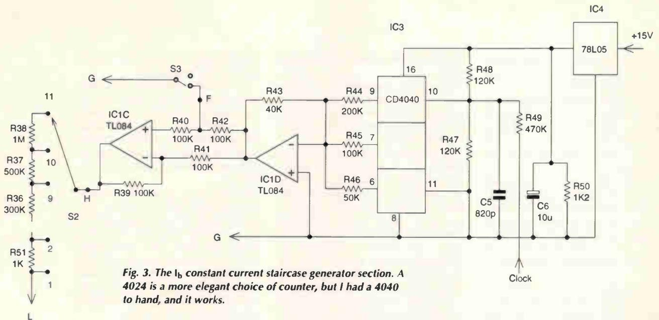
Fig. 3. The  $I_b$  constant current staircase generator section. A 4024 is a more elegant choice of counter, but I had a 4040 to hand, and it works.
