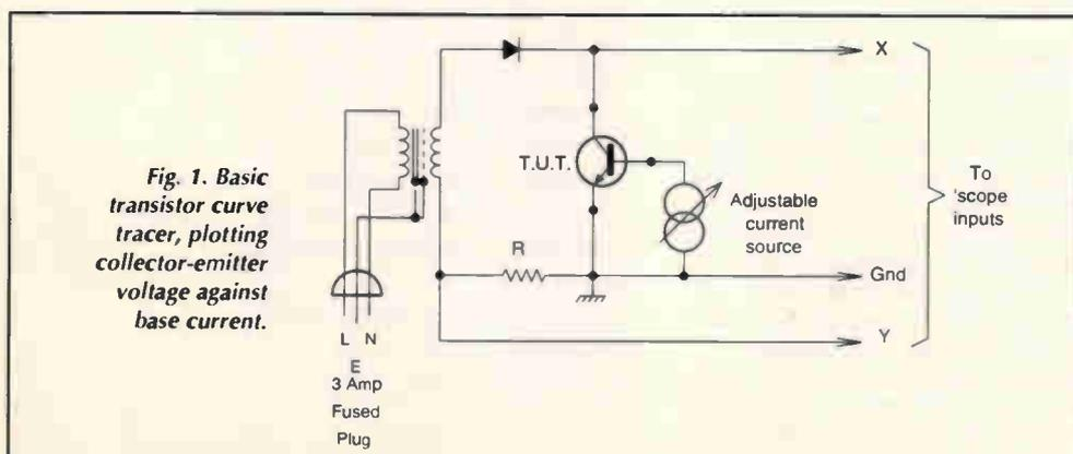
**Fig. 1. Basic transistor curve tracer, plotting collector-emitter voltage against base current.**
