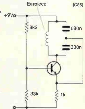
*An earpiece is used both as the sounder and the tank inductance in this audible tone generator.*
