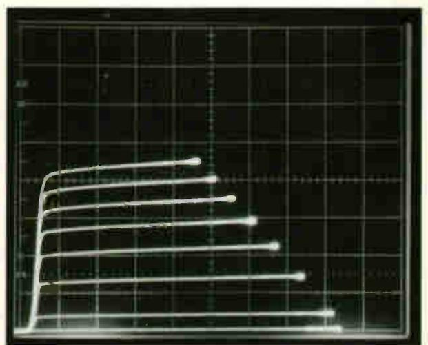
**Fig. 13.** Characteristics of a TIP41A n-p-n silicon power/switching transistor, 200mA/div vertical, 2V/div horizontal, 1mA/step  $I_b$ , nominal 12V for  $V_{ce}$ .
