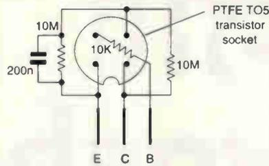
**Fig. 15.** Circuit diagram of an appliqué unit, used to permit the curve tracer to be used for evaluation dual-gate MOSFET devices.
