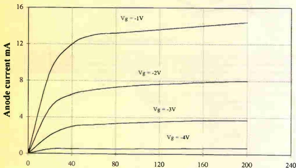
Fig. A. *V-I* characteristic curves for a small-signal pentode. The curves represent the relationship between anode current and anode voltage for various fixed control grid to cathode voltages ( $V_g$ ). The curves have similar shape to those of bipolar transistors and consequently pentodes have similar distortion characteristics to transistors.
