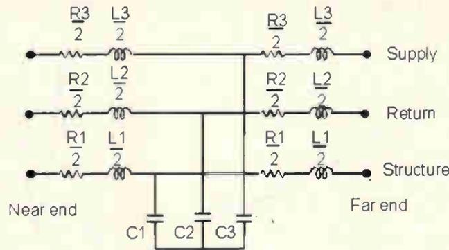
Fig. 2. Basic circuit model of three parallel conductors. This provides fair accuracy up to a quarter-wave frequency.
