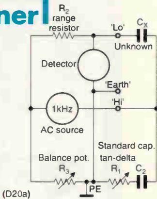
Fig. 2. Outline arrangement to extend the smallest range from 100pF maximum to 10pF maximum.
