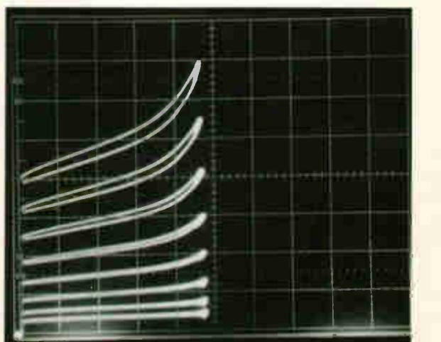
**Fig. 14.** Characteristics of a BC182, 2mA/div vertical, 10V/div horizontal, 20 $\mu$ A/step  $I_b$ , 32V nominal for  $V_{ce}$ , see text.
