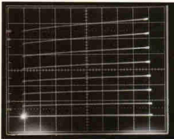
Fig. 4. Display of the  $I_b/V_{ce}$  characteristics of a BC108B, 1mA/div. vertical, 2V/div. horizontal. The excessively bright spot at the origin, where the beam rests for 50% of the time - with danger of spot-burn - is only too obvious.
