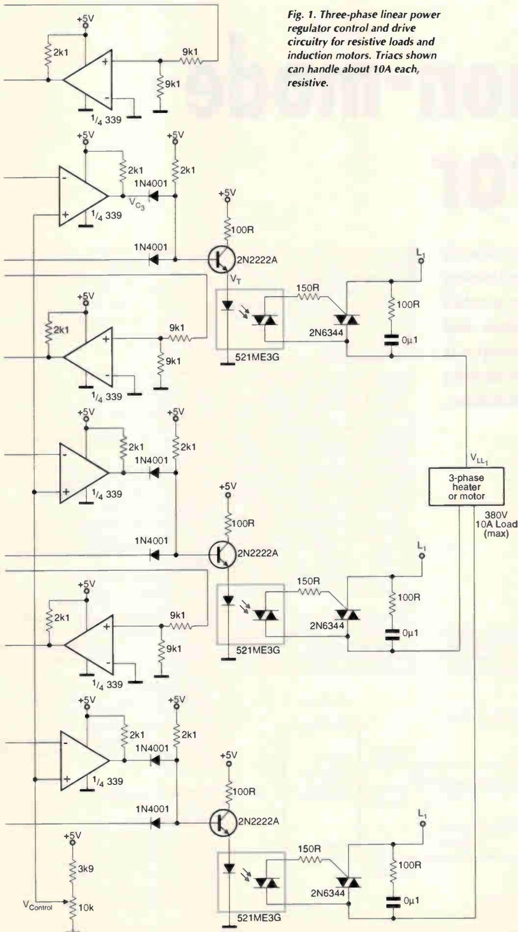
**Fig. 1. Three-phase linear power regulator control and drive circuitry for resistive loads and induction motors. Triacs shown can handle about 10A each, resistive.**
