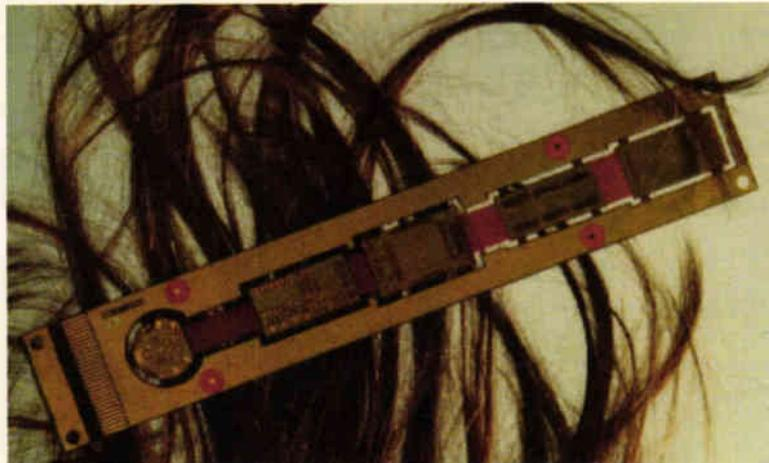
**Hearing aid... Micro-via PCB technology called DYCOstrate has been used to implement a programmable hearing aid by Swiss firm Sulzer Microelectronics. This hearing aid is the smallest of its type, the firm claims. The extreme packaging needs of a hearing aid led the firm to use the flexible substrate which can be folded up after manufacture. DYCOstrate is available in the UK through Rigid and Flex.**
