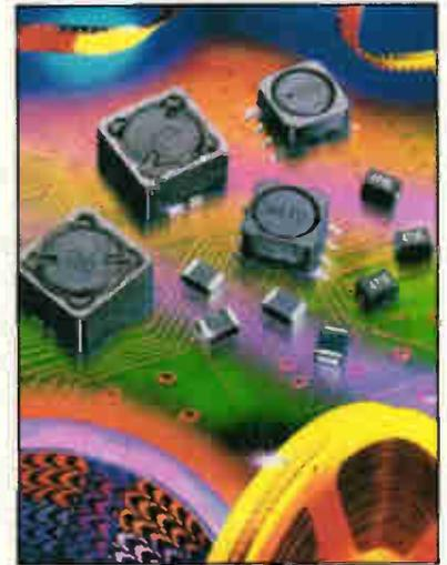
twelve sizes with different height to size to current ratios. The 3622's package is 5mm in diameter, with up to 1mH inductance. Lower values carry
