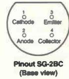
Fig. 4. Pin out of photoreflexive device used in the author's prototype (SG-2BC - Farnell code 441-566). Device diameter is 4mm.
