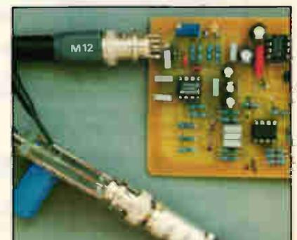
*To evaluate a capacitor for a modern switched-mode power supply, a good test jig is vital. Find out what Cyril Bateman uses on page 696.*
