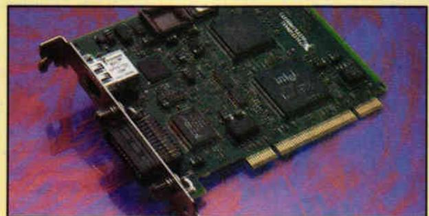
**GPIB and Ethernet Interface for PCI**
