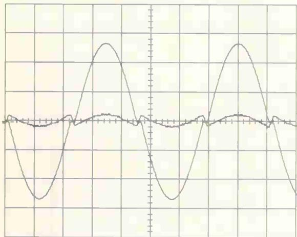
Fig. 5. The larger trace is the (distorted) output signal. The smaller is the distortion, measured as before, but the gain of one channel has been trimmed back, producing the same waveform as the THD meter output in Fig. 4. (The dead space steps in the output waveform are more clearly visible in this view than in Fig. 2.)
