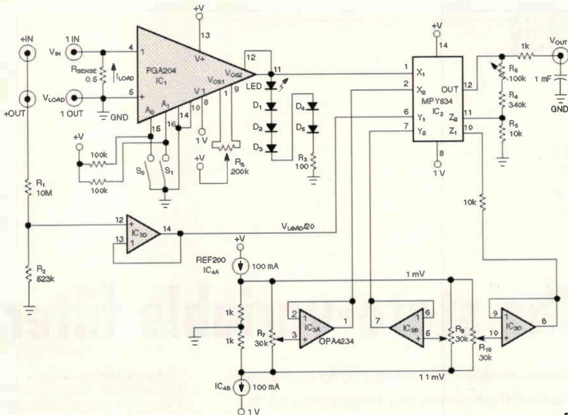
Fig. 5. Described as a 'low-cost bench power meter' this design can measure true power of signals ranging from a few milliwatts to 50W. It is easily calibrated following the published instructions.
