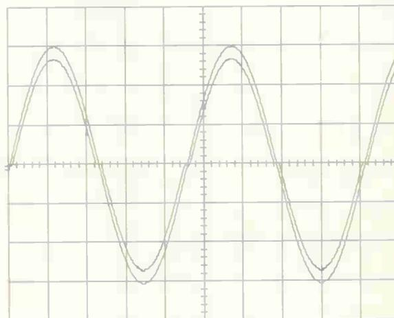
**Fig. 2. Showing the input signal of 440Hz at 12V pk-pk, larger trace, and the output signal, smaller trace, at 2V/div. vertical, 500µs/div. horizontal. The output signal is smaller than the input due to crossover switching error.**
