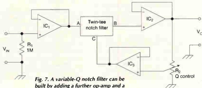
Fig. 7. A variable-Q notch filter can be built by adding a further op-amp and a potentiometer to the circuit of Fig. 6.
