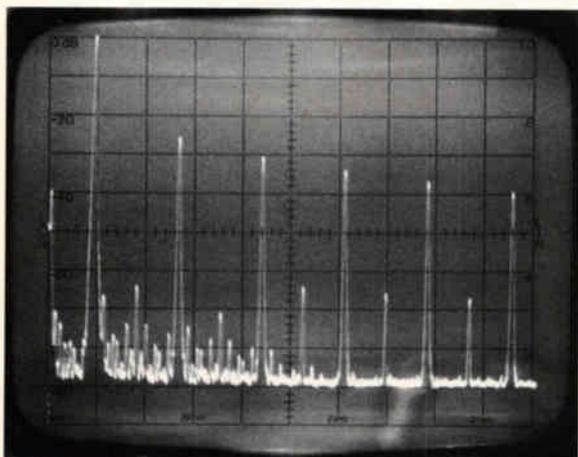
Fig. 7. The spectrum of the output signal, analyser settings as in Fig. 6, showing that crossover distortion is basically a squarewave.
