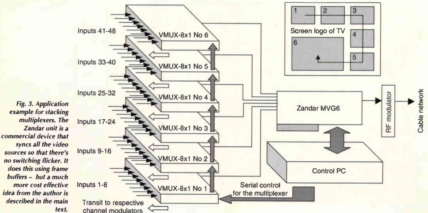
Fig. 3. Application example for stacking multiplexers. The Zandar unit is a commercial device that syncs all the video sources so that there's no switching flicker. It does this using frame buffers - but a much more cost effective idea from the author is described in the main text.
