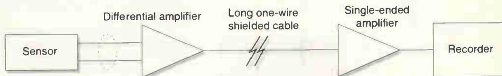
Fig. 2. My new configuration. Putting a true differential amplifier at the sensor end removed the problem of 60Hz interference.
