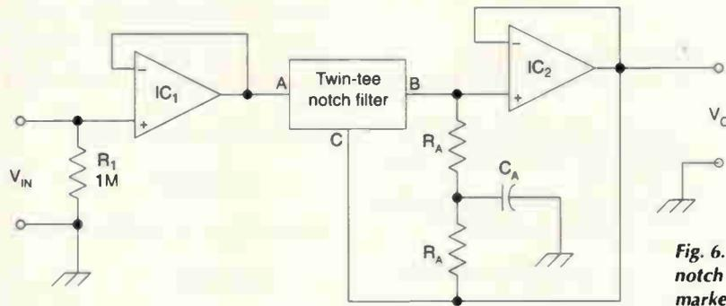
Fig. 6. Active twin-tee notch filter. The box marked Twin-tee notch filter is simply Fig. 5.
