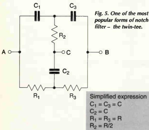
**Fig. 5. One of the most popular forms of notch filter – the twin-tee.**
