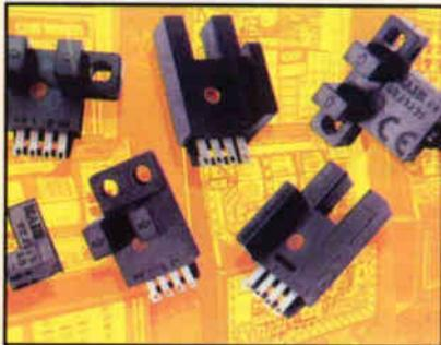
There are 17 configurations or shapes and 29 types including cabled and connector versions. All have two independent transistor outputs for light on or dark on operation and the response time is 20µs – version specific.
