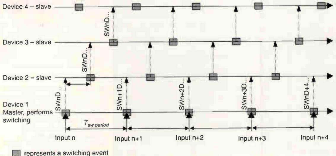
Fig. 6. When using multiple, stacked multiplexers in delayed mode, a switching command is transmitted to each slave sequentially with a delay between each transmit.
