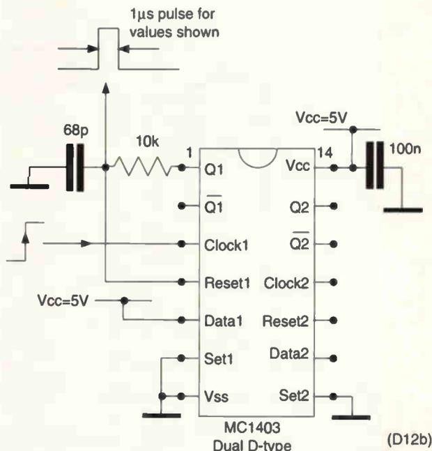
**Fig. 2. A simple adjustable rising-edge pulse generator constructed from the spare side of a D-type bistable device, saving the use of an additional chip in a tight spot.**
