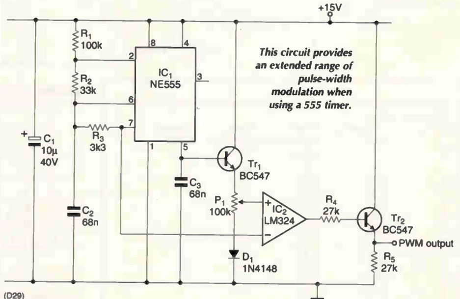
This circuit provides an extended range of pulse-width modulation when using a 555 timer.
