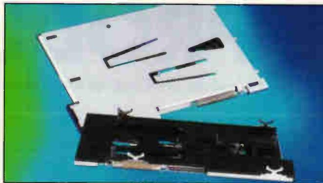
mounted into a through-hole PCB, reinforced by four metal latches on the cover. The cover prevents static discharge and provides mechanical protection. The single piece, moulded body has an integral, double-action blade switch. The normally open switch detects insertion and extraction of the smartcard and has a 2.5µm wiping action for self cleaning. Insertion and extraction forces are 7 and 5.3N respectively. It meets ISO7816 and GSM1111.
