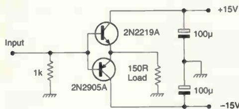
**Fig 1. Circuit of a small low power push-pull output stage with bad cross-over distortion. Cross-over distortion appears at around the midpoint in the signal excursion, where one transistor takes over from the other.**
