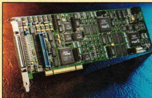
**Single-slot PCI radar input card**
