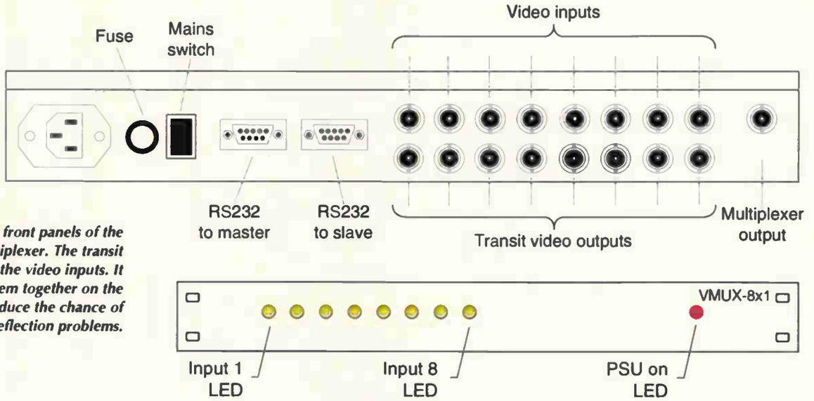
Fig. 2. Back and front panels of the author's multiplexer. The transit outputs connect to the video inputs. It is best to connect them together on the PCB though to reduce the chance of reflection problems.
