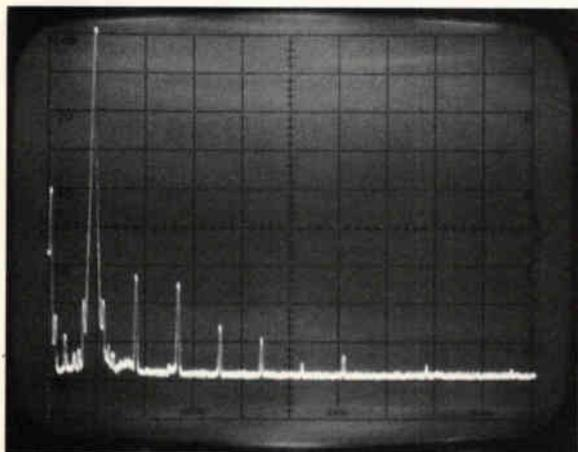
Fig. 6 The spectrum of the input signal, 440Hz. Spectrum analyser settings: span 0 - 5kHz, resolution bandwidth 10Hz, sweep speed 10s/div., display smoothing off.
