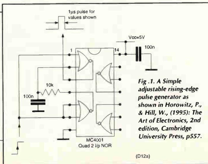
Fig. 1. A simple adjustable rising-edge pulse generator as shown in Horowitz, P., & Hill, W., (1995): *The Art of Electronics, 2nd edition*, Cambridge University Press, p557.
