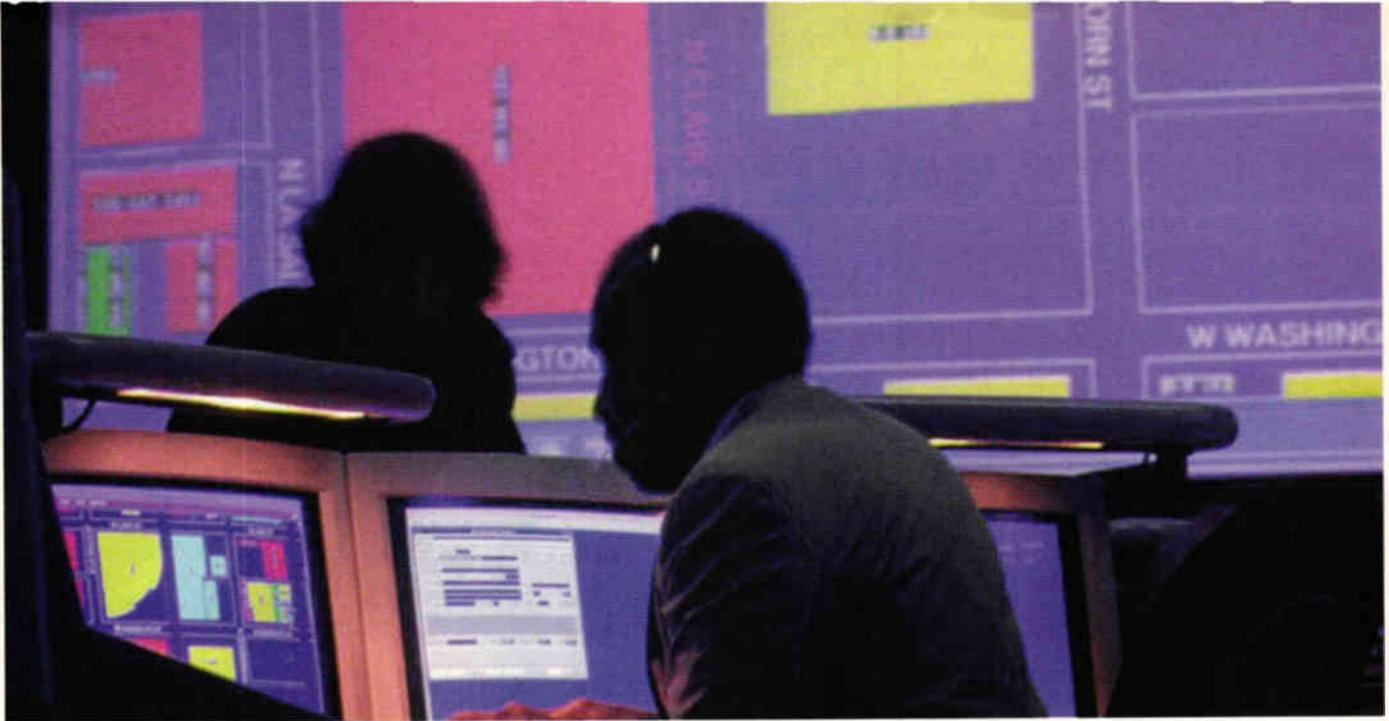
*You are here... If your car is equipped with the RAC Trackstar vehicle security service then it can be located easily in case of theft or emergency. The system was developed by Trafficmaster and combines GPS satellite tracking from Trimble Navigation with a GSM wireless communications module. Together these allow the vehicle to be located and let the driver talk with the control centre.*
