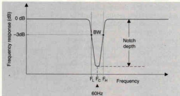
**Fig. 4. Frequency response of notch filter, whose bandwidth, BW, is the bit between the -3dB points of the notch.**
