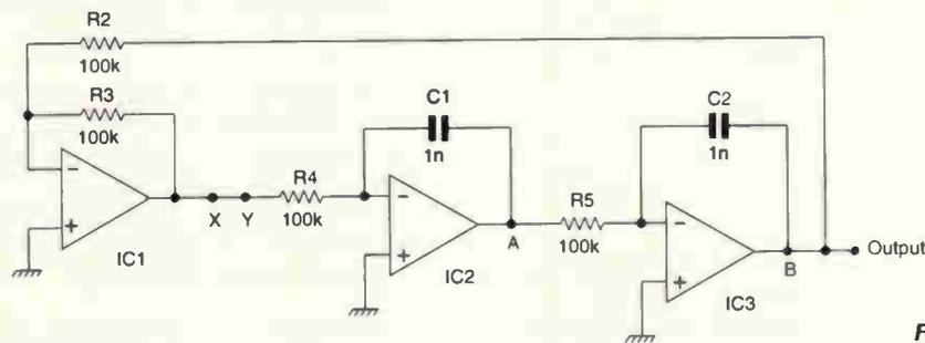
Fig. 3. In a), two integrators and an inverting amplifier are in a loop. Vector diagram 3b) shows the response of the circuit.
