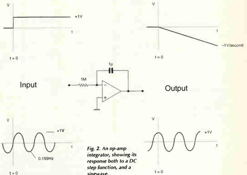
Fig. 2. An op-amp integrator, showing its response both to a DC step function, and a sinewave.
