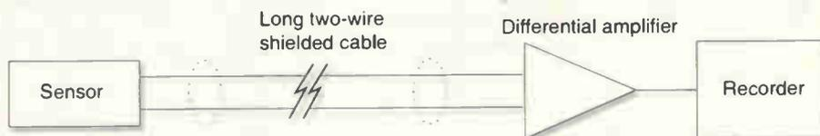
Fig. 1. Original configuration of sensor and amplifier was sensitive to hum.
