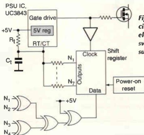
Fig 1. Block diagram of circuit for reducing electrical noise from a switching power supply.
