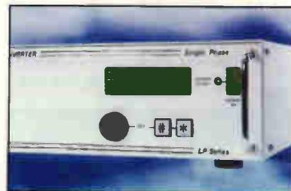
controlled by one multi-turn knob and two pushbuttons. These are operated with a two-line alphanumeric display. The chosen output is microprocessor-stored when the converter is shut down so the setting is immediately available the next time it is switched on.
