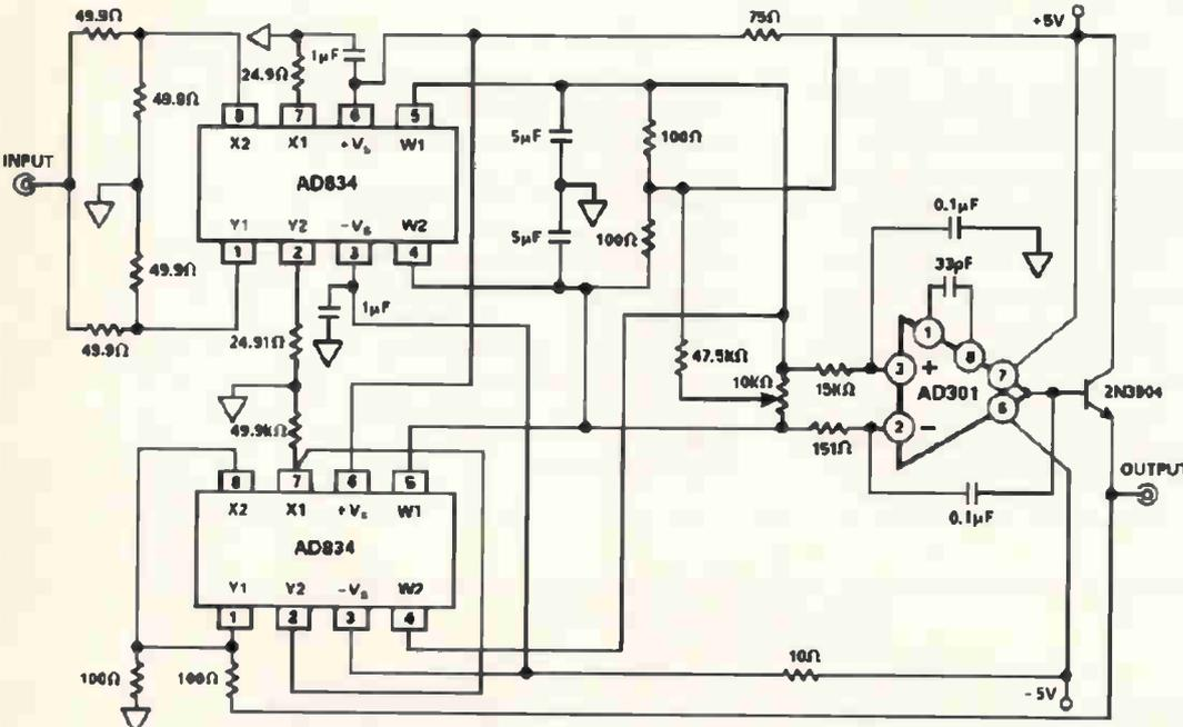
Fig. 4. Using two very fast multipliers both configured as a 'squarer', to measure the true RMS voltage of RF signals, up to +15dBm level, in a 50Ω system.
