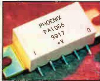
2200MHz, which will shortly be extended to 2500MHz. Input and output impedances are 50Ω. Units can be cascaded and are complete amplifiers that include DC bias, RF blocking and bypass capacitors. They have either one or two stages of amplification using medium to high power GaAs FETs. Third order intercept point is up to 20dB above the 1dB compression point.
