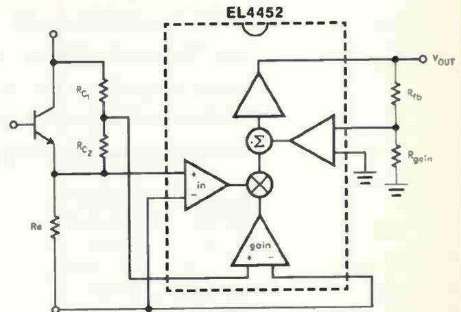
Fig. 6. With a bandwidth of 50MHz, this circuit is able to monitor the actual power dissipated in most power transistor applications, while the transistor is functioning in your design.
