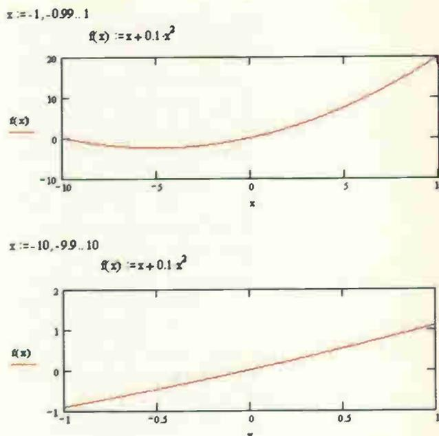
Fig. 8. Showing how second order non-linearity, the major non-linearity in a conservatively rated single ended class A amplifier, affects the transfer characteristic. Over a limited range, lower, it looks fairly linear.
