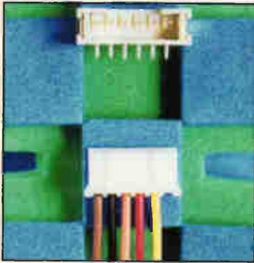
with either header type. The PH crimp style has top or side-entry connections with two to 14 circuits respectively. It is 7.5mm high and 4.5mm wide. Wire-strip holding length is 2.6mm. Crimp contacts are for 32 to 24 AWG wire, rated at 100V, 2A AC or DC for 24 AWG. Connector housings are made from heat-resistant resin compatible with reflow soldering. The solder side of the header has a retention mechanism to prevent floating during soldering.
