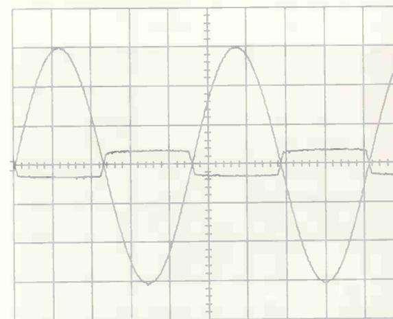
**Fig. 4. The larger trace is the input signal. The smaller is the distortion, measured by probing both the input and output signals, and displaying trace A plus trace B, with trace B inverted, i.e. a differential measurement.**
