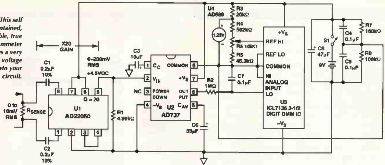
Fig. 3. Self calibrating for time and temperature induced offsets, this true RMS meter can handle up to 2V input and crest factors up to 5.
