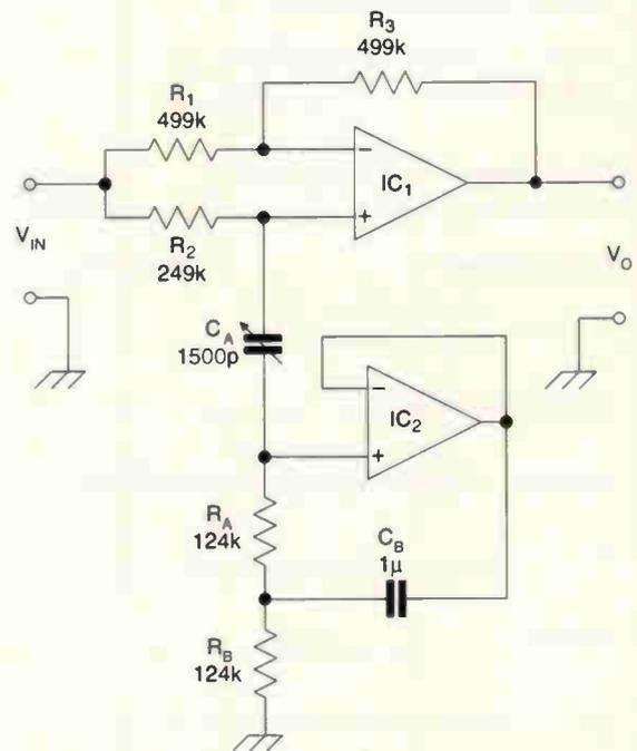
Fig. 8. Gyrator notch filter. The 1500pF variable can be made up of a fixed capacitor and a trimmer in parallel.
