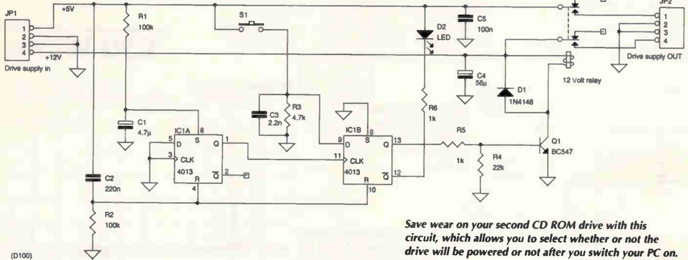
Save wear on your second CD ROM drive with this circuit, which allows you to select whether or not the drive will be powered or not after you switch your PC on.
