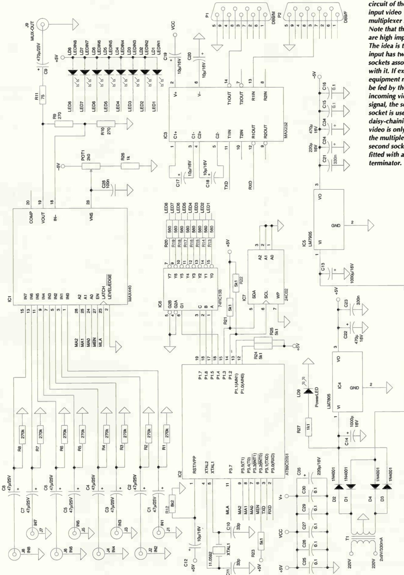
**Fig. 1. Complete circuit of the eight-input video multiplexer system. Note that the inputs are high impedance. The idea is that each input has two sockets associated with it. If extra equipment needs to be fed by the incoming video signal, the second socket is used for daisy-chaining. If the video is only feeding the multiplexer, the second socket is fitted with a 75Ω terminator.**
