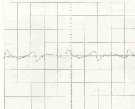
**Fig. 3. Showing the residual signal from the simple class-B output stage, after removal of the fundamental. This residual was obtained using a THD meter.**
