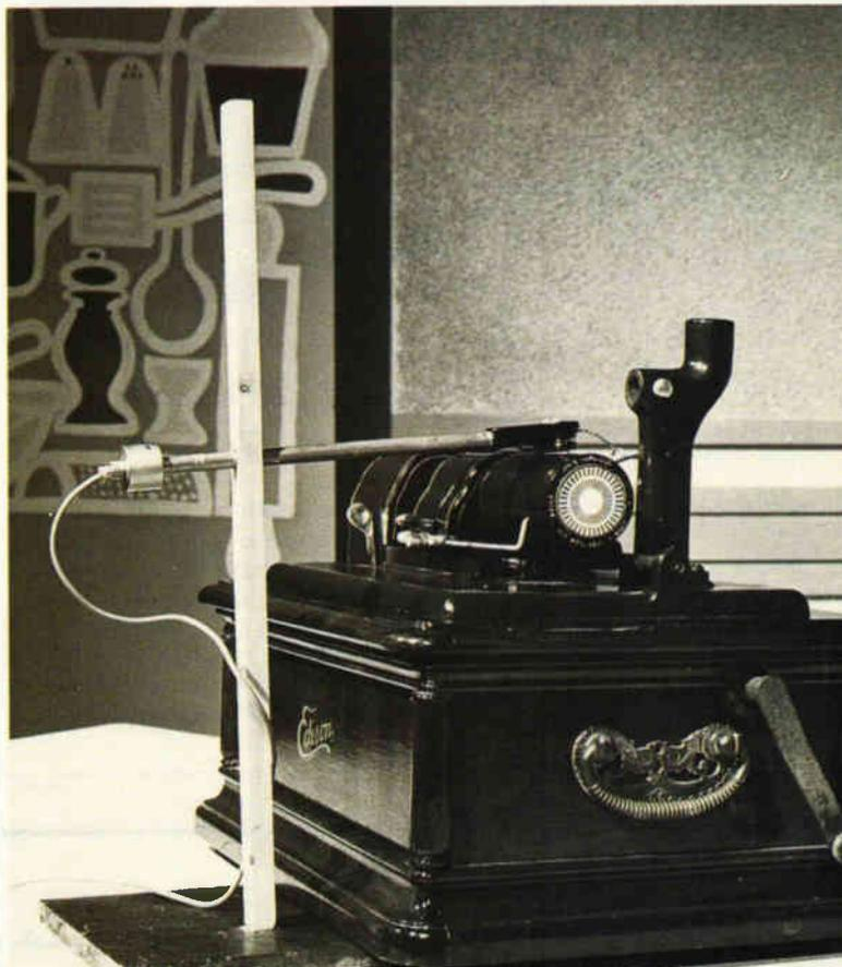
*Fig. 1. Something old, something new – a spring-driven Edison cylinder 'Concert Opera' machine, with its horn replaced by a modern light-weight arm and cartridge.*
