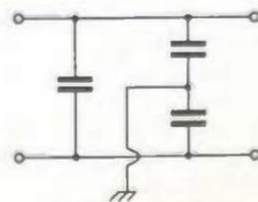
Fig. 9. Filter for both differential and common mode signals.
