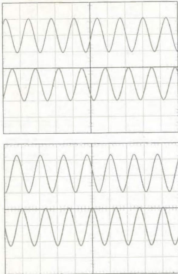
Fig. 13. Top: dual 30kHz, 1V pk-pk signals with DDS2 signal shifted 130°. Bottom: dual 150kHz signals, 0.5V pk-pk signals with DDS1 shifted by 80°.
