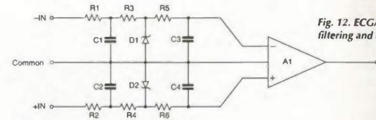
Fig. 12. ECG/EEG preamplifier filtering and defibrillator protection.
