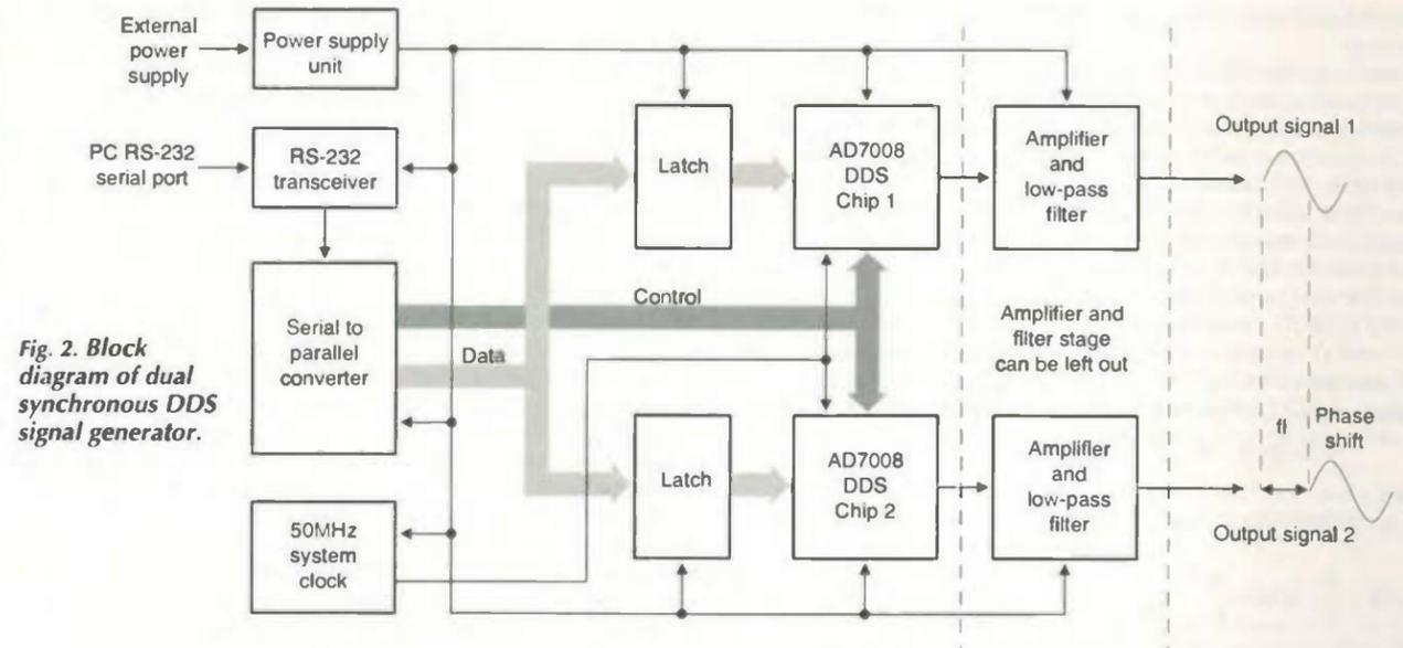
Fig. 2. Block diagram of dual synchronous DDS signal generator.
