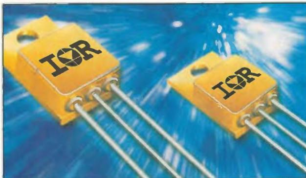
wave tube amplifiers, which are used to amplify microwave signals in satellite communications systems. The 1000V Mosfet is an enhancement-mode n-channel device, made with IR's proprietary radiation-hardened gate- and field-oxidation process to achieve single-event upset and total ionising dose
