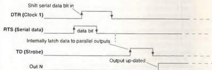
Fig. 7. Timing sequence of the serial-to-parallel converter chip.
