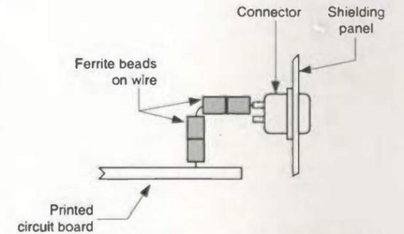
Fig. 13. Computer connector fitted with ferrite beads.
