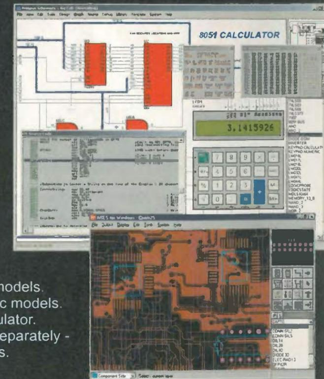
\*E.g. PROTEUS VSM can simulate an 8051 clocked at 12MHz on a 300MHz Pentium II.
