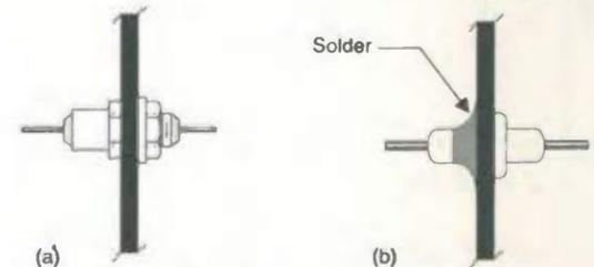
Fig. 5. Two types of feedthrough capacitor.
