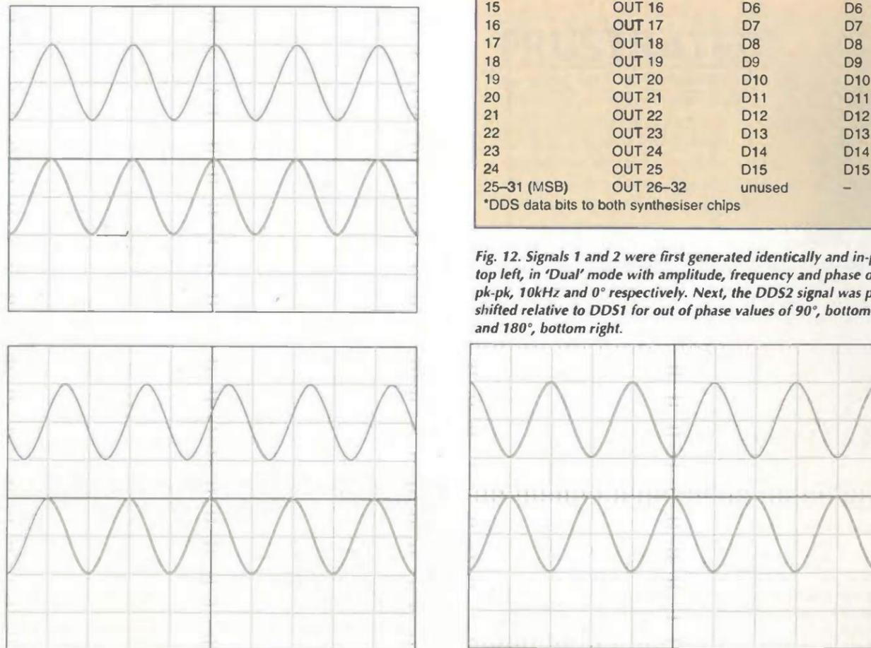
Fig. 12. Signals 1 and 2 were first generated identically and in-phase, top left, in 'Dual' mode with amplitude, frequency and phase of 1V pk-pk, 10kHz and 0° respectively. Next, the DDS2 signal was phase shifted relative to DDS1 for out of phase values of 90°, bottom left, and 180°, bottom right.
