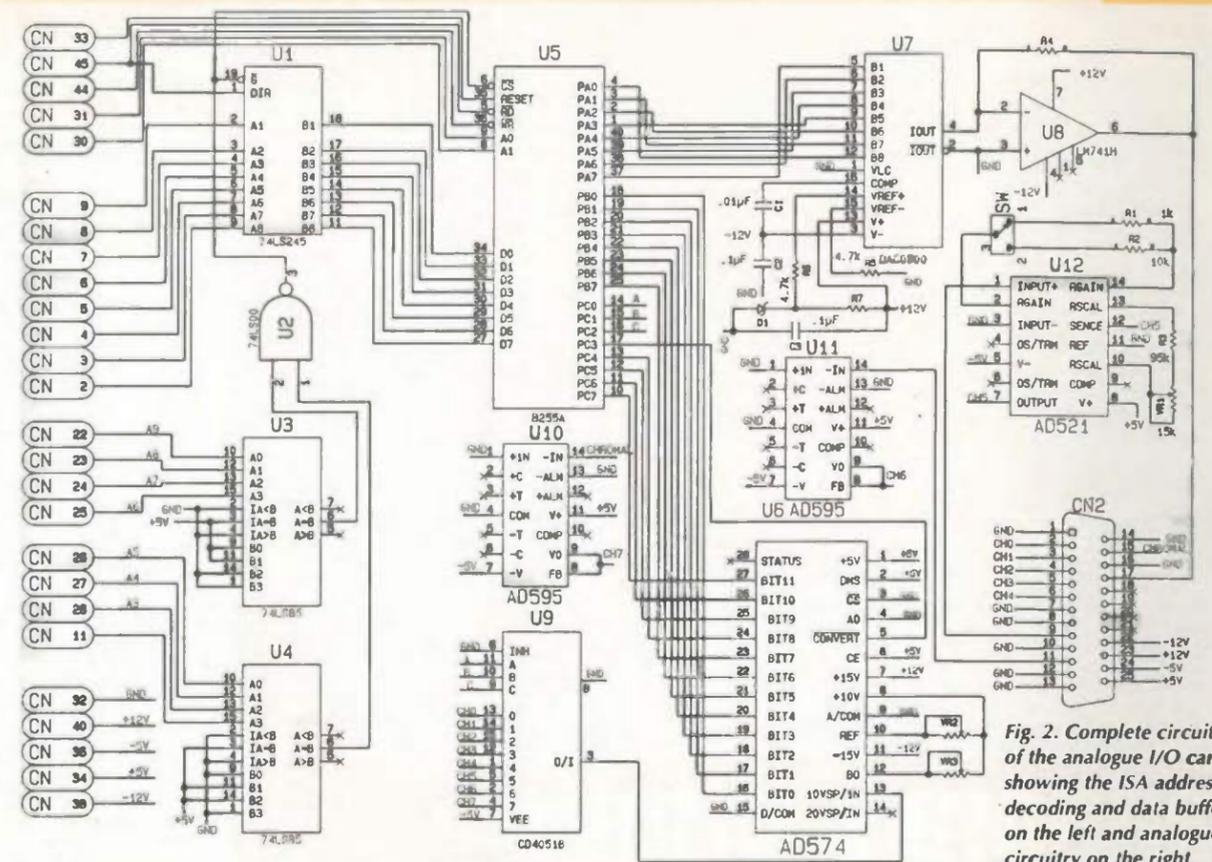
Fig. 2. Complete circuit of the analogue I/O card, showing the ISA address decoding and data buffering on the left and analogue circuitry on the right.
