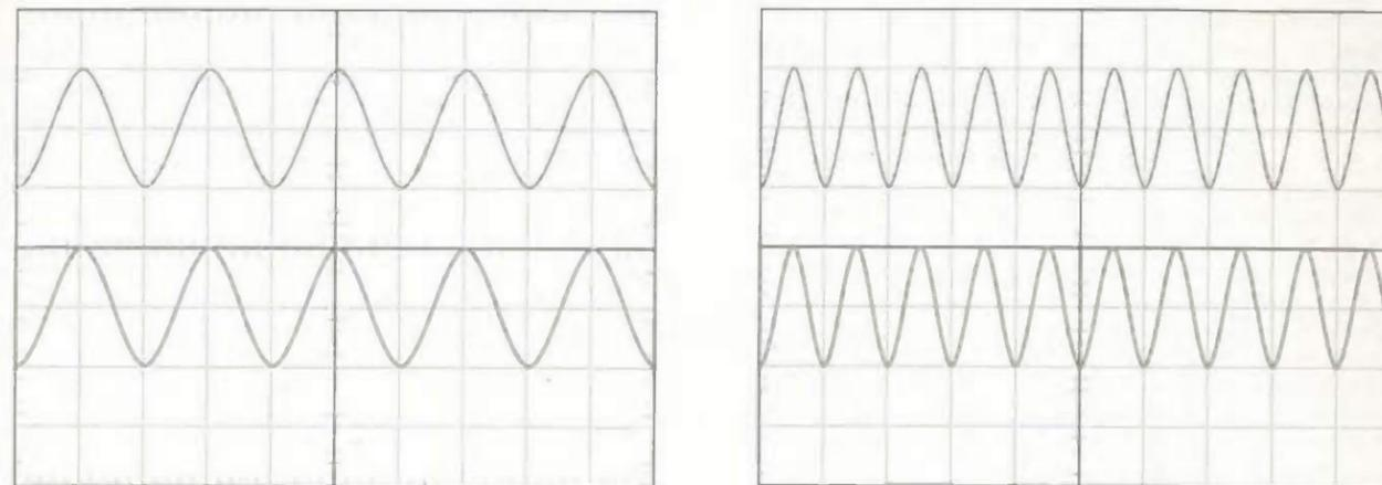
Fig. 11. Signals generated in 'Dual' mode with fixed amplitude and phase of 1V pk-pk and 0° respectively, and varying frequency of 50kHz, left, and 1MHz, right.
