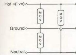
Fig. 10. Metal oxide varistors (MOV) use on AC power mains for clamping spikes.
