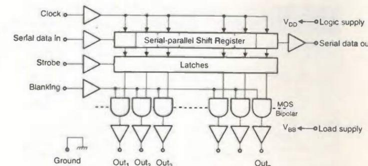
Fig. 6. Pin-out and internal block diagram of the UCN5818AF serial-to-parallel converter.
