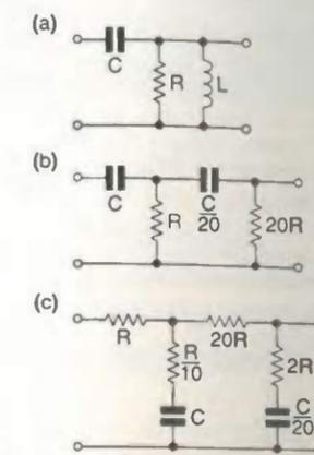
The equivalent circuit of a well-damped system, where the resonance effect can be discounted, will approximate to Fig. 1b). Resistor values are shown increasing in value to prevent the later stages appreciably loading up the earlier ones.
