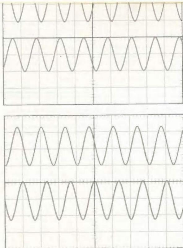
Fig. 13. Top: dual 30kHz, 1V pk-pk signals with DDS2 signal shifted 130°. Bottom: dual 150kHz signals, 0.5V pk-pk signals with DDS1 shifted by 80°.
