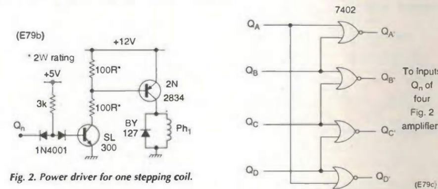
Fig. 2. Power driver for one stepping coil.
