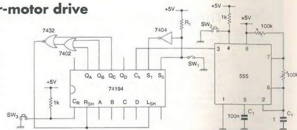
Fig. 1. Stepper motor controller using a shift register.
