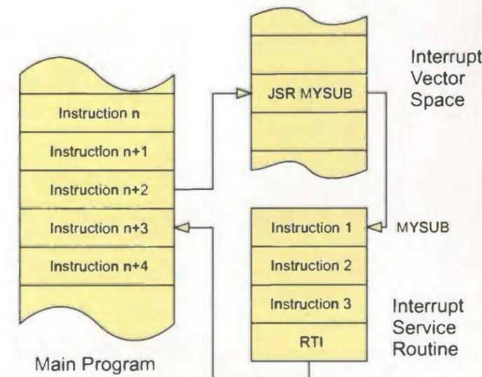
Fig. 2. Sequence of events involved in an interrupt.
