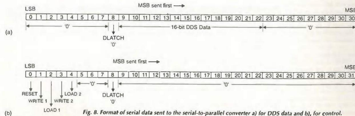
Fig. 8. Format of serial data sent to the serial-to-parallel converter a) for DDS data and b), for control.
