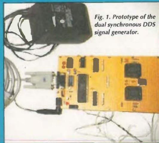
Fig. 1. Prototype of the dual synchronous DDS signal generator.
