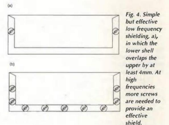
Fig. 4. Simple but effective low frequency shielding, a), in which the lower shell overlaps the upper by at least 4mm. At high frequencies more screws are needed to provide an effective shield.
