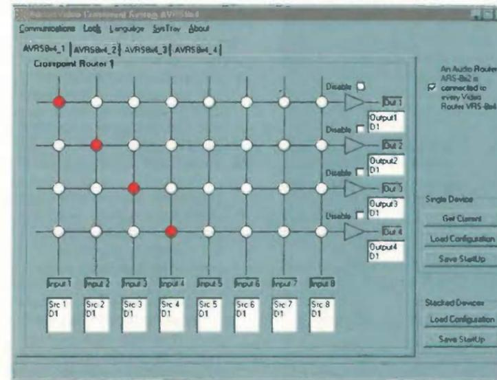
Fig. 2. Screen shot of the author's Windows software for controlling single or multiple audio and video routers.
