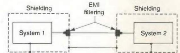
Fig. 3. Shielding and EMI filtering are suitable defenses.
