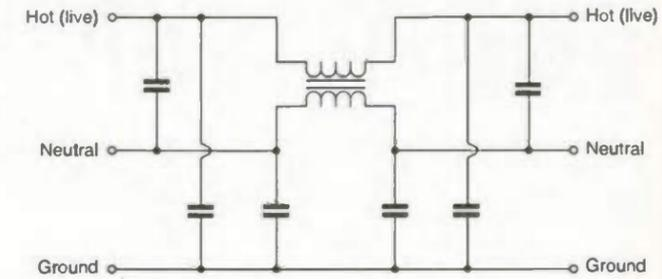
Fig. 11. AC power mains filter.
