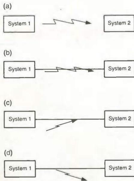
Fig. 1. There are two basic ways in which EMI is transmitted; radiation, a) and conduction, b). Conduction from radiation entering the system is represented in c), while d) shows radiation resulting from conduction.
