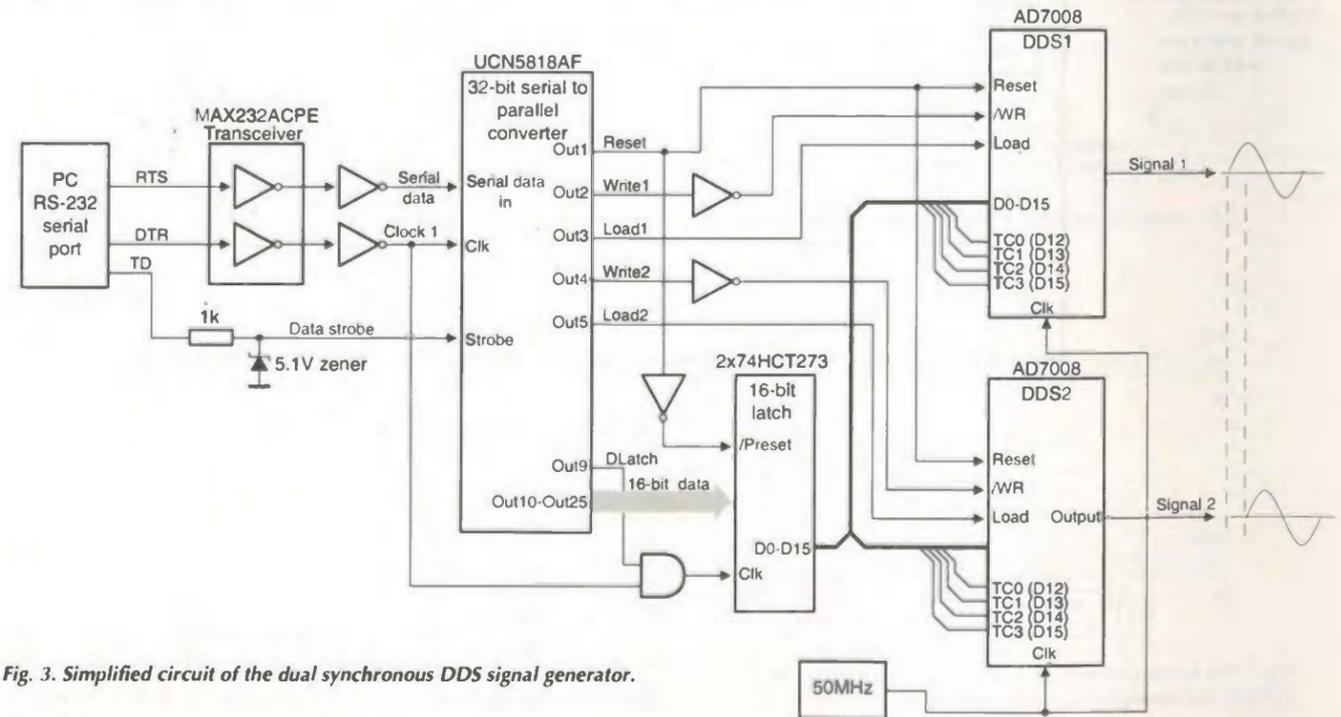
Fig. 3. Simplified circuit of the dual synchronous DDS signal generator.
