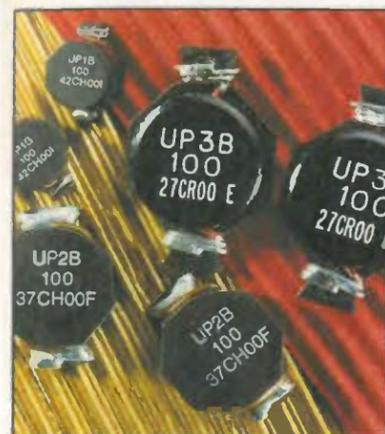
range of Uni-Pac surface mount inductors with the UP1B, UP2B, UP3B and UP4B with protective cases to reduce the risk of core breakage. They are for use within energy storage applications and DC/DC converters. Operating temperature is -40 to +85°C ambient with an rms current rating of 19.2 to 0.47A. Standard inductance is set at 0.47 to 100µH; modified values for higher applications are available on request.
