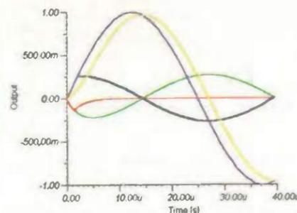
Fig. 1. 20kHz simulation highlighting RC phase lag.
