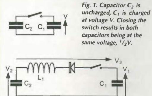
**Fig. 1.** Capacitor  $C_2$  is uncharged,  $C_1$  is charged at voltage  $V$ . Closing the switch results in both capacitors being at the same voltage,  $1/2V$ .
