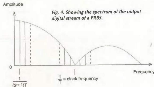
Fig. 4. Showing the spectrum of the output digital stream of a PRBS.
