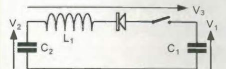
**Fig. 2.** In this circuit, with idealised components, the entire charge and energy are transferred from the charged capacitor when the switch is closed.
