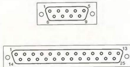
Fig. 5. Pin layout and functions of the RS232 connectors on PCs, a) 9-pin male socket. b) 25-pin male socket.
