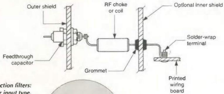
Fig. 6. Simple L-section filters: a) internal capacitor input type. b) external inductor input type.
