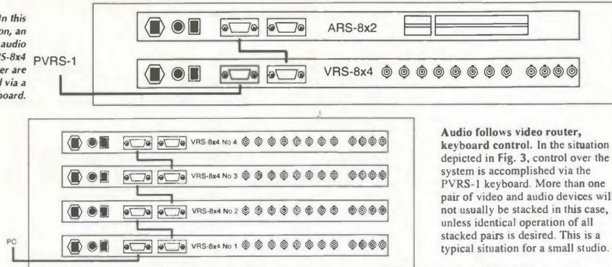
Fig. 4. It is possible to stack just video routers or audio routers and control them via a PC.
