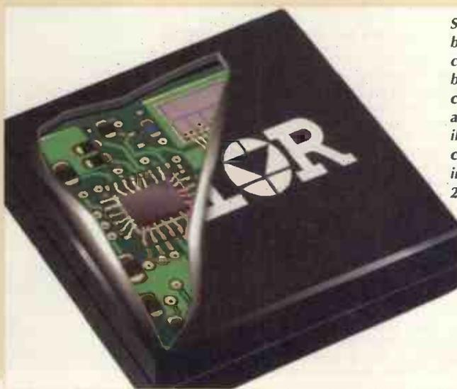
*Sitting between brick-type DC-to-DC converters and on-board discrete-component alternatives, the iP1001 only needs capacitors and an inductor to deliver 20A output.*
