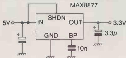
Fig. 1. Power for the preamplifier is derived from the +5V line of a computer's USB interface. This circuit converts the noisy 5V output to a regulated +3.3V for driving the preamplifier.
