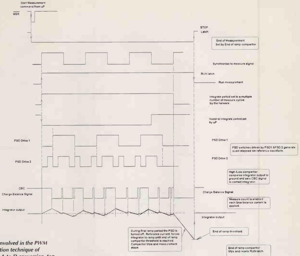
Fig. 3. Waveforms involved in the PWM control-loop regulation technique of quantised feedback A-to-D conversion, top, and basic elements of the converter, below.
