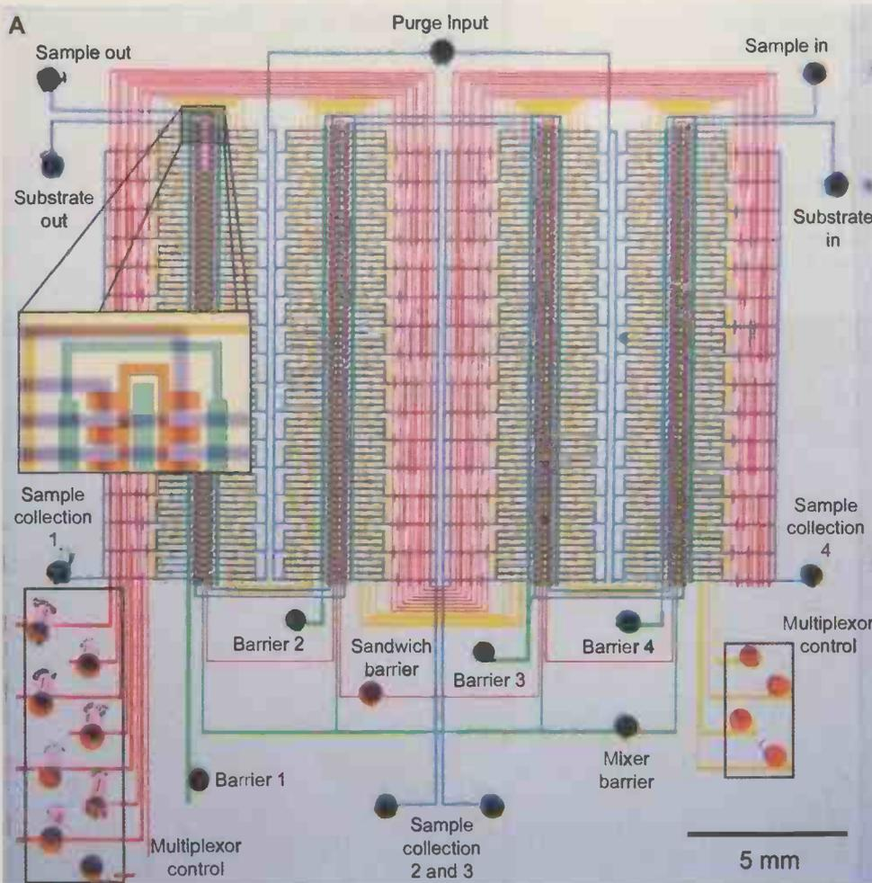
*Coloured food dyes show the multiple channels in this comparator chip. The device contains 2,056 valves and 256 reaction chambers.*
