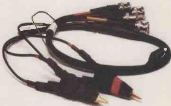
Fig. 8. Photo a) shows a Wayne Kerr four-terminal fixture, b) shows tweezers for measuring chip components using a two terminal connection method and c) shows Kelvin clips, again from Wayne Kerr.
