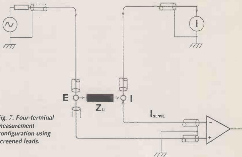
Fig. 7. Four-terminal measurement configuration using screened leads.
