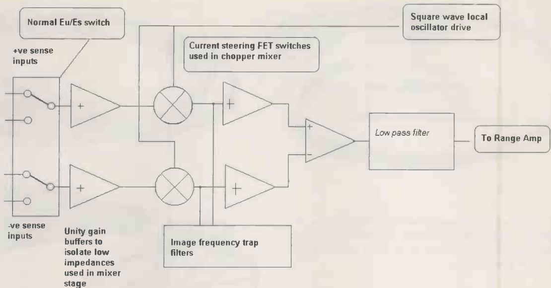
with good resolution and range by simply changing to a DC stimulus and chopping the  $E_u$  and  $E_s$  signals prior to passing to the ac coupled ranging and detector circuits,
