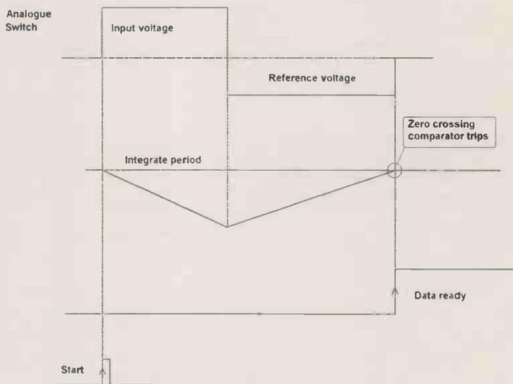
waveforms are designed to have equal and opposite number of switching transitions to cancel switching charge injection at the integrator input, Fig. 4.
