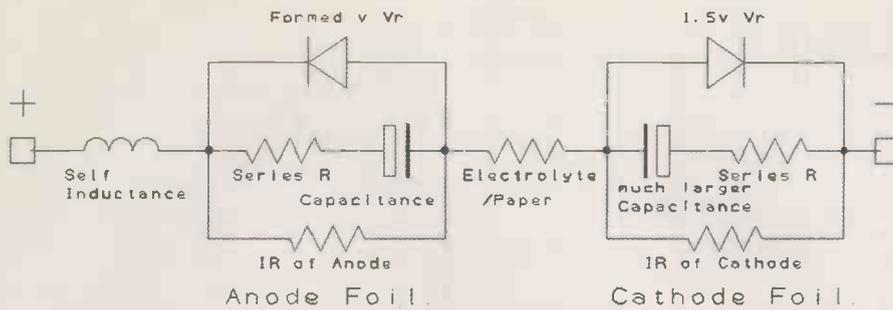
Figure 4: Simplified equivalent schematic shows how a polar electrolytic capacitor behaves with AC signals, with and without DC bias.
