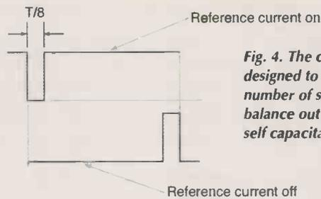
Fig. 4. The charge-balance waveforms are designed to have an equal and opposite number of switch transitions in order to balance out charge injection from switch self capacitance.
