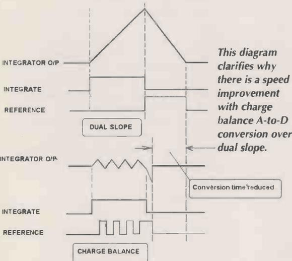
Overall, the charge balancing A-to-D converter gives excellent performance. With very long integration periods, the circuit is limited by low-frequency  $1/f$  noise from the band-gap reference and integrator amplifier. The impedance range of the instrument is therefore reduced to maintain a practicable number of precision range settings.
