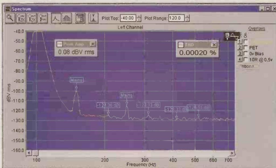
Figure 6: Distortion plot of an assembly of ten Evox Rifa 10 $\mu$ F 63 volt MMK metallised PET capacitors, tested at 0.5 volt. This 100 $\mu$ F assembly was used as the distortion reference for each test.
