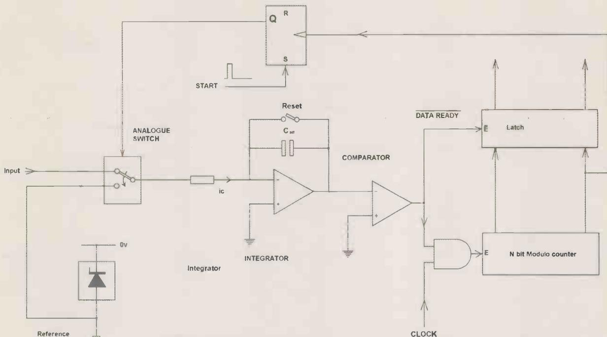
**Fig. 1 Basic dual-slope A-to-D converter and associated waveforms.**
