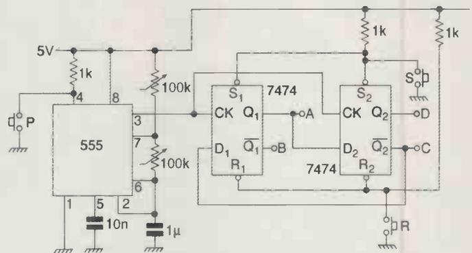
Fig. 1. This two-phase sequencer is clocked by an astable multivibrator.
