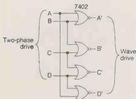
Fig. 3. Drive circuit for one of the four stepper motor windings. The other three are identical.
