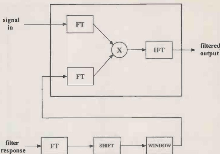
Figure 2: FIR filter implemented by inverse FFT of product of FFTs of impulse response and input signal. Operations within the box constitute convolution. The shift operation re-orders the wrapped data.
