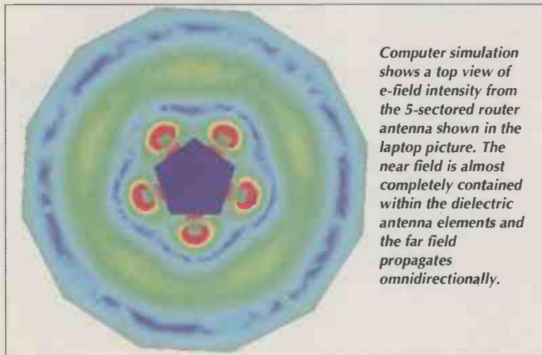
Computer simulation shows a top view of e-field intensity from the 5-sectored router antenna shown in the laptop picture. The near field is almost completely contained within the dielectric antenna elements and the far field propagates omnidirectionally.
