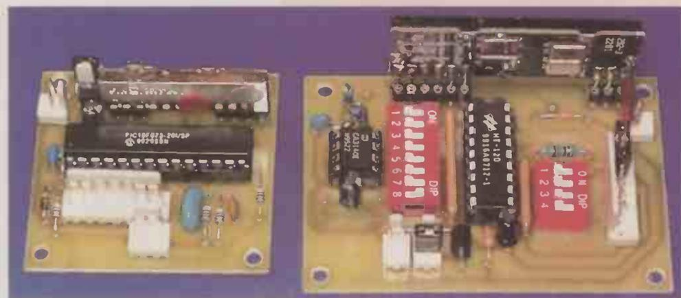
that are suitable for extended range data link at a data rate up to 10kb/s<sup>1</sup>. A range of 10km can be achieved in open ground with a suitable data rate and antennae. They are type-approved to the EN300 220-1 for use at 173.250MHz in the UK and fully screened with extensive internal filtering to ensure EMC compliance to ETS 300 683. Other frequencies are available from the manufacture<sup>1</sup>.
