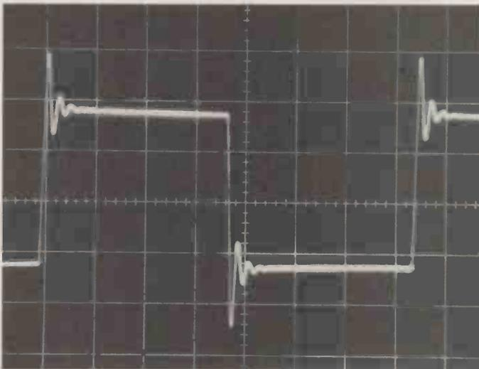
Photo 3 Square wave response (2kHz) at  $CL=1\mu F$
