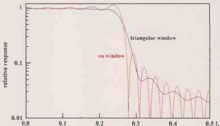
Figure 6. Effect of window function.
