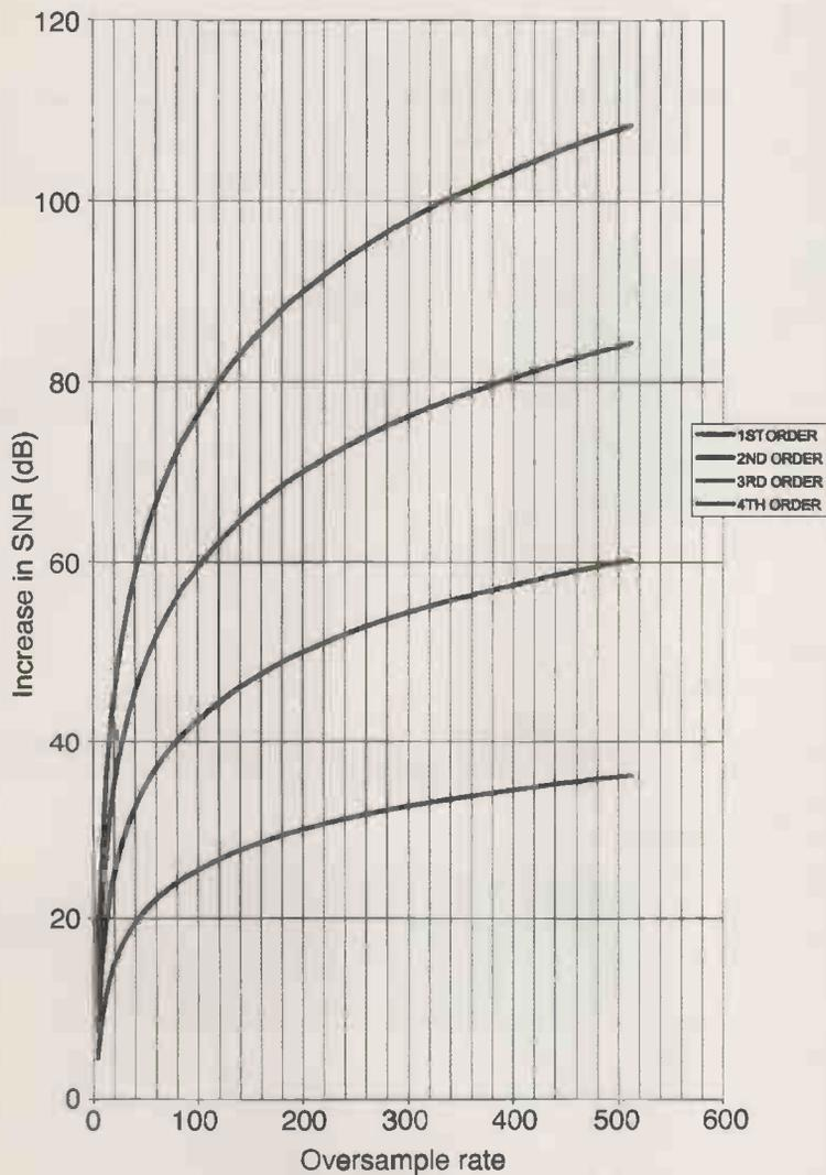
Fig. 12. Plot of signal-to-noise ratio improvement versus sample rate and modulator order.
