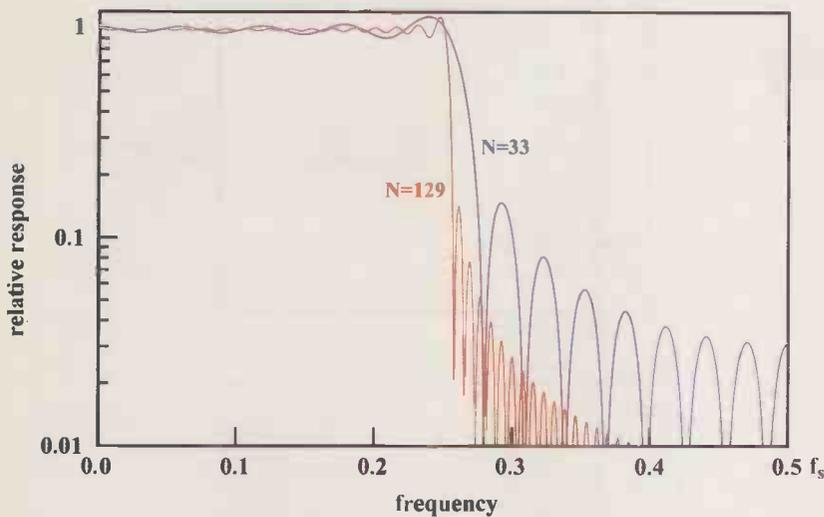
Figure 4. Frequency responses of lowpass filters of lengths 33 and 129.
