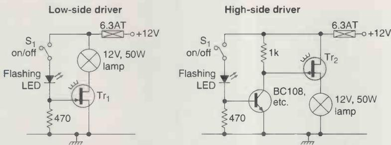
Power flasher with low-side or high-side driver options. Fet  $Tr_1$  is a 30V, 20A n-channel type while  $Tr_2$  is a 30V, 20A p-channel device.
