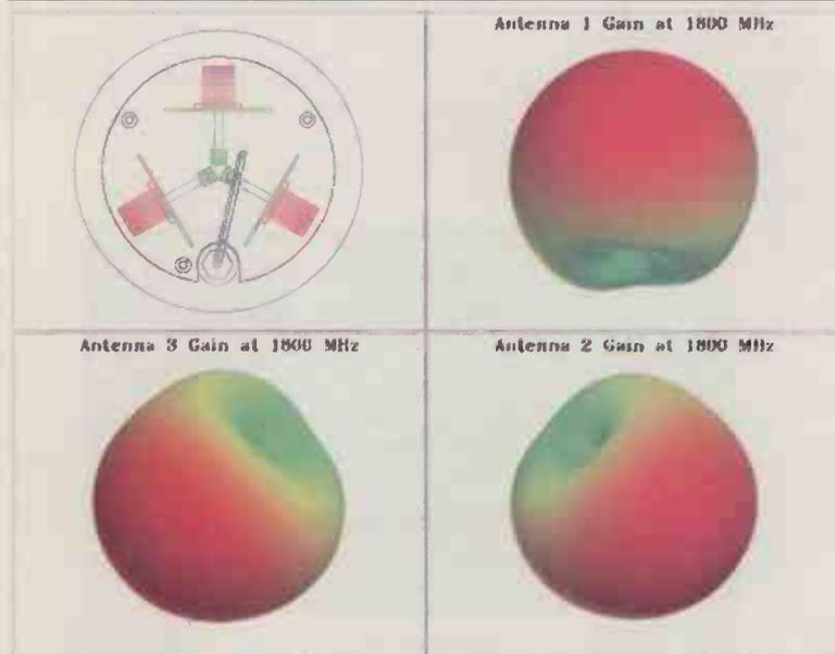
Gain plots for a tri-sectored antenna, showing the 3D gain pattern - with pattern length and deeper colour indicating higher intensity
