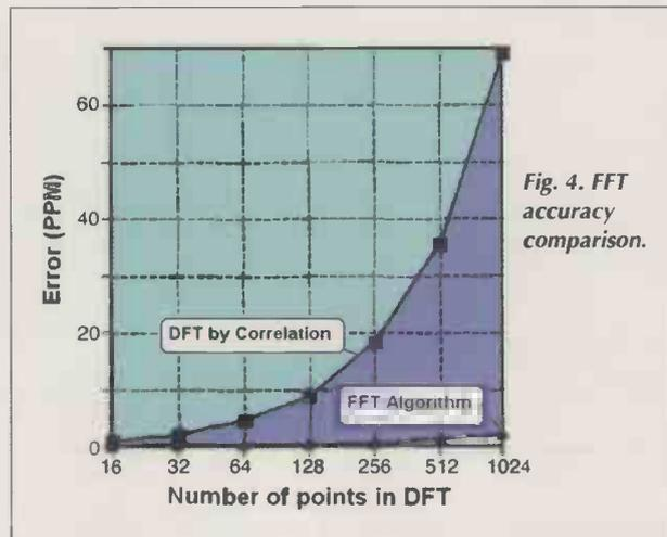
Fig. 4. FFT accuracy comparison.
