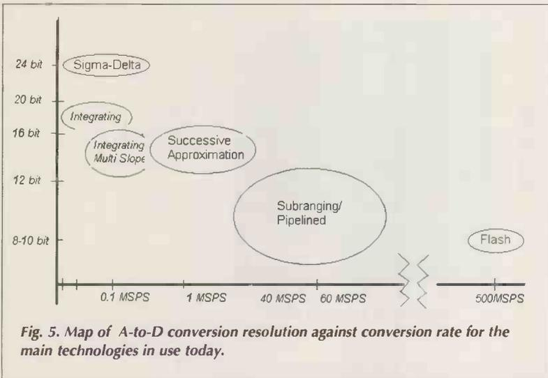
Published dynamic performance for these ICs are at these higher sample rates. By operating then at only 20.48kHz, it may still be possible to achieve near 24-bit effective resolution. The availability of such chips shows what could be possible with a custom-designed A-to-D converter using separate ICs for the analogue and digital functions and more sophisticated digital filtering for best noise performance.
