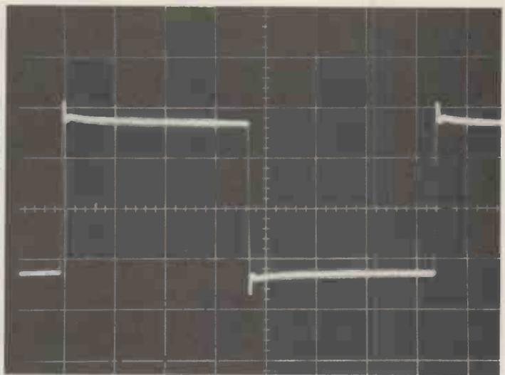
Photo 2 Square-wave response (2kHz) at  $RL=8\Omega$
