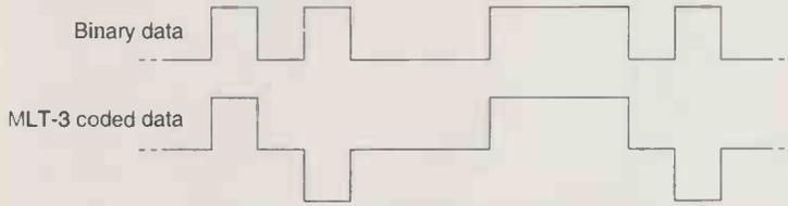
Fig. 3. A standard binary serial stream, top waveform, and an MLT-3 stream, bottom.
