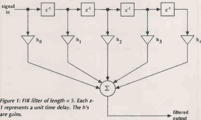
Figure 1: FIR filter of length = 5. Each  $z^{-1}$  represents a unit time delay. The  $h$ 's are gains.
