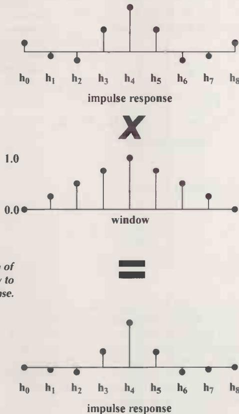
Figure 5. Application of triangular window to impulse response.
