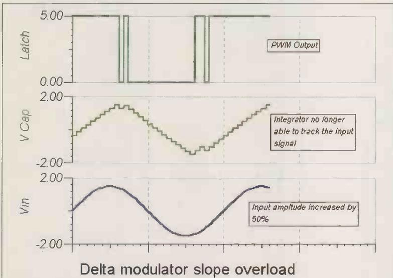
Fig. 11. Waveform of delta modulator overload.
