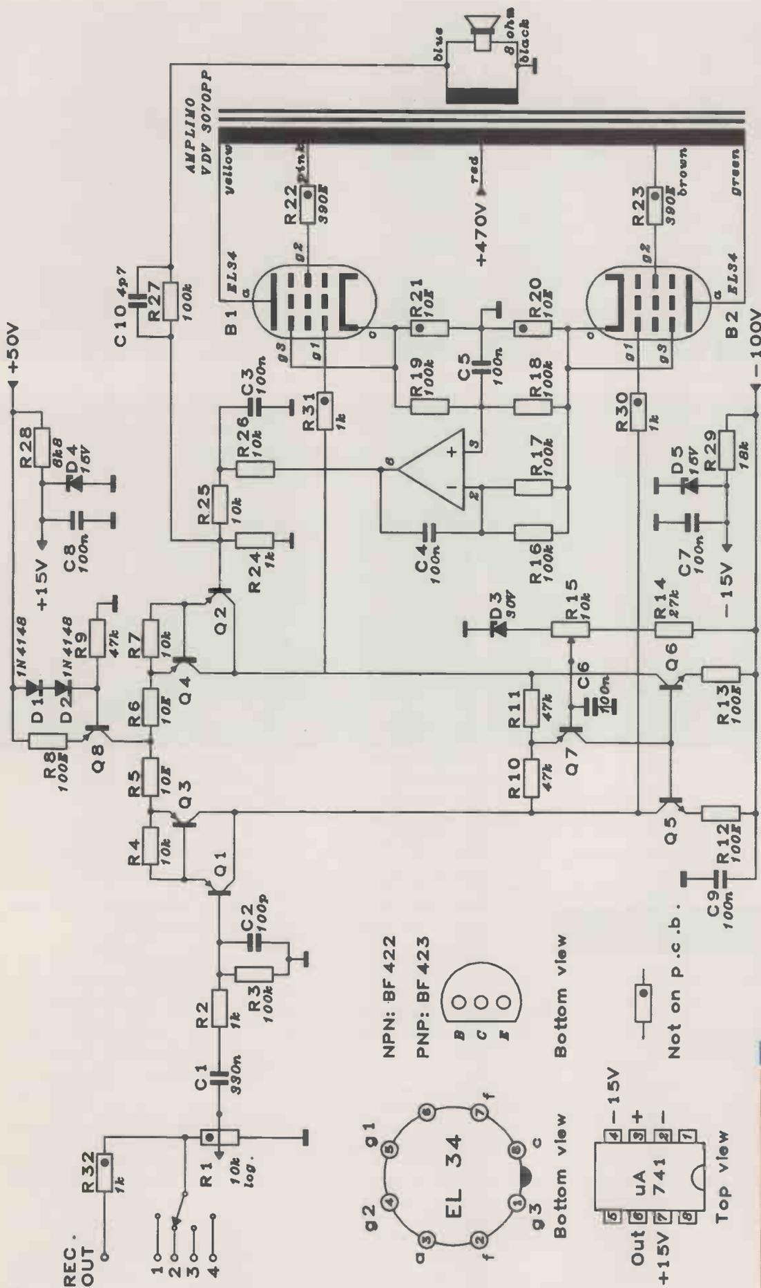
Fig.1 The improved hybrid 40W power amplifier uses transistors for phase splitting, an IC integrator for dc feedback and valves for power driving and features a 30Hz-100kHz Full Power Bandwidth.
