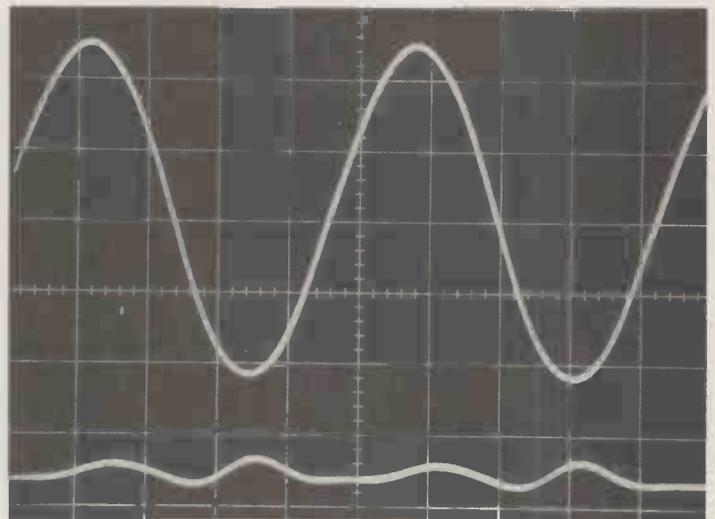
Photo 4 Waveform resulting from driving the amplifier at 40W,  $8\Omega$  with a 100kHz sine-wave illustrates the absence of switching distortion.
