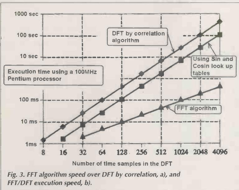
Fig. 3. FFT algorithm speed over DFT by correlation, a), and FFT/DFT execution speed, b).
