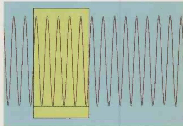
Fig. 14. By sampling from zero crossings and whole multiple periods of the measured signal, perfect windowing is obtained by the FFT. This avoids spectral leakage or blurring of the FFT output spectrum.
