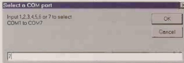
The screen for users to input the number of the COM port to be used with this device. Input 1,2,3 or 4 to select COM1, COM2, COM3 or COM4.
