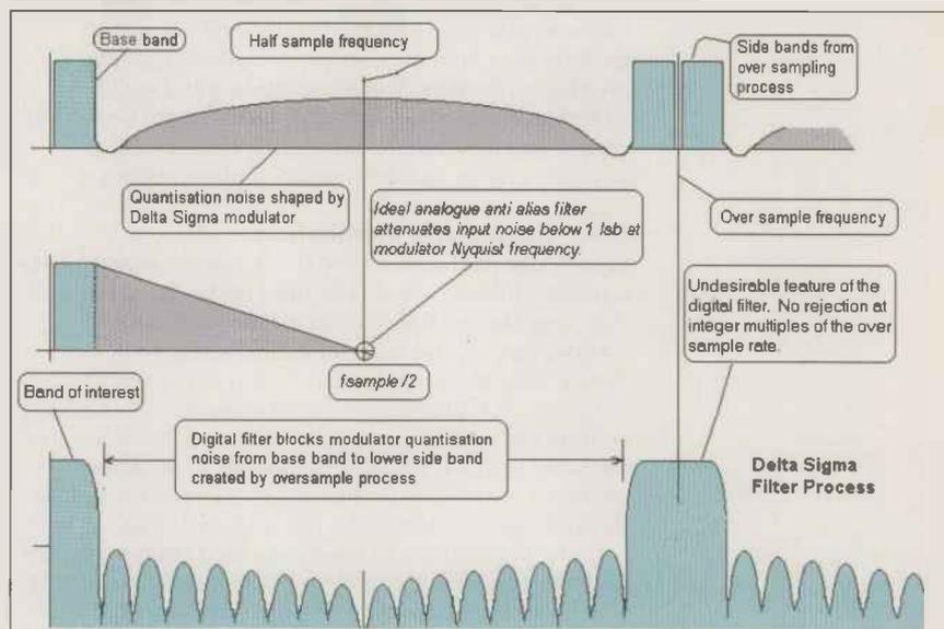
Fig. 8. Digital filtering in frequency plane, a), and sigma-delta mod output noise, b).
