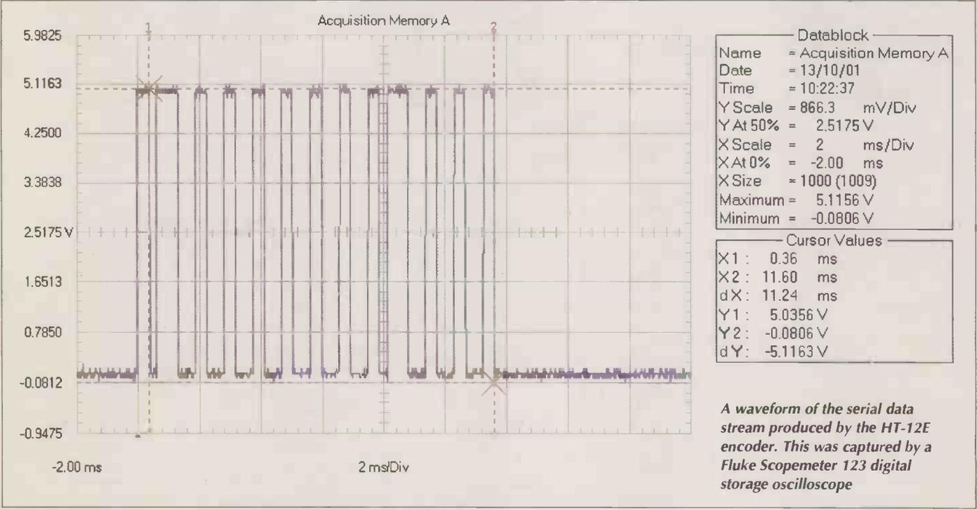
A waveform of the serial data stream produced by the HT-12E encoder. This was captured by a Fluke Scopemeter 123 digital storage oscilloscope
