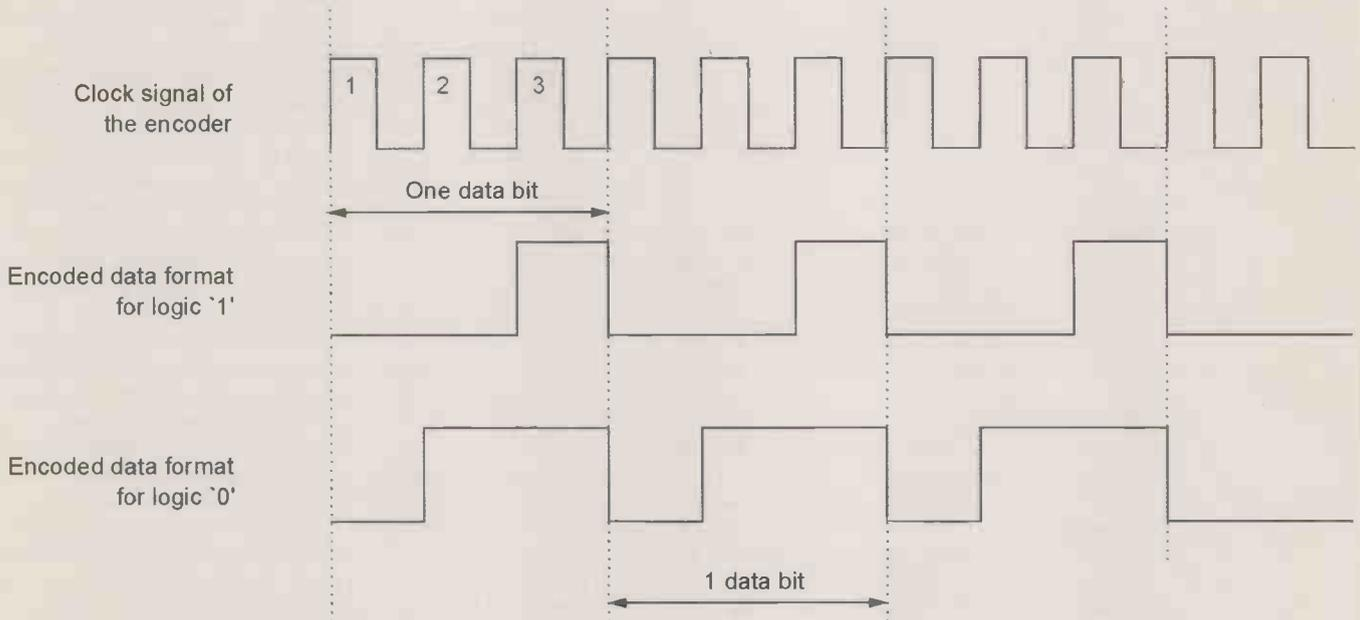
This figure shows how bit '0' and '1' are encoded by the HT-12E encoder
