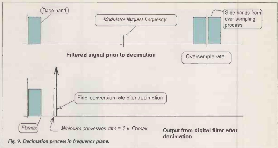
Fig. 9. Decimation process in frequency plane.
