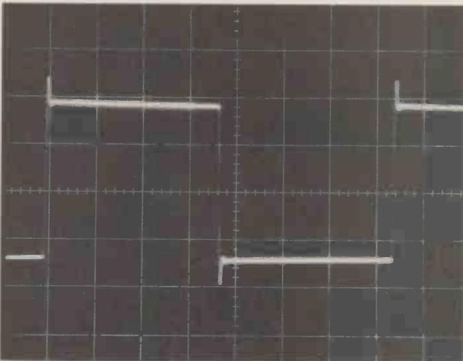
Photo 1 Square-wave response (2kHz) with open output
