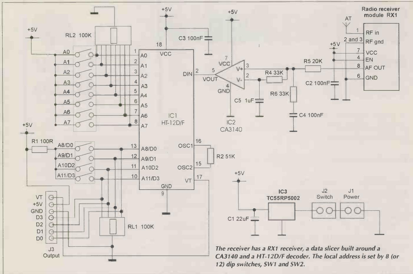
The receiver has a RX1 receiver, a data slicer built around a CA3140 and a HT-12D/F decoder. The local address is set by 8 (or 12) dip switches, SW1 and SW2.
