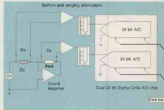
Fig. 13. Elements of a simplified LCR bridge based on DSP.
