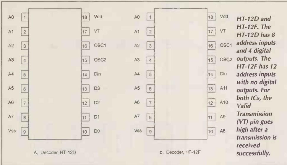
**HT-12D and HT-12F. The HT-12D has 8 address inputs and 4 digital outputs. The HT-12F has 12 address inputs with no digital outputs. For both ICs, the Valid Transmission (VT) pin goes high after a transmission is received successfully.**
