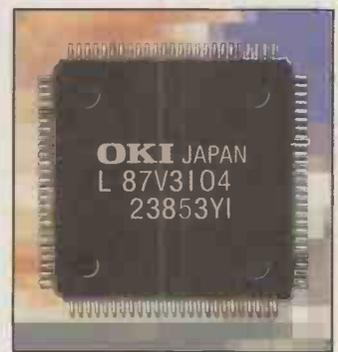
16/256 colours out of 4,096 colours (pseudo colours) and 4,096/6,5536 (direct colours). Output data complies with STN 4/8-bits parallel or TFT 12-bits (R4, G4, B4) or 16-bits (R5, G6, B5). An extended temperature version is available (-45 to 85°C).
