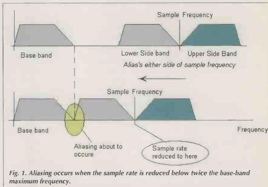
Fig. 1. Aliasing occurs when the sample rate is reduced below twice the base-band maximum frequency.
