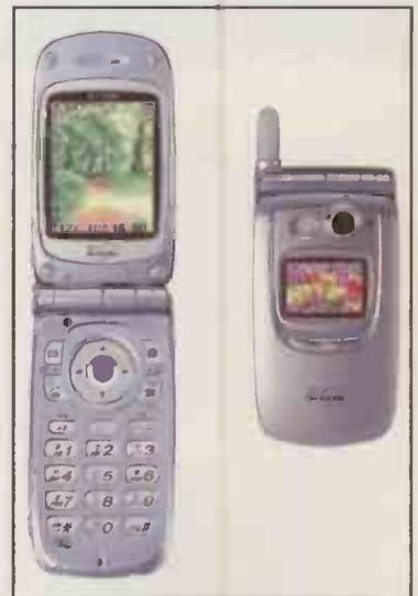
DoCoMo has released a phone using a 5.6cm 65,536-colour switchable 2D-3D display from Sharp. Part of the i-shot range, the SH251i allows users to receive or take 2D photos and translate them into 3D images for display. The on-board camera is a CCD with 310,000 pixels.
