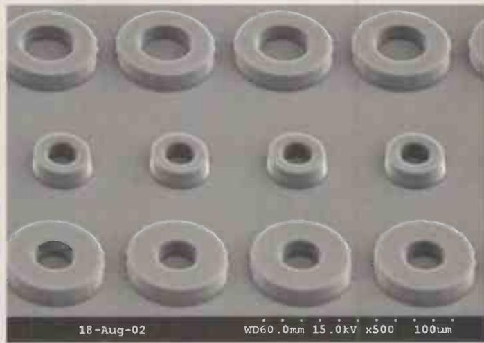
Micrograph of a set of polymer cups.
