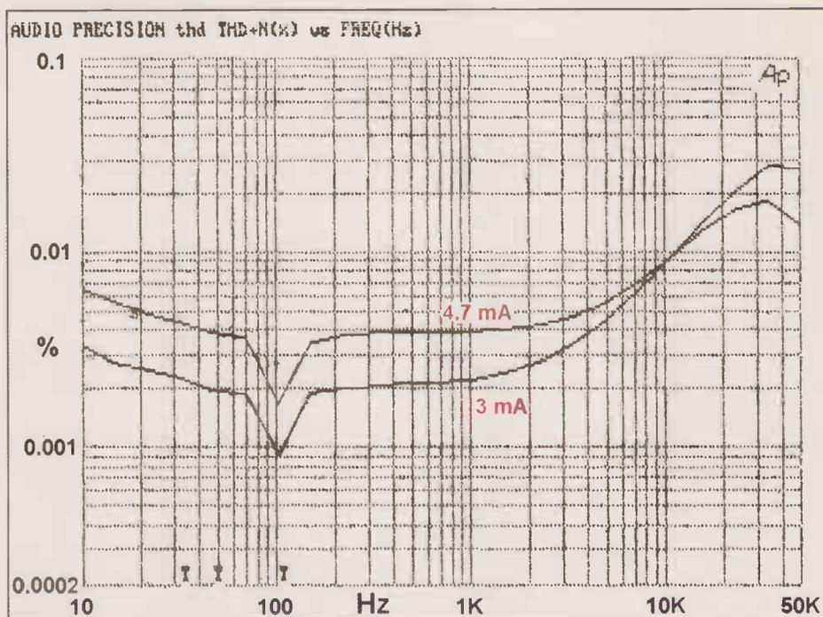
Fig. 4. Reducing the tail current improves things at low frequencies but increases HF distortion above 10kHz. The notches at 100Hz indicate that the ripple content is still substantial.
