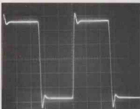
Fig. 7. Square-wave response  $f=100\text{kHz}$ , vert.  $1\text{V/div.}$ ,  $C_{(\text{load})}=2.2\text{nF}$ .
