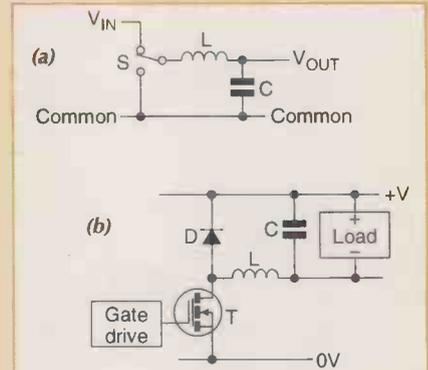
**Fig. 7. The converter is simply a changeover switch and LC smoothing circuit.**
