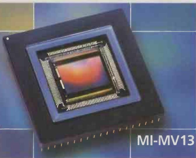
CMOS image sensors can now equal the quality of charge coupled device (CCD) sensors, according to Micron Technology. Better known for its DRAM, Micron has been working on CMOS imagers for some time.
