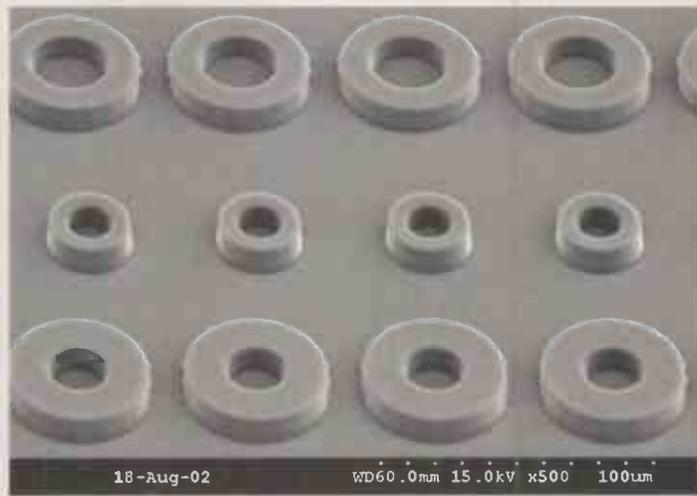
Micrograph of a set of polymer cups.
