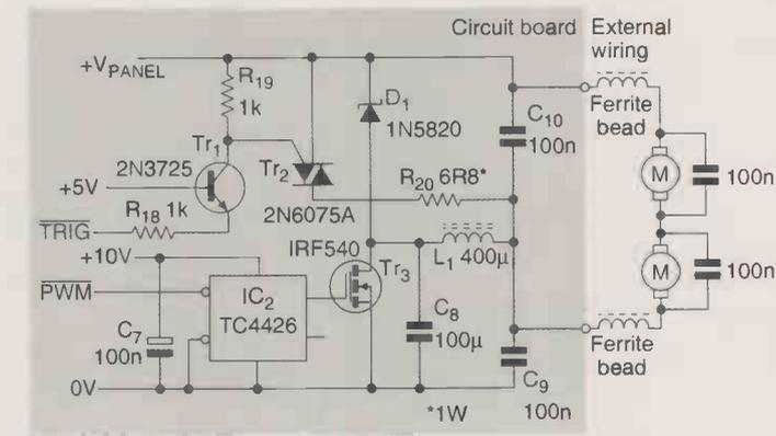
Fig. 6. The motor drive circuits, including the buck converter and triac brake.
