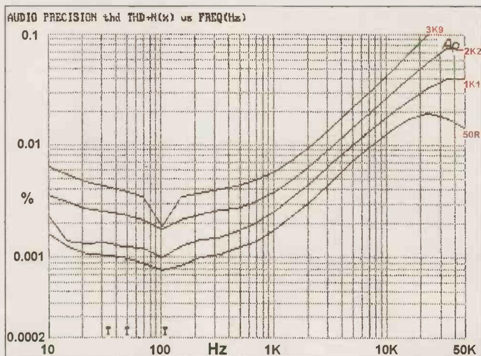
Fig. 1. Second-harmonic distortion and 100Hz ripple get worse as the source impedance rises from 50 Ohms to 3.9K. 50 Watts into 8 Ohms.
