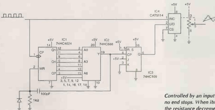
*Controlled by an input pulse train, this digital potentiometer has no end stops. When its resistance reaches minimum or maximum, the resistance decrement or increment changes direction.*
