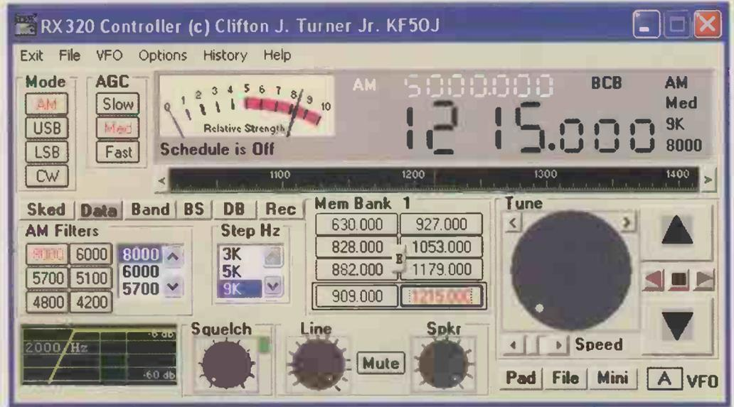
Fig. 6. Example of RX-320 control software (written by Clifton Turner).
