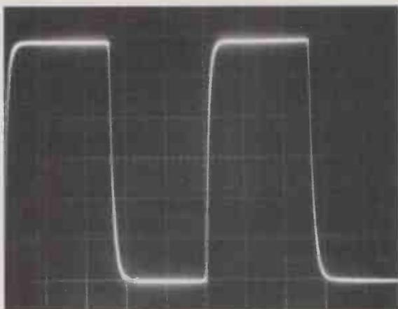
Fig. 6. Square-wave response  $f=100\text{kHz}$ , vert.  $1\text{V/div.}$ ,  $R_{(\text{load})}=600\Omega$ .
