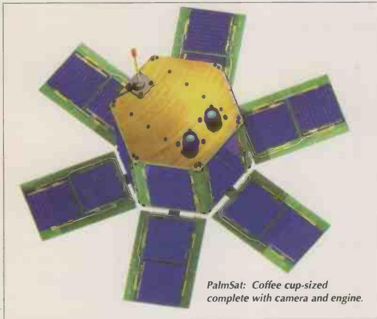
*PalmSat: Coffee cup-sized complete with camera and engine.*
