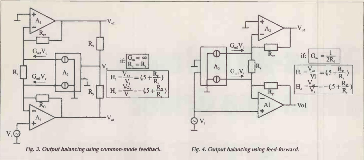
Firstly, the input of A3 is connected to the input of the line driver, so there are no feedback restrictions. Secondly, there is an optimal value of the transconductance.
