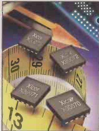
backplane. The controllers integrate several new hotswap functions to meet the demands of 30V to 110V live power backplanes. A selectable gate current feature provides for design flexibility to account for variations of load, current and transients. Hardshort detection with retry, overcurrent safety limit during insertion, and built-in contact bounce and high frequency noise filter allow for additional protection during live insertion and system start-up.
