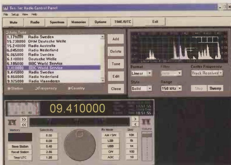
Fig. 3. Ten-Tec RX-320 control program screen.
