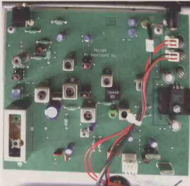
Fig. 10. RF board - rear panel at top of picture.
