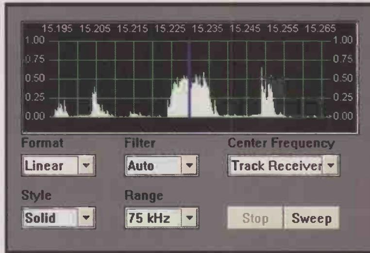
Fig. 14. 19 metre spectrum scan centred on a DRM Deutsche Welle test broadcast.
