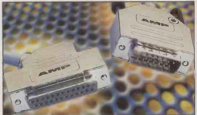
applications such as computer peripherals, industrial equipment, medical and instrumentation. The backshells feature straight or 45 degree cable entry, rugged and compact design as well as excellent EMI/RFI shielding performance. They are suitable for a range of cable sizes while a unique metal filled cable grommet ensures 360 degree shielding. The zinc die-cast nickel plated shells have a -40 to 120°C temperature range, 4.0 to 13.0mm cable diameter and an attenuation factor of over 40dB between
