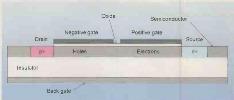
one over each end. As well as this, the channel is doped differently at each end. The result can be likened to two half MOSFETs, a p-channel and an n-channel, in series.
