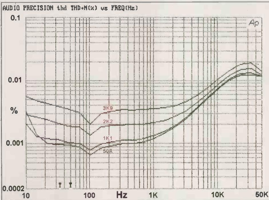
Fig. 3. There is less introduction of ripple and distortion with high-beta input transistors and the same set of source resistances as Fig. 1.
