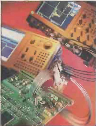
challenges of gaining access to signals with minimal effect on signal integrity; laying out test connectors in limited development board space; real-time triggering on data errors, protocol violations and other anomalies; and correlation of events on microprocessor, internal system bus and external serial bus ports. Analogue and digital timing uses a listing window display.
