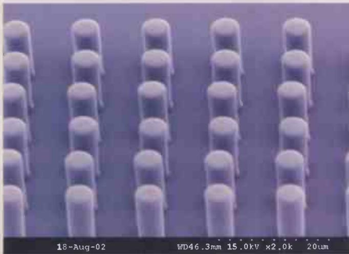
Micrograph of  $5\mu m$  wide polymer pillars distributed on a  $12\mu m$  pitch.
