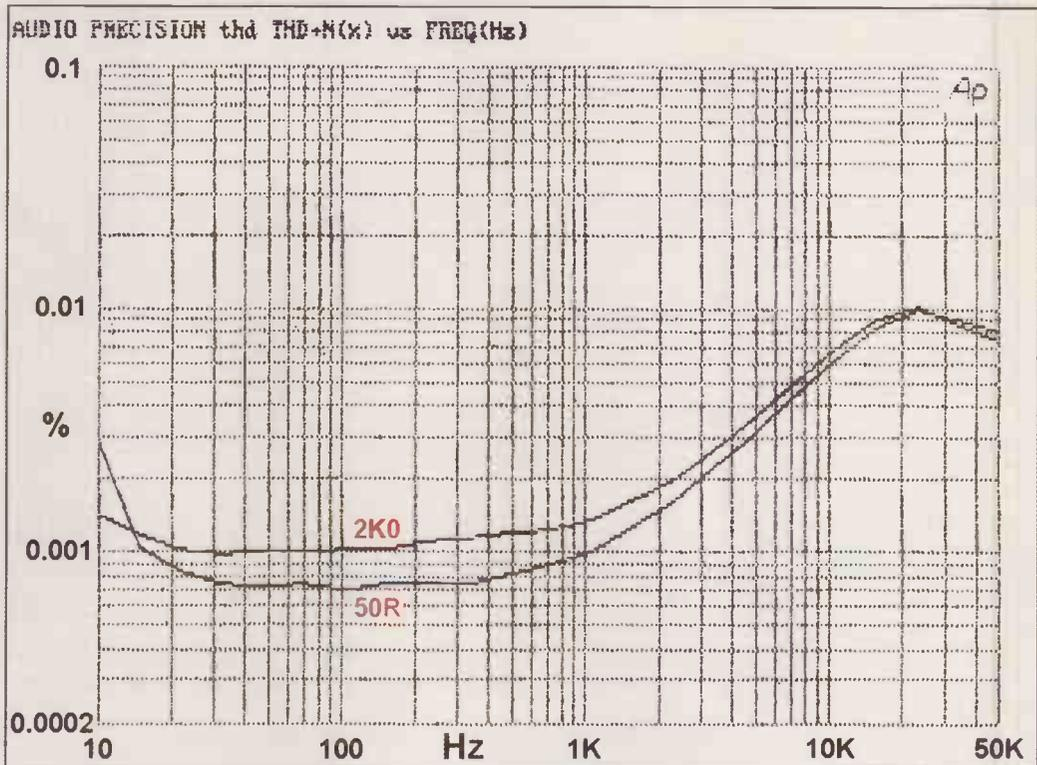
Fig. 6. Cascoding the input tail removes the ripple problem, but not the extra distortion.
