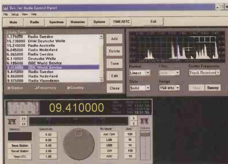
Fig. 3. Ten-Tec RX-320 control program screen.
