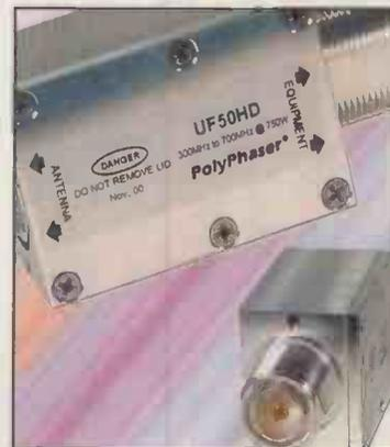
throughput energy. The UF series can be used for transmitters as well as receivers. It also provides positive and reverse voltage protection. Both models feature multi-strike and multi-carrier capability, and are designed to operate over a temperature range of -40 to +85°C. Surge throughput has been measured at significantly less than 5µJ at 3kA (8/20ms waveform).
