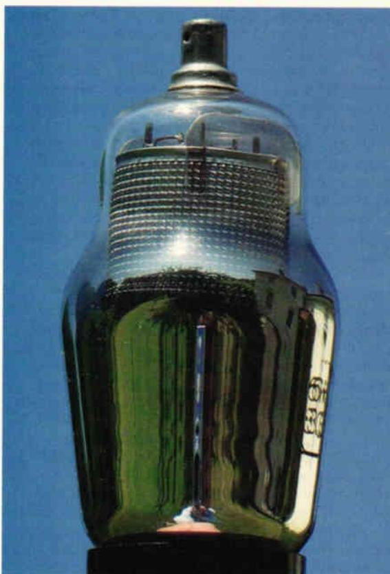
Fig. 5. Valves using oxide coated or thoriated tungsten cathodes appear silvery because of the use of a getter. This is a small amount of reactive metal that is vaporised during the valve manufacture and precipitates on the inside of the glass. Its function is to bind free gas molecules within the valve. It is called a getter because it 'gets' free gas molecules. For a similar reason it is sometimes referred to a 'keeper'.
