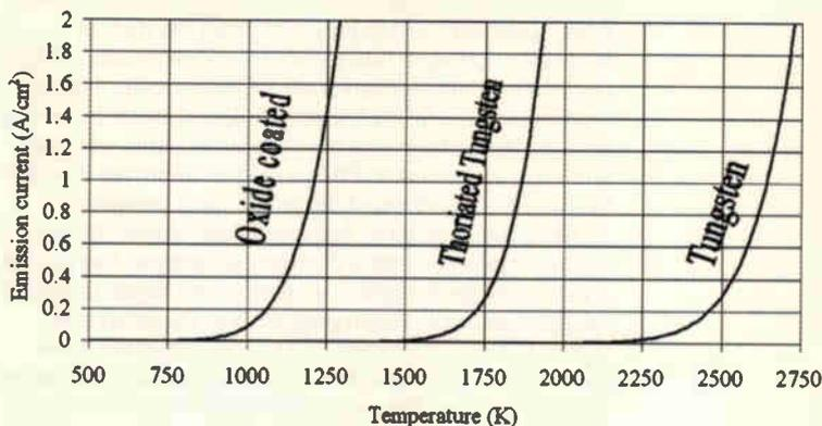
Fig. 1. Plots of emission current per cm<sup>2</sup> against temperature for the three main thermionic cathode types.
