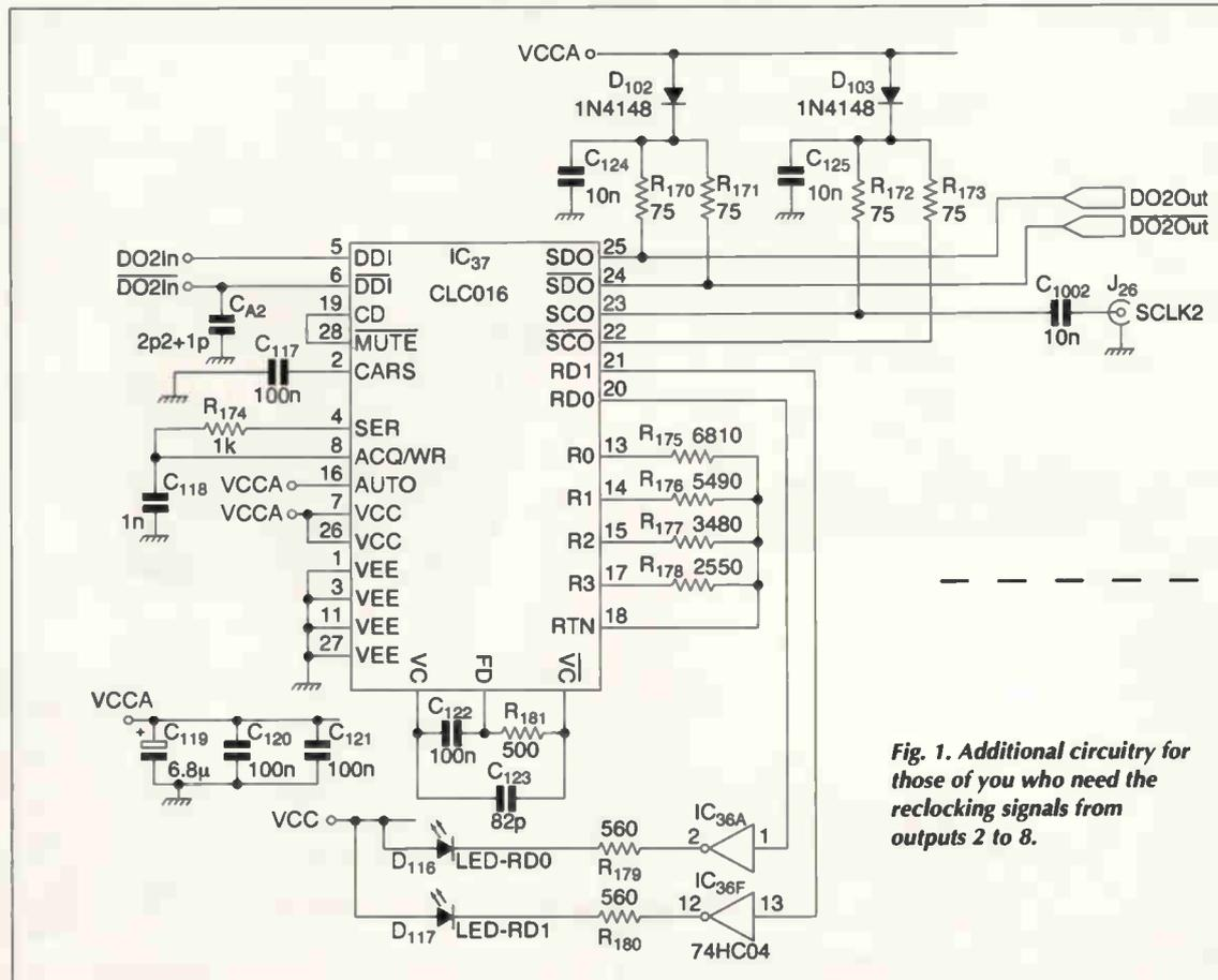
Fig. 1. Additional circuitry for those of you who need the reclocking signals from outputs 2 to 8.
