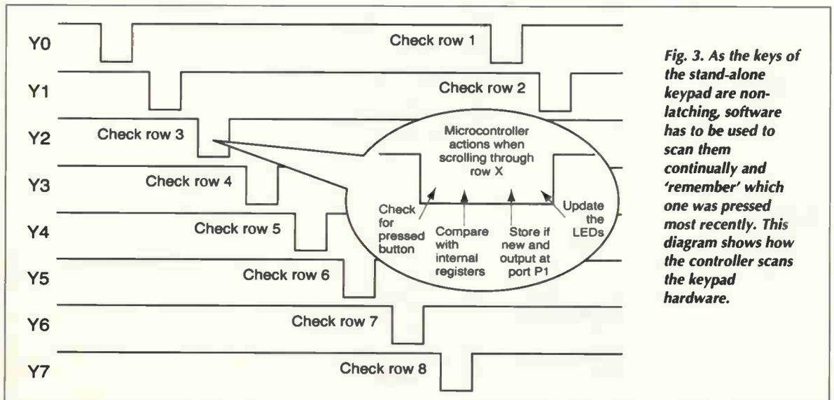
Fig. 3. As the keys of the stand-alone keypad are non-latching, software has to be used to scan them continually and 'remember' which one was pressed most recently. This diagram shows how the controller scans the keypad hardware.
