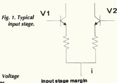
Fig. 1. Typical input stage.
