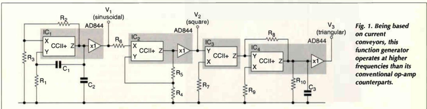
**Fig. 1. Being based on current conveyors, this function generator operates at higher frequencies than its conventional op-amp counterparts.**
