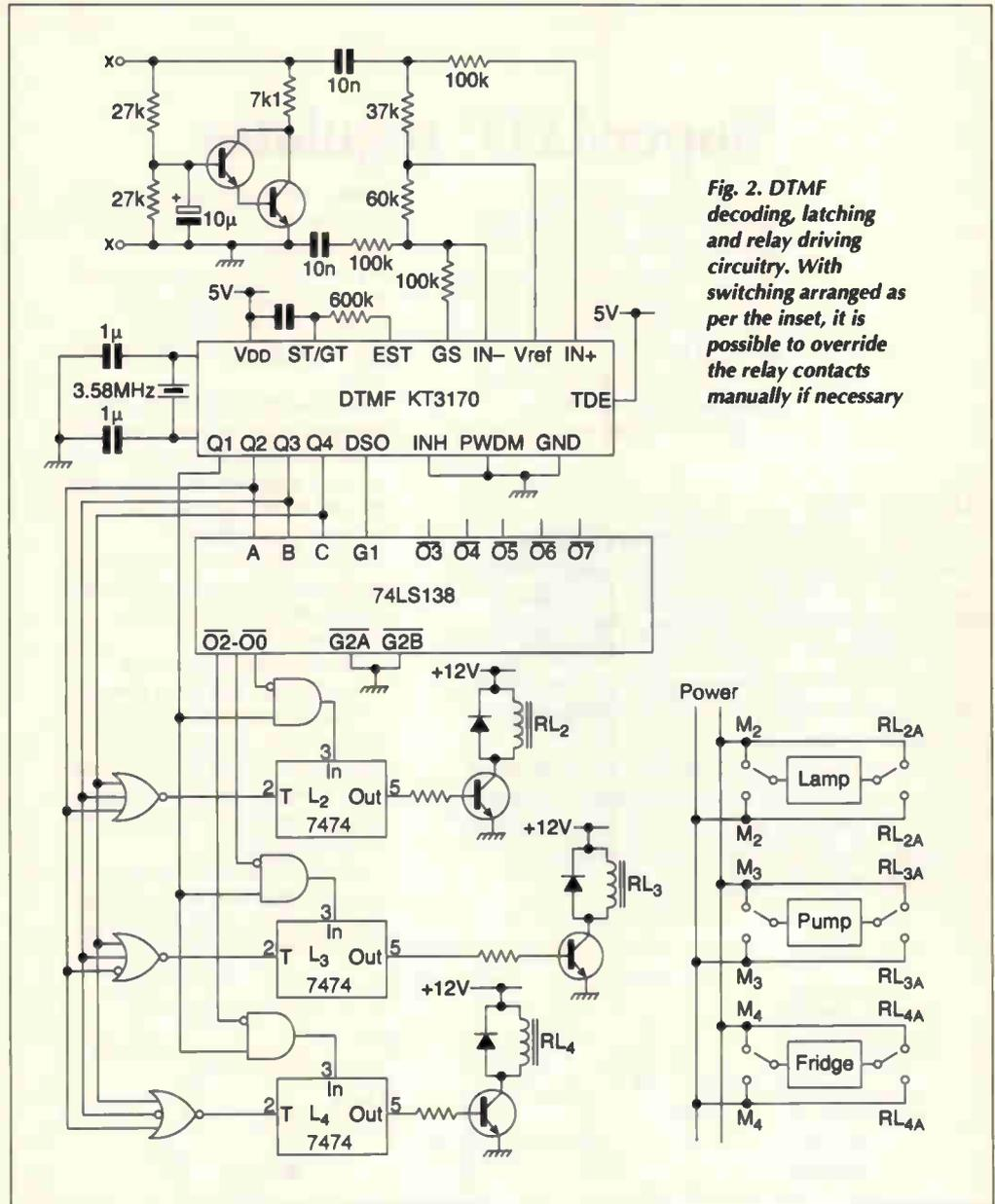
Fig. 2. DTMF decoding, latching and relay driving circuitry. With switching arranged as per the inset, it is possible to override the relay contacts manually if necessary
