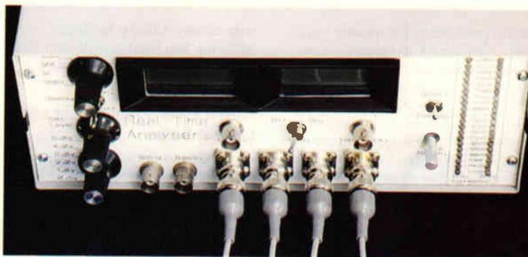
Fig. 2. The four BNC connectors mounted at 22mm centres, provide true four terminal measurements, isolating the test current from the voltage being measured. Enable a quick change from measuring capacitors to amplifier circuits simply by change of test jig, with no change of any internal circuitry.
