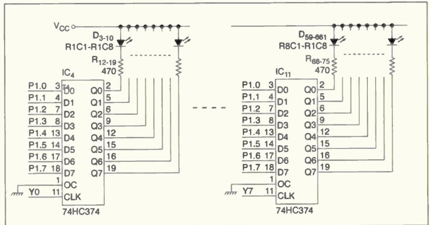
Fig. 4. The router's keyboard's LED display matrix forms a map reflecting which signal's routed where.
