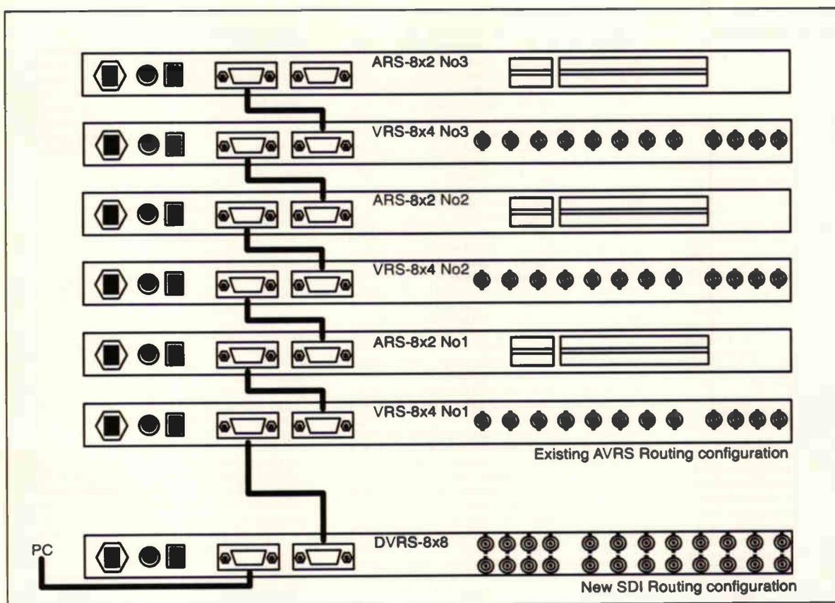
Fig. 7. In studio applications, routers can be stacked in a daisy-chain fashion so that only one command interface is needed.
