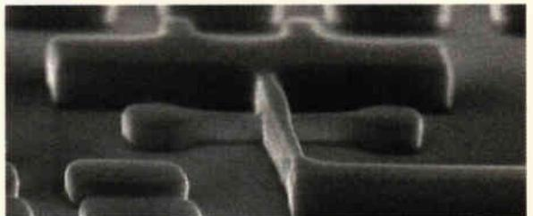
*This 30nm transistor has its silicon channel running from left to right - source to drain - with the gate passing over the top. Thus it contacts the channel on three sides.*
