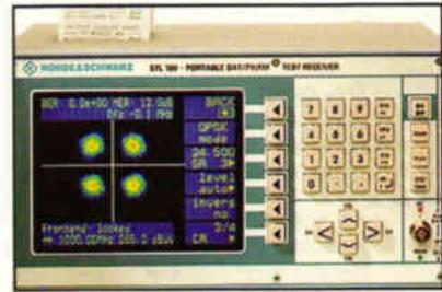
analogue and digital TV and FM radio. The portable instrument includes an on-screen TV picture and built-in printer. In addition the instrument can receive and measure digital TV signals (DVB-Sat, cable, terrestrial) as well as analogue TV and FM radio signals. The on-screen TV picture, the built-in printer for measurement results and diagrams plus the integrated loudspeakers facilitate the operation of the EFL 100. *Rohde & Schwarz*
