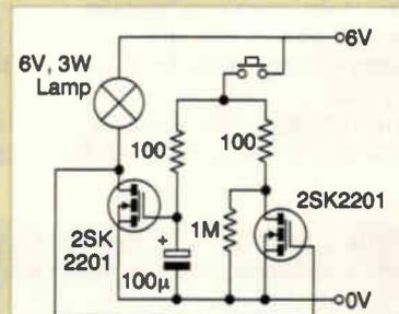
*Battery-operated lamps are popular for applications where it's difficult, or just not worth it, to run mains lighting. Intended to prevent discharge of the batteries if the lamp is left on accidentally, this circuit turns the lamp off after a preset period.*
