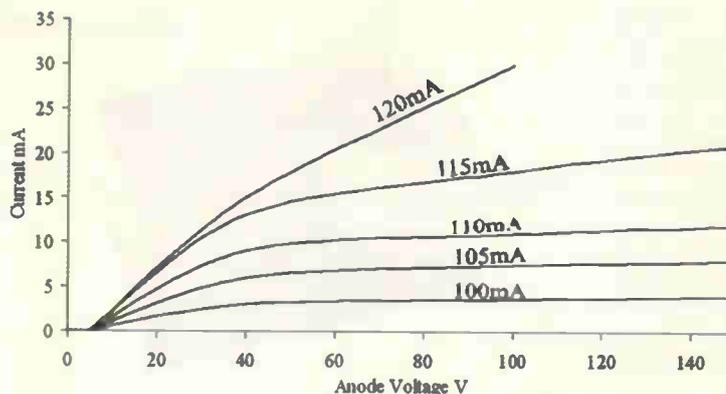
Fig. 4. Characteristic curves of a diode valve to illustrate emission behaviour<sup>6</sup>. Saturation currents are dependent on anode voltage. This is particularly pronounced with oxide cathodes.<sup>6</sup>
