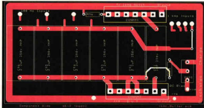
**Fig.5.** Screen shot showing how I modified my original DC bias printed board for use in this cased assembly. By simply cutting three tracks and adding a short link wire, I isolated C91 from the five 2.2 $\mu$ F C92-96 capacitors to provide full four terminal capability to the test jig, allowing capacitor or amplifier distortion measurement
