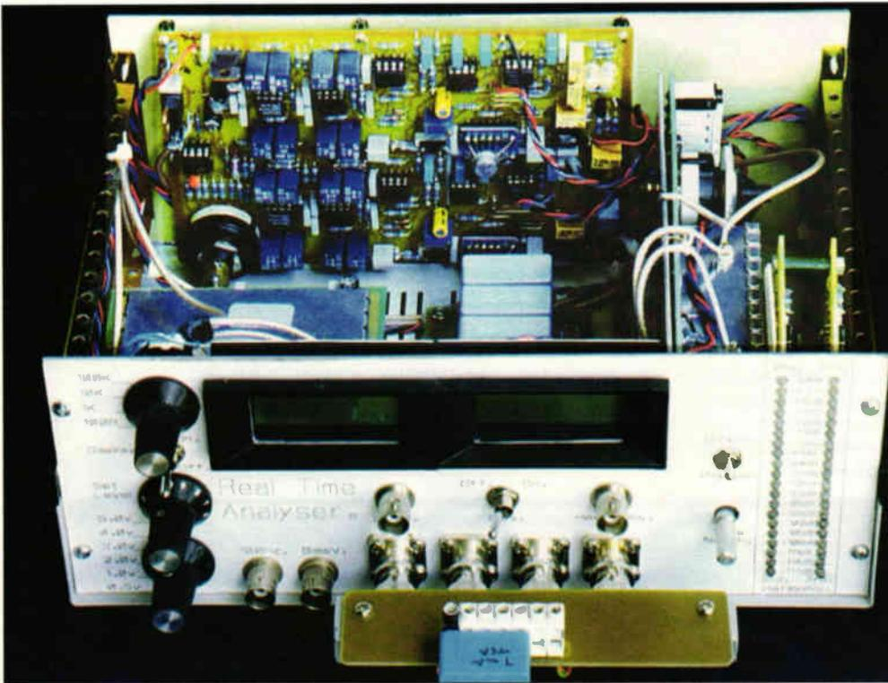
**Fig. 7.** The same assembly now viewed from the front shows the Real Time printed board mounted on the case back panel. This view also shows the added insulation inserted between the LED display board and the notch filter/preamp case lid.
