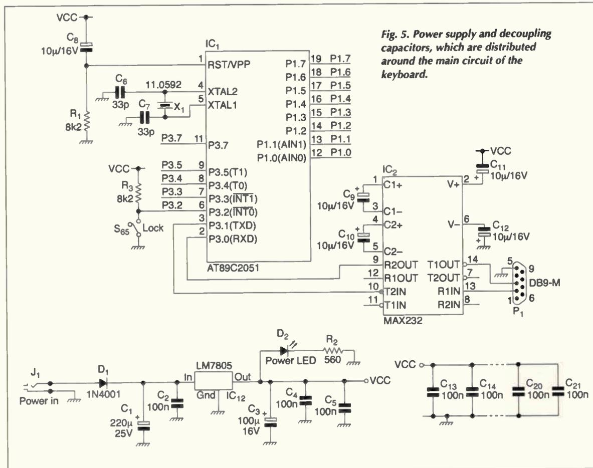
Fig. 5. Power supply and decoupling capacitors, which are distributed around the main circuit of the keyboard.
