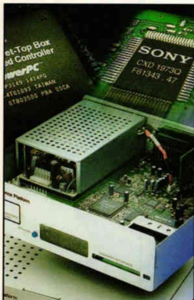
AV SCART switch and common interfaces. IBM provides PowerPC 405 microcontrollers and MPEG-2 compression subsystems. Sony and IBM selected Wind River's VxWORKS operating system, embedded software platform and Tornado cross-development tools for the reference design.
