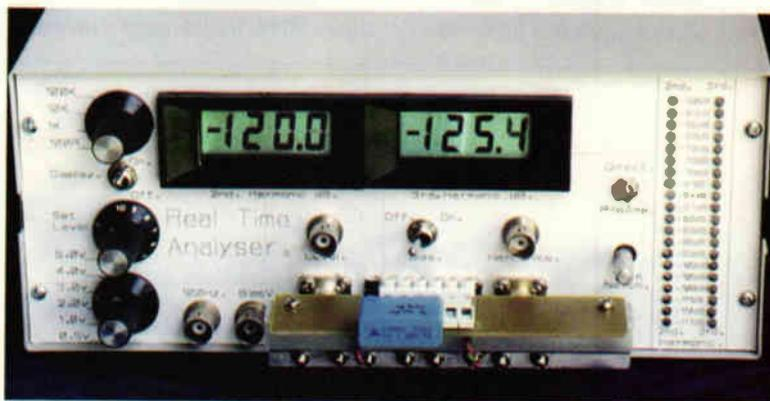
Fig. 3. Testing the 1µF 250V B32653 capacitor which featured in my last article, mounted in my easily fabricated, low cost, four terminal 'replica' capacitor test jig made from a 100mm length of 15mm Aluminium angle, four panel mounting BNC connectors at 22mm centres and a terminal test strip.
