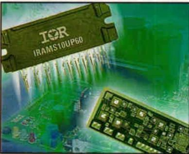
10A, the module is designed for 400W to 750W motor drives found in washing machines, in-room air conditioners and commercial refrigerators. According to the supplier, the module will support the design of multi-shunt current feedback for a vector control loop, in V/Hz control loop, with no circuit layout limitation.
