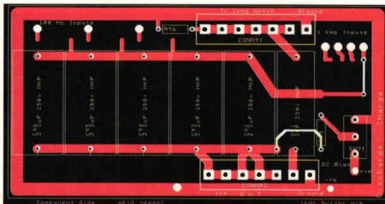
*Fig.5. Screen shot showing how I modified my original DC bias printed board for use in this cased assembly. By simply cutting three tracks and adding a short link wire, I isolated C91 from the five 2.2µF C92-96 capacitors to provide full four terminal capability to the test jig, allowing capacitor or amplifier distortion measurement*
