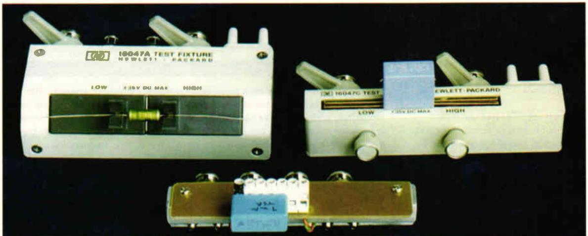
**Fig. 8.** The jigs used for capacitor measurements. The HP16047A jig left, has plug in exchangeable adapters for axial and radial leaded components. The HP16047C jig right, my reference standard, has gold plated contacts which clamp onto component leads. My low cost alternative with a B32653 capacitor, is shown for comparison.
