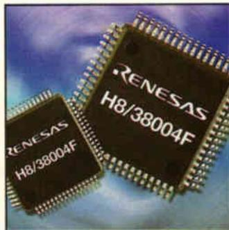
powered and metering applications. Operating voltage is 2.2 to 3.6V, with a fast oscillator start-up, typically about 20µs using an external resonator. This makes it ideal for applications that spend the majority of time in the low power modes. The device has an eight channel 10-bit A/D converter. A peripheral set includes a 10MHz clock oscillator, a 16-bit timer and three 8-bit timers, a USART, and a 25 x 4 LCD display drive. *Renesas*
