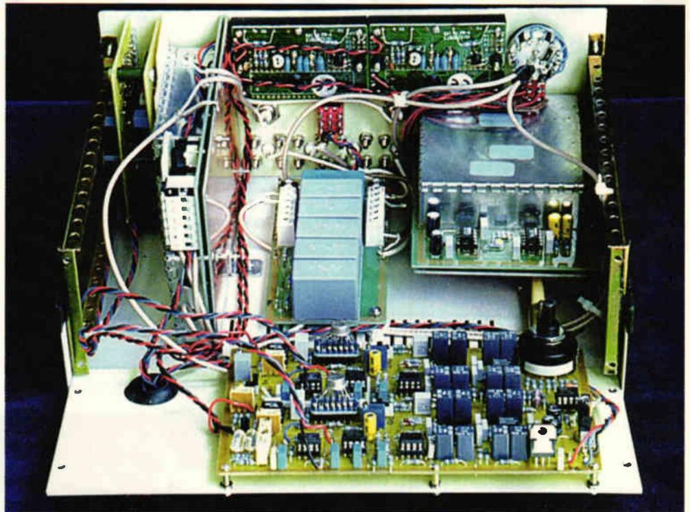
**Fig. 6.** Rear view with the back panel laid flat shows the various coaxial cable connecting between the modules and front panel, in my assembly. The right hand top switch, with three coax cables is the new combined 100Hz and 1kHz source impedance selector, with the 100Hz source impedance arranged ten times larger than for 1kHz, matching the capacitors impedance at these frequencies.
