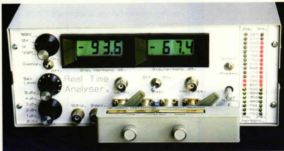
Fig. 1. The Real Time hardware system as described in the July issue, fitted into the low cost LC960 250 x 180 x 100mm case, is shown measuring a 1 $\mu$ F 50v X7R ceramic capacitor at 0.5V using my reference Hewlett Packard test jig. The LED's respond quickly, revealing how this capacitor's distortion changes with time and bias voltage.
