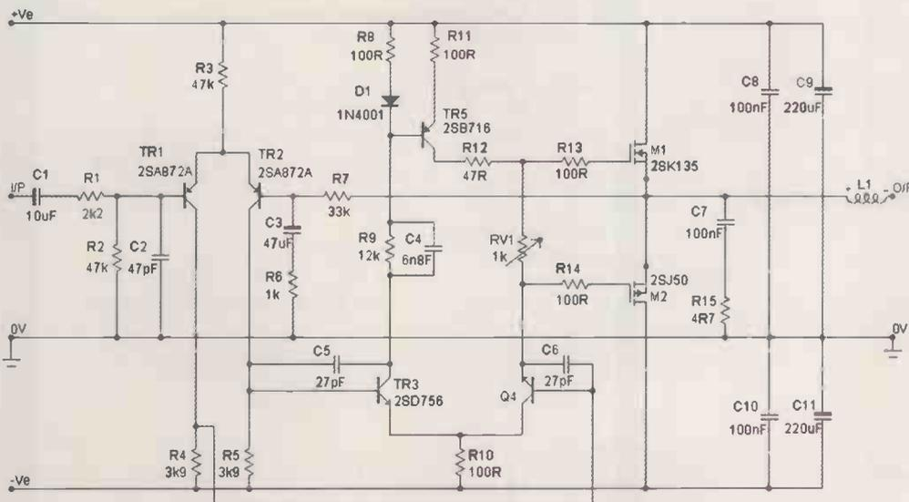
voltages could occur in the circuit sufficient to generate measurably increased distortion. However at my 1kHz distortion measurement frequency, all four capacitors have low impedance, so are subject only to small AC signal voltage drops, apparently not sufficient to explain my measured reduction in distortion when replaced by the same value and voltage bi-polar types.
