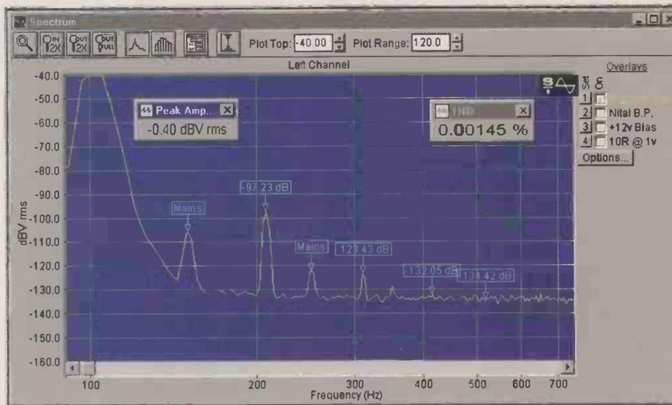
**Fig. 9.** Two 220 $\mu$ F 63 volt Nitai bi-polar capacitors in series made this 100 $\mu$ F "Double bi-polar" capacitor. Measured using a 1 volt AC and 12 volt DC bias as Figure 2, it generates almost twenty times less distortion. Second harmonic measured -101.75dB with 6 volt bias, -117dB unbiased.
