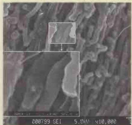
These SEM images show (a) randomly oriented and (b) aligned composites of carbon nanotubes and polypyrrole.
