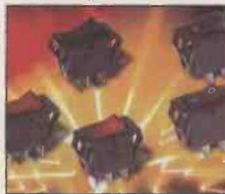
with white, red, amber, or green actuators. Additionally, the actuators can be marked. The CL series feature a positive detent and were designed for easy snap-in mounting. With constant ratings of 16A at 125VAC or 10A at 250VAC, both series have UL and CSA approvals. The CG series also have VDE approval.
