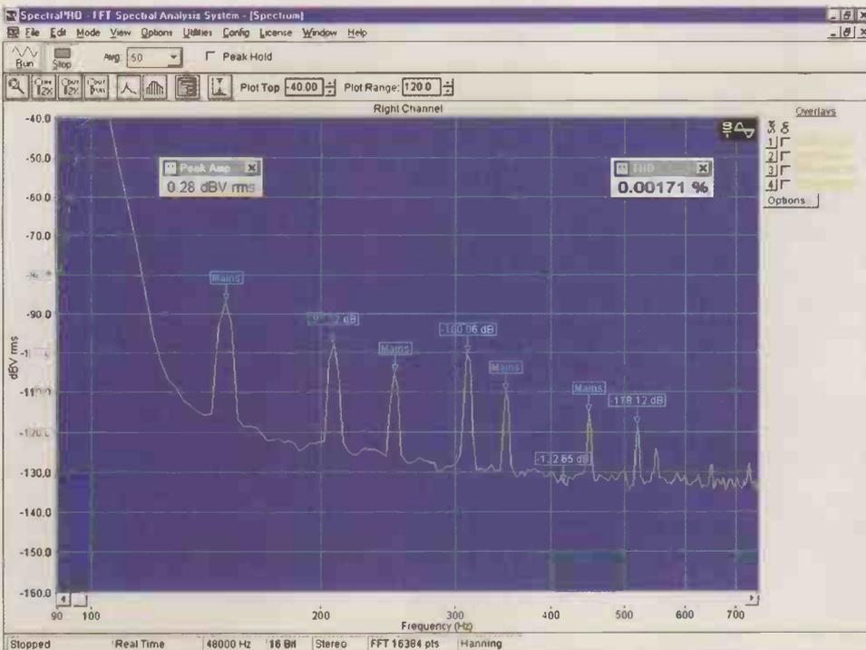
I extracted the feedback resistor network with this capacitor from the main circuit and used the amplifier's output voltage for 100 watt into 8Ω as the stimulus. I measured a radial lead, 47µF 50 volt Panasonic 'S' bi-polar electrolytic, the type used when exchanging the capacitors, for capacitance and ESR by frequency. Self resonance was 300kHz, so estimating 10nH for its self inductance, typical of many radial lead aluminium electrolytics in a 20 × 10mm case, completed the model. Fig. 3.
