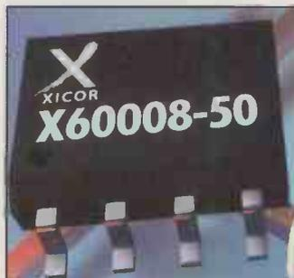
Power consumption is 500nA of supply current. Both devices feature a noise voltage figure of 30μV p-p (0.1 to 10Hz), and an operating temperature range of -40 to +85°C. They are the first devices in an extensive family of precision voltage references manufactured using Xicor's proprietary FGA technology, which the firm claims achieves performance levels that exceed conventional burid-zener and band-gap technologies.
