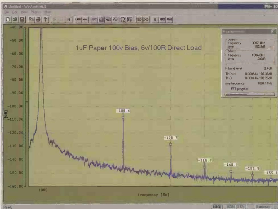
Fig. 10. A typical 1 $\mu$ F paper capacitor, with 6 volts AC at 1kHz and 100 volt DC bias, produced this excessively large second harmonic distortion. The 630 volt 1 $\mu$ F MKP Polypropylene capacitor was five times better with second harmonic - 123dB, third - 130dB, just 0.00008% distortion. This plot was measured using the Dr.Jordan software, the SpectraPlus232 gave almost identical results.
