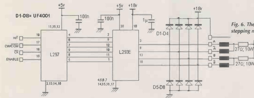
Fig. 6. The simple schematics of the stepping motors drivers.
