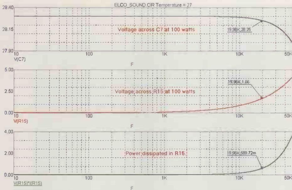
Fig. 7. Using the Figure 3 simulation circuit to analyse for C7, we see the capacitor is highly stressed not resistor R15 and badly chosen C7 can generate large distortion. When an amplifier is used for high frequency sinewave tests with or without load, this capacitor frequently fails open, disabling the Zobel, the amplifier may oscillate. Yet R15 is frequently specified as 3 watt rating and C7 ignored.
