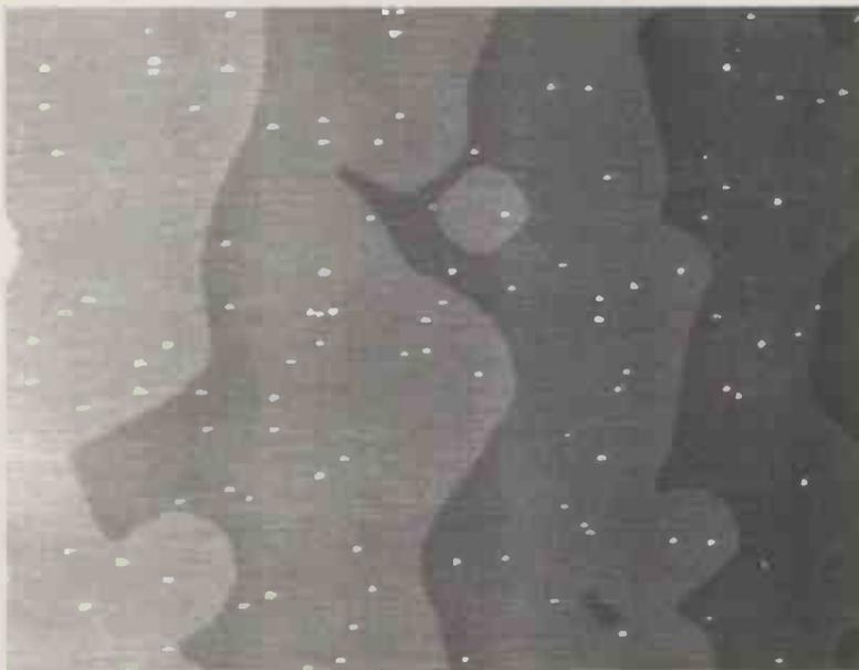
Arsenide nanostructures (white dots) grown onto the substrate by Metal Organic Vapor Phase Epitaxy.
