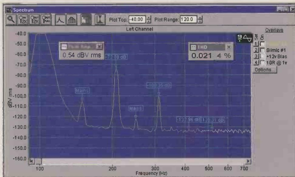
Fig. 2. Distortion results for a Silmic 100 $\mu$ F 25 volt rated polar aluminium electrolytic capacitor, with 12 volt DC bias and tested using 10 $\Omega$  source impedance generating 1 volt across the capacitor. With no bias, second harmonic distortion for this capacitor was -93.2dB and -77.9dB with 6 volt bias.
