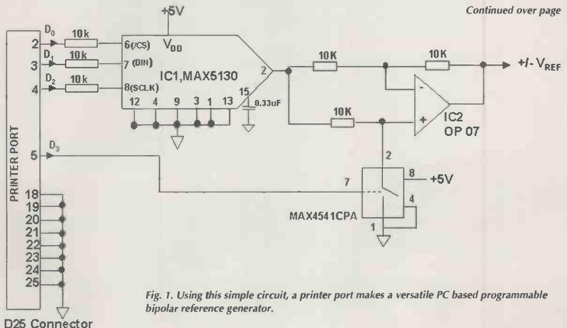
Fig. 1. Using this simple circuit, a printer port makes a versatile PC based programmable bipolar reference generator.
