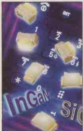
new devices are in the region of 35mcd at a forward current ( $I_F$ ) of 5mA. Maximum  $I_F$  is rated at 20mA, while each LED will handle a peak  $I_F$  of 100mA (pulse duration 30ms).
