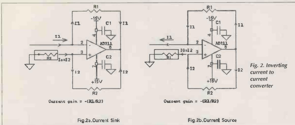
Fig. 2. Inverting current to current converter
