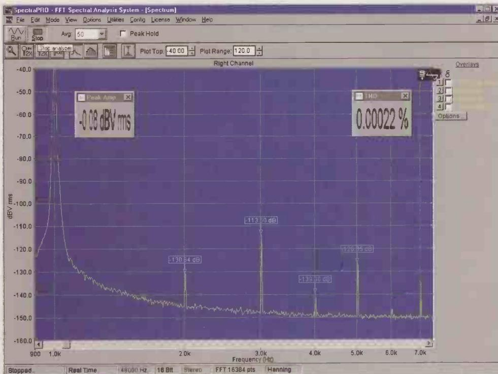
gain reduces with increasing frequency, C4 is subjected to a significant signal voltage. At 10kHz I measured 1.15 volt AC using an AC coupled DVM to ignore the DC voltage. Any polar aluminium electrolytic capacitor subject to such AC voltage will generate very large second and third harmonic distortions.
