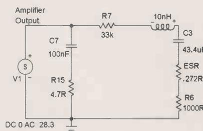
Fig. 3. To simplify my simulations, I extracted the C3 and C7 capacitor sub circuits from the Figure 1 schematic and used the amplifier output voltage as my calculation stimulus. Much simpler, quicker and less prone to simulation errors than when modelling the amplifier.
