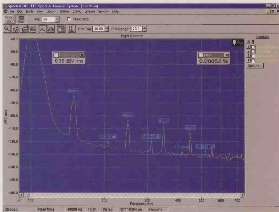
Fig. 6. Without diodes, but otherwise exactly as Figure 5, this Panasonic 'S' 47 $\mu$ F 50 volt bi-polar aluminium electrolytic capacitor shows the distortion reduction available by changing a polar capacitor for a bi-polar type. With diodes, third harmonic increased more than 20dB to -99.24dB, further proof of the diode effect.
