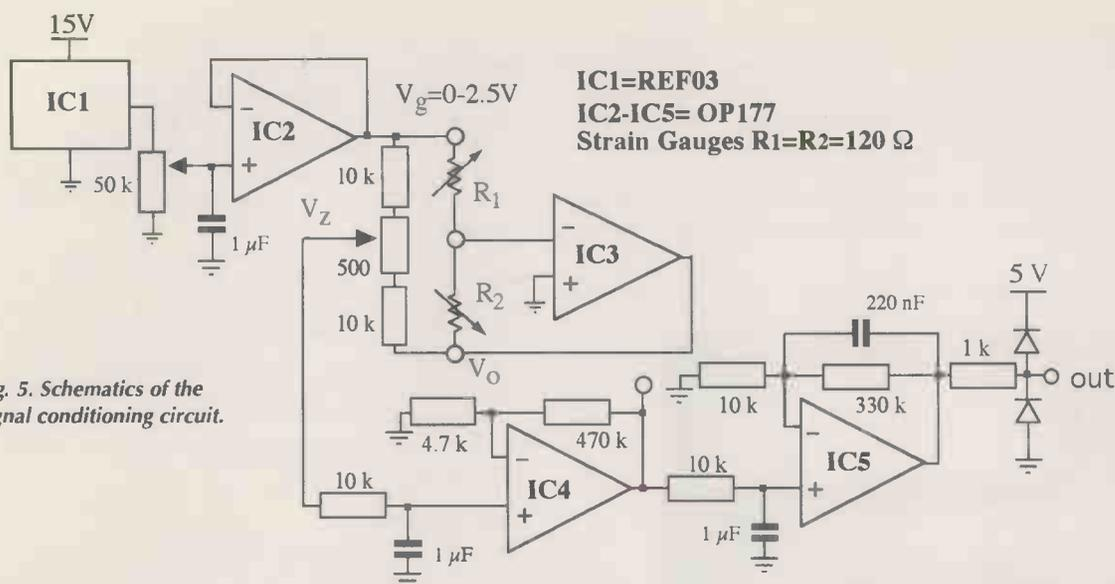
Fig. 5. Schematics of the signal conditioning circuit.
