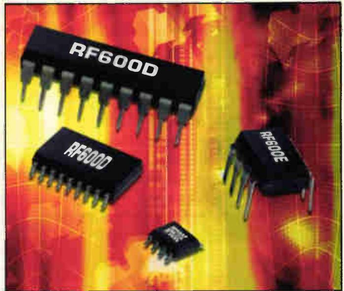
transmission, or buffer data received over the radio link before it is transmitted to the host. Control lines are used to handle the flow of data to and from the host. Data packet generation is automatically performed along with 'Manchester' encoding and CRC-based error checking. Further hardware features include two digital telemetry lines and an asynchronous serial host interface.
