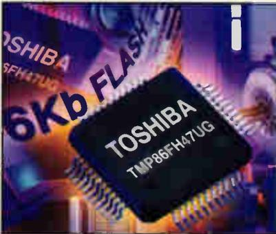
There is dual-clock operation and, in addition to the built-in stop mode, it has eight power-down modes. These comprise slow 1 and 2, idle 0, 1 and 2, and sleep 0, 1 and 2.
