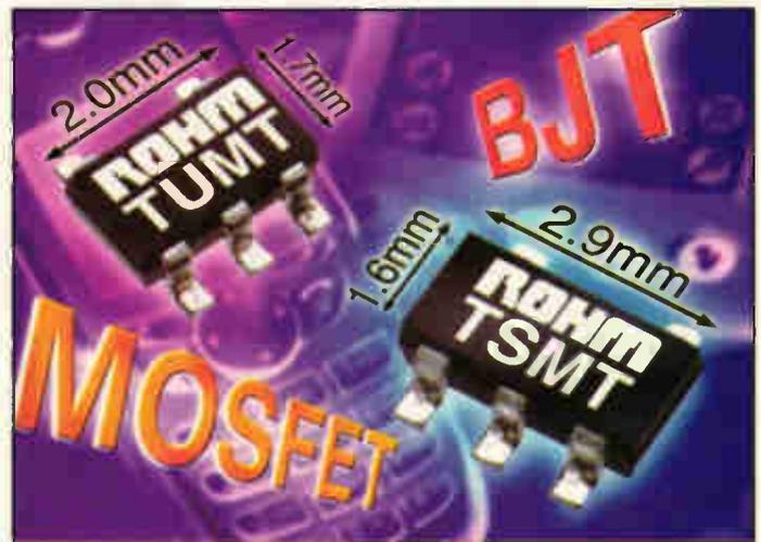
Typical on-resistance values are down to 31mΩ at a V<sub>GS</sub> of 4V (dependent on device chosen). The TUMT-packaged Mosfets have drain currents up to 3A, while on-resistance values are 50mΩ at a V<sub>GS</sub> of 4V. Power dissipation for TUMT devices is rated at 0.8W. Both series include single- and dual- Mosfet options, each of which can be supplied with or without a built-in Schottky diode.
