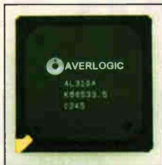
applications that require input switching. As well as the ability to directly display panels, the AL310 has triple embedded video DACs, which provides RGB or YPbPr progressive analogue output. Resolutions up to SXGA (1280 x 1024) are supported. The device is capable of accepting multiple digital formats (RGB/YCbCr/YPbPr).
