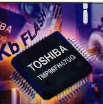
There is dual-clock operation and, in addition to the built-in stop mode, it has eight power-down modes. These comprise slow 1 and 2, idle 0, 1 and 2, and sleep 0, 1 and 2.
