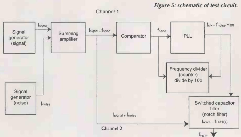
Figure 5: schematic of test circuit.
