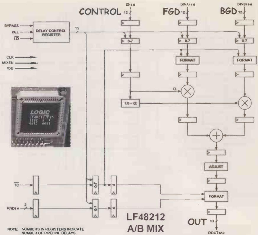
registers, which are set to correct the delay due to the key processing stage. Satisfactory luminance and very simple 'blue screen' keying using the Cb signal has been achieved.
