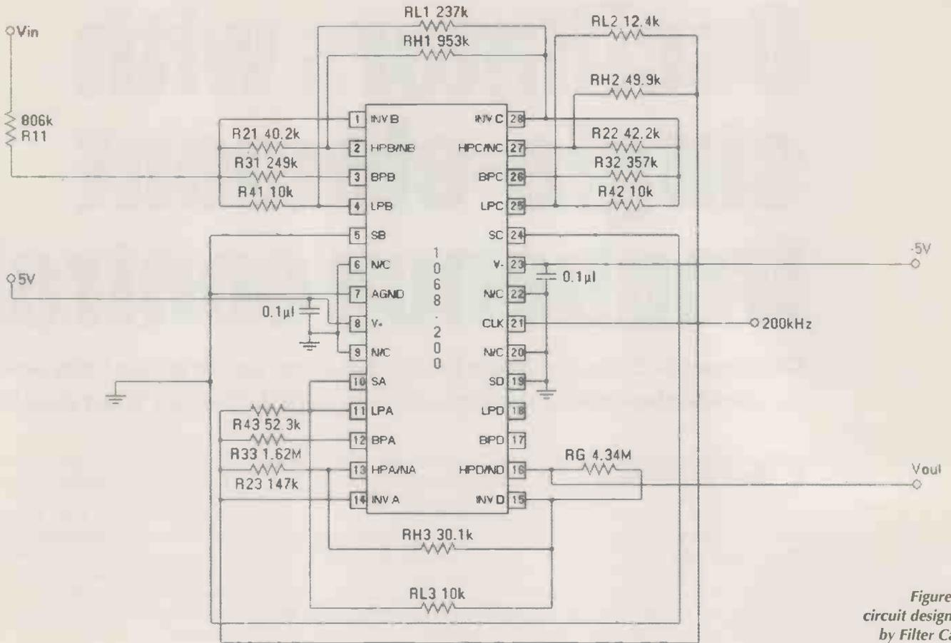
Figure 9: circuit designed by Filter Cad.
