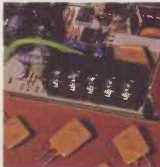
on the primary side of the circuit, in proximity to potential heat-generating components such as magnets, FETs or power resistors, the LVR device can help provide undercurrent and overtemperature protection with a single installed component. Available in straight-lead or kinked-lead configurations the devices can be supplied in tape-and-reel packaging for compatibility with high-volume assembly.
