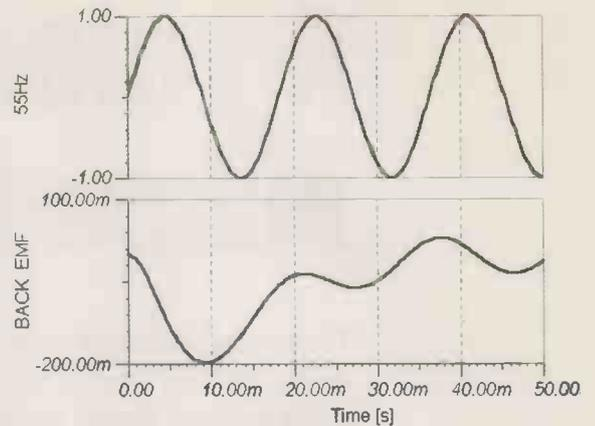
**Figure 9: The first cycle error potential that develops at an amplifier's output terminals when a real-world loudspeaker loads an internal 4,700 $\mu$ F series output capacitor.**
