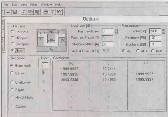
Figure 8: results screen from Filter Cad.
