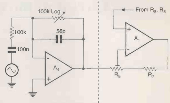
Figure 5: adding an input buffer/attenuator turns the circuit into a selective amplifier. For maximum  $Q$ ,  $R_8$  is set for 'just not oscillating'. In the oscillating state application of a near-synchronous signal can lock the frequency
