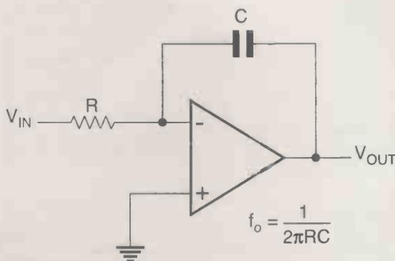
Figure 2: Inverting switched capacitor integrator.
