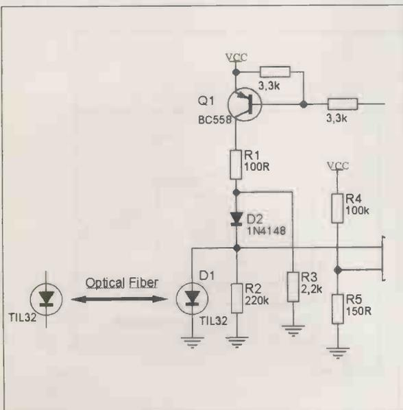
Optical fibre is the best transmission medium when reliable communication has to be performed in electrically noisy environments; especially when galvanic isolation is required. However, a drawback of fibre optics is that usual transmitters and receivers are unidirectional, since they must be optically coupled to the fibre. Two-way communication usually requires two fibres running in parallel, and also two pairs of optical transmitters + receivers.
