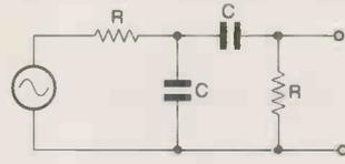
Figure 3a: Cascade RC, CR network has a response like the Wien.
