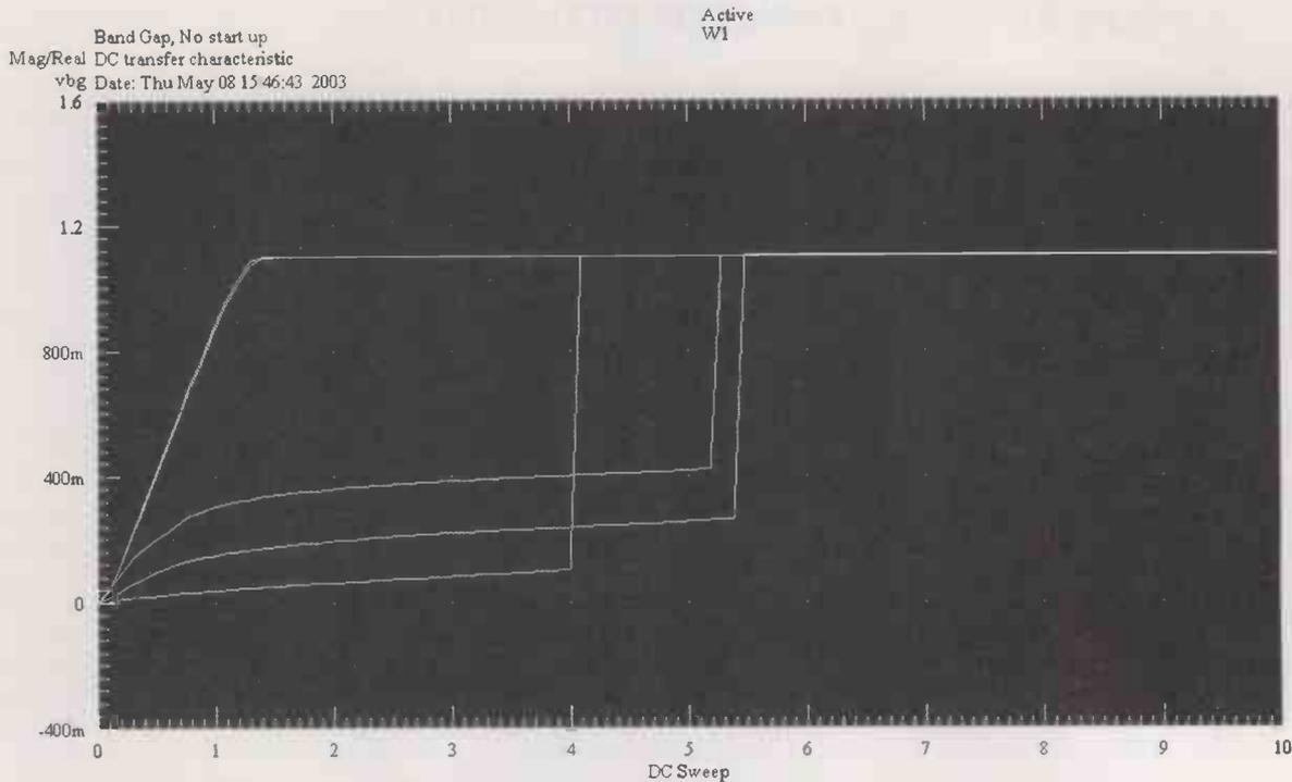
this case  $\Delta V_{be}$  is a standard 52mV from  $25mV \cdot \ln(8)$ , giving a current of  $3\mu A$ . If QN6 and QP8 are non conducting, indicating that the main circuit is off, MN1 will pull current through QP1 forcing QN11 and QN12 to turn on, which will force Q6 to turn on. Once Q6 is on, it will cause the startup current of MN1 to be diverted away from QP1.
