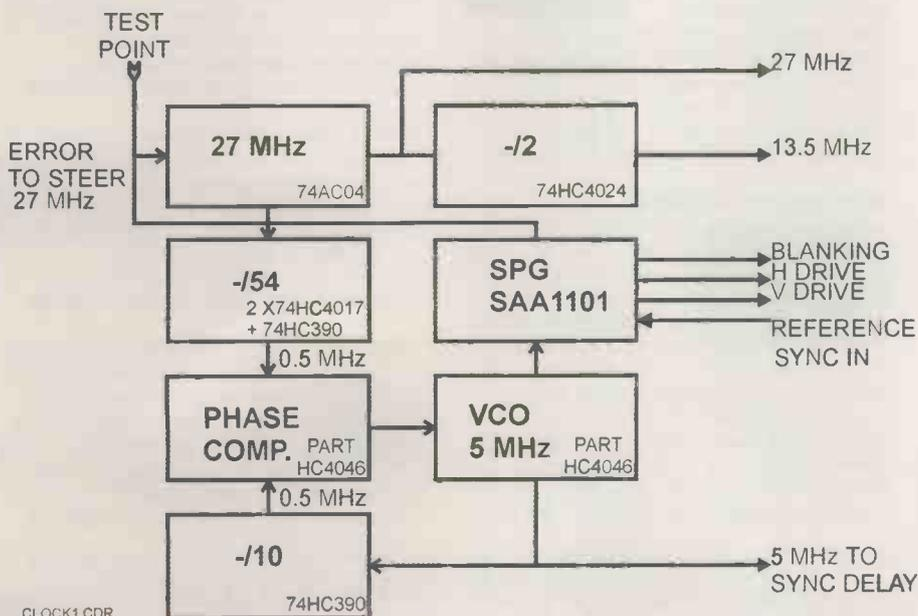
mixer had been used in anger, it was found that this was not the optimum arrangement for jitter performance. Subsequently, the 5MHz crystal was removed from the SPG and the 74HC4046 reconfigured to act as a 5MHz VCO. The VCO output fed the SPG oscillator input. The dividers remained as before, and the SPG error steered the 27MHz clock oscillator directly. This resulted in greatly improved jitter performance.
