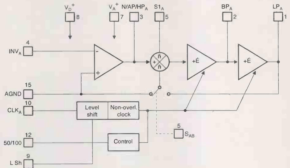
Figure 4: LMF100 schematic.
