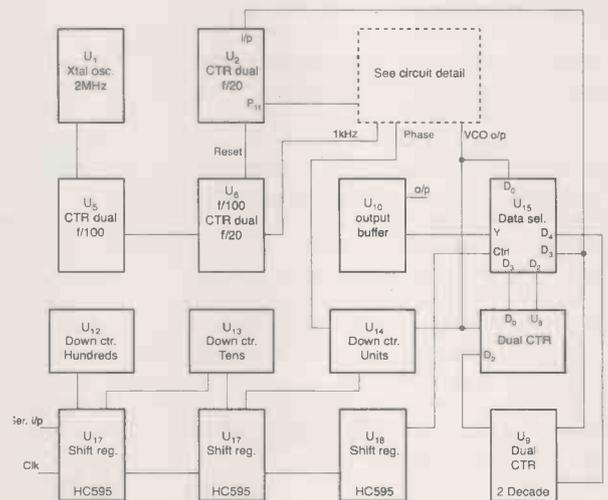
HCMOS available when this project was built as a switch controlled version. The zener control of  $U_4$  was to get the best performance from the 4046 PLL. The use of all HC devices with a 5V supply would probably extend operation several MHz by the use of the range switching idea described here, with component selection and the range switching frequency chosen.
