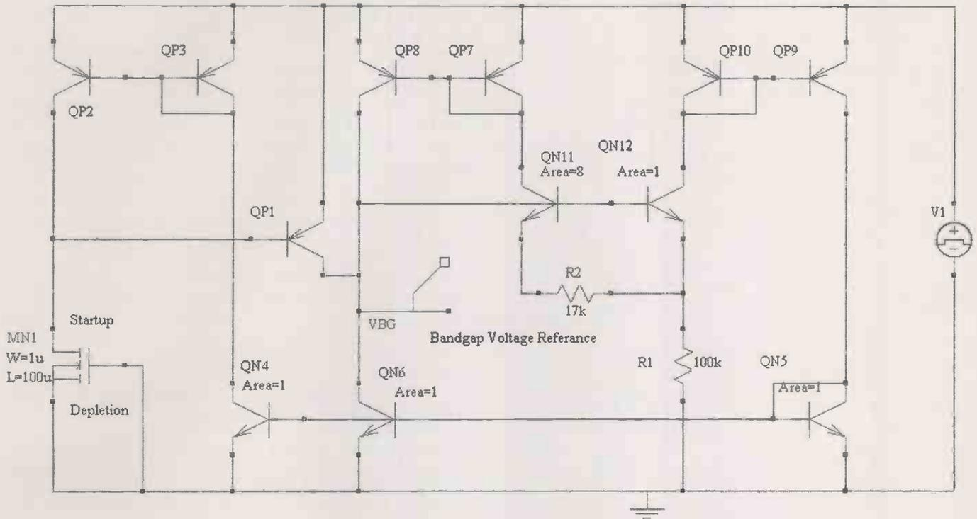
The circuit design described here was developed to solve some specific issues in a design of a Band Gap voltage reference in a BiCmos process. However, the technique described here can be applied to many alternative situations.
