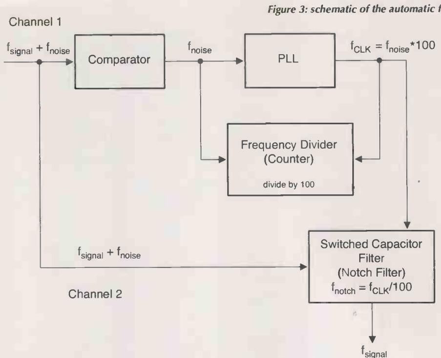
Figure 3: schematic of the automatic filter.
