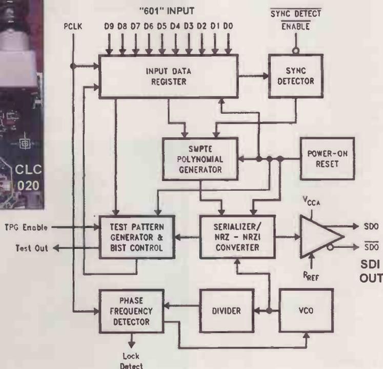
Block diagram of the serialiser, and its place on the output card.
