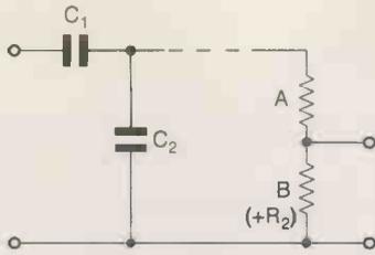
Figure 2c: effective network at very low frequency.
