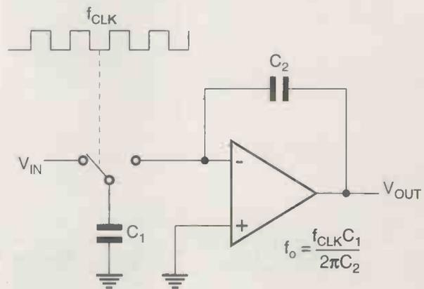
the filter centre frequency usually 50 or 100 times the frequency. This means that we can build a versatile notch or peak filter using only four chips. The schematic is shown in Figure 3.
