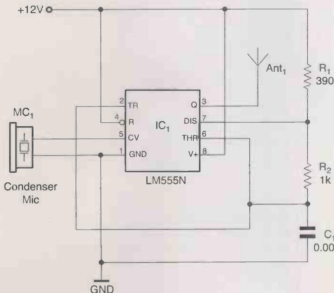
Here is a simple radio transmitter for transmission up to 25 metres. It is basically an AM modulator whose signal can be received on a normal AM radio. It can also be used as an AM radio tester.
