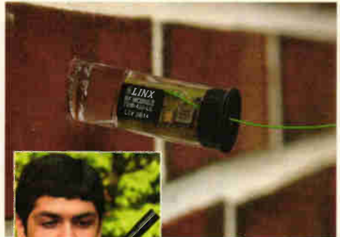
Top: A sticky-tipped wireless sensor, the green lead is an aerial.
