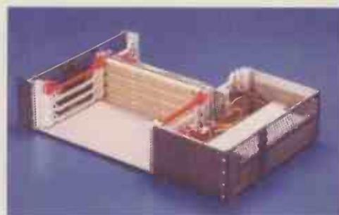
The systems that can be configured as 482.6mm rack mounting units or, without mounting flanges, as desk or bench top systems are built from steel, with mounting flanges that may be fitted either at the front or up to 100mm towards the rear if preferred. Inside, each 1U of height is equipped with 4 codable guide rails to create 2 standard (4HP) slots, with additional models also having 80mm rear I/O (CPCI) or 160mm rear I/O (VME).
