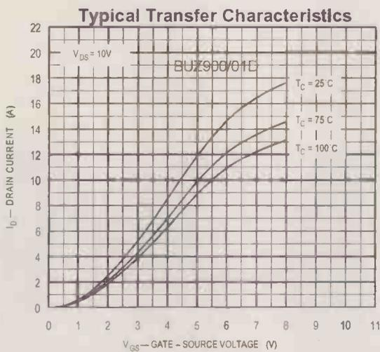
Figure 4: The datasheet curves for the BUZ900/01D MosFet are small, so difficult to read especially for small currents. These transfer curves were printed as large as possible, then annotated with actual spot values to facilitate developing my model.
