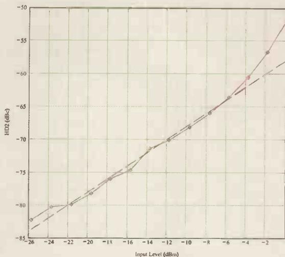
**Figure 1:** Measured second harmonic distortion characteristic of an Advantest R3261C spectrum analyser at 1.1MHz.
