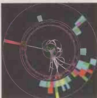
*Simulated response of linear collider detector to supersymmetry displaying the characteristic signature of a lepton, a hadronic jet and missing transverse energy.*
