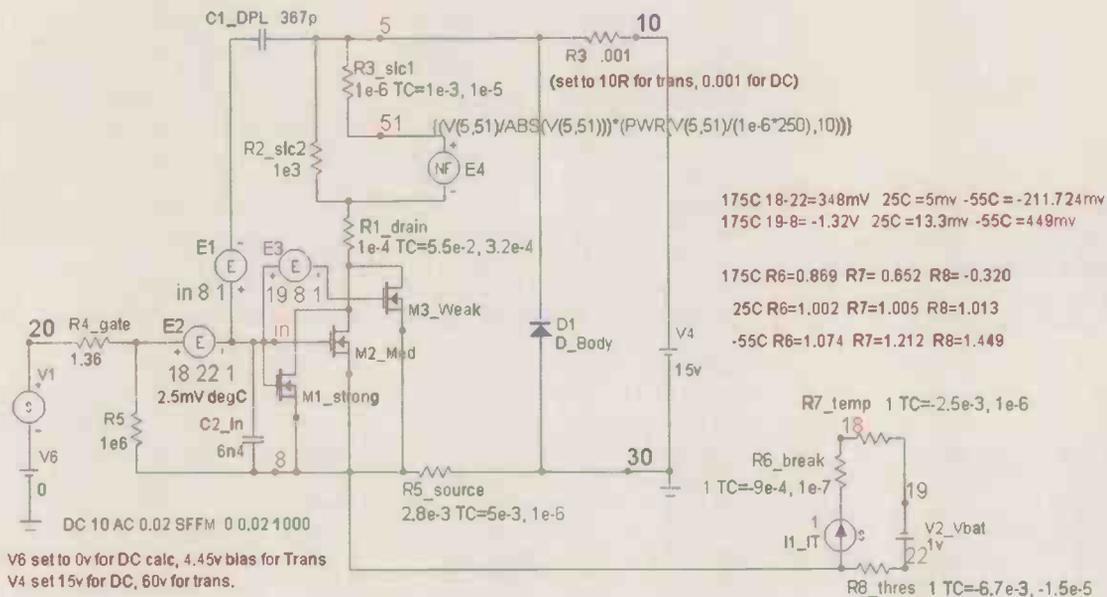
**Figure 2:** Nodes 10, 20, 30, representing drain, gate and source connections into the subcircuit model, will be translated by the MC6 schematic shape editor into the connecting nodes 1, 2 and 3 for the final subcircuit model. This schematic was used to plot and quickly refine the model, the first step towards the netlist needed for our subcircuit model.
