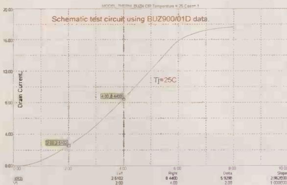
Figure 5: Attaining this smooth merging of the sub threshold conduction - square law regions, important when modelling distortion, completes stage 1 for our model. Our 25°C curve shows good agreement with the datasheet.
