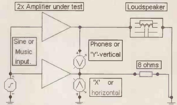
Figure 24: The 'X-Y' amplifier interface distortion monitoring arrangement
