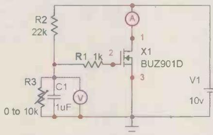
Figure 8: The simple test circuit used to measure the subthreshold region transfer curves, providing additional data points for this critical crossover region. Measuring a 'P' MosFet the supply polarity should be reversed.
