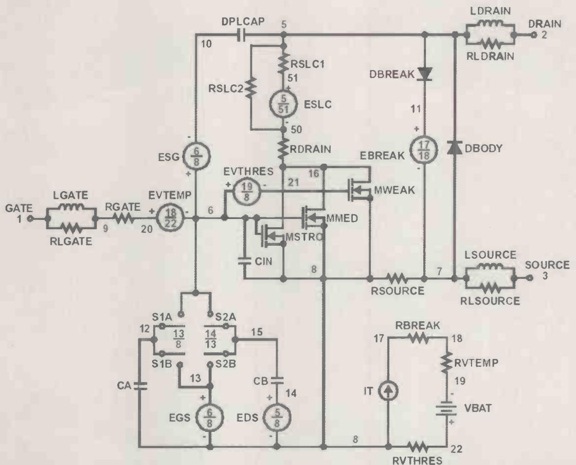
Figure 1: Fairchild's PSpice schematic for their FDP038 subcircuit model. Modelling audio frequency distortion, the circuit voltages used to drive the gate-source capacitance switches should not occur. To minimise convergence problems these switches were deleted from my audio models.
