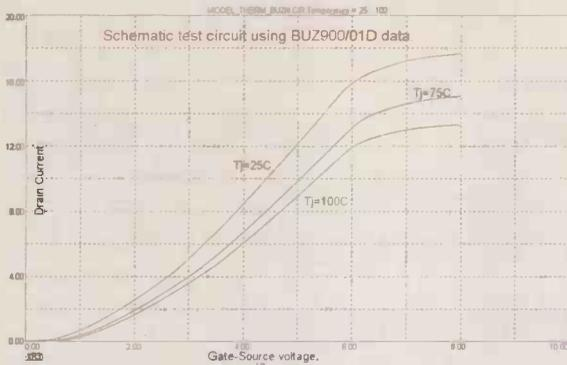
Figure 7: Using the values shown in figure 6, these temperature plots display particularly good agreement with the datasheet for drain currents up to some 12A.
