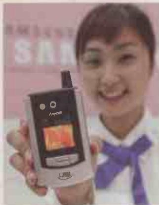
Samsung's SPH-V5400 is claimed to be the first mobile phone with an internal hard drive. The drive, which measures 25mm diagonally, can hold 1.5Gbyte of data, compared with a maximum of 100Mbyte in more conventional phones, said the firm. The phone is also equipped with a 56mm QVGA LCD and a mega-pixel camera as well as features including an MP3 player, electronic book and Korean-English/English-Korean dictionaries. Initially, the phone is only being sold in Korea.
