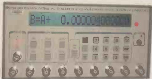
Four Channel Digital Delay Generator
