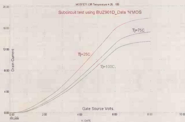
Figure 11: Having completed the netlist needed for the subcircuit models, we can at last test the finished subcircuit models. Using MC6 I found some final tweaking was needed.
