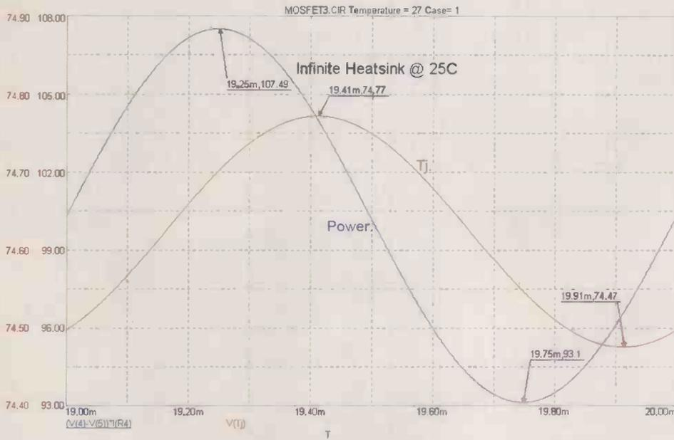
Figure 9: Proving the models do work. This 20th cycle transient simulation using the figure 1 subcircuit model and infinite heatsink, shows power dissipated peaking at 107.5W and 93.1 minimum or 100.3W mean power, giving a theoretical junction temperature of 75.1°C, close to the models 74.77°C, which temperature has not yet fully stabilised.
