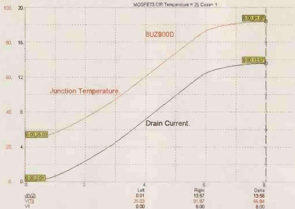
Figure 7: Used in self heating mode with an infinite heatsink at 25°C ambient, this DC sweep of gate voltage from 0 to 8 volts with 10V drain-source, using the figure 1 circuit, shows how the junction temperature rise lags behind the power dissipated in the transistor, with increasing gate volts. Initially at room temperature, by the end of this sweep, junction temperature has risen to near 92°C.
