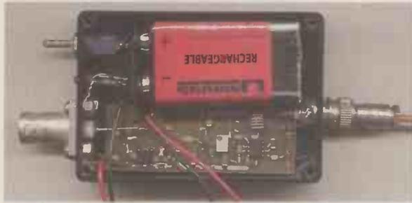
This uses the double balanced mixer/oscillator in the Philips SA612. The tuned components (L1 wound on a 1/4 inch former; 6 turns) are set up for the 100MHz area, but can hopefully be scaled up to 200MHz. The 30pF tank capacitor can probably be replaced with a small trimmer if required, to extend the
