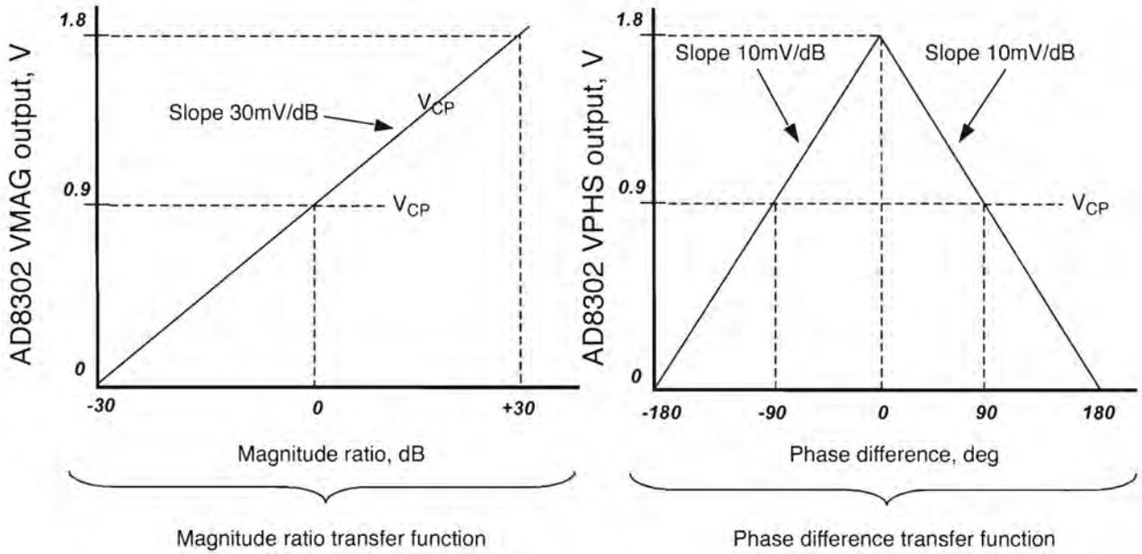
Figure 2: AD8302 gain and phase transfer functions
