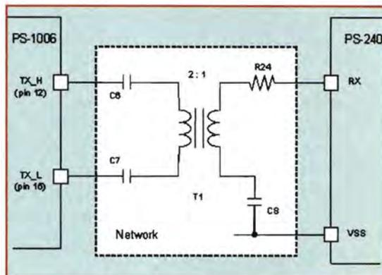
**Figure 6:** Communication link components
