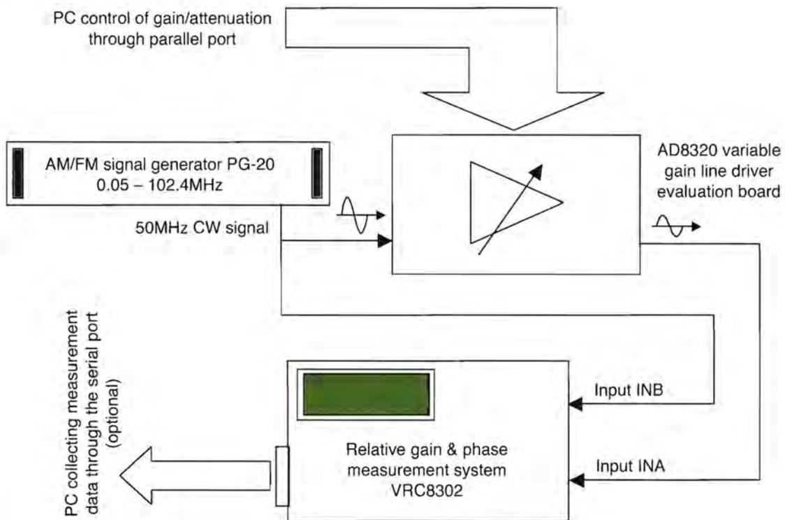
Figure 6: Magnitude ratio measurement set-up implementing a programmable attenuator/amplifier
