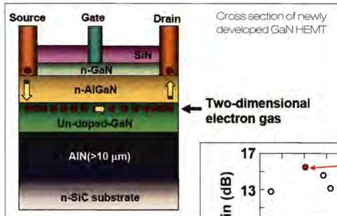
Fujitsu overcame these by forming an aluminium nitride (AlN) epitaxial layer of above 10 $\mu$ m on the conductive n-type SiC substrate, followed by depositing an epitaxial layer of GaN HEMT developed on top of that substrate. The firm discovered that the parasitic capacitance is lower when the AlN thickness goes above 10 $\mu$ m, which in turn, yields high gain. In addition, by using AlN, which features
