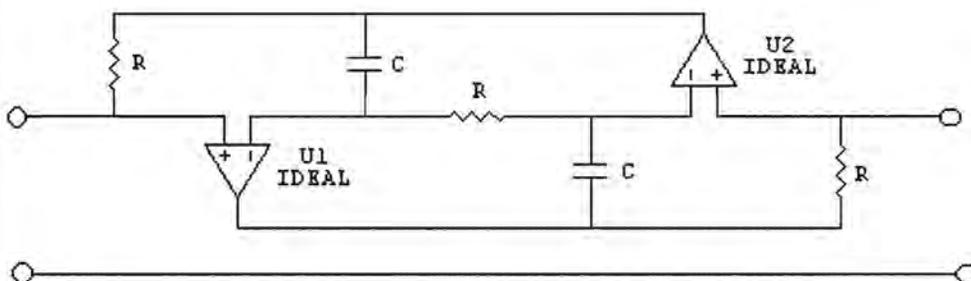
The end circuit represents a floating negative inductor using only two op-amps. It obviates use of GIC (General Impedance Converter) that requires more than four op-amps for the same purpose. It requires two matched capacitors and three matched resistors.
