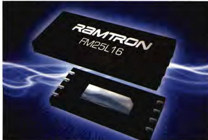
lead-free 8-pin SOIC package.
