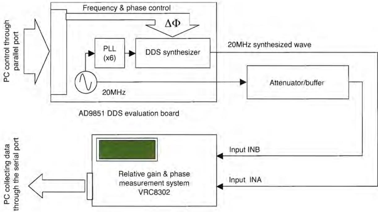
Figure 5: Phase response measurement set-up using a DDS synthesiser and its local oscillator
