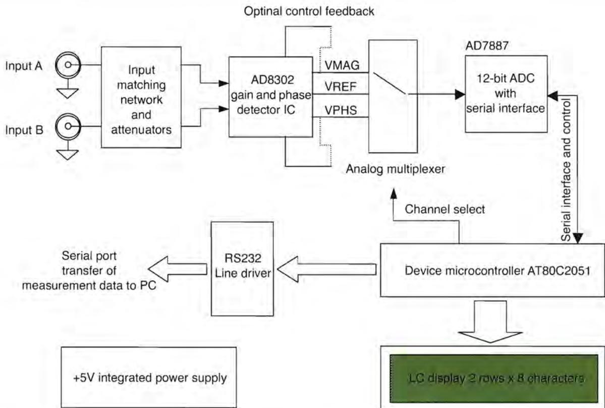
Figure 3: Functional structure of the gain and phase measurement system
