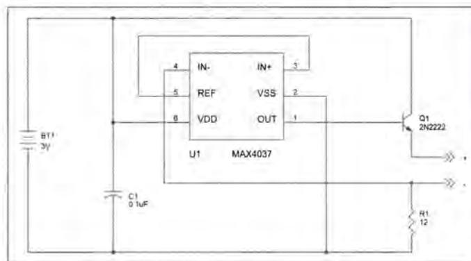
tional amplifier with a built-in 1.232V reference. The positive input of the op-amp is connected to the reference directly. The negative input is through a 12Ω resistor to ground. Output of the op-amp drives an NPN transistor to increase the driving current. Terminals '+' and '-' are used
