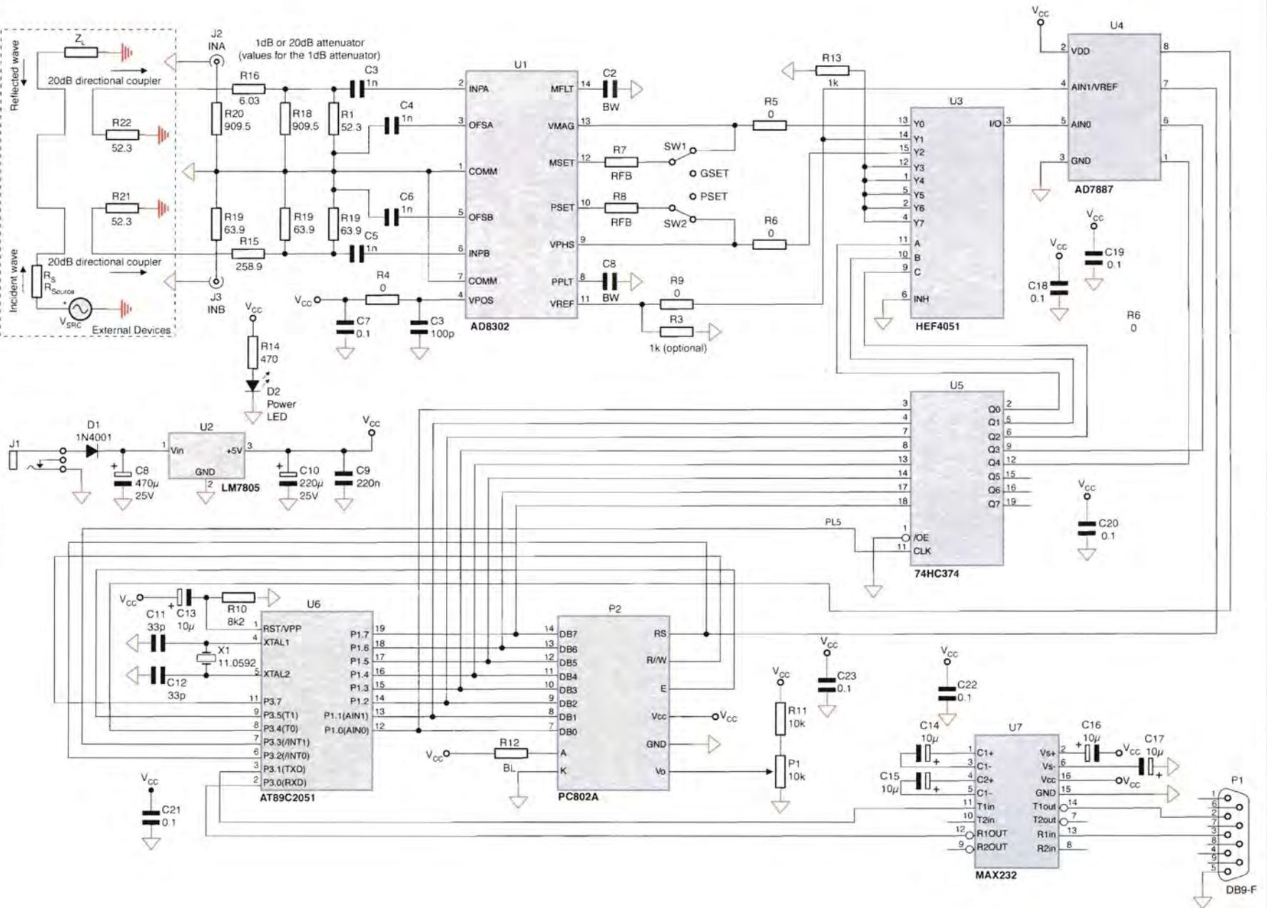
Figure 4: Schematic diagram of the gain and phase measurement system, VPC8302
