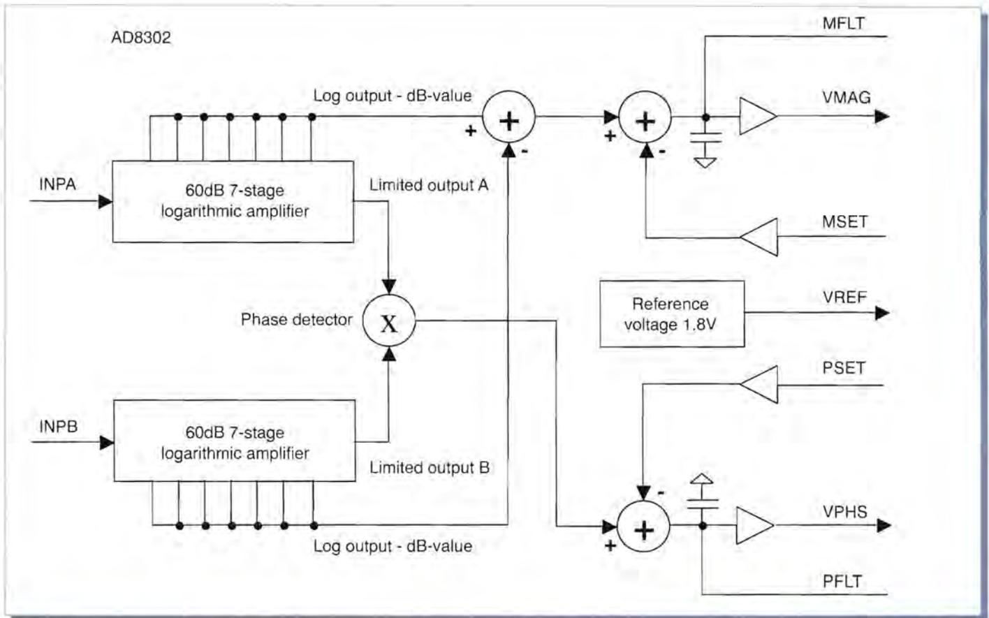
**Figure 1:** AD8302 gain and phase detector internal structure
