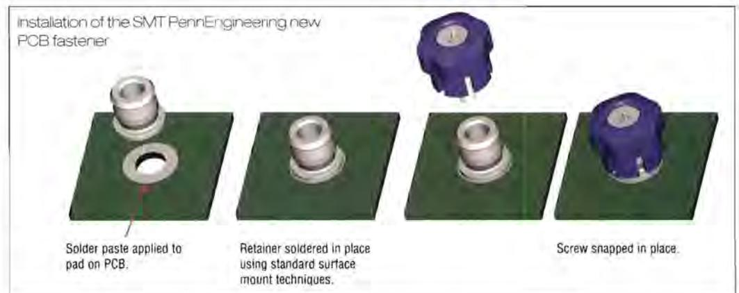
fastener consists of a metal retainer and a plastic cap-and-screw that is snapped into place by hand, it may prove labour intensive. "The alternative – broaching fasteners – are even more labour intensive," said Mark O'Reilly, business development director at Arconix, a UK-based division of PennEngineering. "This year,
