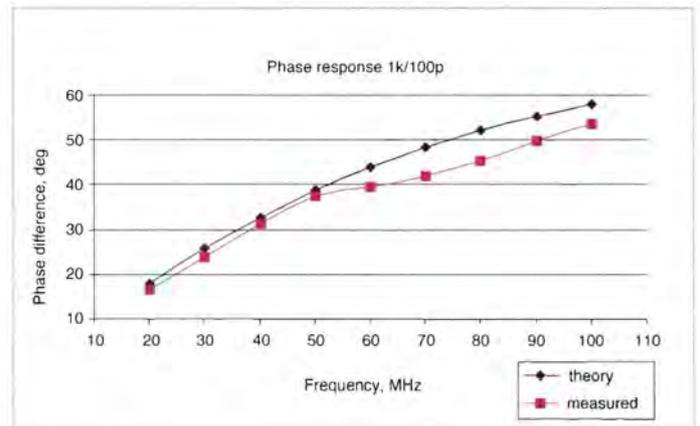
Figure 9b: Experimental results with a simple 1st order filter set-up with attenuators 20dB/20dB
