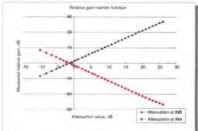
**Figure 8:** Measurement results for the magnitude ratio with the set-up from Figure 6
