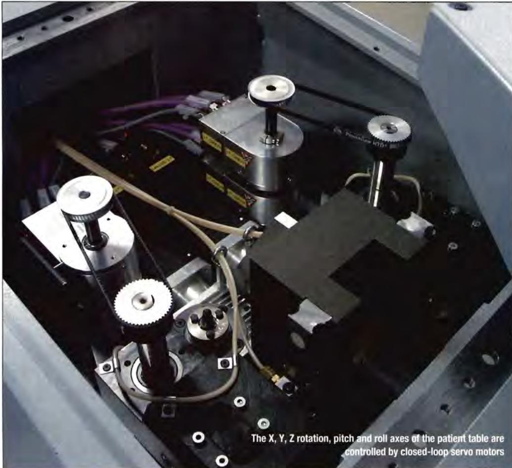
The X, Y, Z rotation, pitch and roll axes of the patient table are controlled by closed-loop servo motors
