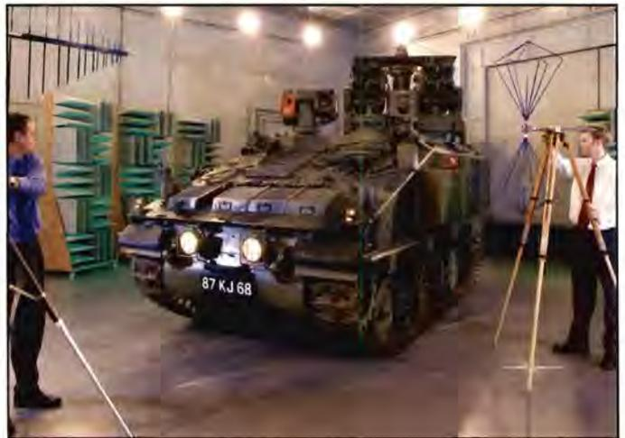
UK-based test and certification company TRL Compliance has opened a new 18x14x6m EMC test facility in Malvern, the UK. This is a large size chamber, which could easily accommodate large military, agricultural and industrial vehicles and equipment.
