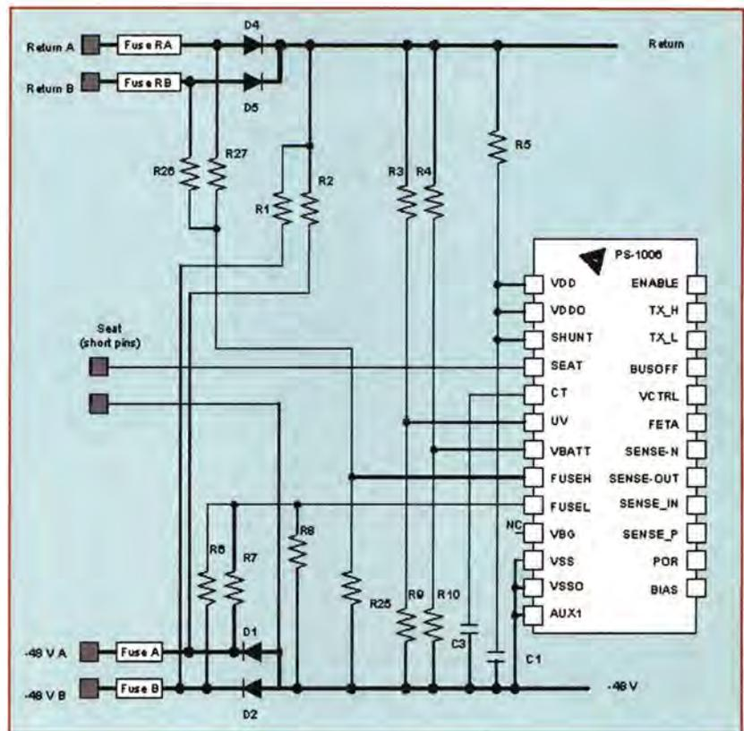
**Figure 4:** Primary side voltage and fuse monitor
