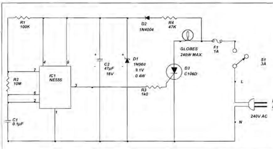
The power source for IC1 is fed from the AC mains via resistor R4 and rectifier diode D2. Zener diode D1 is used to maintain a stable 9V DC while capacitor C2 smoothes out the low level 50Hz ripple.
