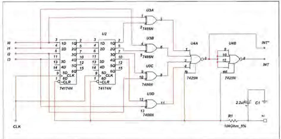
ages are wired to logic high through a 10kΩ resistor. The 2.2mF capacitor should be a tantalum type and serves to bypass power supply glitches from accidentally resetting the D latches.
