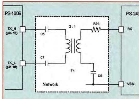
**Figure 6:** Communication link components
