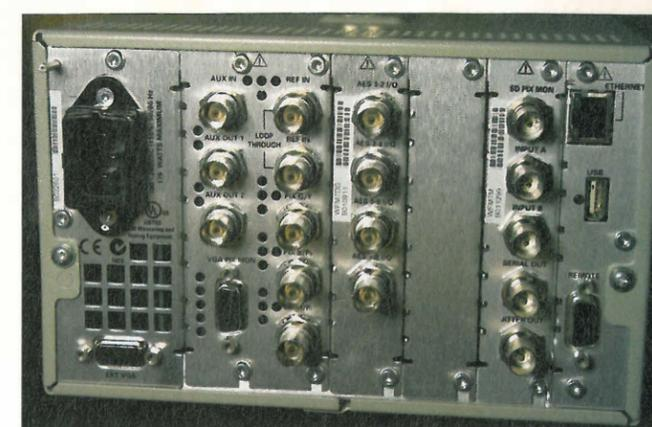
Figure 1: Optional modules may be plugged in at the rear of the unit. This example has additional inputs for AES digital audio.
