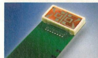
Antenova, the Cambridge-based developer of high-dielectric antennas, has created a drop-in antenna module for mobile phones that offers higher efficiency under torque and an improved specific absorption rate (SAR).
