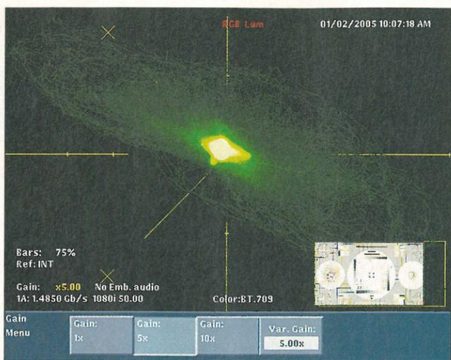
**Figure 4:** Magnified view of vectorscope display, showing a correctly white-balanced camera.
