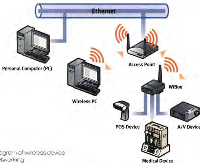
Diagram of wireless device networking
