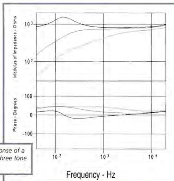
**Figure 6:** Response of a microphone - three tone settings
