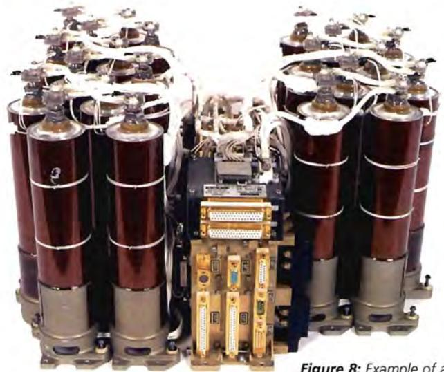
Figure 8: Example of a Li-ion battery for a GEO satellite
