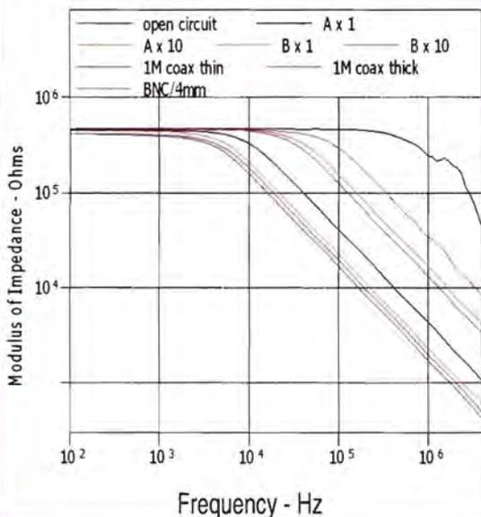
**Figure 9:** Scope probe impedance
