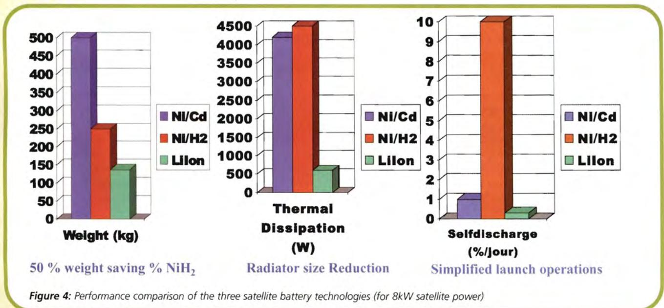
Figure 4: Performance comparison of the three satellite battery technologies (for 8kW satellite power)
