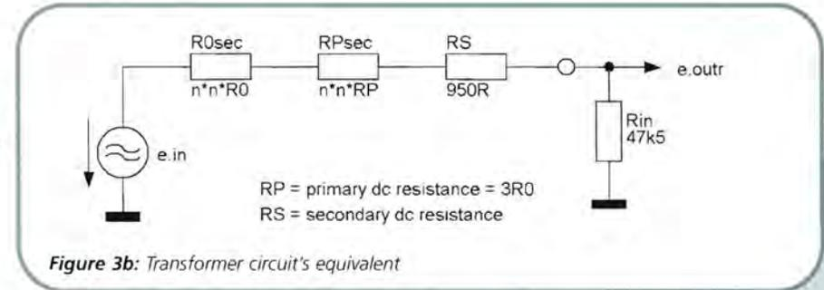
Figure 3b: Transformer circuit's equivalent
