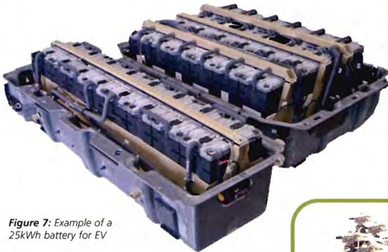
Figure 7: Example of a 25kWh battery for EV
