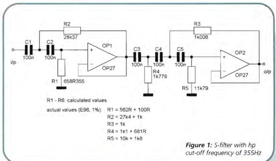
Figure 1: S-filter with hp cut-off frequency of 355Hz
