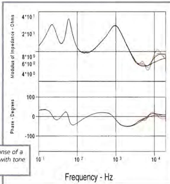
**Figure 5:** Response of a studio monitor with tone control
