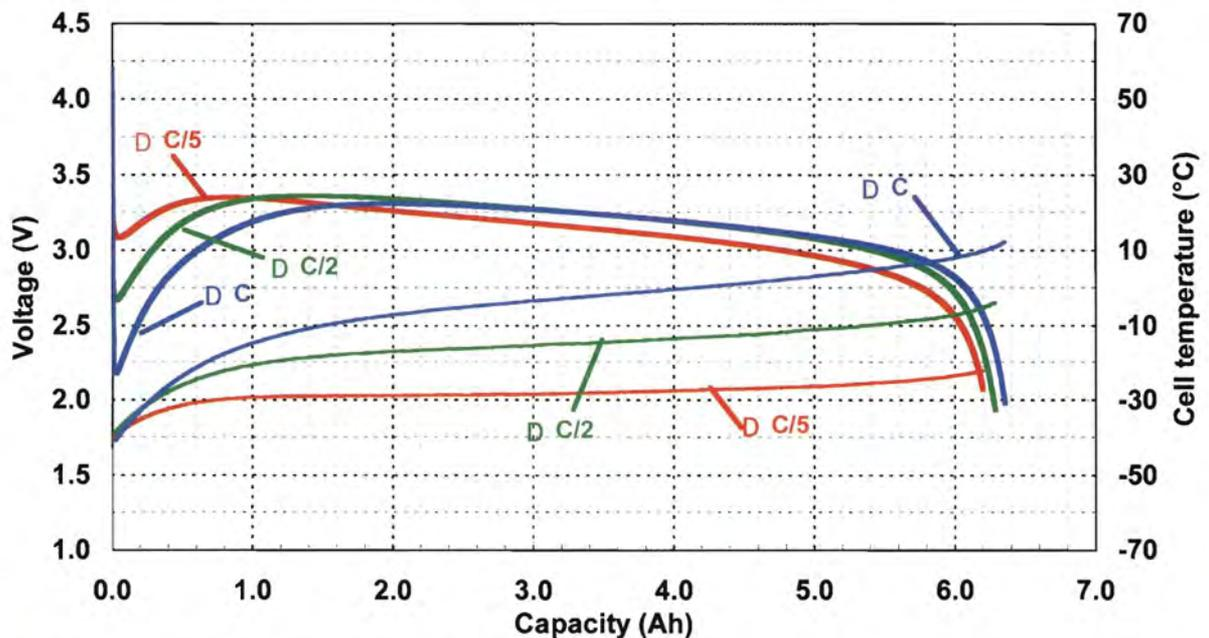
Figure 9: Discharge voltage profile of Saft MP cell at low temperatures
