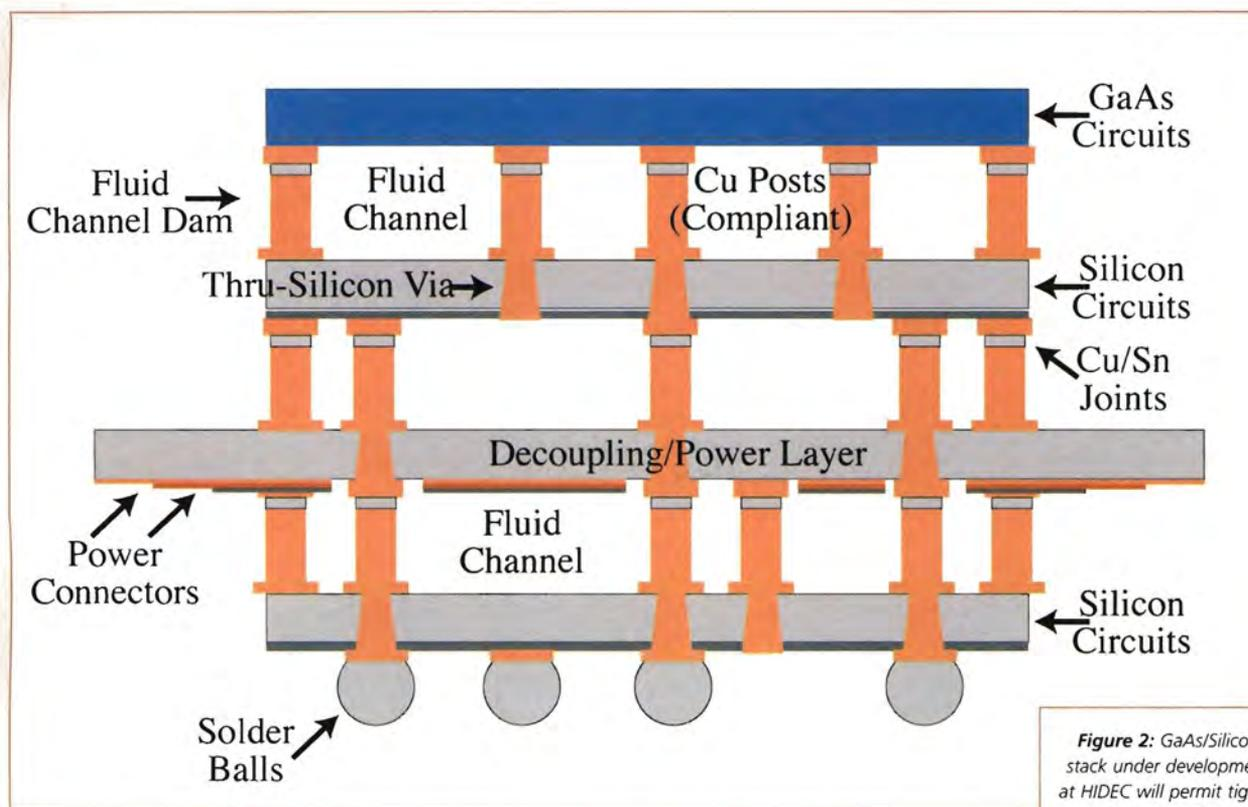
**Figure 2:** GaAs/Silicon stack under development at HIDEC will permit tightly packed I/Os, very high speed and a high level of compliance
