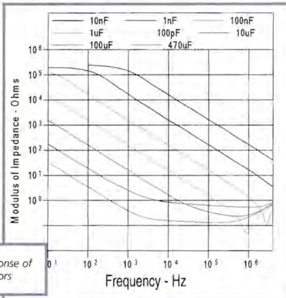
**Figure 10:** Response of different capacitors
