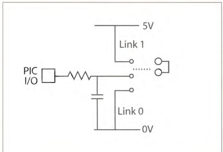
depending on the I/O output voltage allowing the "not connected" state. Software should check the "not connected" state first by driving I/O high, reading 1 and driving I/O low and reading 0. The "Link 1" and "Link 0" states are read directly.
