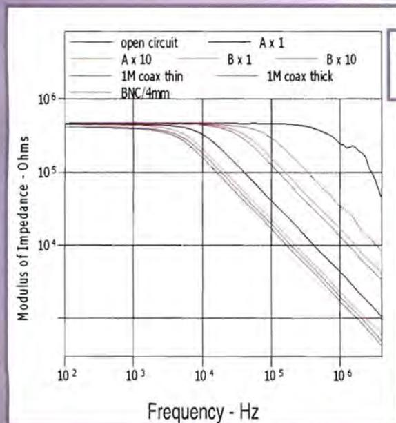
**Figure 9:** Scope probe impedance
