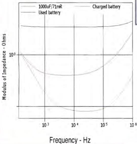
**Figure 8:** Battery impedance; two Ni-MH AA cells
