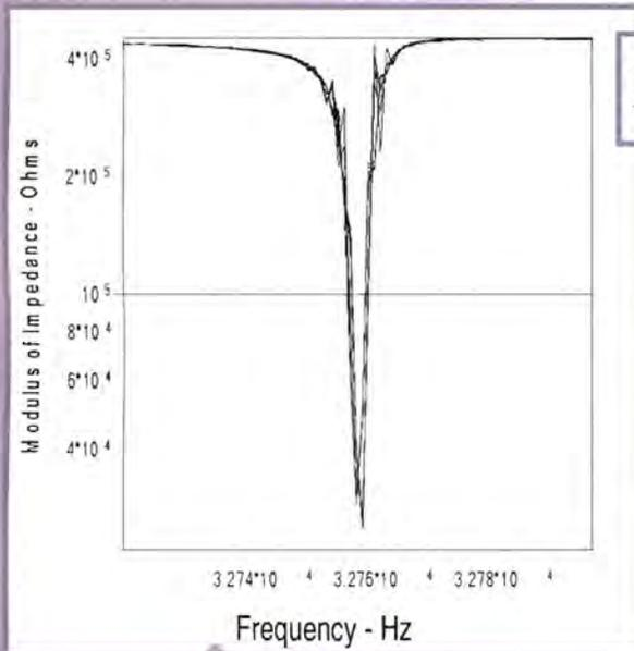
**Figure 3:** Response of a 32768Hz crystal
