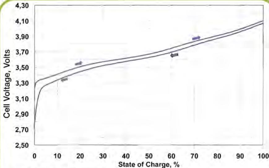
**Figure 2:** Typical Li-ion voltage profile (LiNixCoyAlzO<sub>2</sub>/graphite system). Charge/discharge curves at low rate
