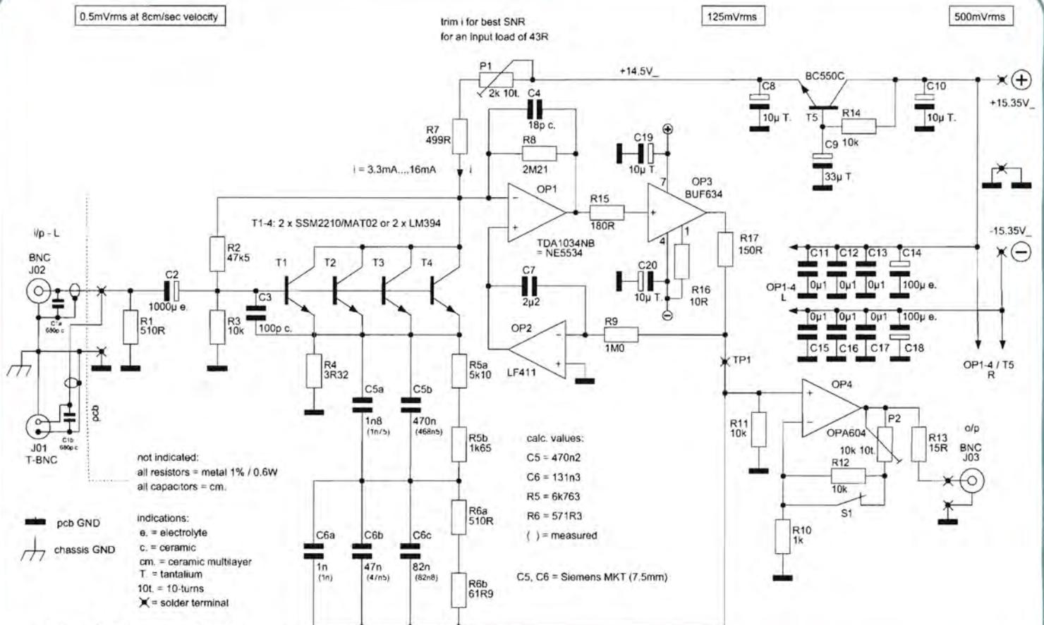
very low source resistances. But for a source resistance of 43R, a device with  $R_B$  of only 4R0 and  $h_{FE} = 40$  (BFW16A), is not able to beat the SN ratios of BJTs with higher  $R_B$  and much higher  $h_{FE}$  (see Table 2, column G). It's hard to find a lowest- $R_B$  transistor with  $h_{FE} \gg 40$ . The latter is essential for low input noise currents. Basically, the (base) input noise current  $i_N$  of any BJT can be calculated as follows:
