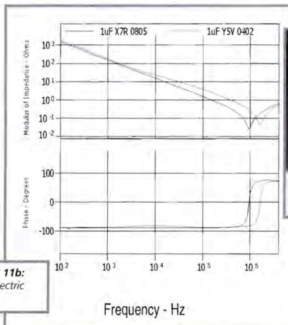
**Figure 11a and 11b:** Response of dielectric capacitors
