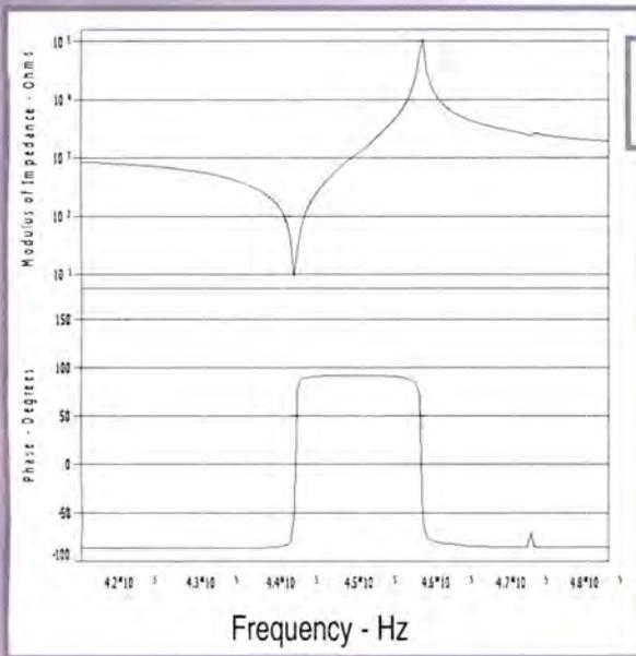
**Figure 2:** Complex response of a 455kHz resonator
