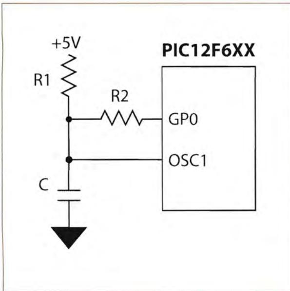
1. After reset I/O pin is High-Z
