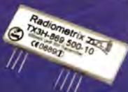
The TX3H-869-10 is a FM transmitter module with a power output of 450mW nominal. The module operates on European 869.40 - 869.65MHz sub-band allocation for 500mW and is designed for applications requiring operating range in excess of 3km or it can be used when space or ergonomic limitations dictate the use of small and inefficient antennas.
