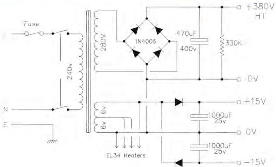
Figure 1: Hot audio amp power supply
