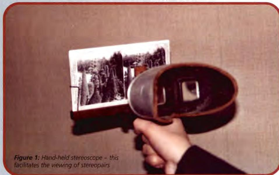
**Figure 1:** Hand-held stereoscope – this facilitates the viewing of stereopairs
