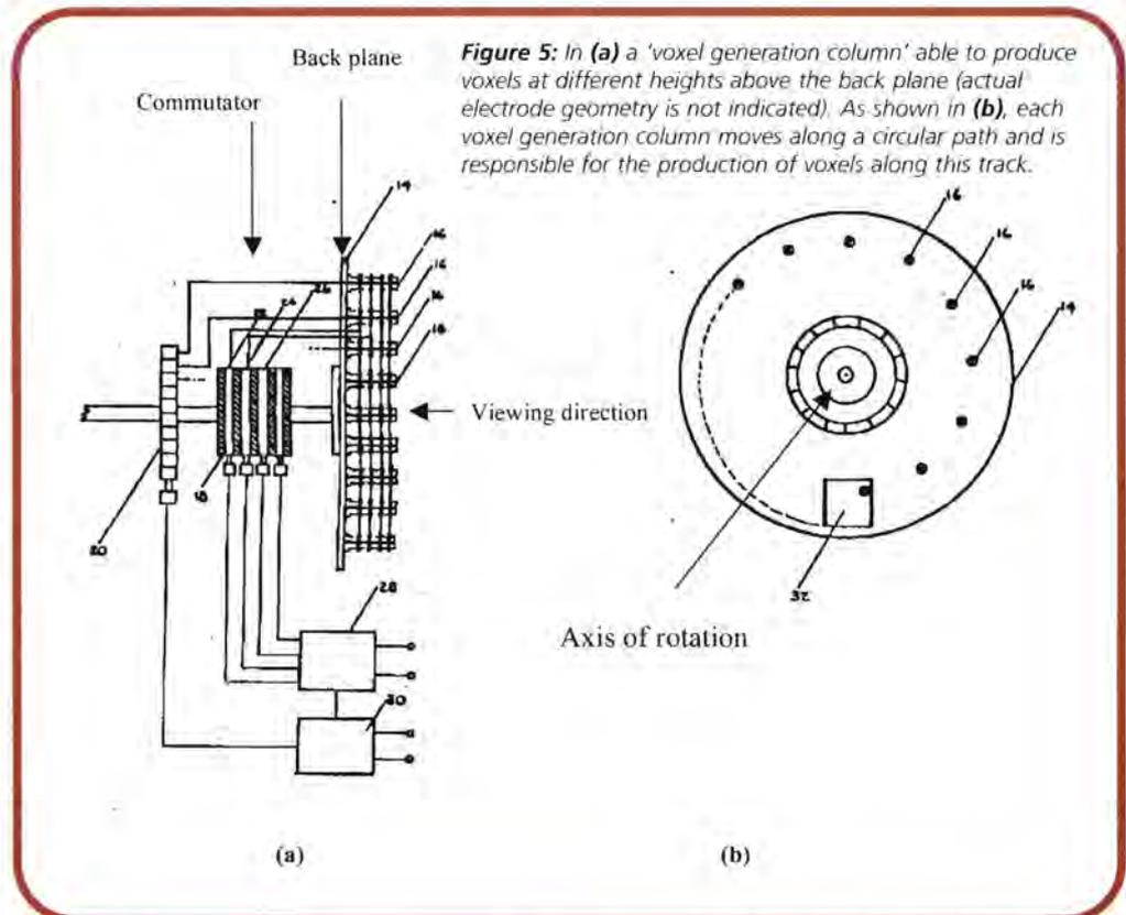
**Figure 5:** In (a) a 'voxel generation column' able to produce voxels at different heights above the back plane (actual electrode geometry is not indicated). As shown in (b), each voxel generation column moves along a circular path and is responsible for the production of voxels along this track.
