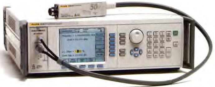
*The Fluke 9640A comes with a 50Ω levelling head and has an option to add a 75Ω head, which extends the instrument's capability to calibrate workloads with 50Ω and 75Ω inputs*
