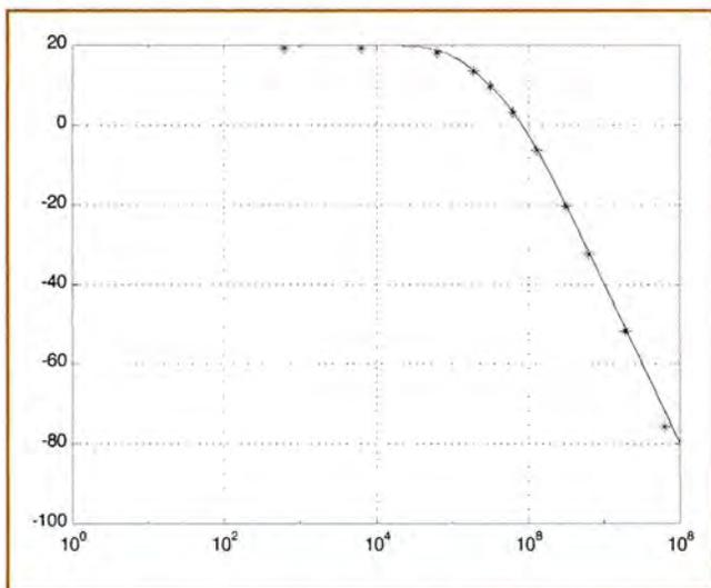
Figure 4: Calculated ( \_\_\_\_\_ ) and simulated ( \*\*) lowpass filter
