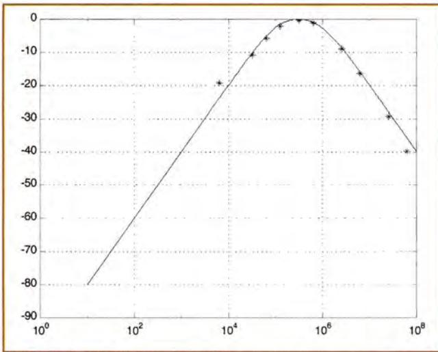
Figure 2: Calculated ( \_\_\_\_\_ ) and simulated ( \*\*) bandpass filter
