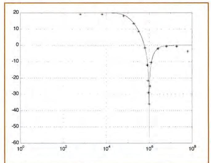
Figure 5: Calculated ( \_\_\_\_\_ ) and simulated ( \*\*) lowpass notch filter
