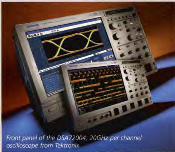
Front panel of the DSA72004, 20GHz per channel oscilloscope from Tektronix
