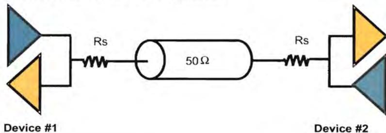
Figure 12: Termination in multi-drop bi-directional buses
