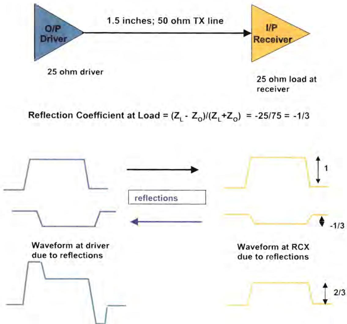
**Figure 3:** Reflections that can occur in a transmission line
