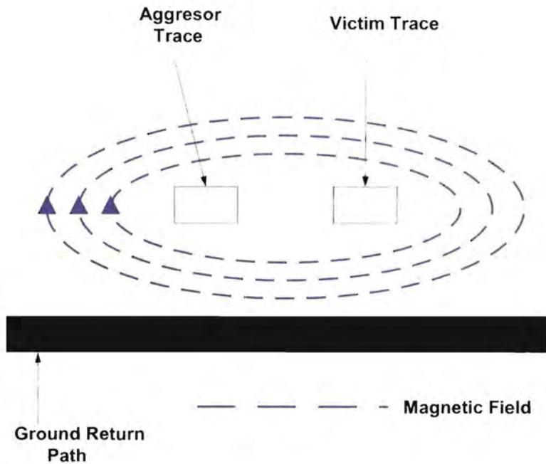
**Figure 4:** Interference caused by two adjacent transmission lines
