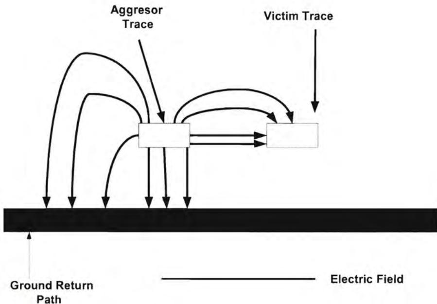
must find a path around the hole, thus increasing the loop size and degrading signal quality and increasing EMI. This is why ground and power planes should be kept as solid as possible. Also, the current return path of signals that cross between routing layers that use different reference planes can result in the formation of large loops. This should be avoided as much as possible.
