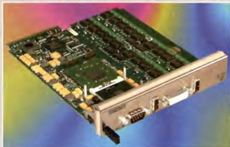
combines server-class memory and I/O controller functions into a single component.
