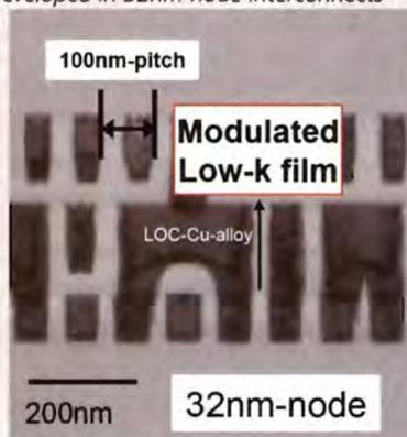
A new low-k dielectric technology based on a plasma co-polymerisation technique has led to the development of the first 32nm node multilayer interconnect for large scale integrated circuits (LSIs). In advanced LSI devices, the number of interconnects between transistors increases with device complexity, while the amount of space between interconnects decreases owing to miniaturisation. The resulting line
