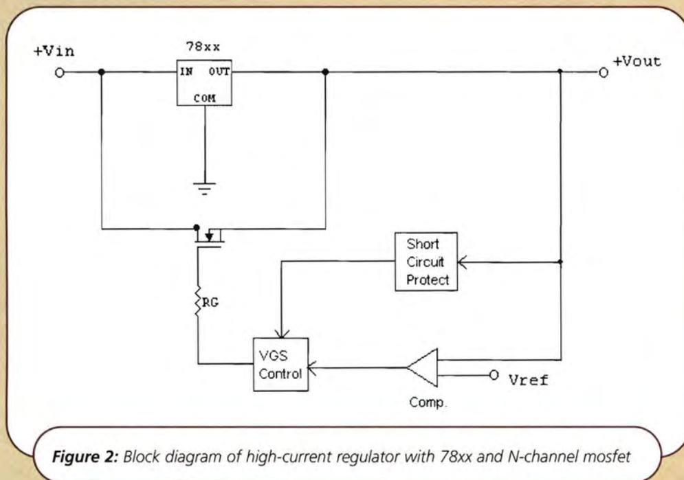
**Figure 2:** Block diagram of high-current regulator with 78xx and N-channel mosfet
