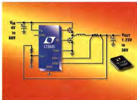
1.23V to 36V at load currents up to 20A. Applications include 12V and 42V automotive, 48V telecom supplies, heavy equipment systems, avionics, industrial controls and distributed power systems.
