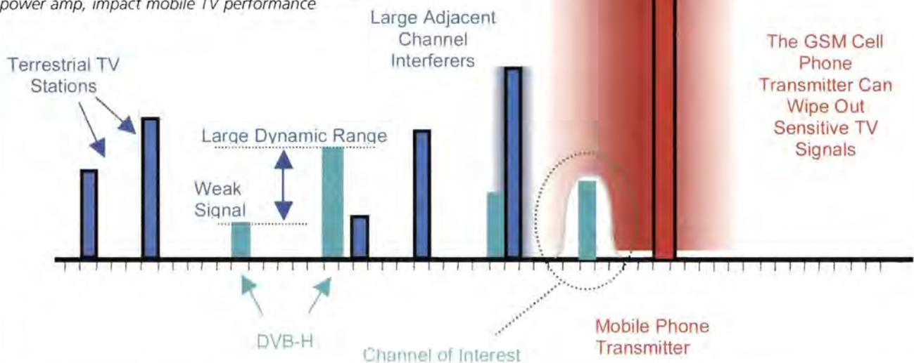
Television (DVB-T) open industry standard for digital broadcasting, DVB-H uses time slicing, modulation techniques and error correction to overcome issues of power and interference.
