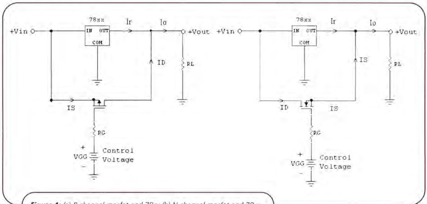
Figure 1: (a) P-channel mosfet and 78xx (b) N-channel mosfet and 78xx
