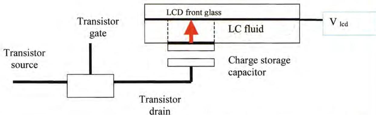
*Basic structure of the active matrix TFI LCG unit*
