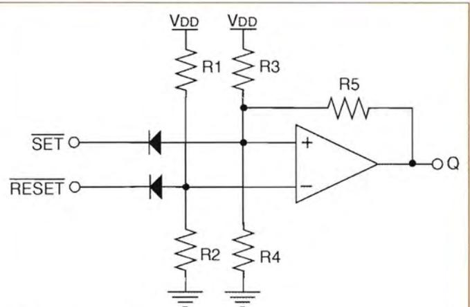
Figure 7: Set/reset flip-flop
