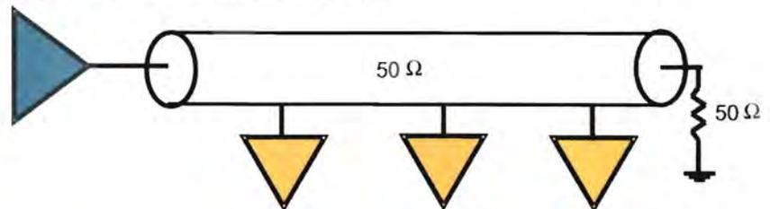
Figure 11: Series termination in a bi-directional bus
