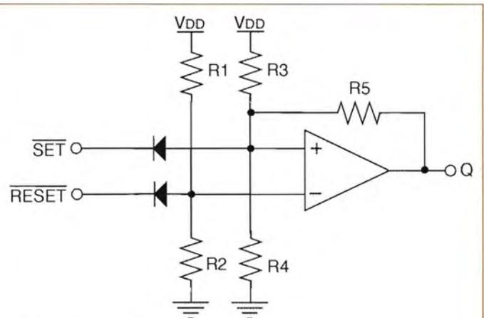
Figure 7: Set/reset flip-flop
