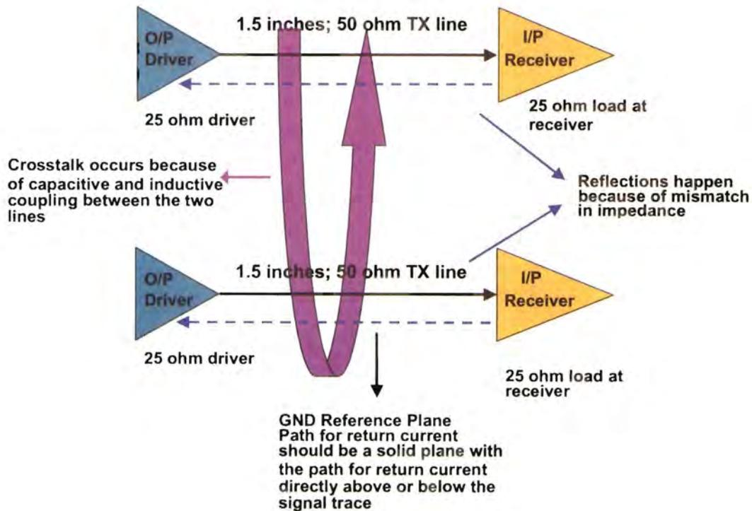
to the impedance of the transmission line changing. When a driver launches a signal onto a transmission line, the initial voltage will propagate down the line until it reaches the end. If the end of the line exhibits impedance different to the impedance of the transmission line, a portion of the signal will be reflected back down the transmission line toward the source. The amount of the signal that is reflected back is determined by the reflection coefficient as described in the equation below.
