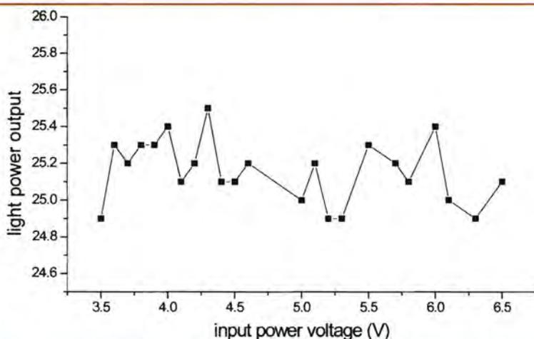
Figure 6: The relationship between light power output of LED and input power
