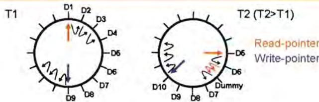
Figure 11: Ring buffer FIFO with read pointer catching up over time, clock correction active
