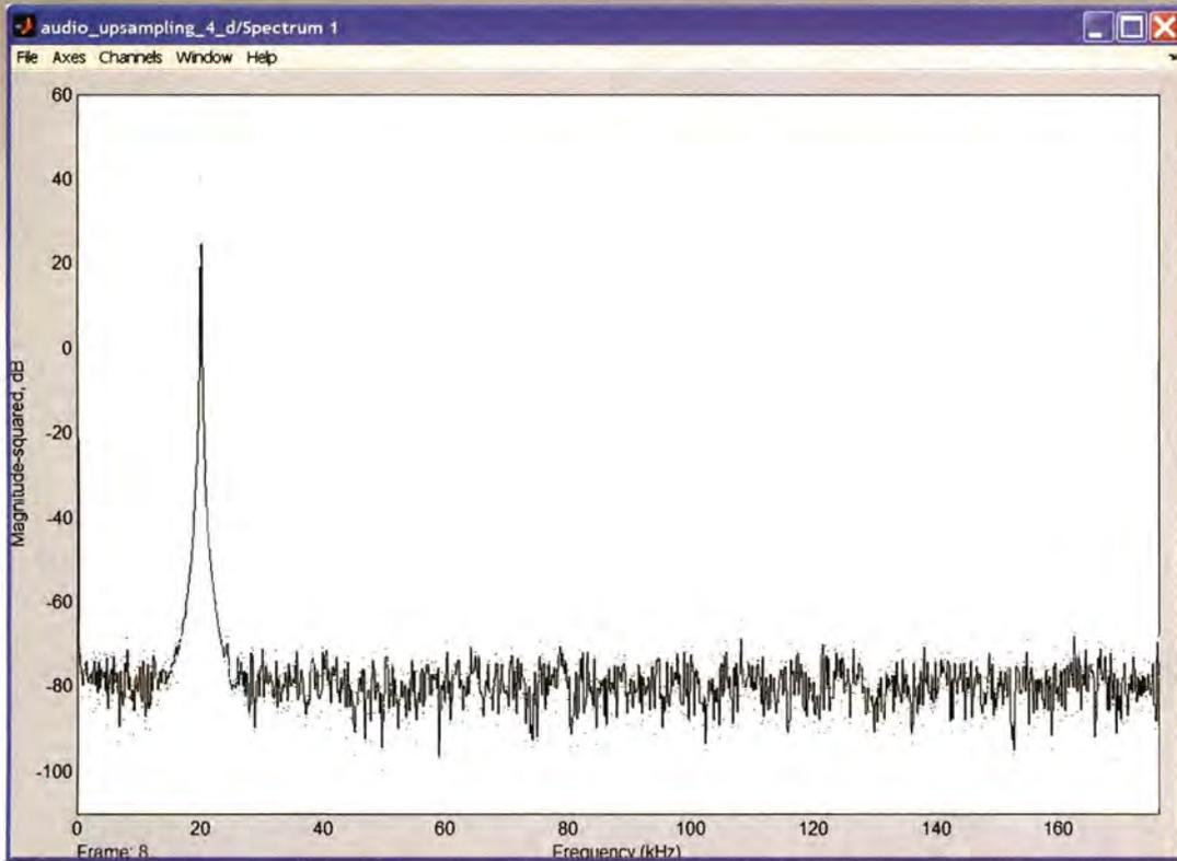
**Figure 4:** Signal-to-noise ratio > 100dB. The algorithm meets all quality requirements for implementing audio sampling frequencies
