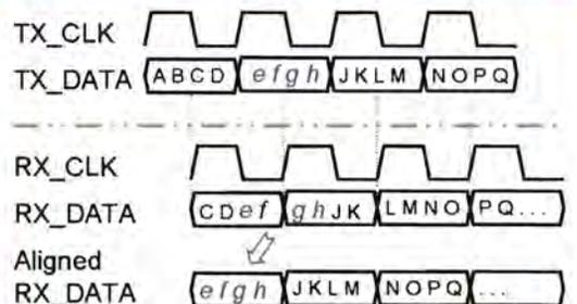
Figure 8: Alignment of data to explicit bit-patterns
