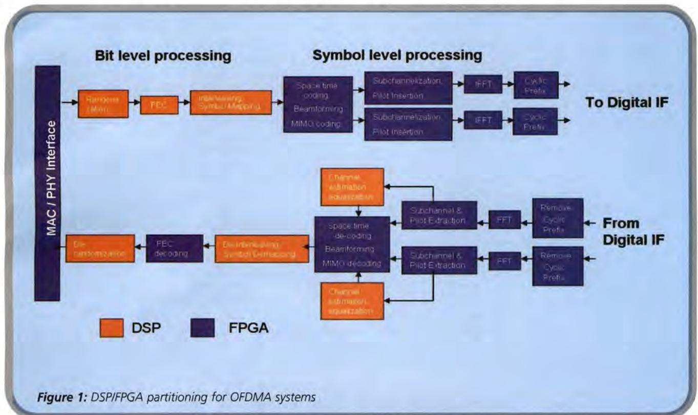
Figure 1: DSP/FPGA partitioning for OFDMA systems
