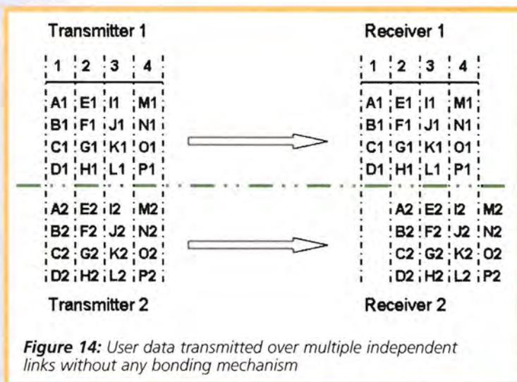
**Figure 14:** User data transmitted over multiple independent links without any bonding mechanism
