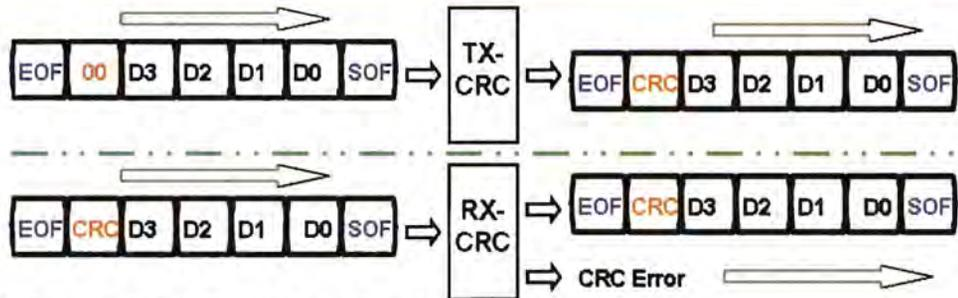
Figure 12: Functionality of CRC inserter and checker
