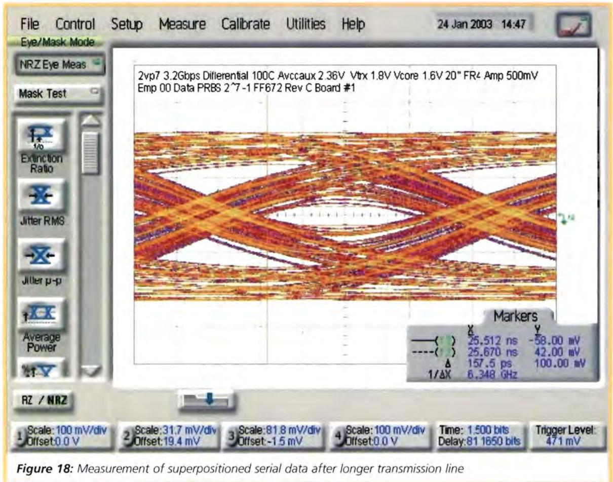
**Figure 18:** Measurement of superpositioned serial data after longer transmission line
