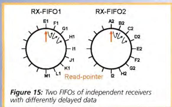
**Figure 15:** Two FIFOs of independent receivers with differently delayed data
