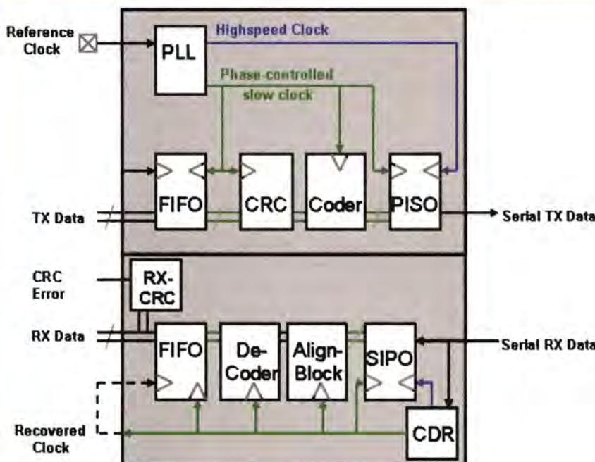
Figure 13: Block diagram with CRC added on TX and RX
