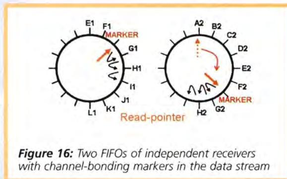
**Figure 16:** Two FIFOs of independent receivers with channel-bonding markers in the data stream
