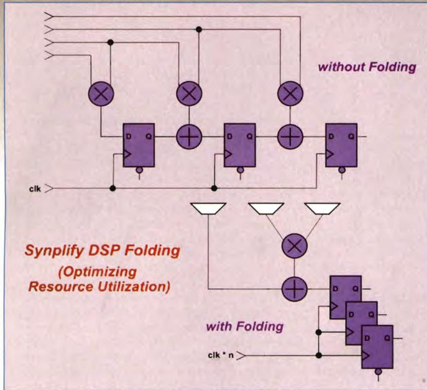
**Figure 6:** The FPGA resources required can be reduced dramatically by using the folding feature
