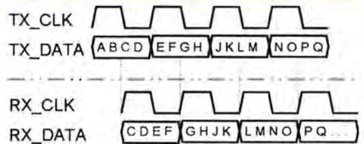
Figure 7: Raw unaligned data, directly after the de-serialiser
