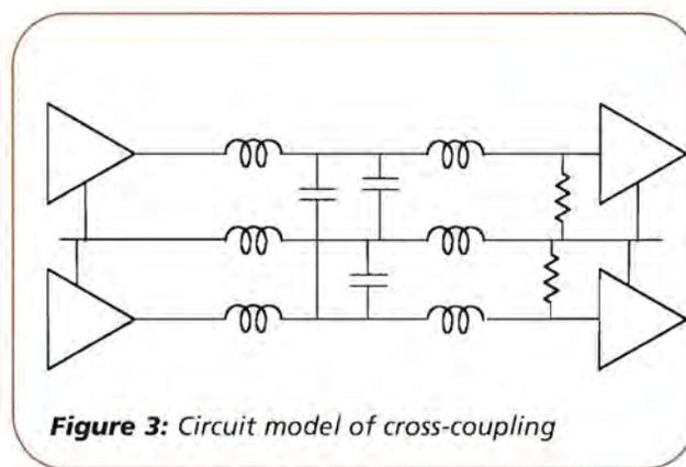
**Figure 3:** Circuit model of cross-coupling
