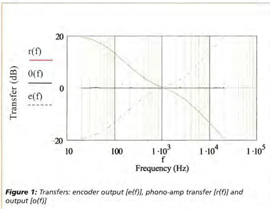
**Figure 1:** Transfers: encoder output  $[e(f)]$ , phono-amp transfer  $[r(f)]$  and output  $[o(f)]$
