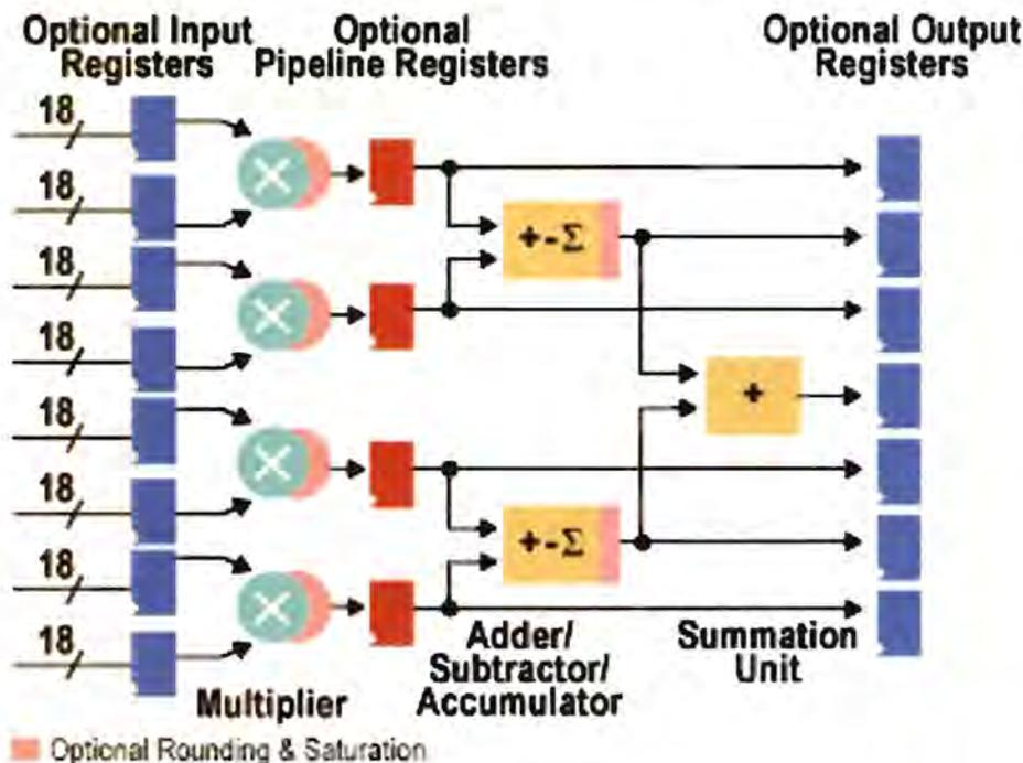
Figure 2: Embedded DSP blocks in FPGAs
