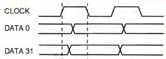
**Figure 2:** Clocking data between devices with central clock
