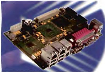
There's a high number of front-mounted I/O connections for reduced cabling and ease of accessibility. The boards include four high-speed USB 2.0 interfaces and two 10/100 BaseT LAN ports among others. For solid state operation, a compact flash socket is also provided. Additional on-board interfaces include two USB 2.0 interfaces, three COM ports, an 8-pin GPIO interface, EIDE, floppy and a Compact Flash socket. System memory of up to 2GB is possible with two DDR SODIMM sockets.
