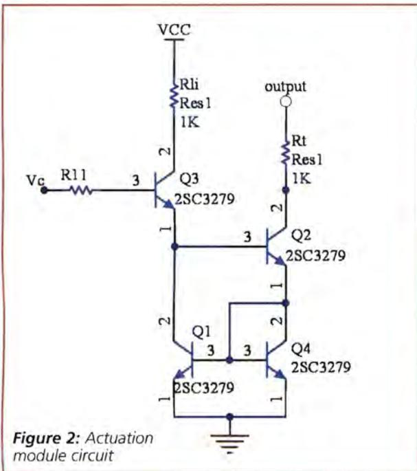
Figure 2: Actuation module circuit
