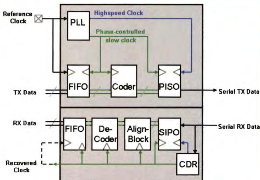
**Figure 10:** Block diagram with RX-FIFO added for phase compensation on recovered clock, routed in fabric
