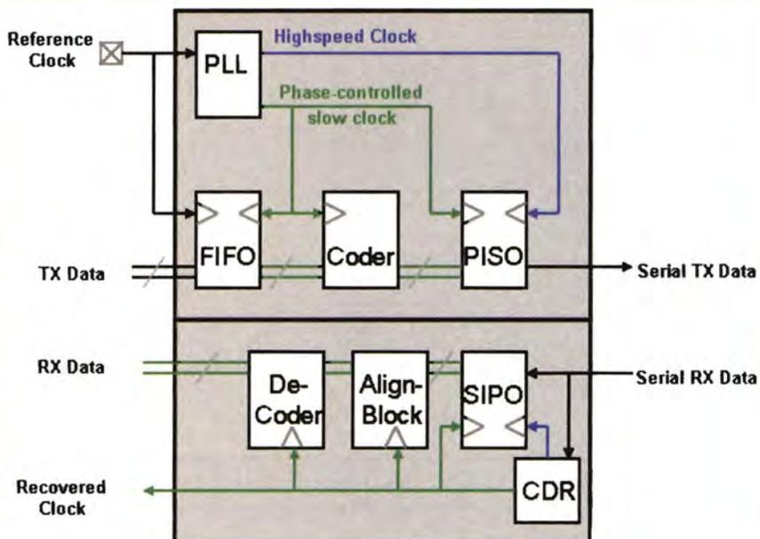
**Figure 9:** Block diagram with an alignment block added to find original word boundaries
