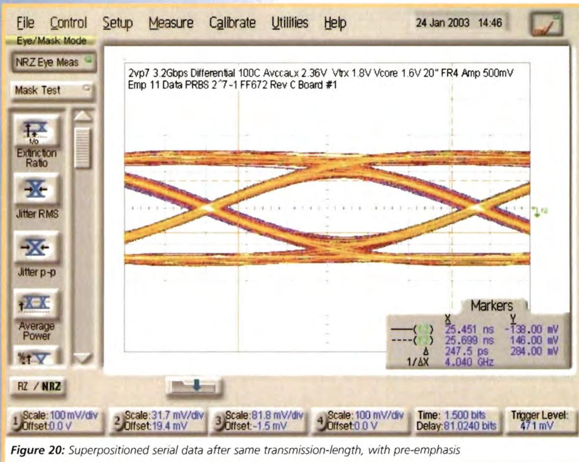
Figure 20: Superpositioned serial data after same transmission-length, with pre-emphasis
