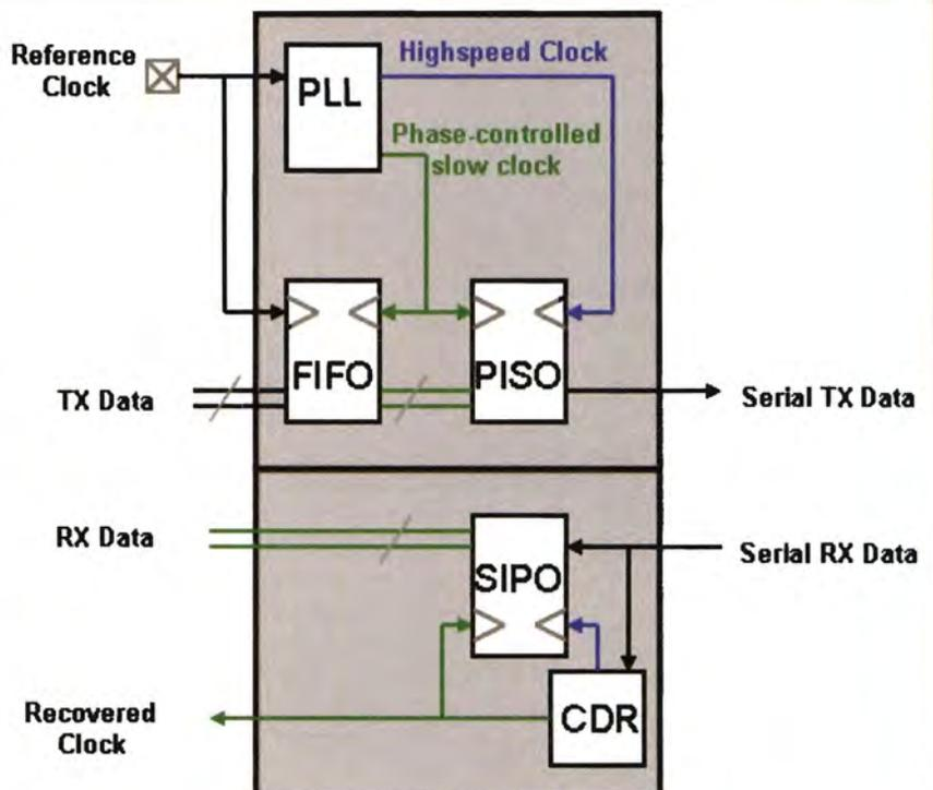
Figure 5: Transceiver with the basic blocks for TX and RX
