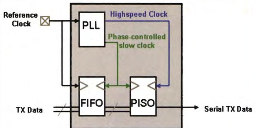
Figure 4: Basic components for serial transmission
