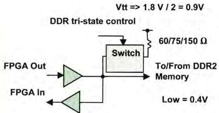
Figure 4: LatticeSC switchable I/O termination
