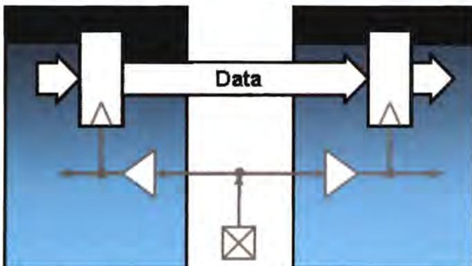
**Figure 1:** System with central clock
