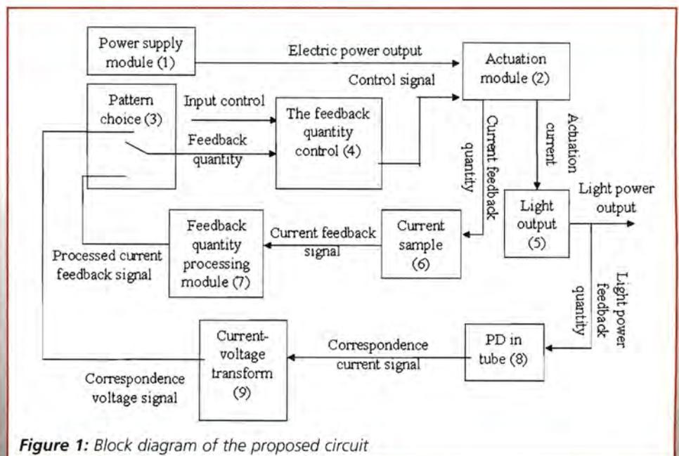
Figure 1: Block diagram of the proposed circuit
