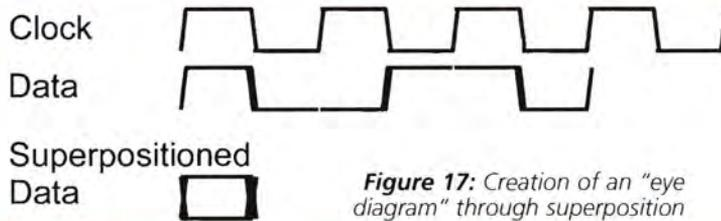
**Figure 17:** Creation of an "eye diagram" through superposition
