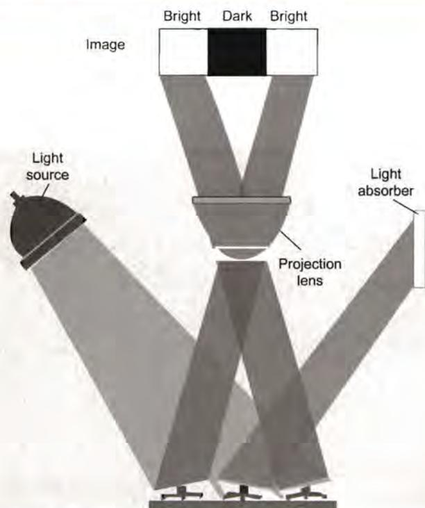
**Figure 1:** The component parts of a simple DLP
