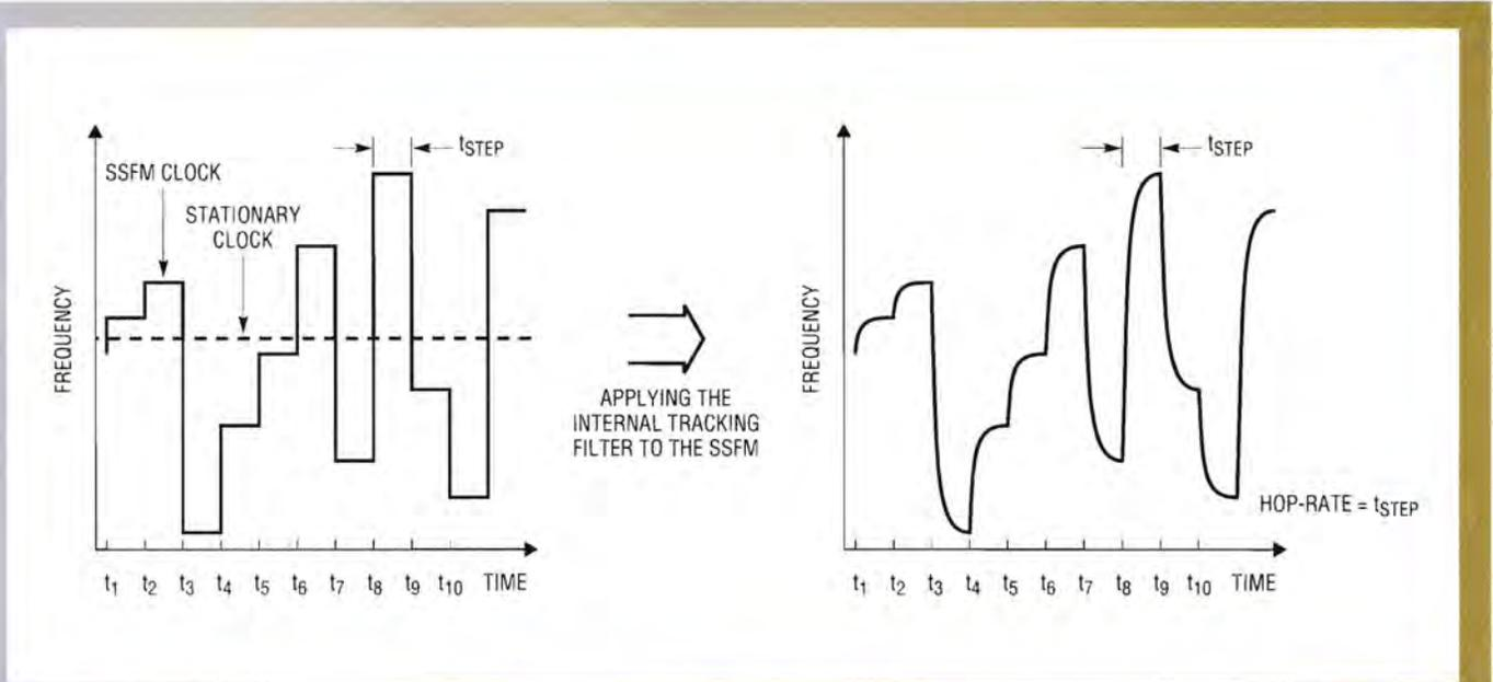
**Figure 2:** Pseudo-random modulation illustrating the effect of the LTC6908 internal tracking filter
