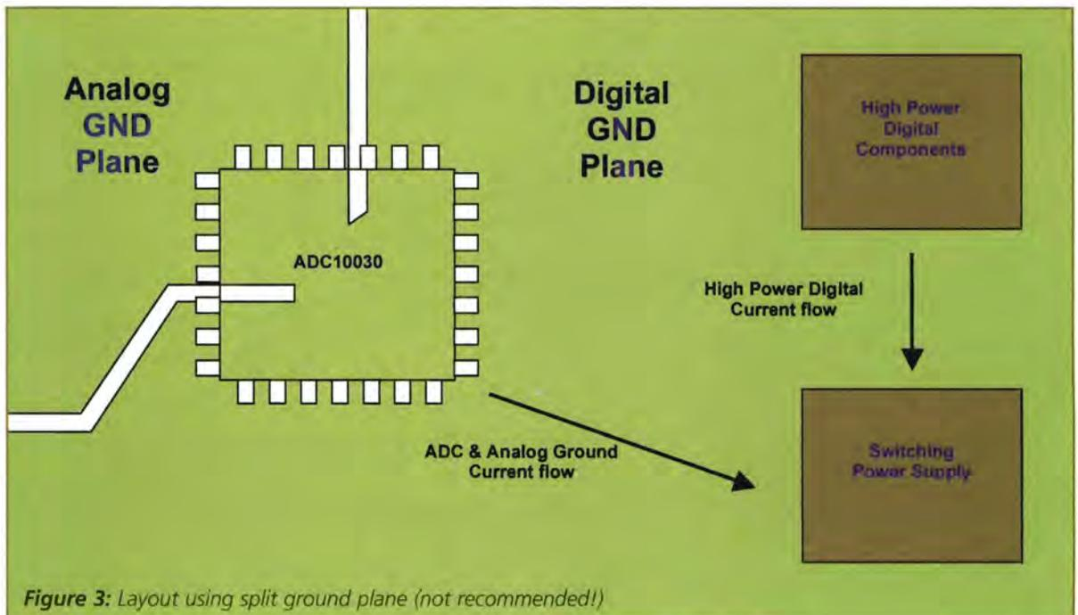
Figure 3: Layout using split ground plane (not recommended!)
