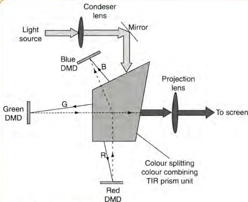
Figure 7: An outline of a three-chip DLP system
