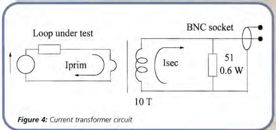
Figure 4: Current transformer circuit
