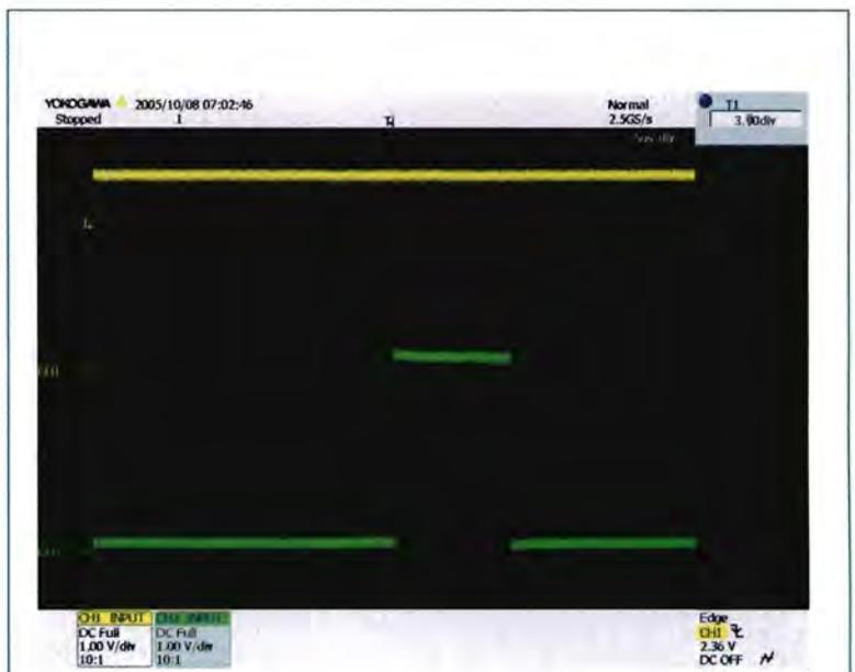
**Figure 2:** Output of the comparator in response to a 8ns pulse at the input. Pulse length is approximately 8 microseconds
