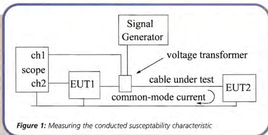
**Figure 1:** Measuring the conducted susceptibility characteristic
