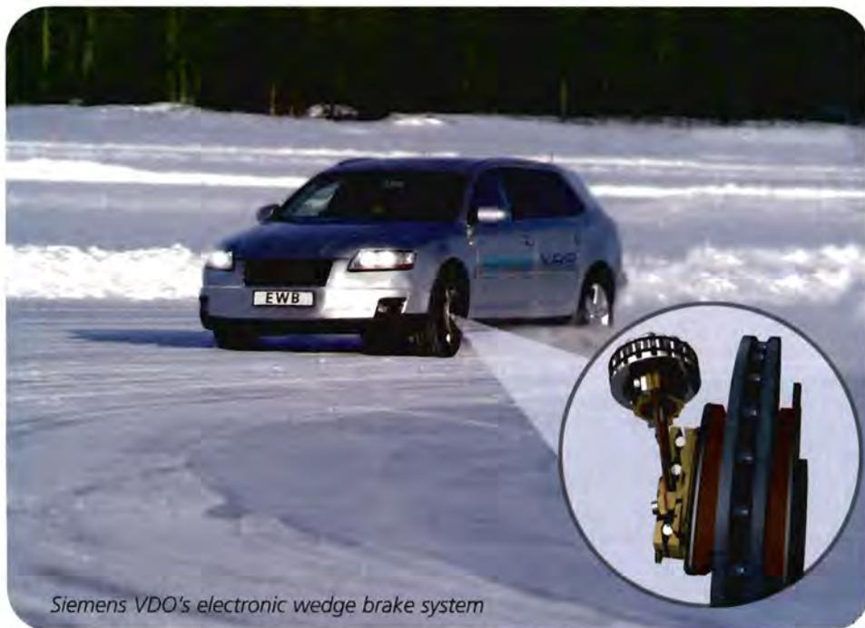
*Siemens VDO's electronic wedge brake system*
