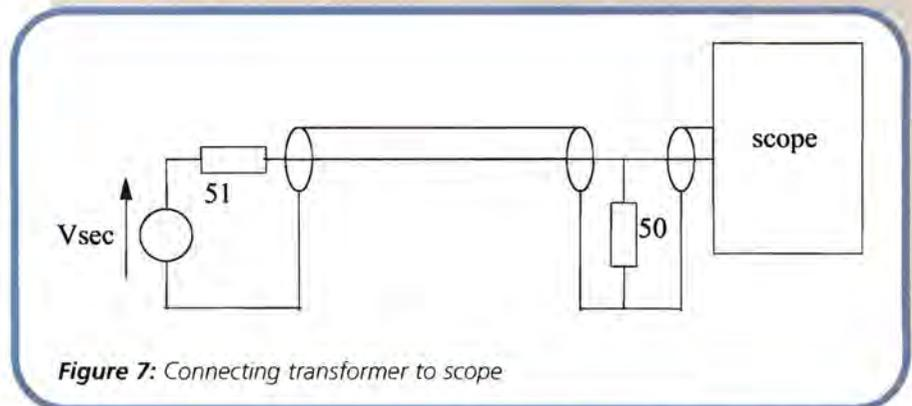
Figure 7: Connecting transformer to scope
