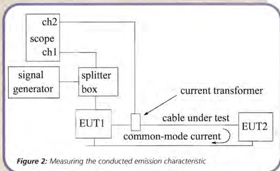
Figure 2: Measuring the conducted emission characteristic
