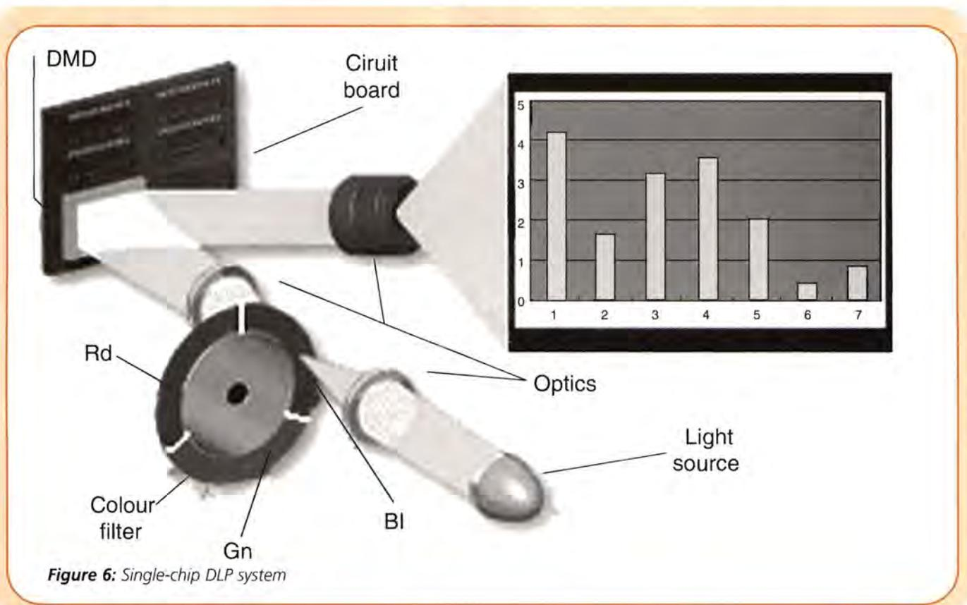
**Figure 6:** Single-chip DLP system
