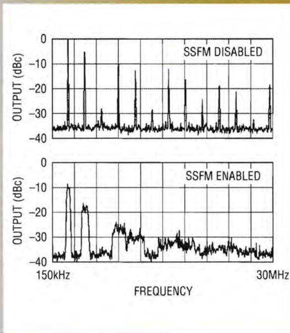
**Figure 4:** Switching regulator output emissions using a 9kHz resolution bandwidth, peak detector (LTC6908)
