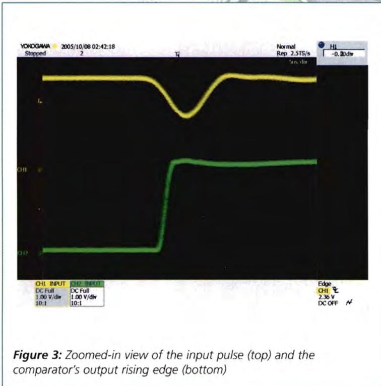
Figure 3: Zoomed-in view of the input pulse (top) and the comparator's output rising edge (bottom)
