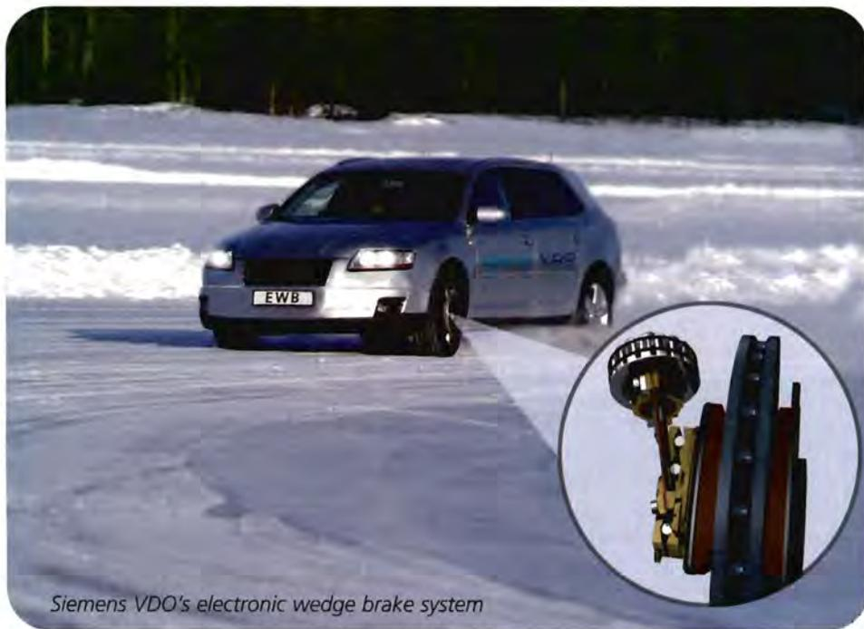
*Siemens VDO's electronic wedge brake system*
