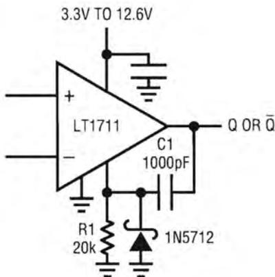
**Figure 1:** A simple one-shot circuit with a high-speed comparator and three external components. Any event that triggers the comparator will cause the output to go high and stay high for a minimum of 2.5 microseconds
