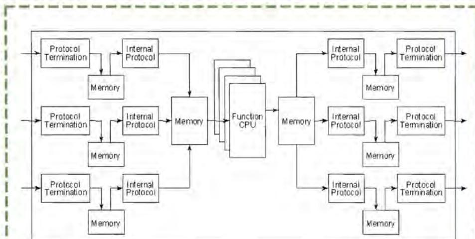
**Figure 1:** Each stage in the data pipeline must either terminate or encapsulate protocols as data passes the boundary into new systems. Each protocol that has to be resolved, however, must be temporarily stored in memory and processed multiple times, leading to increased processing load and latency
